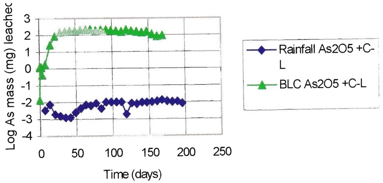
Figure 4.39 – Comparison between the masses of arsenic leached from the column(rainfall) and column (BLC) leaching tests
