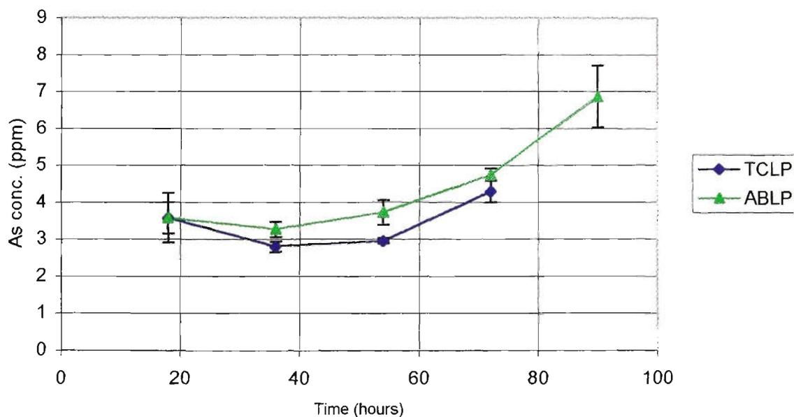
**Figure 3.16 – Similarities between the sequential leaching results obtained using both the TCLP and the ABLP for the  $\text{PbHAsO}_4 + \text{C-Fe}$  formulation**
