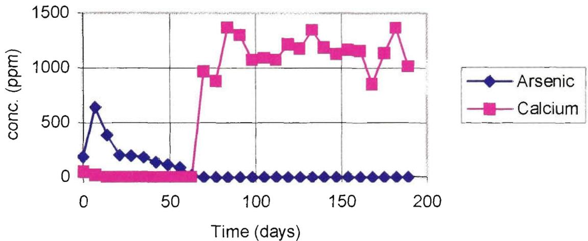
**Figure 4.29 - Arsenic and calcium levels leached using column (rainfall) leaching,  $\text{Na}_2\text{HAsO}_4 + \text{C-L}$  formulation**
