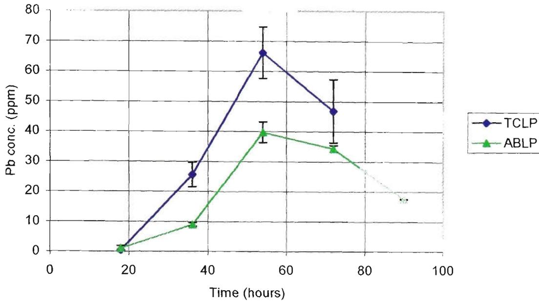
**Figure 3.20 – Similarities between the lead sequential leaching results obtained using both the TCLP and the ABLP for the  $\text{PbHAsO}_4 + \text{C-L}$  formulation**
