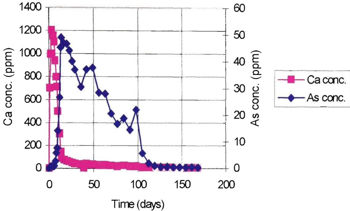
Figure 4.6 – Relationship between the calcium and arsenic concentrations for the  $\text{As}_2\text{O}_5 + \text{C}$  formulation
