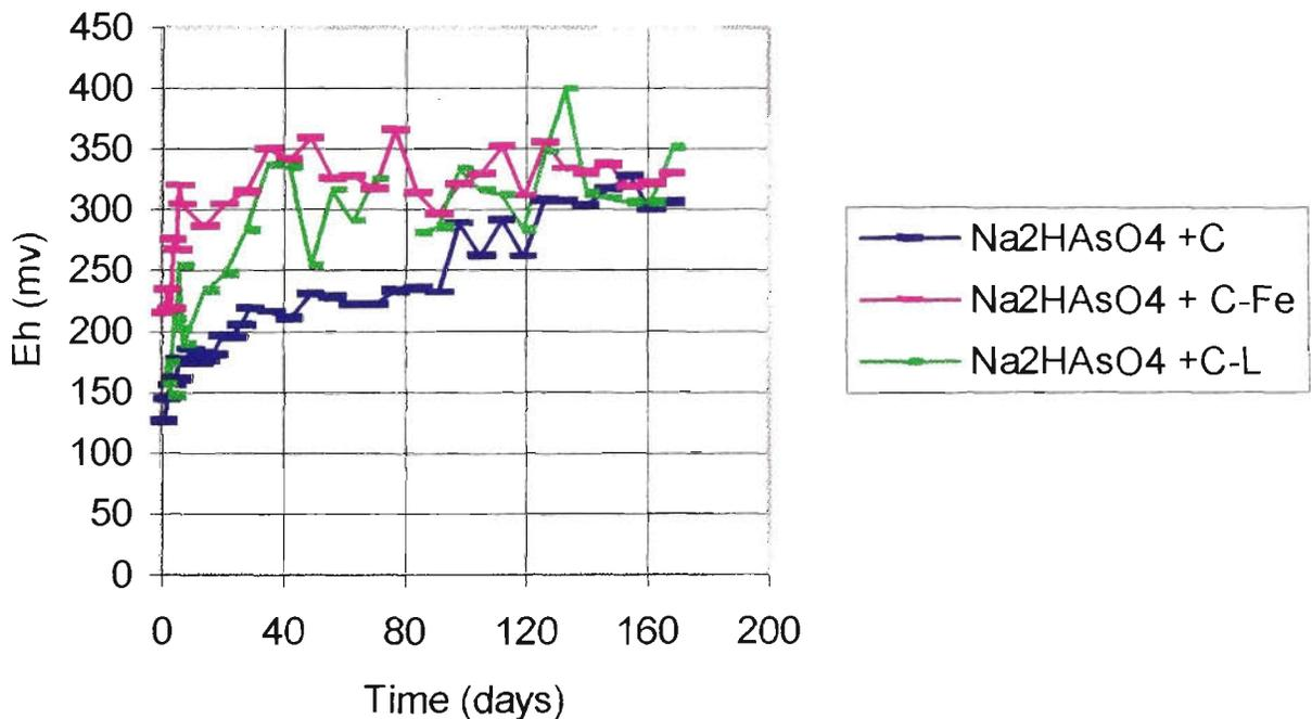
Figure 4.66 - Redox potential recorded for the sodium arsenite formulations, Column (BLC) leaching
