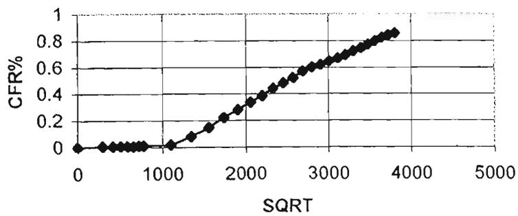
Figure 4.13 – CFR versus SQRT for the arsenic pentoxide S/S formulations
