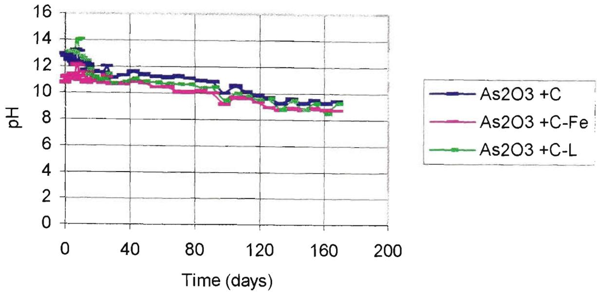
Figure 4.58 - pH values recorded for the arsenic pentoxide leachates collected from the column (BLC) leaching tests
