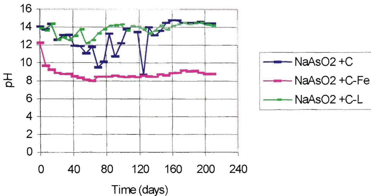
**Figure 4.62 - pH values recorded for the arsenic trioxide leachates collected from the column (Rainfall) leaching tests**
