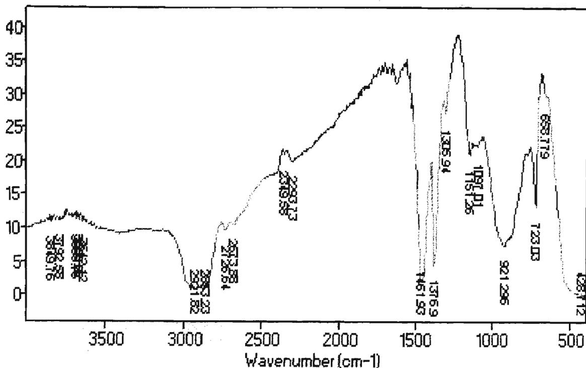
Figure 5.1 – FTIR spectrum of hydrated cement
