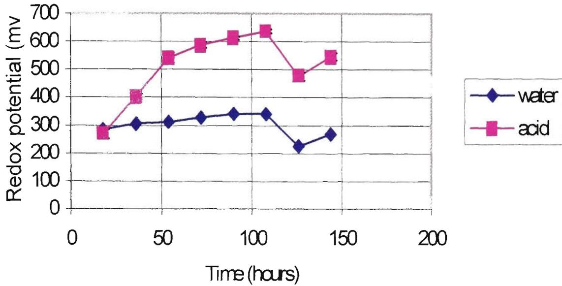
Figure 3.68 – Redox potentials of the  $\text{Na}_2\text{HAsO}_4 + \text{C-Fe}$  formulations when leached with deionized water or the acidic leachant
