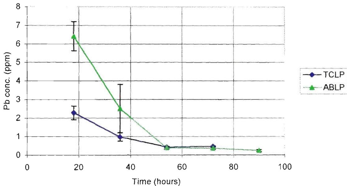
**Figure 3.19 – Similarities between the lead sequential leaching results obtained using both the TCLP and the ABLP for the  $\text{PbHAsO}_4 + \text{C-Fe}$  formulation**
