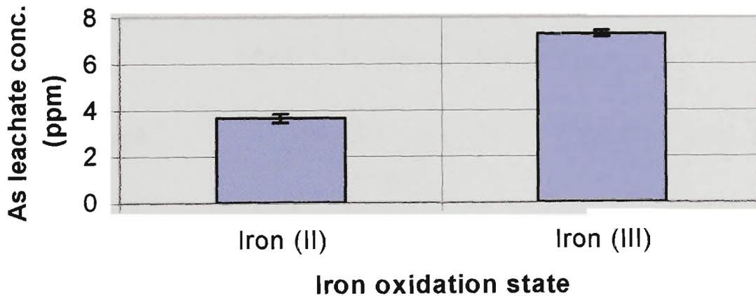
**Figure 3.50 - ABLP arsenic leachate concentrations from the [cement + iron] stabilization of sodium arsenate using the acidic leachant**
