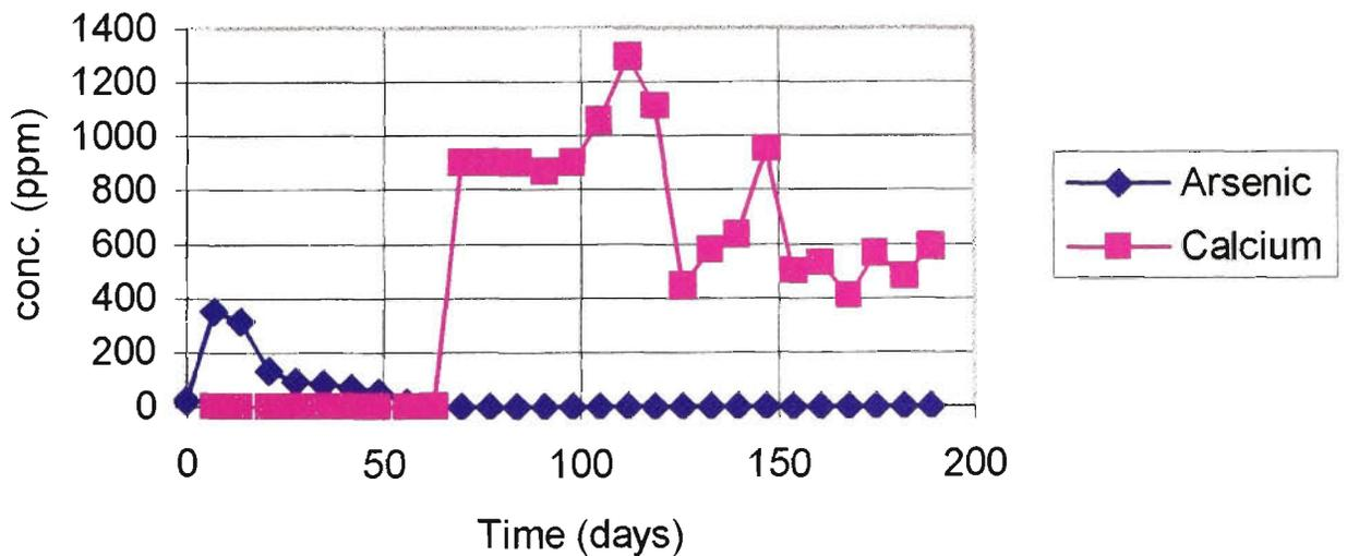
Figure 4.30 - Arsenic and calcium levels leached using column (rainfall) leaching,  $\text{Na}_2\text{HAsO}_4$  + C-Fe formulation
