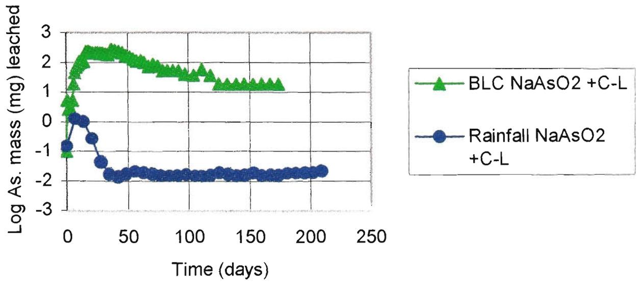
Figure 4.40 – Comparison between the masses of arsenic leached from the column (rainfall) and column (BLC) leaching tests
