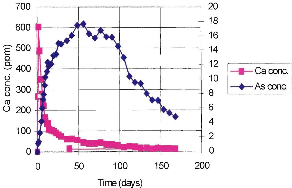
Figure 4.5 – Relationship between the calcium and arsenic concentrations for the  $\text{As}_2\text{O}_3 + \text{C-L}$  formulation
