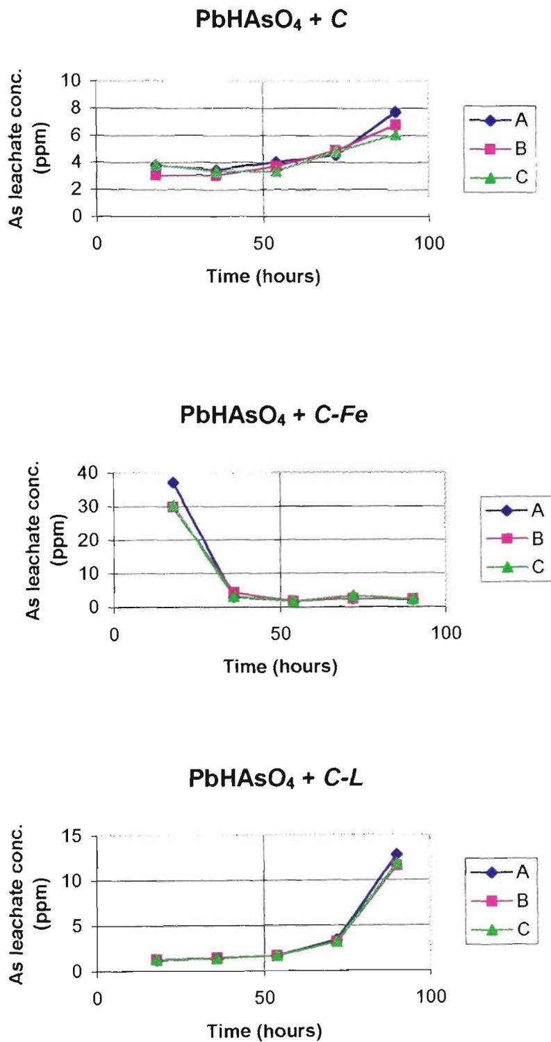
Figure 3.28 – Precision of the Sequential leaching (acid) tests and the Lead Arsenate formulations (Lead concentrations)
