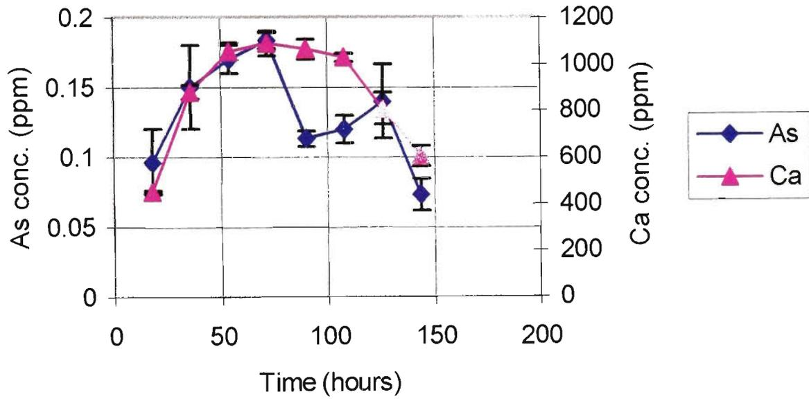
**Figure 3.41 – Relationship between Calcium and Arsenic levels in the sequential leaching (water) lechates for the Arsenic pentoxide formulations**
