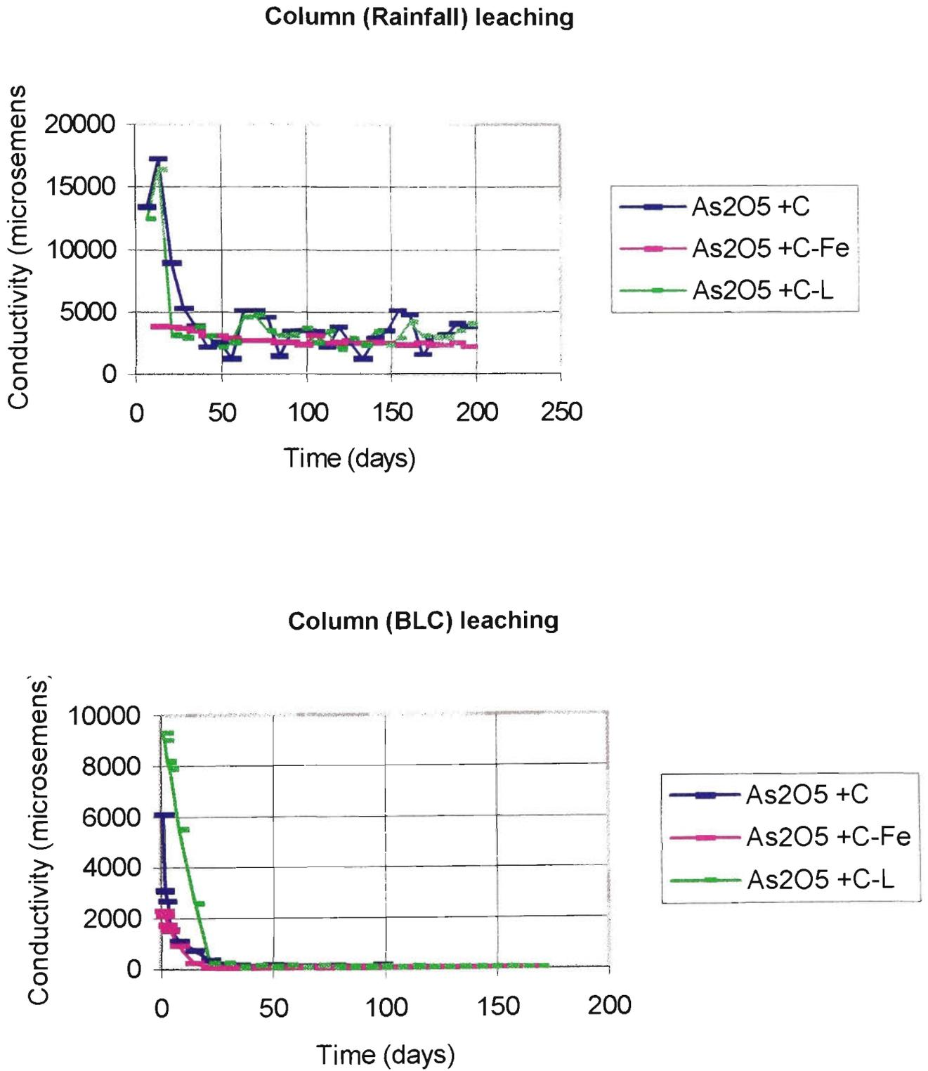
Figure 4.76 - Conductivities recorded for the Arsenic Trioxide formulations
