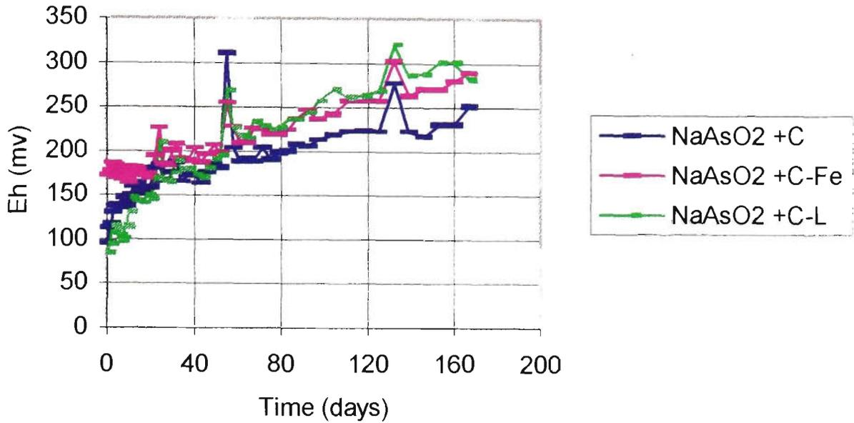
Figure 4.67 - Redox potential recorded for the arsenic trioxide formulations, Column (BLC) leaching
