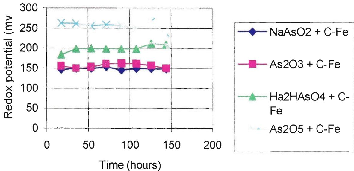
Figure 3.63 – Redox potentials of the Sequential Leaching (water) leachates of the [cement + lime] formulations
