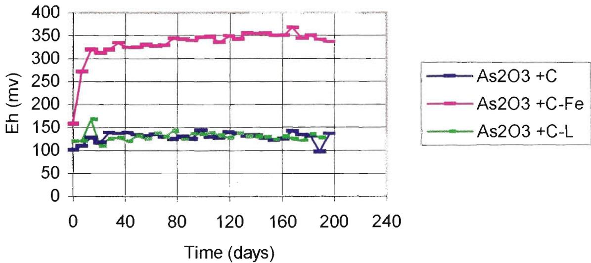
Figure 4.72 - Redox potential recorded for the arsenic pentoxide formulations, Column (Rainfall) leaching
