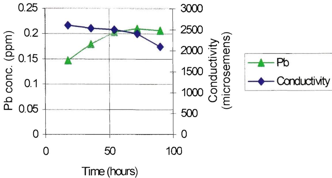
Figure 3.83 – Lead and conductivity, PbHAsO<sub>4</sub> + C-L leachates
