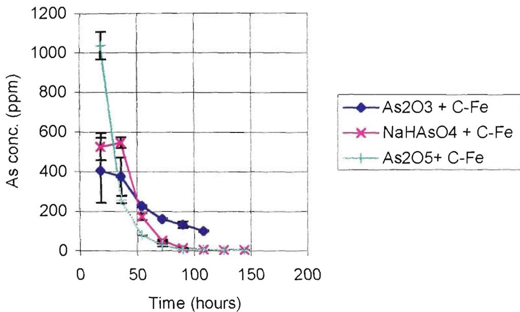
Figure 3.14 – Sequential leaching (acid) [cement + lime] stabilization
