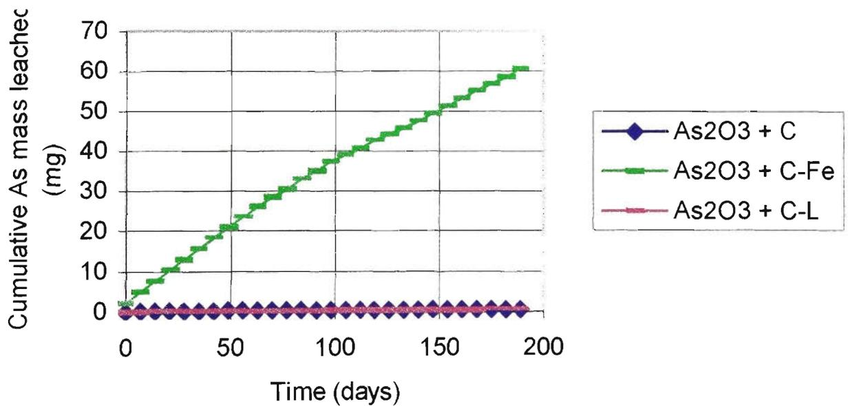
**Figure 4.24 - Cumulative mass of arsenic leached from the Column (rainfall) leaching tests – Sodium Arsenite formulations**
