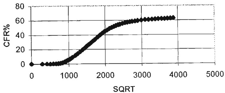
Figure 4.11 – CFR versus SQRT for the arsenic trioxide S/S formulations
