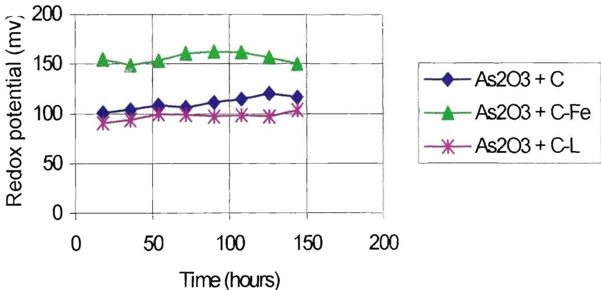
**Figure 3.65 – Redox potentials recorded from the leachates of the arsenic pentoxide formulations (deionized water leachant)**
