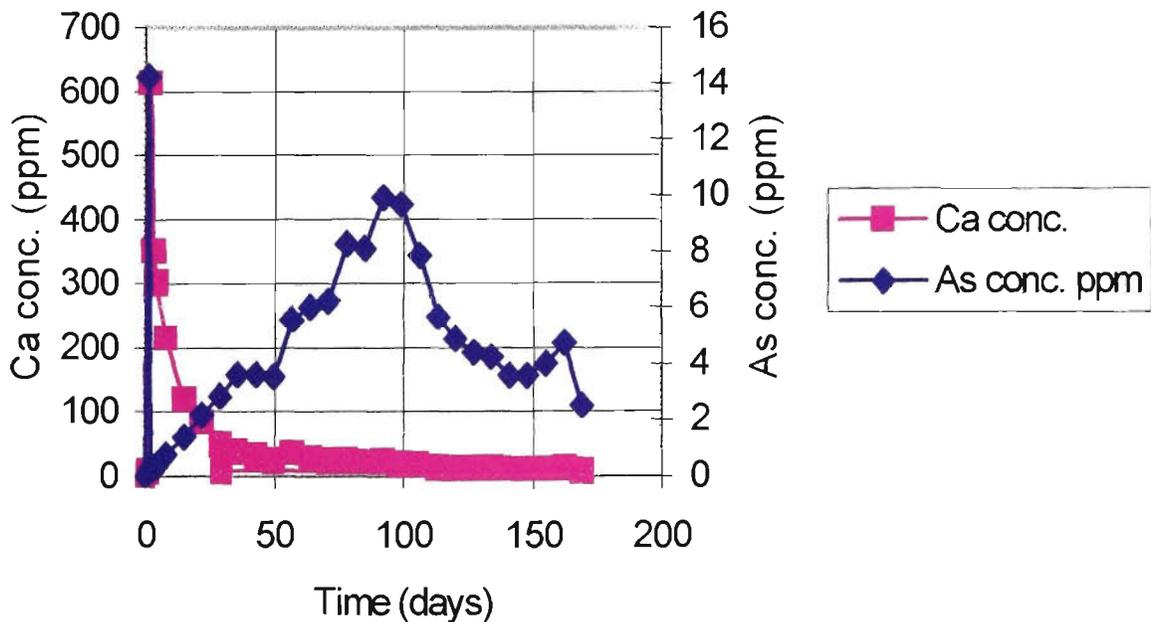
**Figure 4.7 – Relationship between the calcium and arsenic concentrations for the  $As_2O_5$  + C-L formulation**
