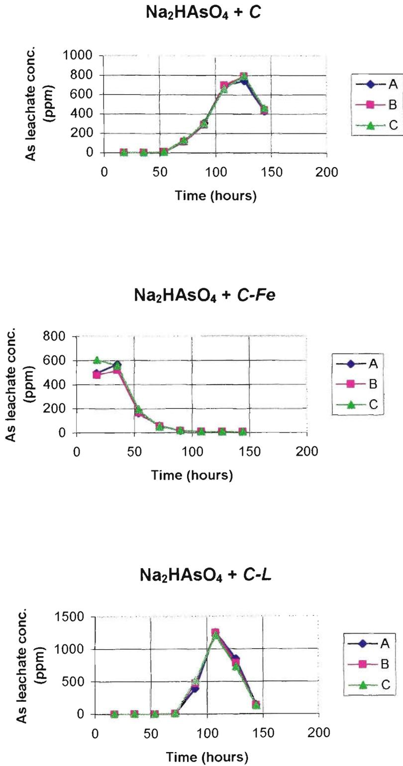
Figure 3.27 – Precision of the Sequential leaching (acid) tests and the Lead Arsenate formulations (Arsenic concentrations)
