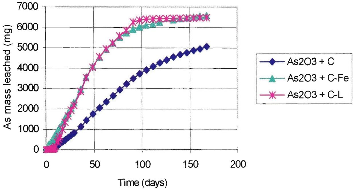
**Figure 4.3 – Column (BLC) leaching of sodium arsenite formulations**
