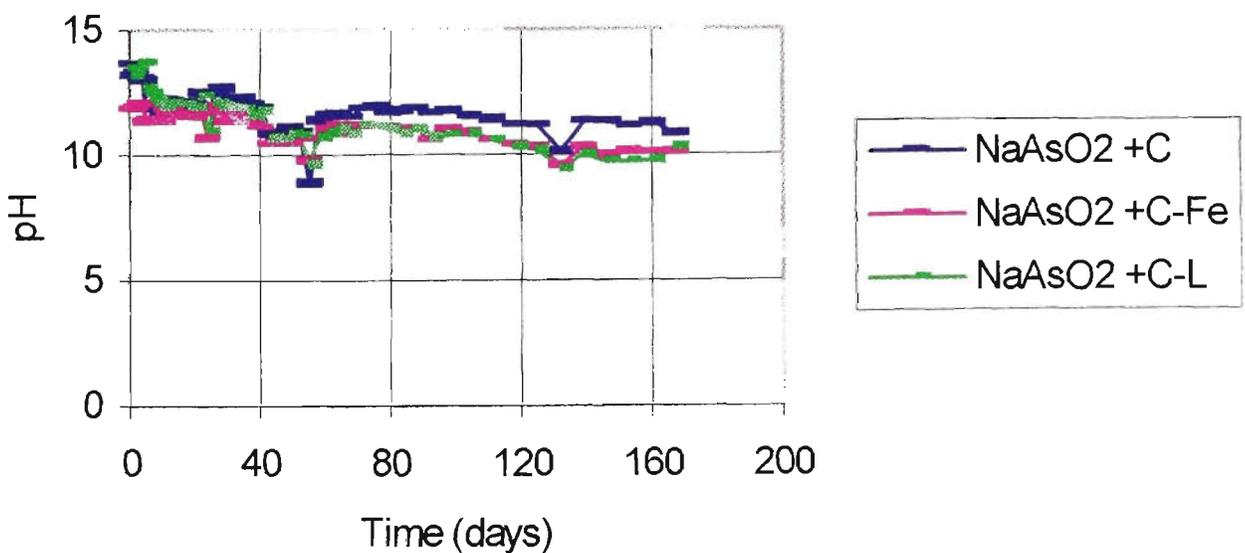
Figure 4.57 - pH values recorded for the arsenic trioxide leachates collected from the column (BLC) leaching tests
