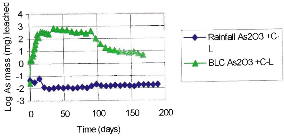
Figure 4.38 – Comparison between the masses of arsenic leached from the column(rainfall) and column (BLC) leaching tests
