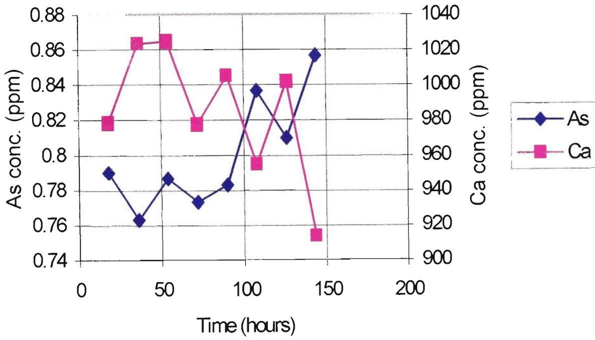
Figure 3.40 – Relationship between Calcium and Arsenic levels in the sequential leaching (water) leachates for the Sodium Arsenate formulations
