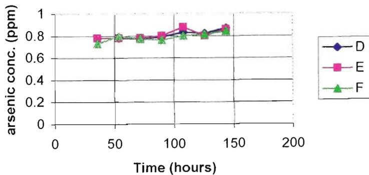
Figure 3.9 – Precision of the arsenic pentoxide S/S formulations
