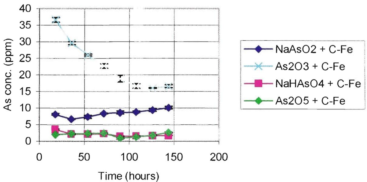
**Figure 3.3 – Sequential leaching (water) [Cement + lime] stabilization**
