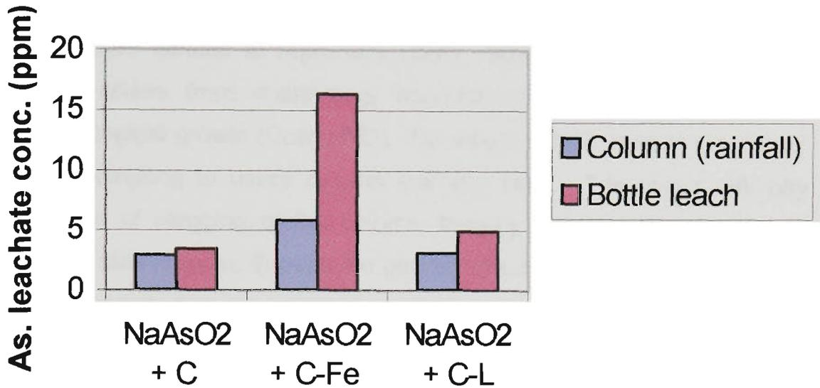
Figure 4.44 – Total mass of arsenic leached (mg) for the Sodium Arsenate formulations
