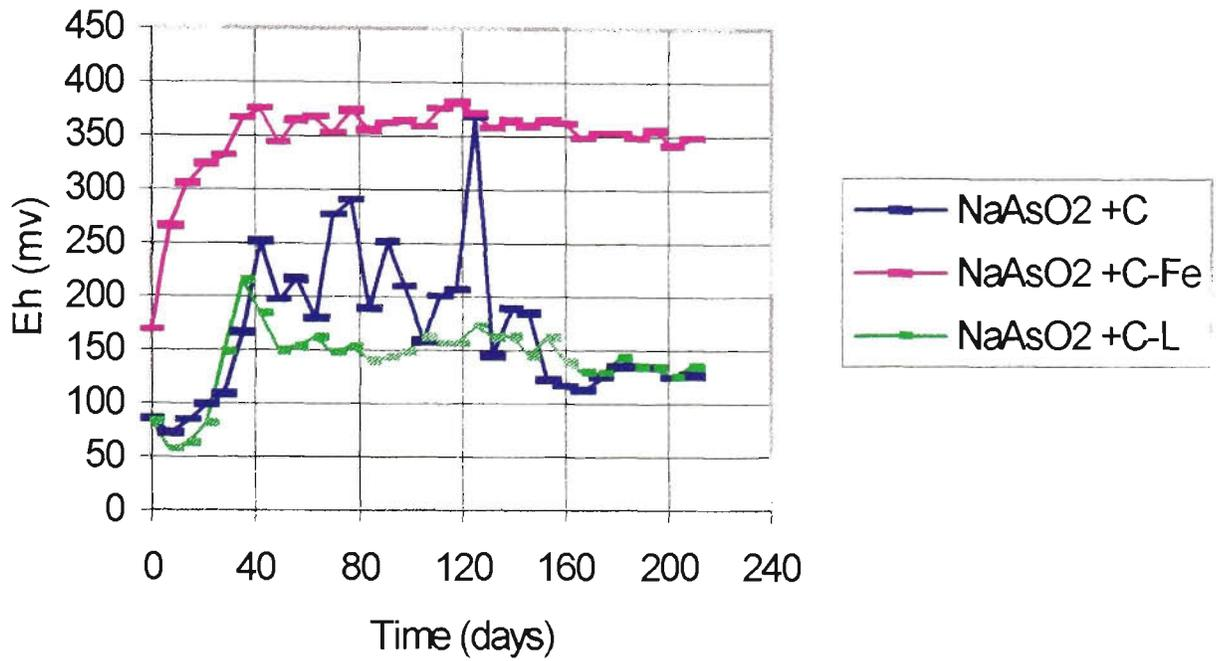
**Figure 4.71 - Redox potential recorded for the arsenic trioxide formulations, Column (Rainfall) leaching**
