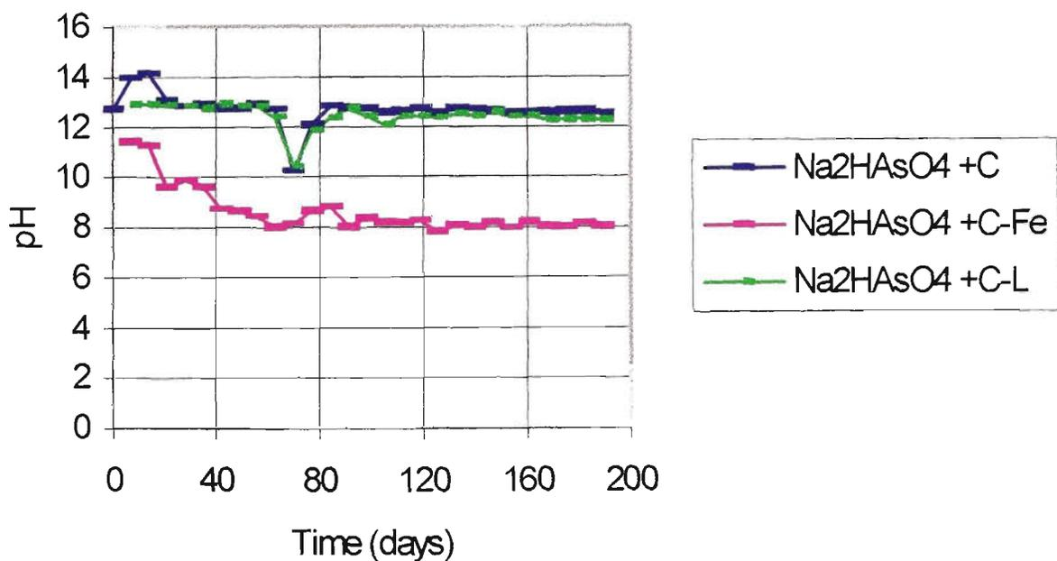
**Figure 4.61 - pH values recorded for the sodium arsenite leachates collected from the column (Rainfall) leaching tests**
