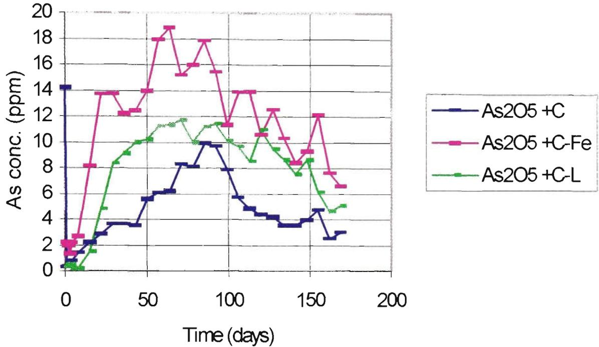
Figure 4.78 - Arsenic leachate concentrations for the arsenic pentoxide formulations, Column (Rainfall) leaching tests
