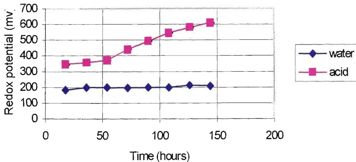
Figure 3.69 – Redox potentials of the  $\text{Na}_2\text{HAsO}_4 + \text{C}$  formulations when leached with deionized water or the acidic leachant
