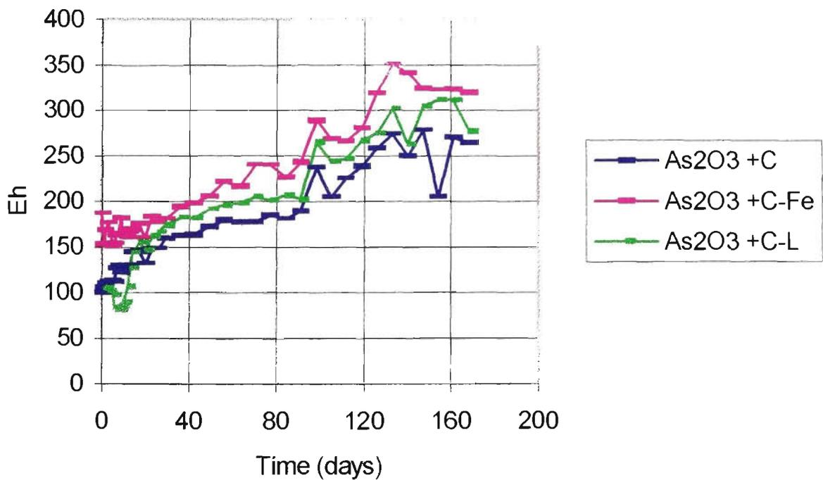
**Figure 4.68 - Redox potential recorded for the arsenic pentoxide formulations, Column (BLC) leaching**
