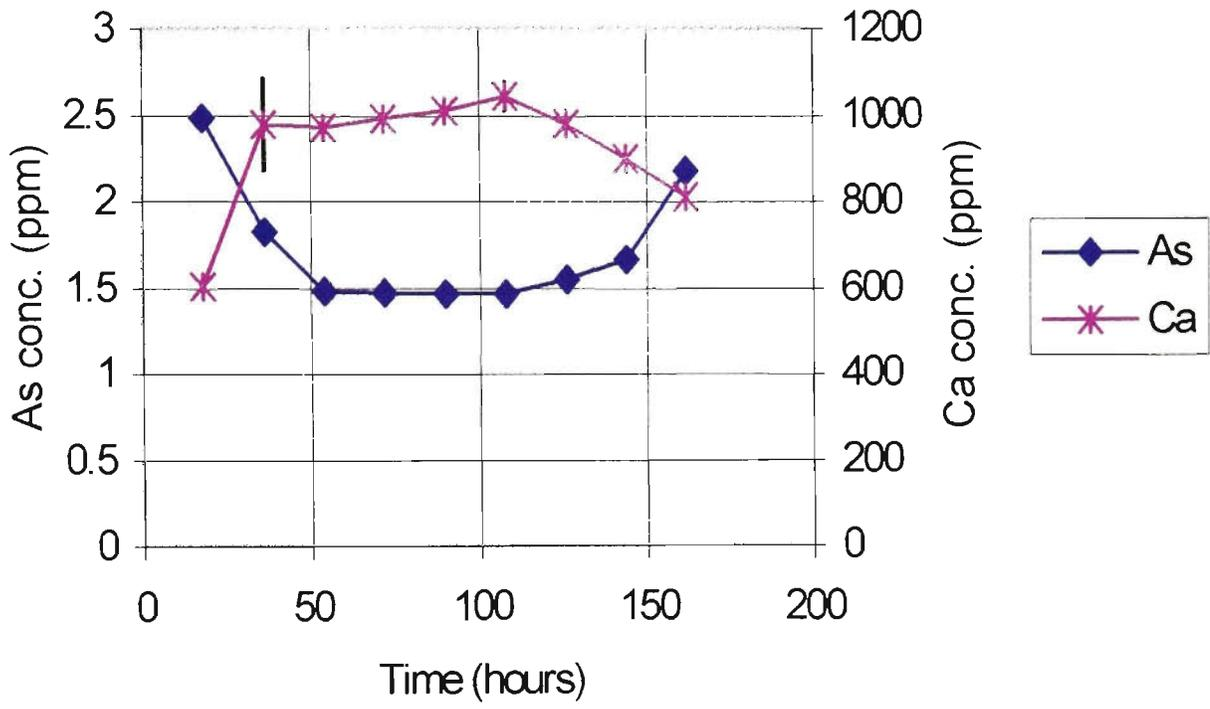
Figure 3.39 – Relationship between Calcium and Arsenic levels in the sequential leaching (water) leachates for the Arsenic Trioxide formulations
