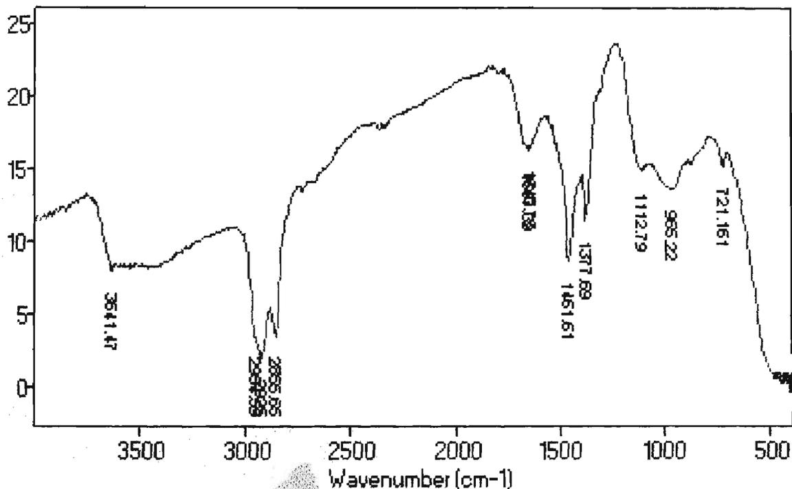
**Table 5.0 – Frequency of the Si-O band ( $\nu_3$ ) for arsenic doped cement**
