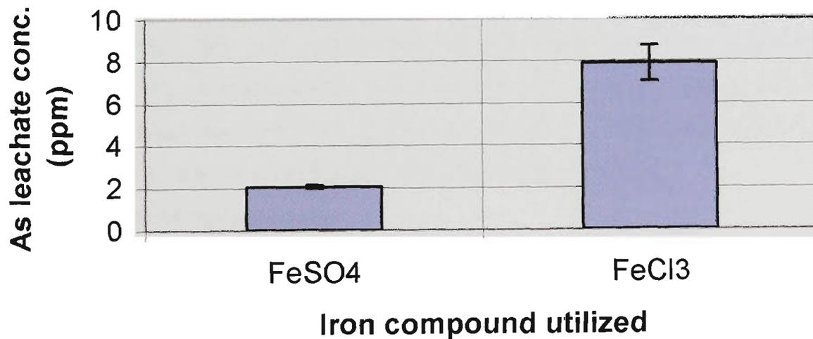
**Figure 3.52 - ABLP (acidic leachant) leachate concentrations obtained for the cement + ferrous sulfate and cement + ferric chloride stabilization of arsenic pentoxide**
