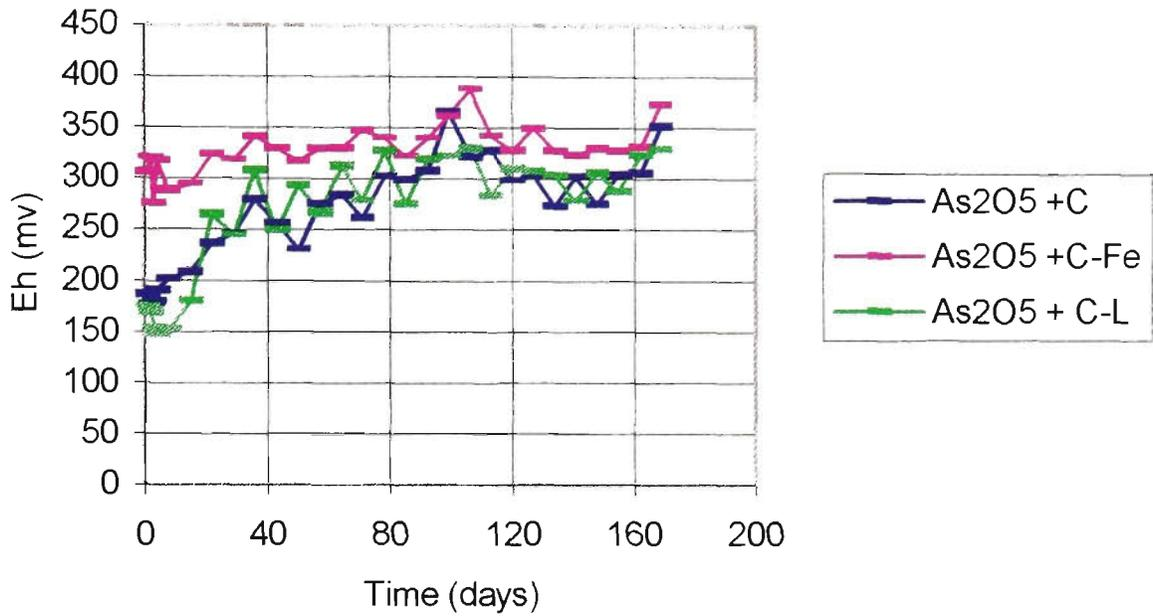
**Figure 4.69 - Redox potential recorded for the sodium arsenate formulations, Column (Rainfall) leaching**
