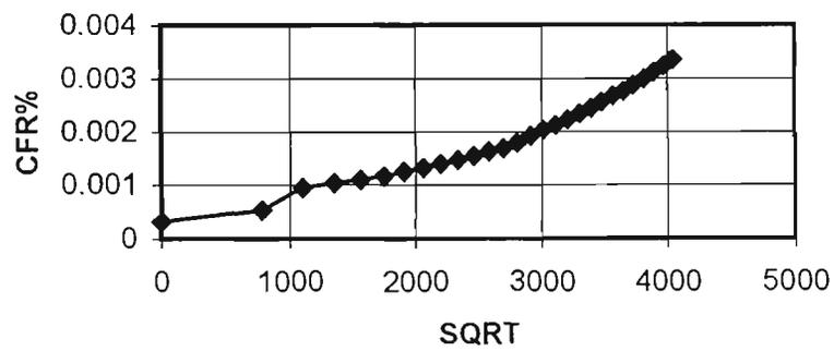
Figure 4.36 – CFR versus SQRT, Sodium Arsenite formulations
