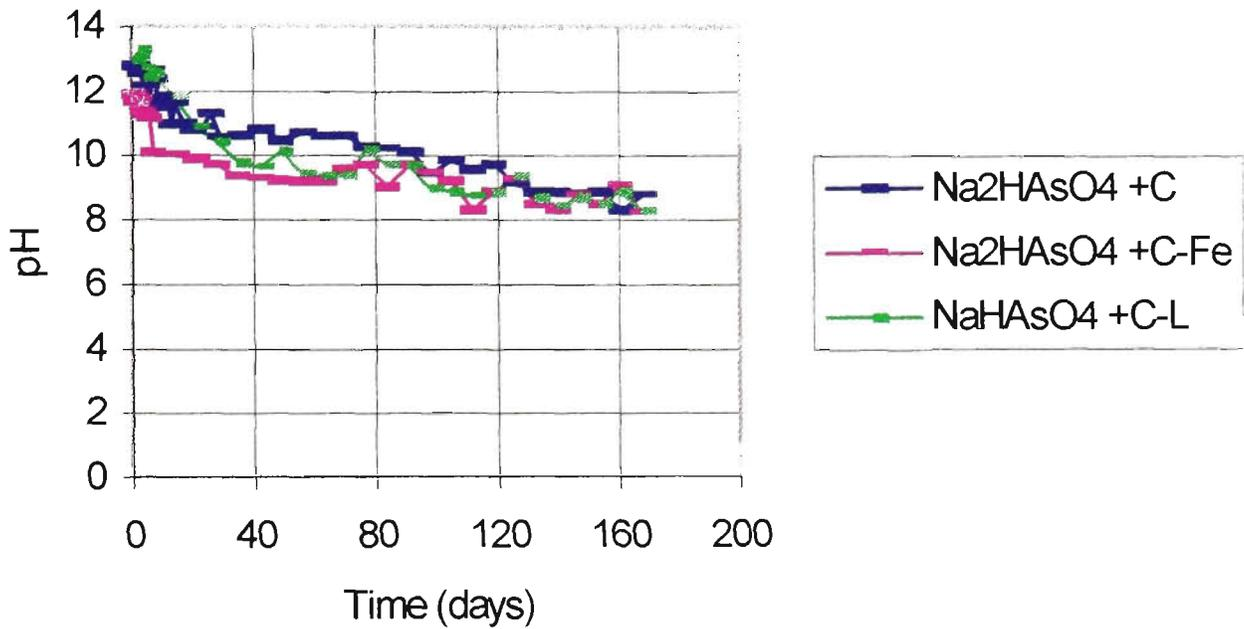
Figure 4.56 - pH values recorded for the sodium arsenite leachates collected from the column (BLC) leaching tests
