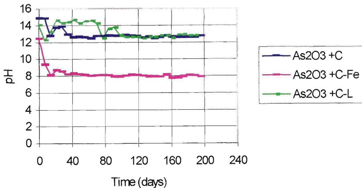
Figure 4.63 - pH values recorded for the arsenic pentoxide leachates collected from the column (Rainfall) leaching tests
