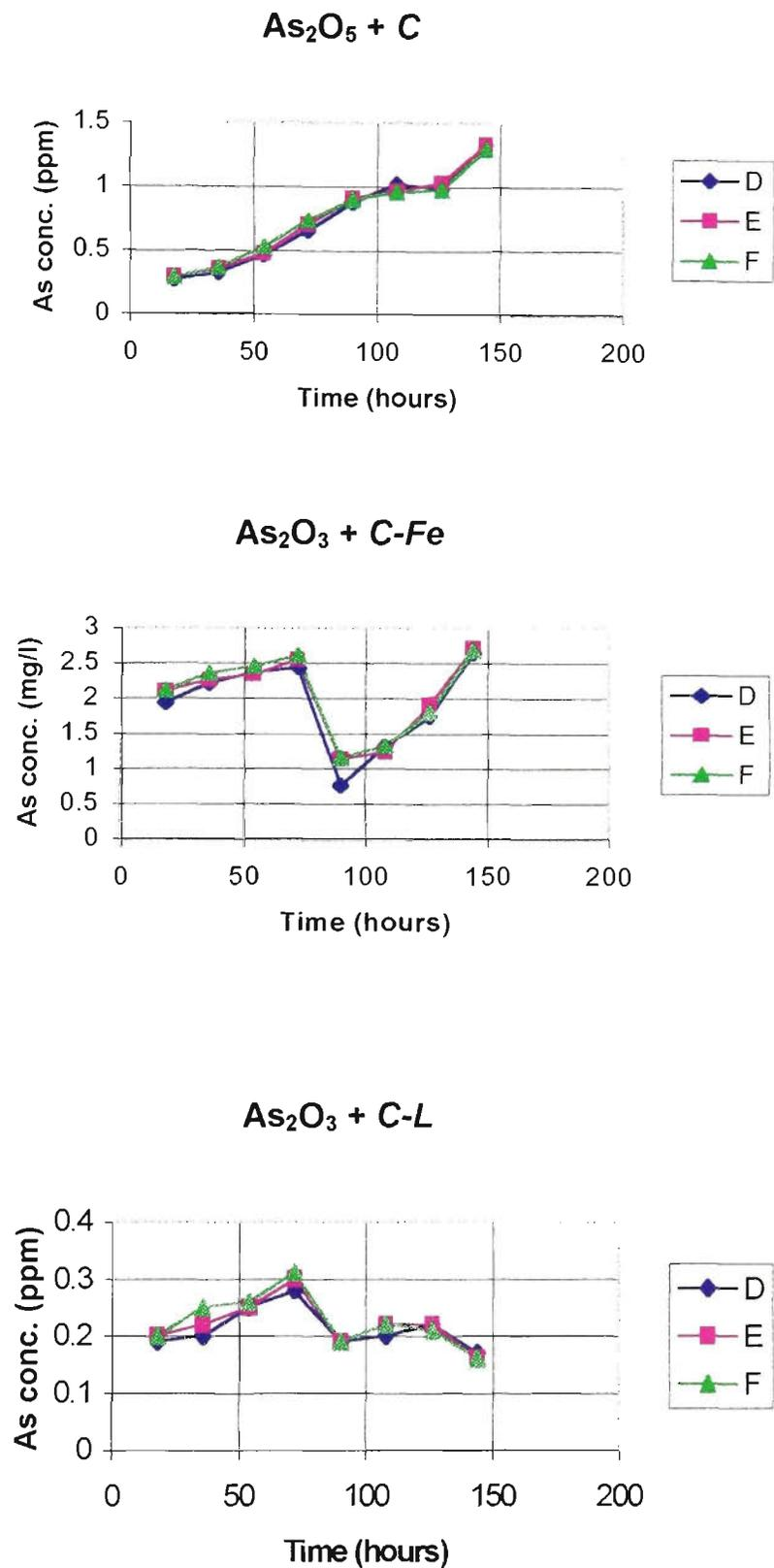
Figure 3.10 – Precision of the sodium arsenite S/S formulations
