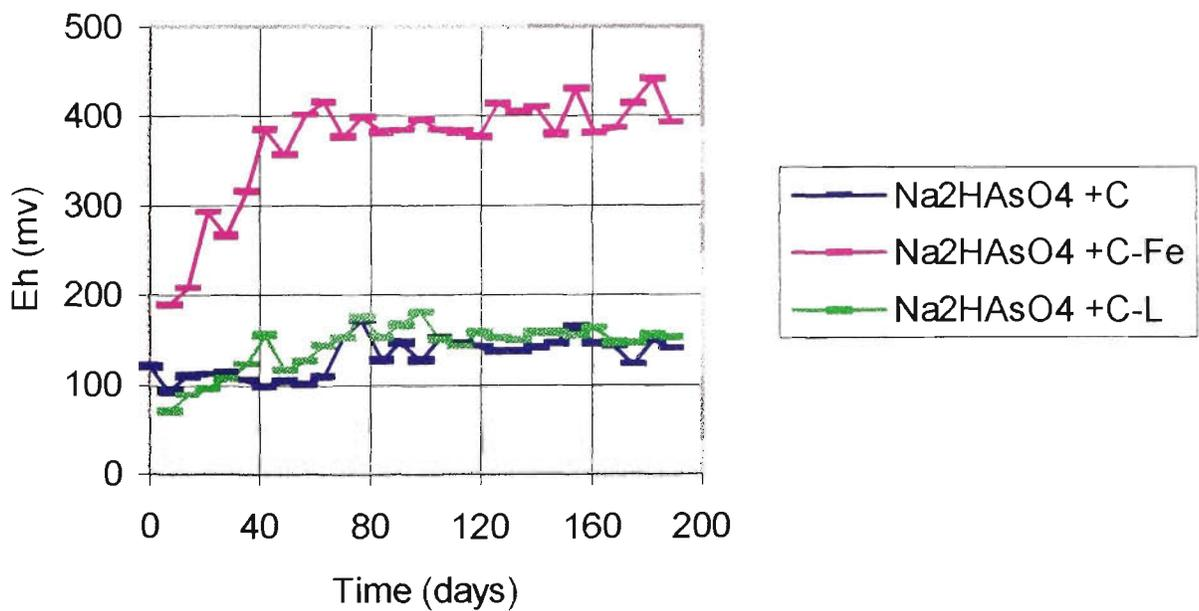
**Figure 4.70 - Redox potential recorded for the sodium arsenite formulations, Column (Rainfall) leaching**
