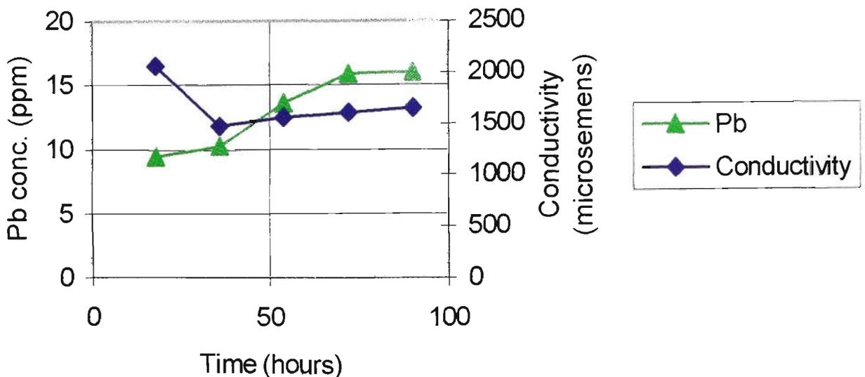
Figure 3.82 – Lead and conductivity, PbHAsO<sub>4</sub> + C-Fe leachates
