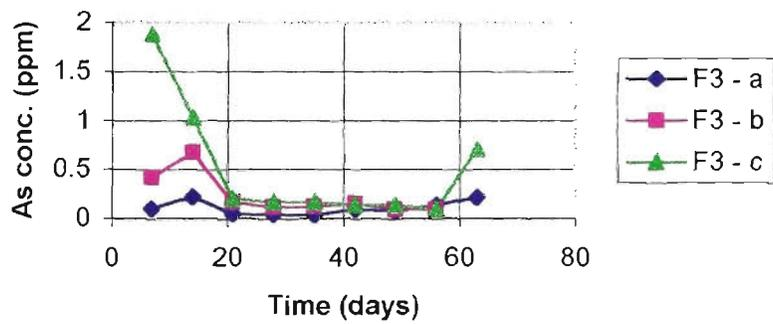
**Figure 4.54 - Precision of the Column (Rainfall) leaching tests
