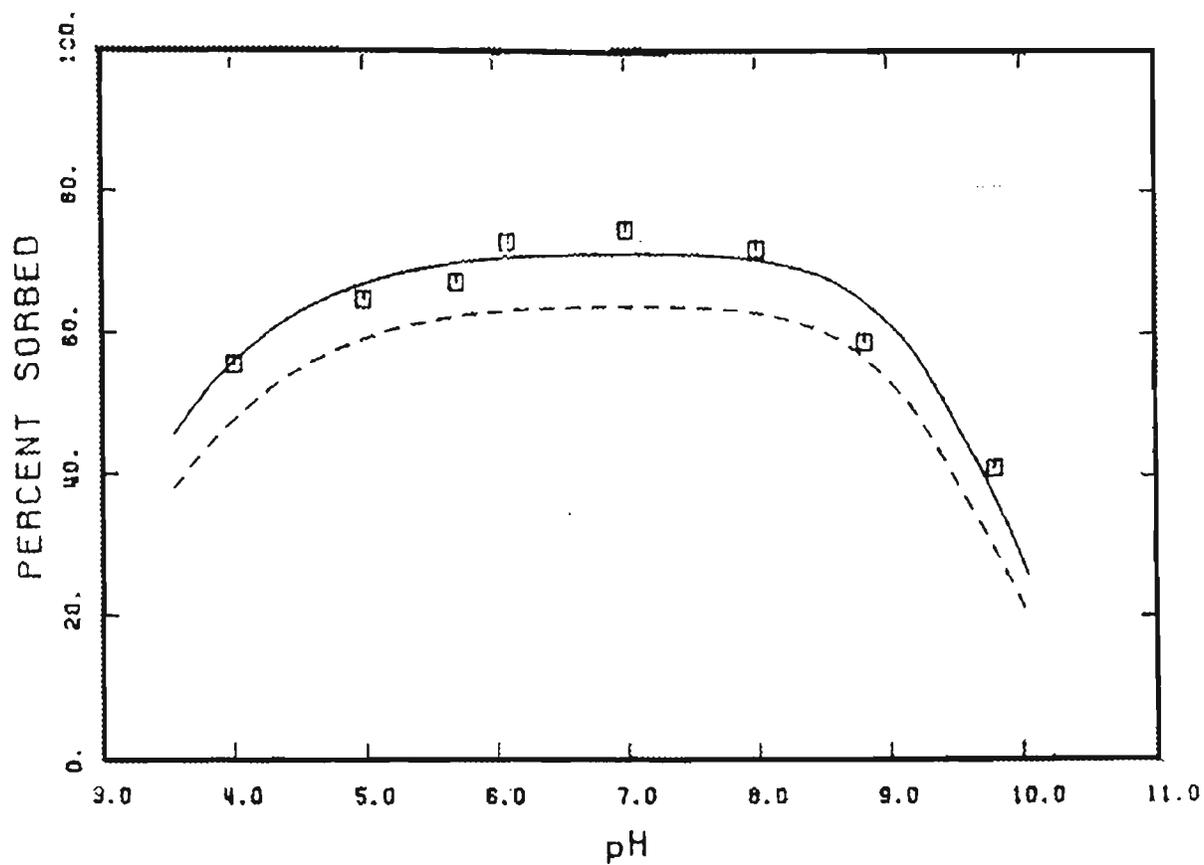
Figure 3.35 –Arsenate sorption on hydrous ferric oxide
