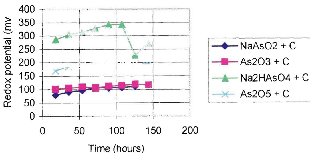
Figure 3.62 – Redox potentials of the Sequential Leaching (water) leachates of the [cement + iron] formulations
