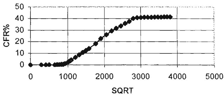
Figure 4.12 – CFR versus SQRT for the sodium arsenate S/S formulations
