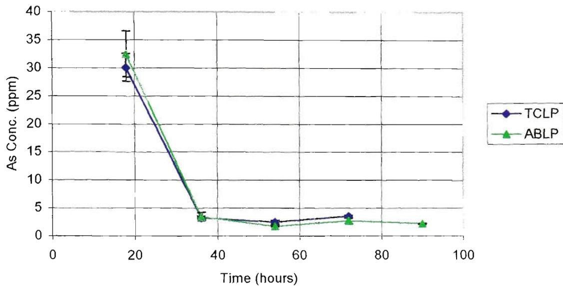
**Figure 3.17 – Similarities between the sequential leaching results obtained using both the TCLP and the ABLP for the  $\text{PbHAsO}_4 + \text{C-L}$  formulation**
