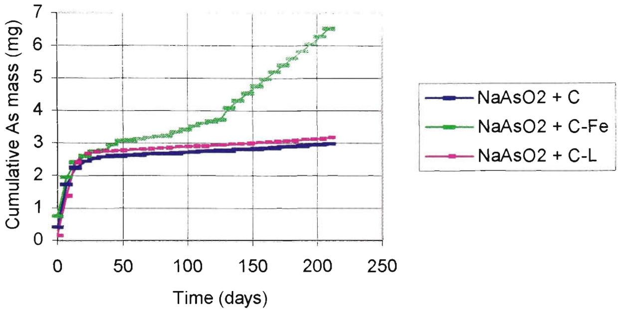
**Figure 4.25 - Cumulative mass of arsenic leached from the Column (rainfall) leaching tests – Sodium Arsenate formulations**
