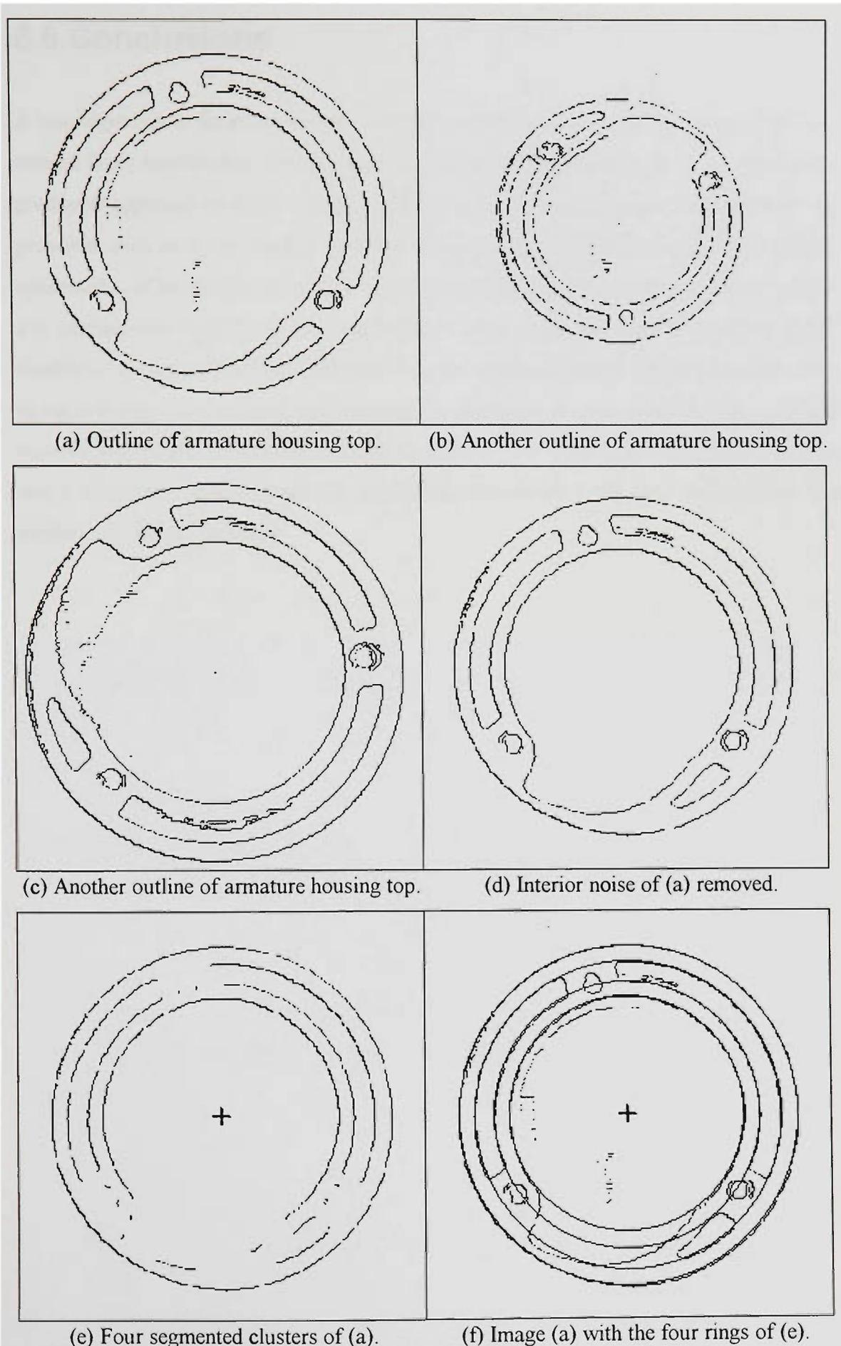
Figure 6.5 Segmented outlines of an armature housing top, acquired in different orientations and positions. (e) Clusters parameters of (e) are:  $q=12$  and  $N_{min}=112$ .
