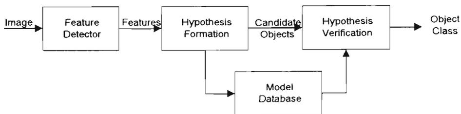
Figure 1.2 Basic steps to object recognition. Adapted from [Jain et al., 1995].
