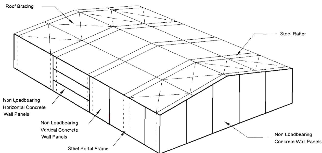
*NOTE: The Non-Loadbearing Concrete Wall Panels are Either Pinned or Fixed at the Base*
