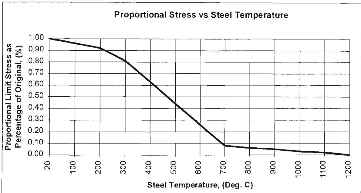
**Figure B.2:** Proportional Limit Stress versus Temperature - (Steel)
