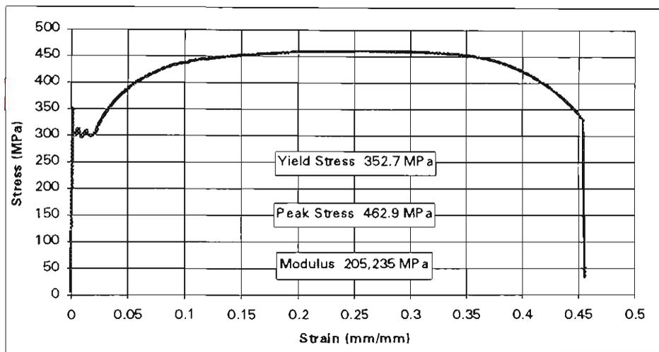
Figure E.6 Stress-Strain Relationship for Coupon Test 2
