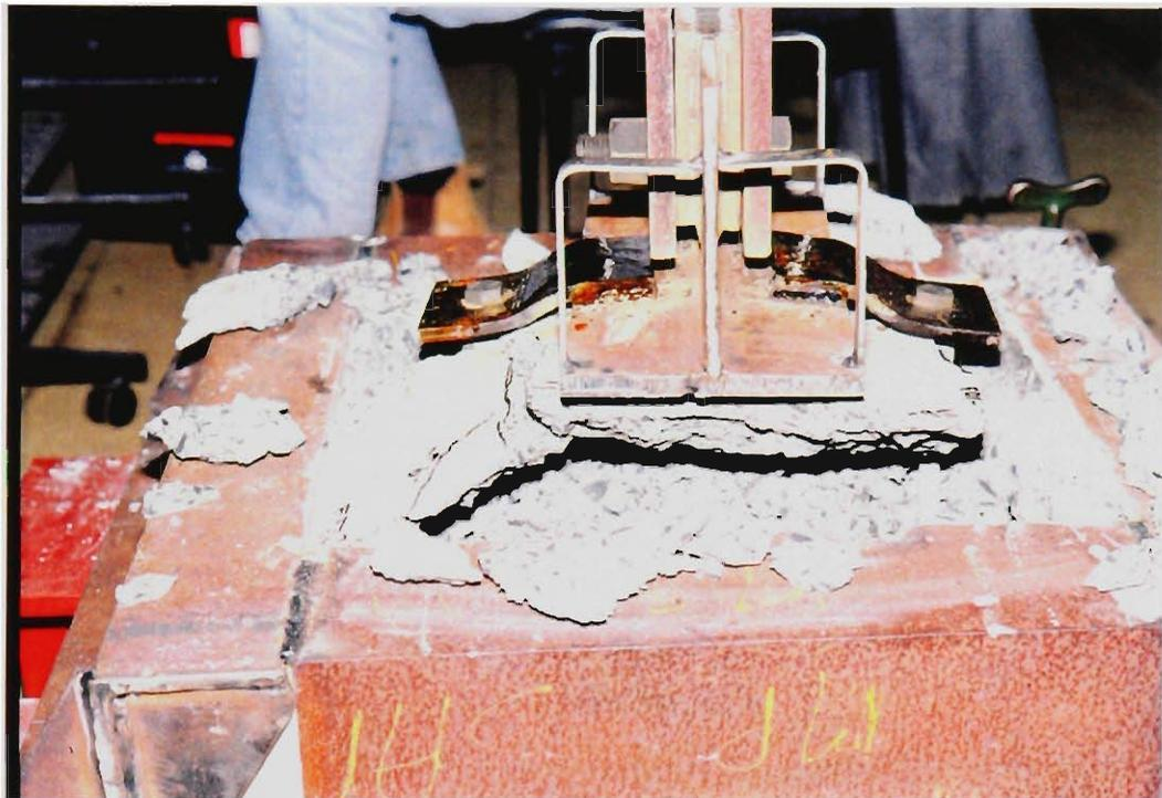
**Figure 5.18** Proper Failure of W-20 Clip Plate Test
