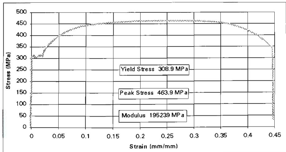
Figure E.7 Stress-Strain Relationship for Coupon Test 3
