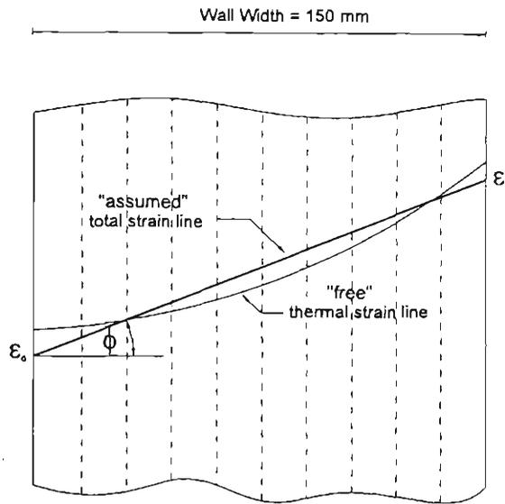
Figure 3.9 Locations of Initial Strain and Curvature Estimates at Segment j.
