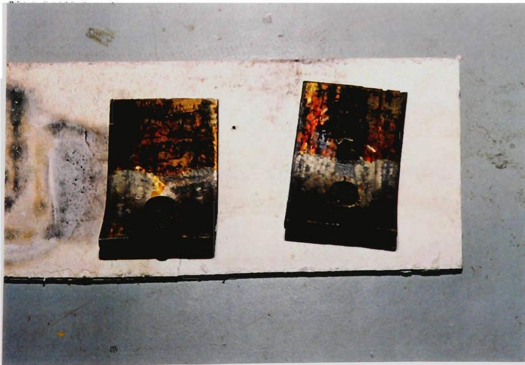
Figure 5.11 Failed NW-20 Clip Plates
