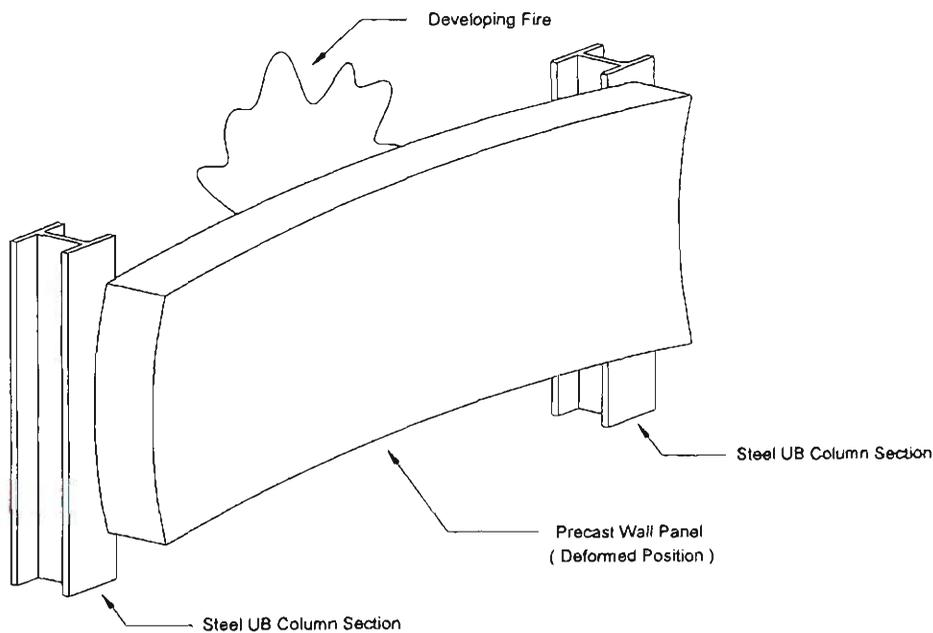
**Figure 4.7** Typical Horizontal Wall Panel Orientation and Deformation Characteristics
