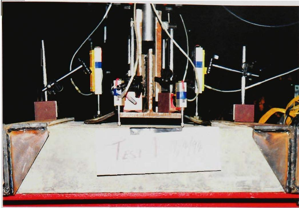
Figure 5.10 Lacquered Clip Plate Under Strain
