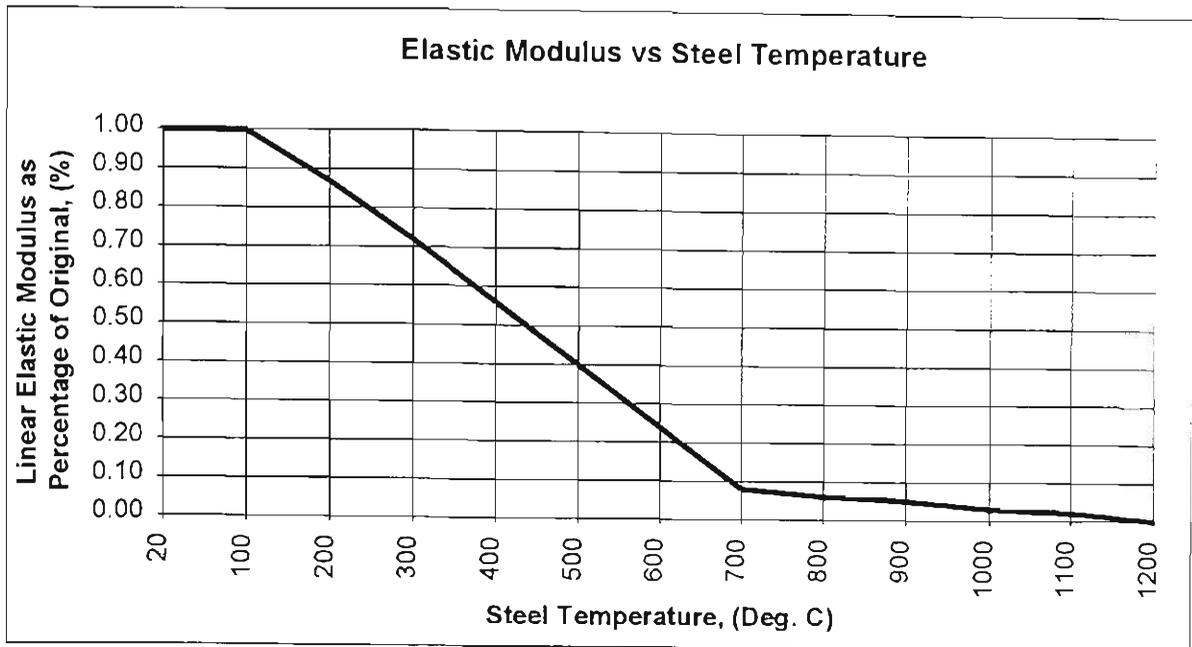
**Figure B.1:** Elastic Modulus versus Temperature - (Steel)
