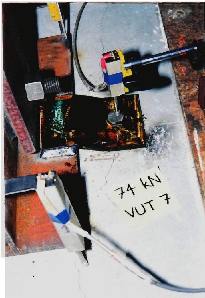
Figure 5.14 W-20 Test Clip Plate Under Strain
