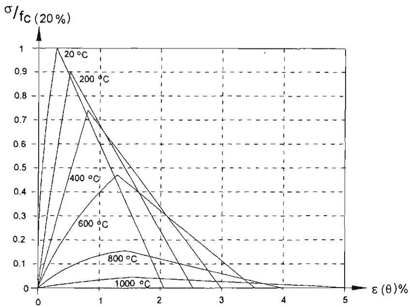
Figure 3.6 Stress-Strain Relationships for Siliceous Concrete at Elevated Temperatures
