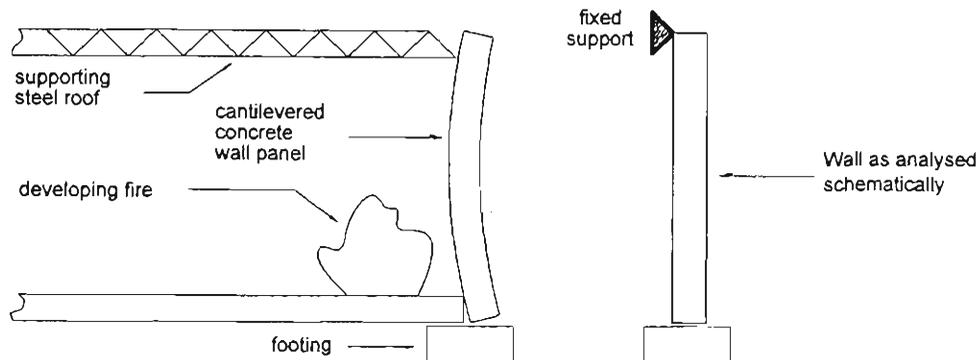
**Figure 2.11** Behaviour of Cantilevered Concrete Wall in Tilt-Up Construction; (Gnanakrishnan, 1993)
