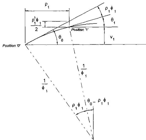
**Figure 3.8** Geometric Relationships Between Successive Points on a Curve
