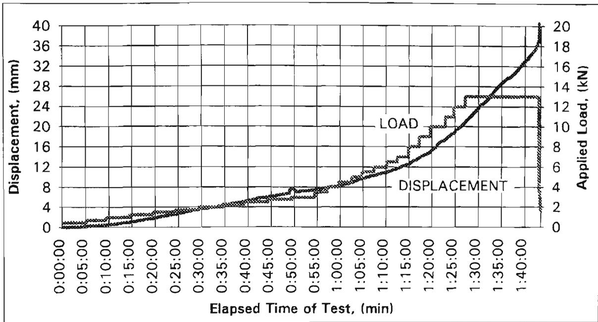
Figure 5.25 Creep Effects for Welded Connection Tested at 800 °C
