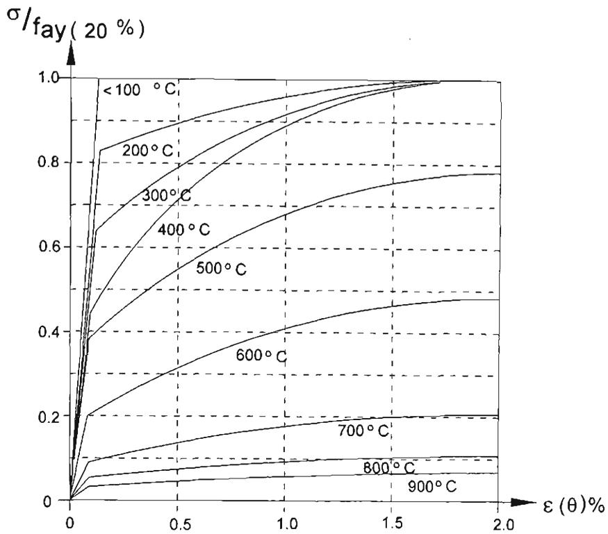
Figure 3.5 Stress-Strain Relationships for Reinforcing Steels at Elevated Temperatures
