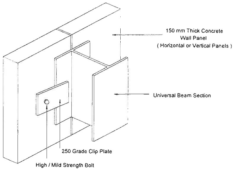
**Figure 2.4** Typical Steel Clip Plate Bearing Connection
