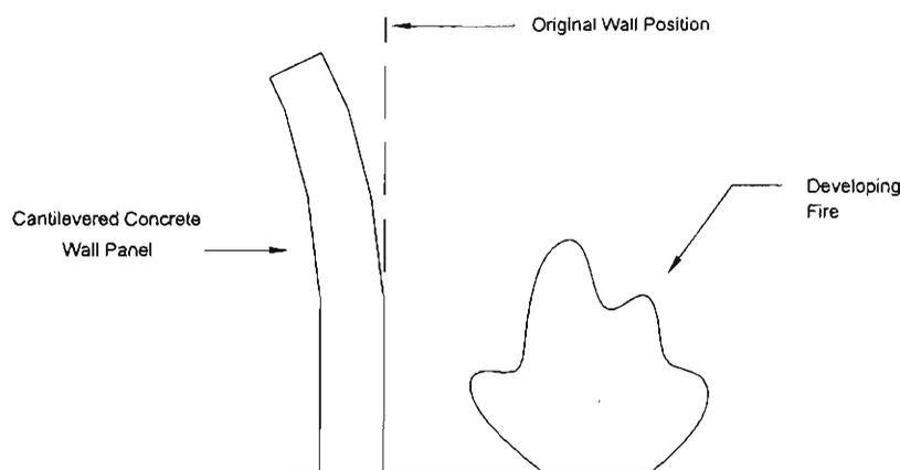
Figure 2.10 Deformation of a Cantilevered Wall
