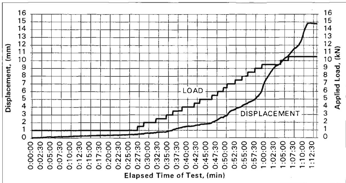
Figure 5.19 Creep Effects for Non-Welded Connection Tested at 600 °C
