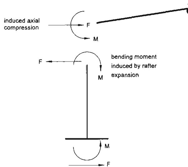
**Figure 2.7** Forces and Moments Acting on the Portal Frame Members - Free Body Diagram
