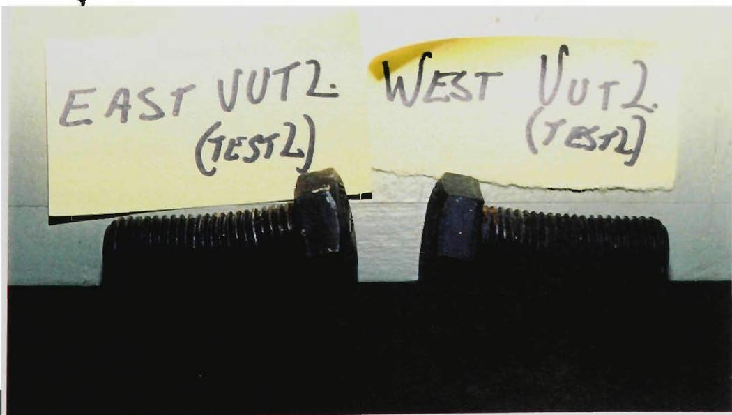
Figure 5.13 Bolt Elongation And Deformation of Test NW-20
