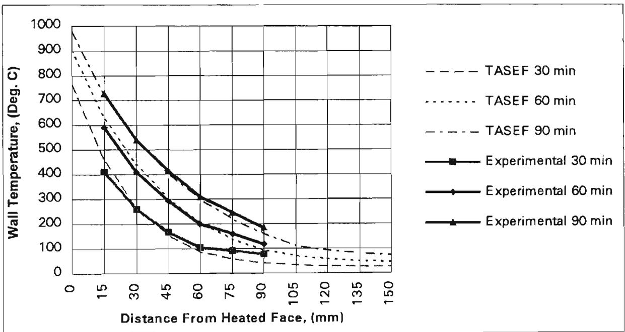
Figure 3.1 Standard Fire Temperature Gradients at Varying Times of Exposure for 150 mm Thick Concrete Wall - [TASEF-2 versus Experimental Results]
