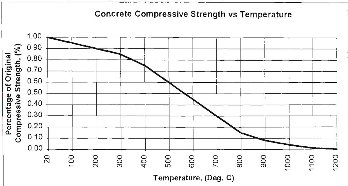
**Figure B.5:** Compressive Strength versus Temperature - (Concrete)
