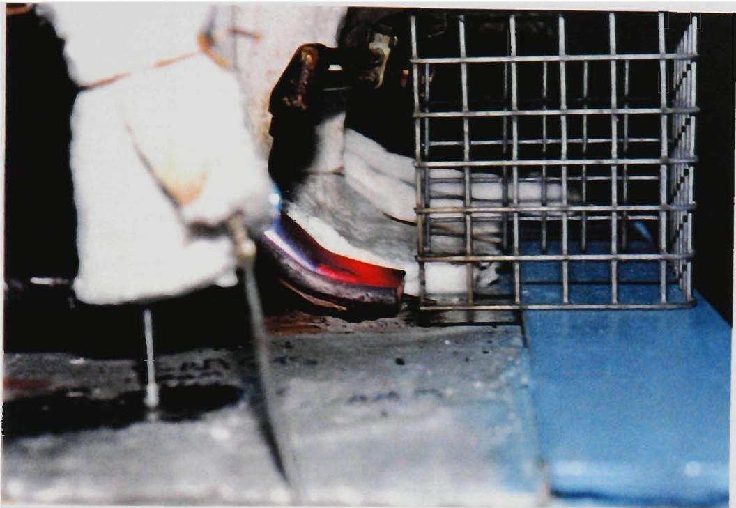
**Figure 5.23** Plate and Bolt Deformation of W-600 Test
