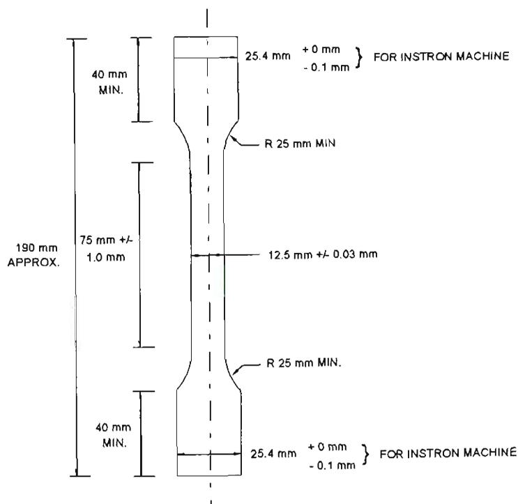
Figure E.4 Standard B-34 Tensile Coupon Test Specimen
