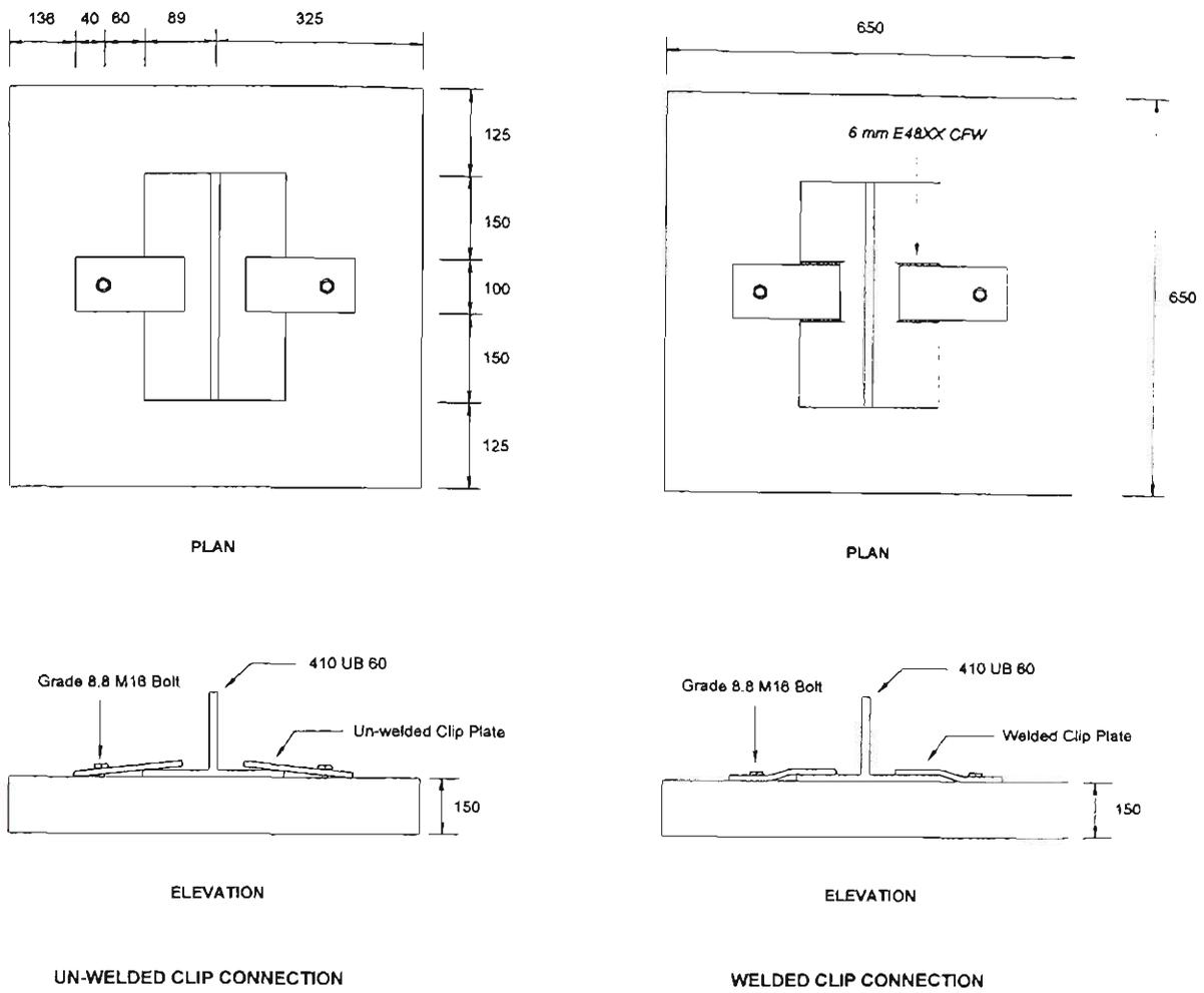
**Figure 5.4** Details of Connection Samples Tested
