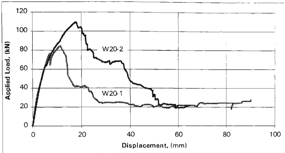
**Figure 5.15** Load Displacement Chart for Welded Connections Tested at Ambient Temperature
