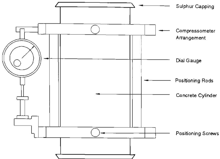
**Figure E.1** Typical Compressometer Arrangement for Measurement of Longitudinal Strain
