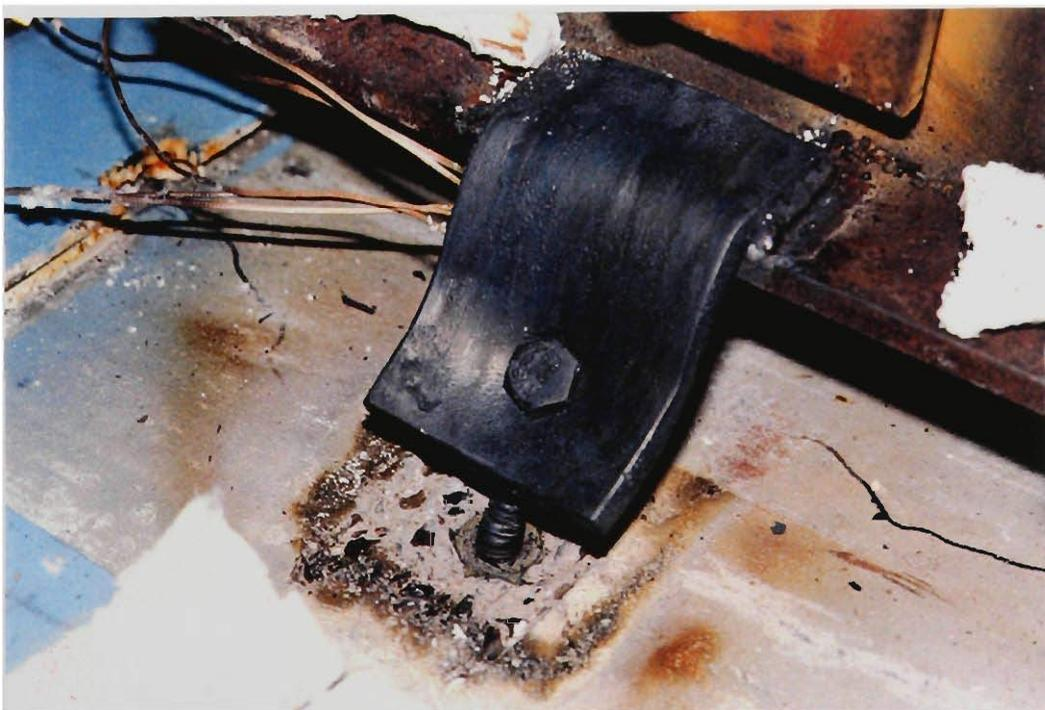
Figure 5.26 Failure of W-800 Test Showing Bolt Yielding
