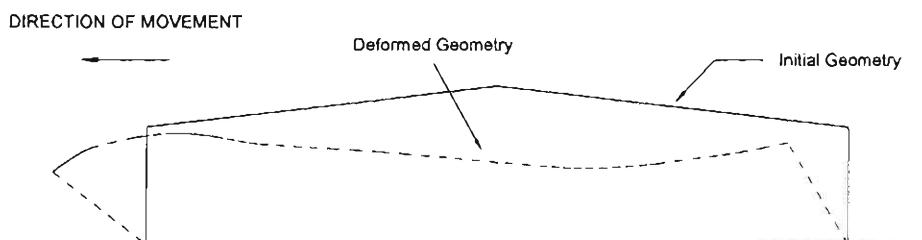
**Figure 2.8 (b)** Unacceptable Outwards Collapse of Portal Frame
