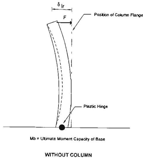
**Figure 4.5** Force at Connection where relative displacement is  $\delta_{lr}$
