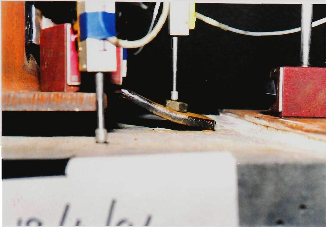
Figure 5.12 Deformation of NW-20 Clip Plate
