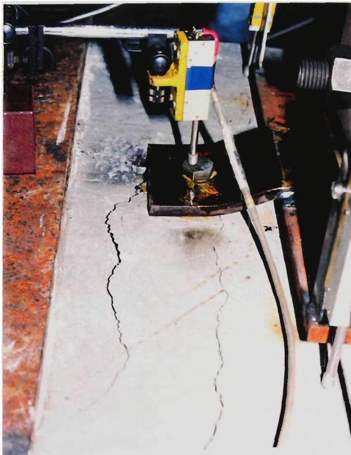
**Figure 5.16** Premature Failure of W-20 Clip Plate
