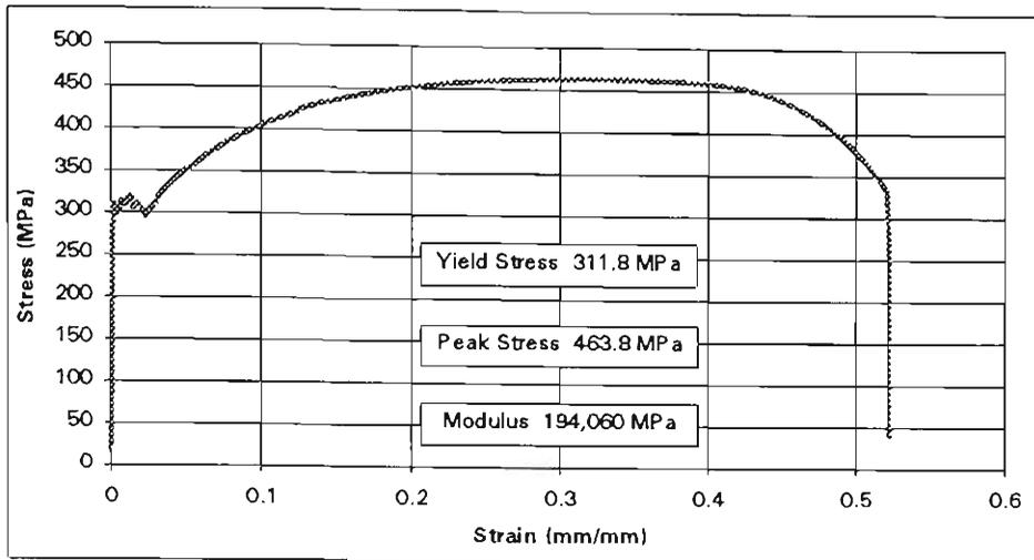
Figure E.5 Stress-Strain Relationship for Coupon Test 1
