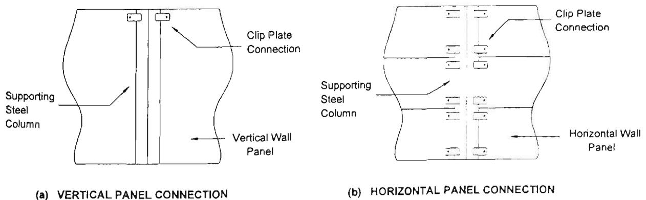
Figure 5.1 Common Forms of Connections that Utilise Steel Clips
