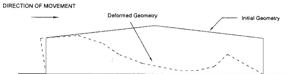
**Figure 2.8 (a)** Acceptable Inwards Collapse of Portal Frame
