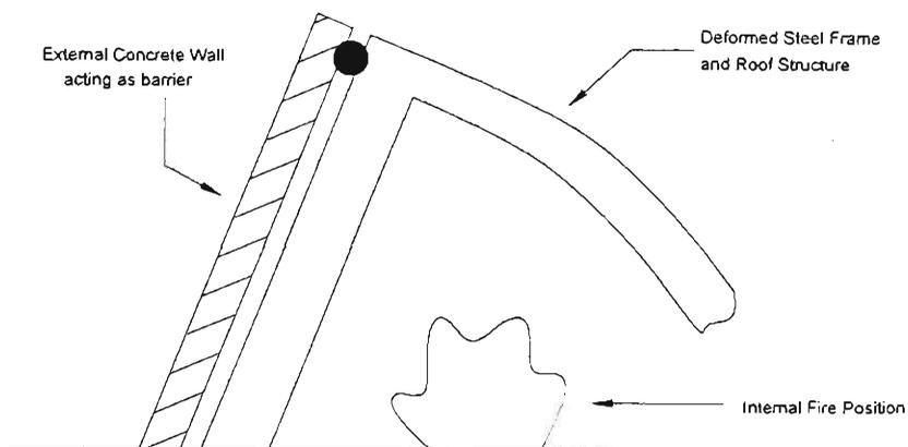
**Figure 2.2** Possible Deformed Shape of Single-Storey Industrial Building
