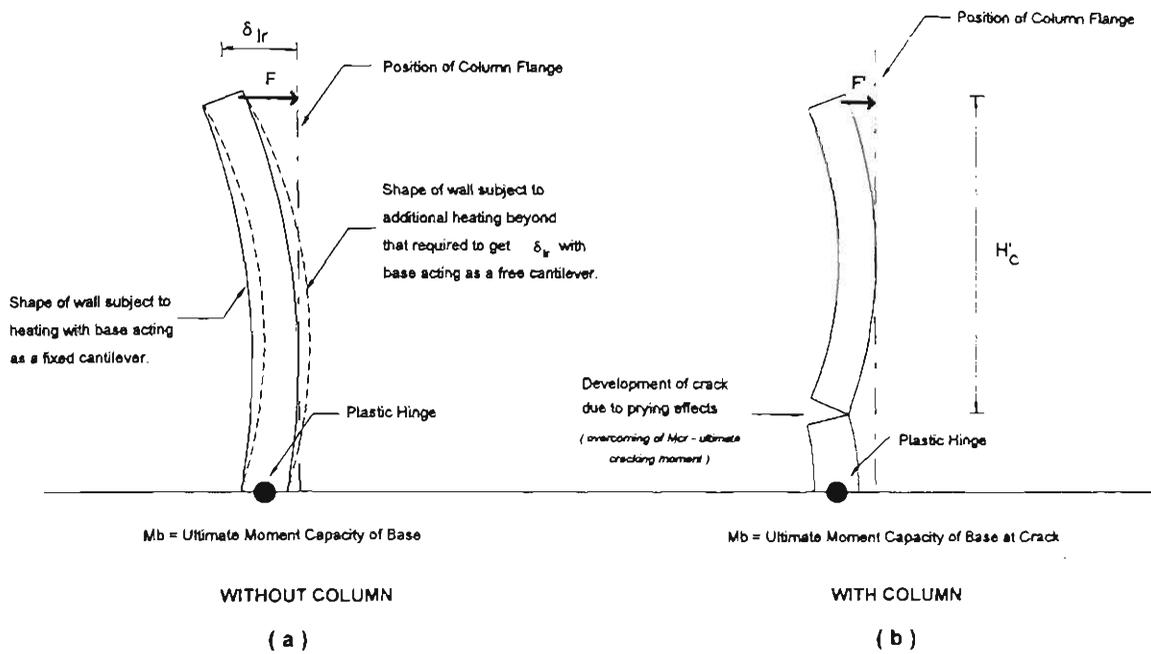
**Figure 4.6** Wall Deformation Effects With and Without Supporting Structure
