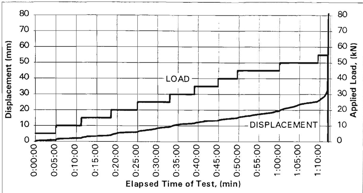
**Figure 5.24** Creep Effects for Welded Connection Tested at 600 °C
