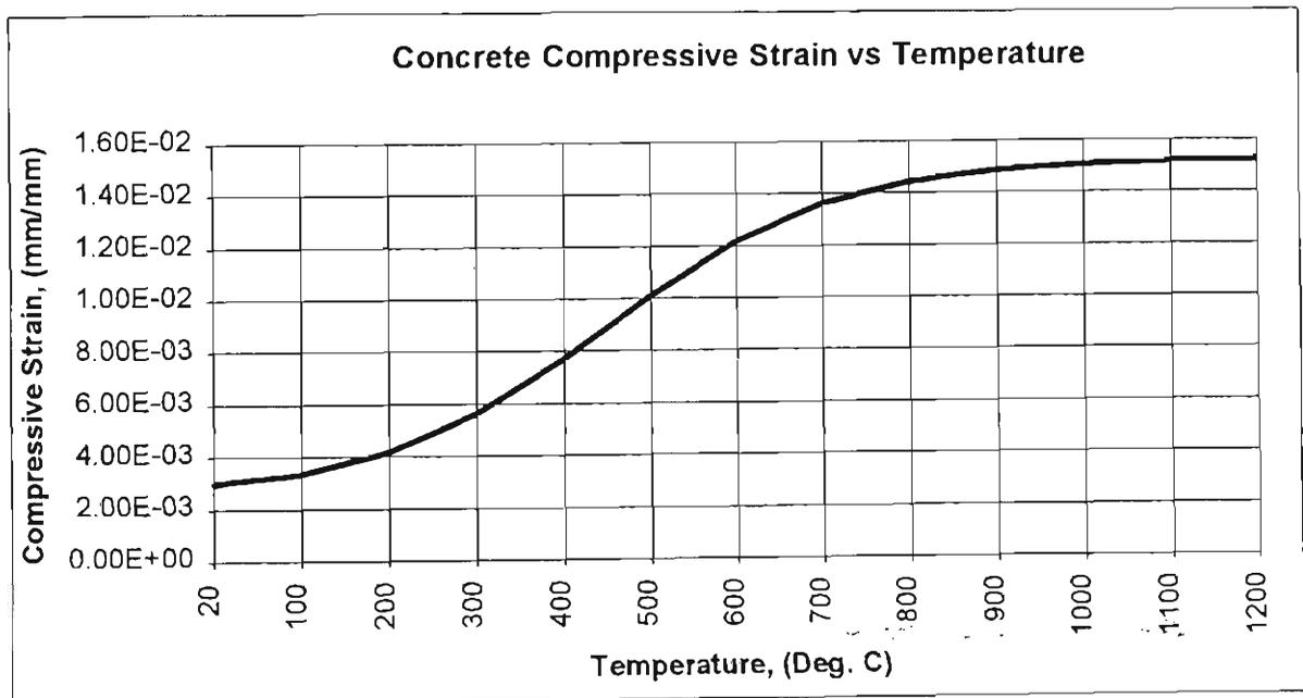
**Figure B.4:** Compressive Strain versus Temperature - (Concrete)
