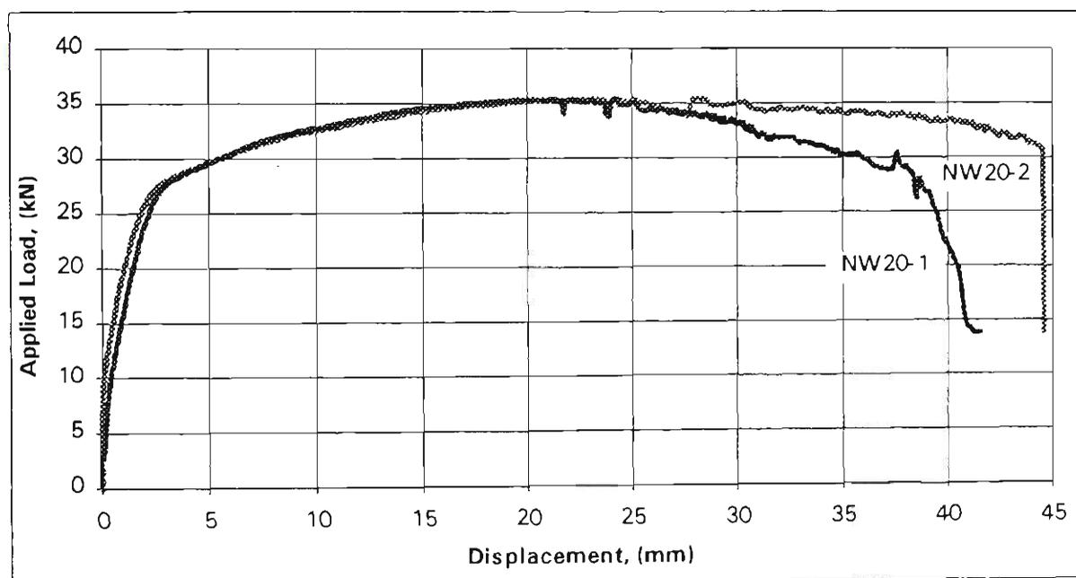
Figure 5.9 Load Displacement Chart for Non-Welded Connections Tested at Ambient Temperature
