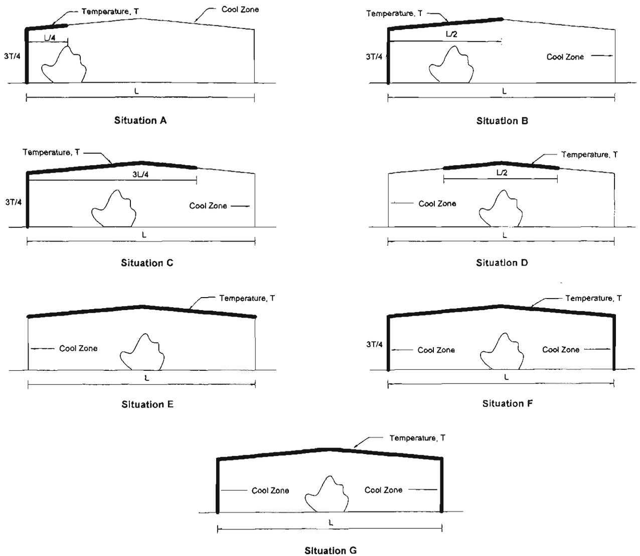
**Figure 2.9** Heating Situations Considered by O'Meagher et al. (1990)
