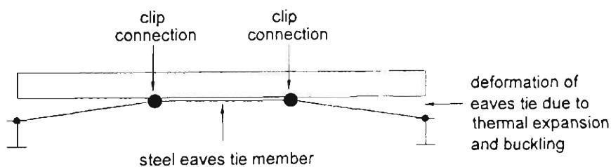
Figure 5.2 System Capable of Minimising Prying Effects
