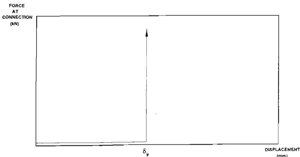
**Figure 4.4** Idealised Connection Characteristics
