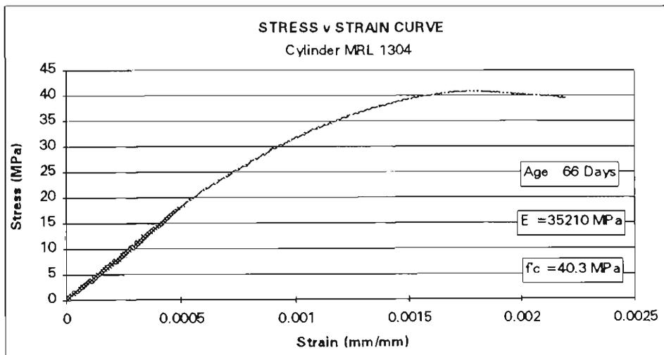
**Figure E.2** Stress-Strain Relationship for Cylinder MRL 1304
