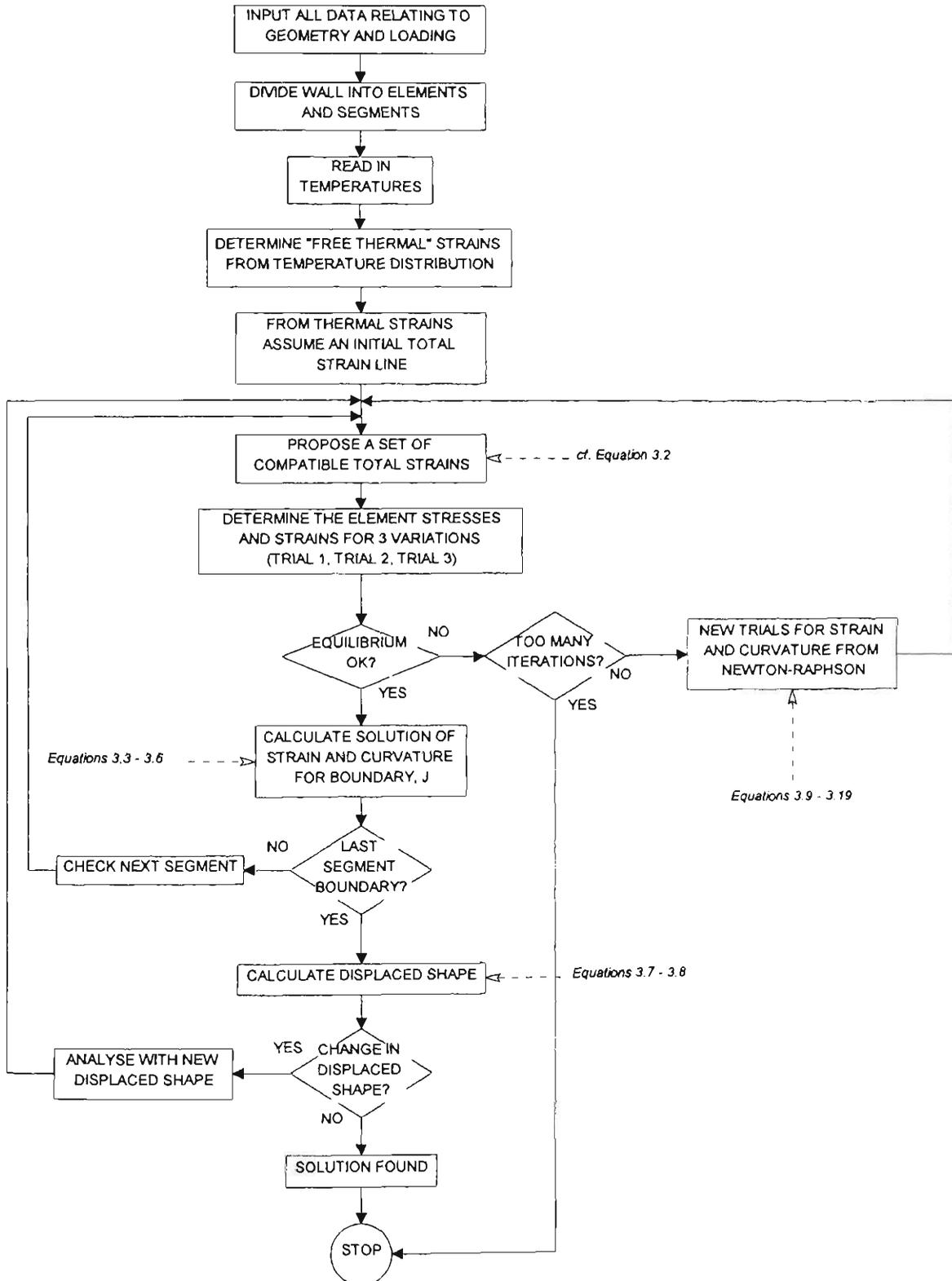
Figure 3.10 Analysis Flow Chart for the Solution of the Wall Model
