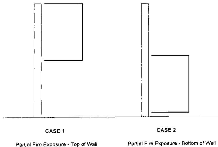
**Figure 4.2**      Simplified Cases Analysed for Differential Heating
