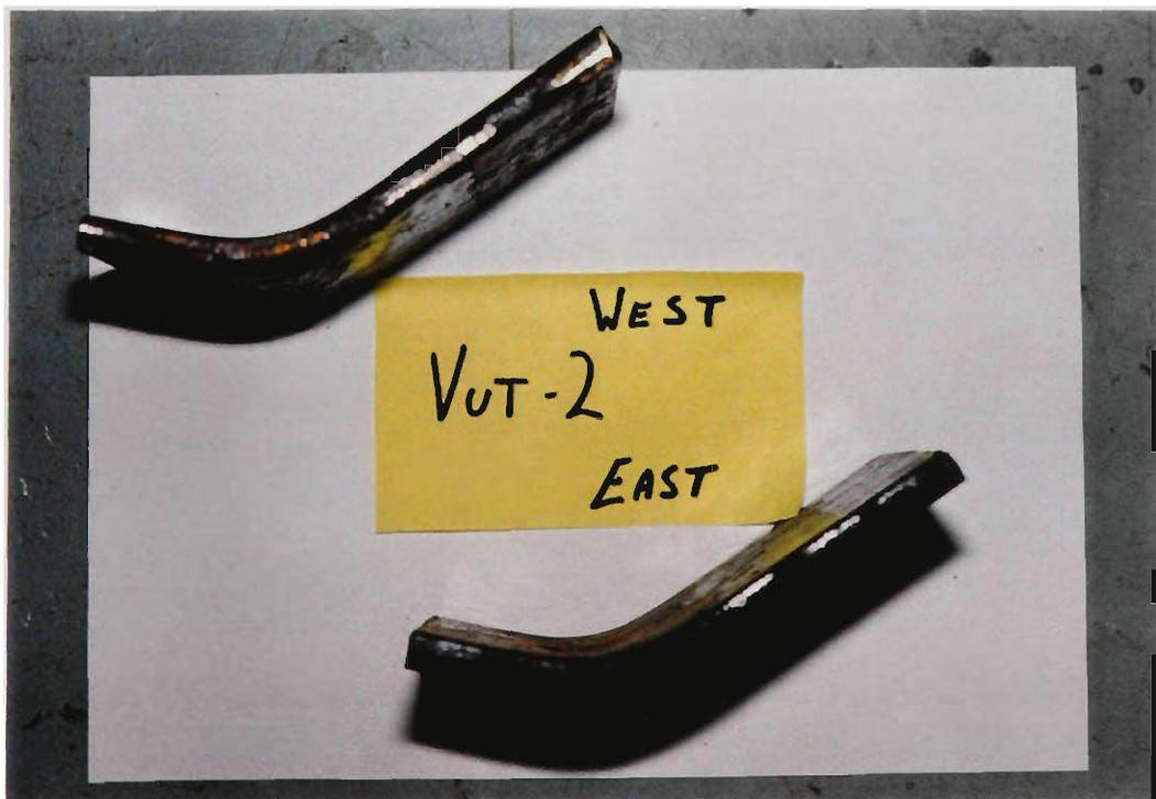
Figure 5.22 Final Plate Deformation of NW-600 Test
