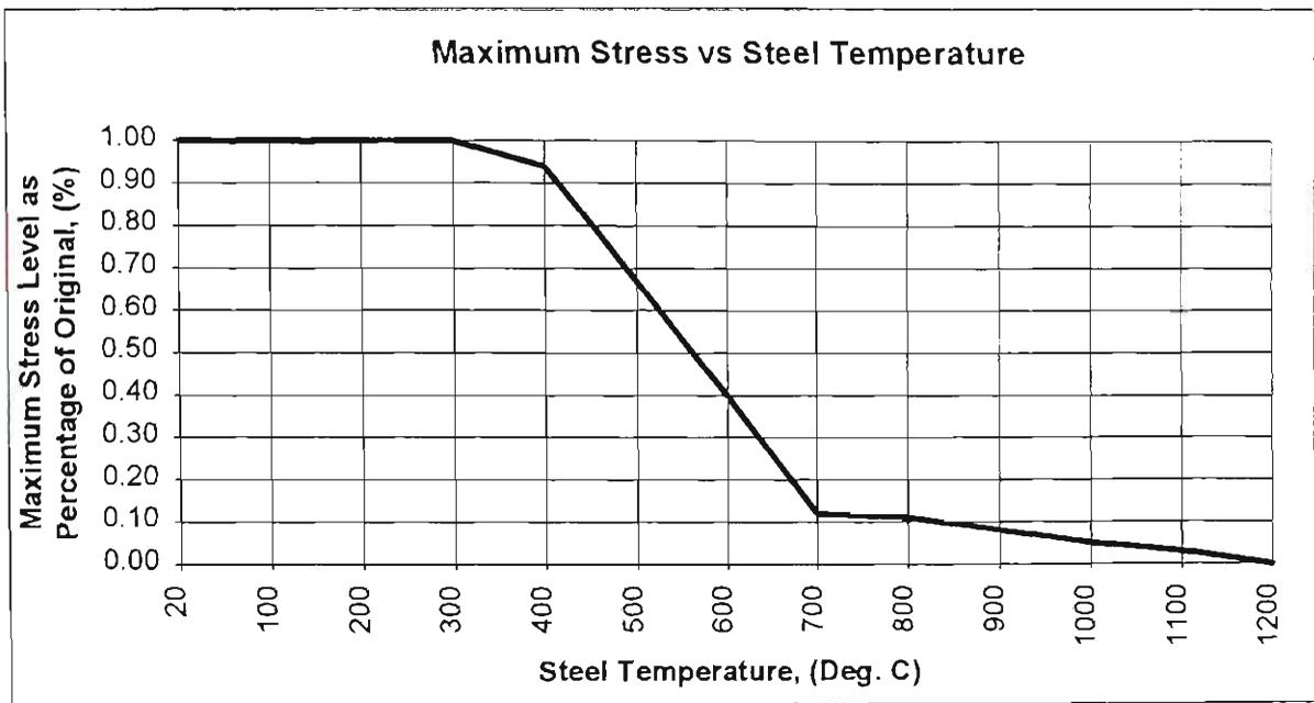
**Figure B.3:** Maximum Stress Level versus Temperature - (Steel)
