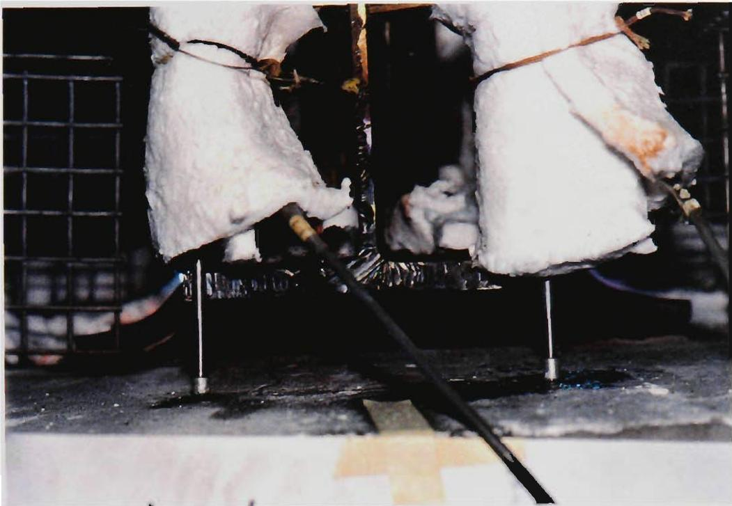
Figure 5.21 Deformation of NW-600 Clip Plate Test
