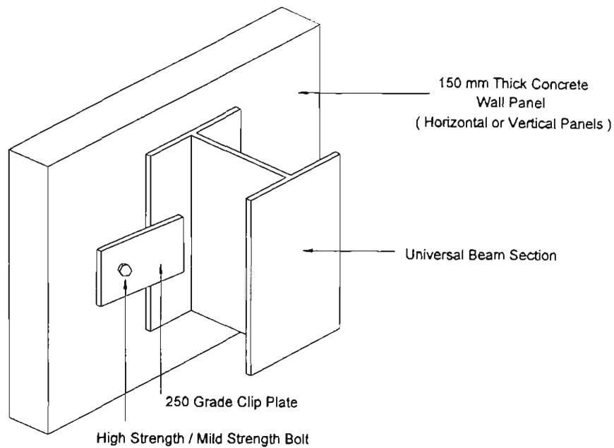
**Figure 5.3** Typical Clip Plate Bearing Connection Used in Experimental Testing
