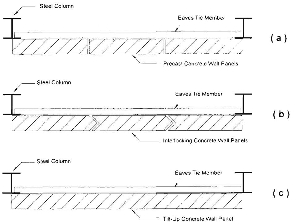
**Figure 2.5** Schematic View of Various Vertical Panel Lateral Support Systems
