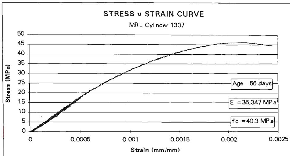
Figure E.3 Stress-Strain Relationship for Cylinder MRL 1307
