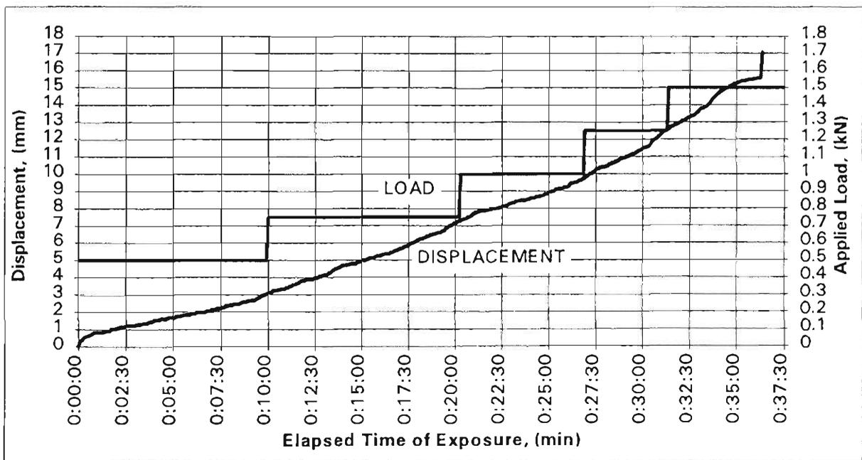
Figure 5.20 Creep Effects for Non-Welded Connection Tested at 800 °C
