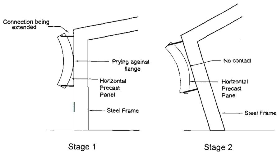
Figure 4.10 Interaction Between Deforming Horizontal Panel and Steel Frame
