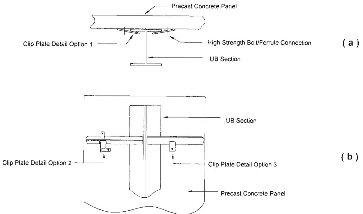
**Figure 2.6** Methods of Connection for Support in Fire
