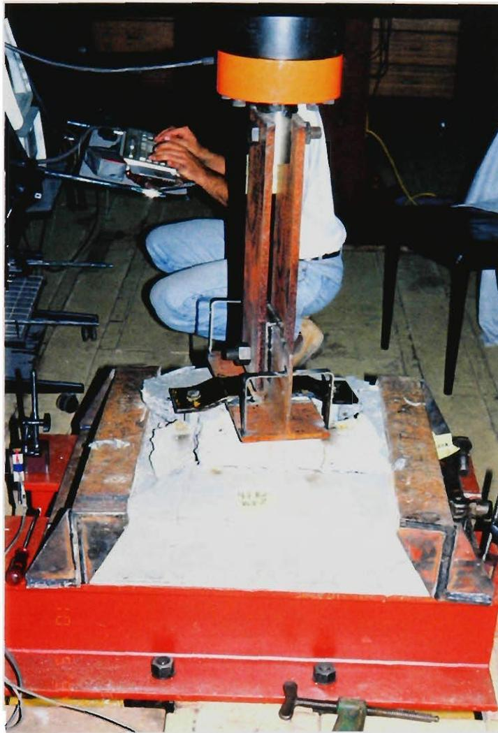
Figure 5.17 Premature Failure of Two-Way Support
