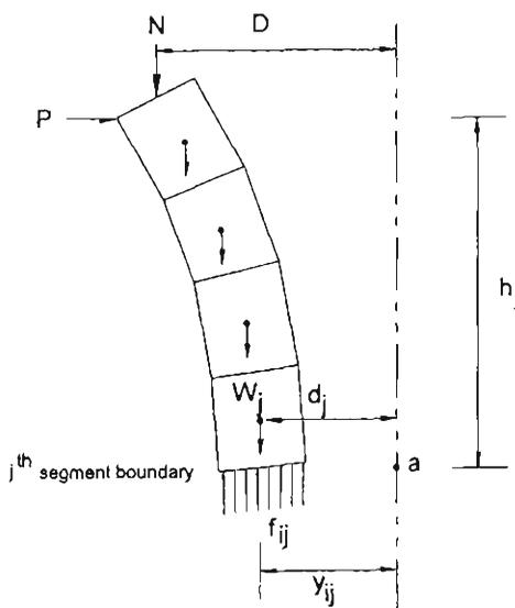
Figure 3.7 Equilibrium Equations for the Cantilevered Wall
