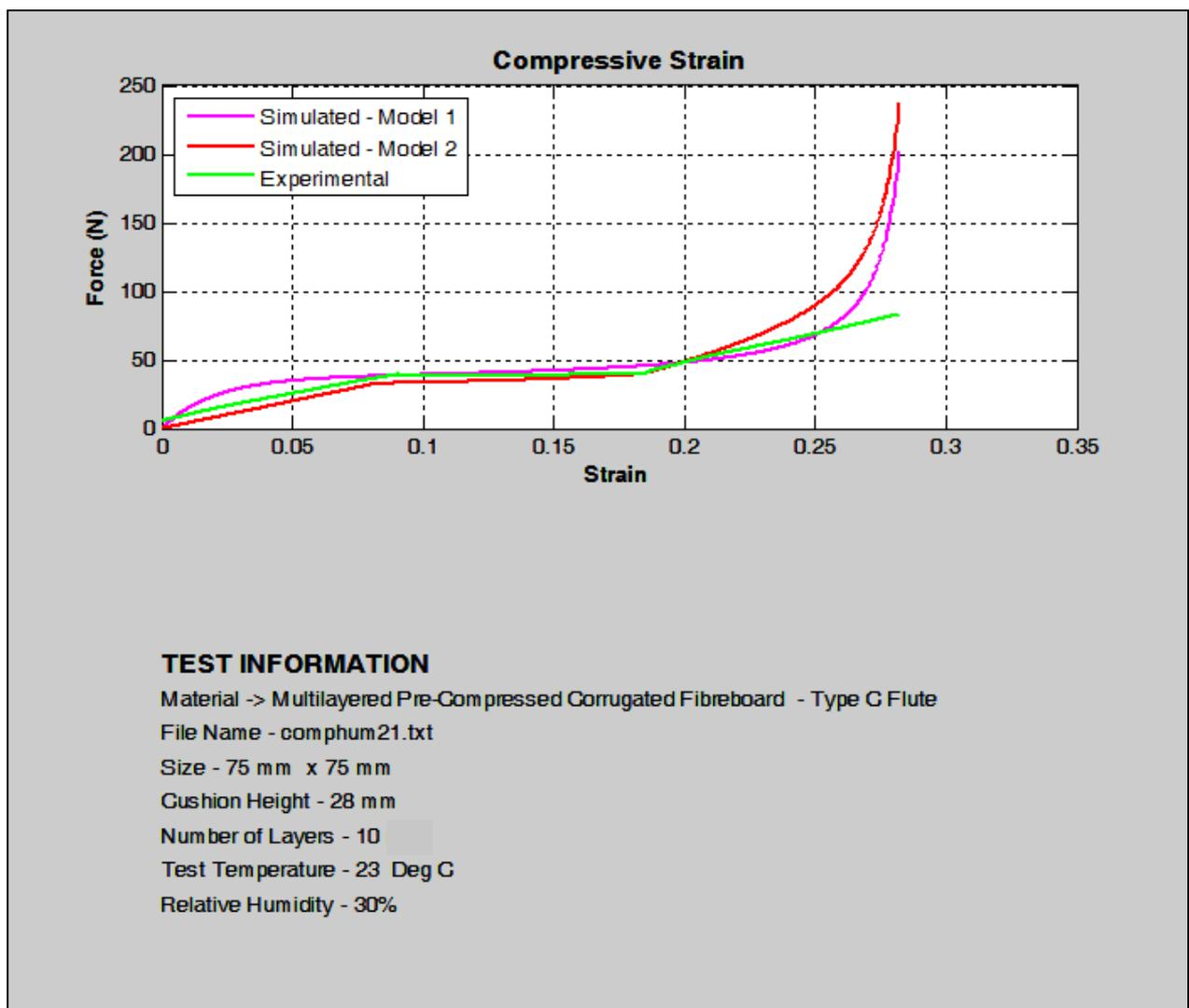
Figure 4.4 Compression and Simulation at 30% Humidity based on Equations 4.2 and 4.3
