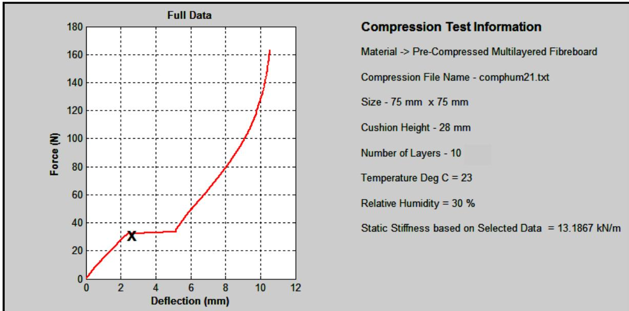
Figure 3.3 Typical Compression Test
