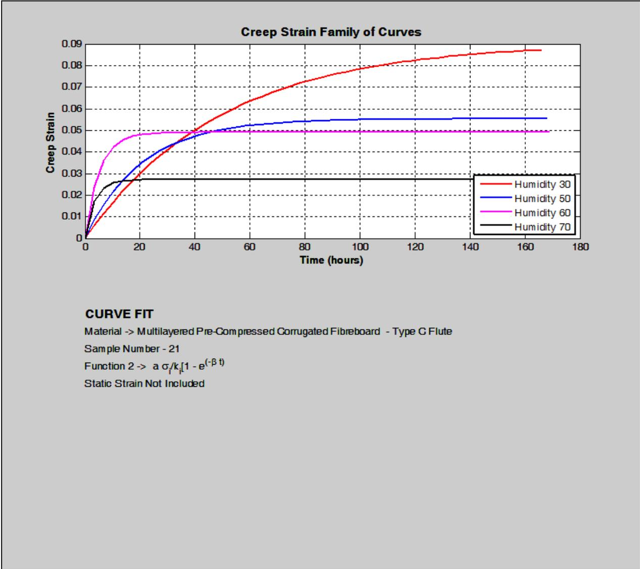
Figure 5.4 Simulated Curve Family for Sample 21 using Function 2 with no Static Strain
