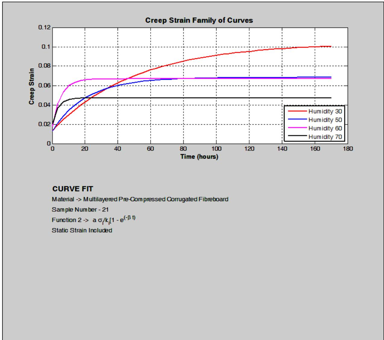
Figure 5.5 Simulated Curve Family for Sample 21 using Function 2 with Static Strain
