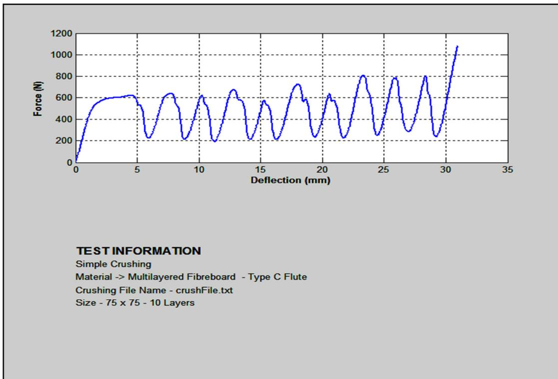
Figure 4.1 Typical Cushion Crushing Results
