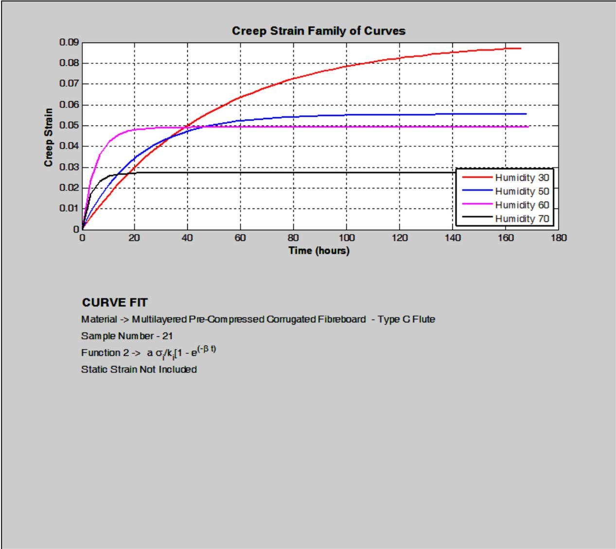
Figure 4.17 Simulated Curve Family for Sample 21 over the experimental Humidity Range, no Static Strain
