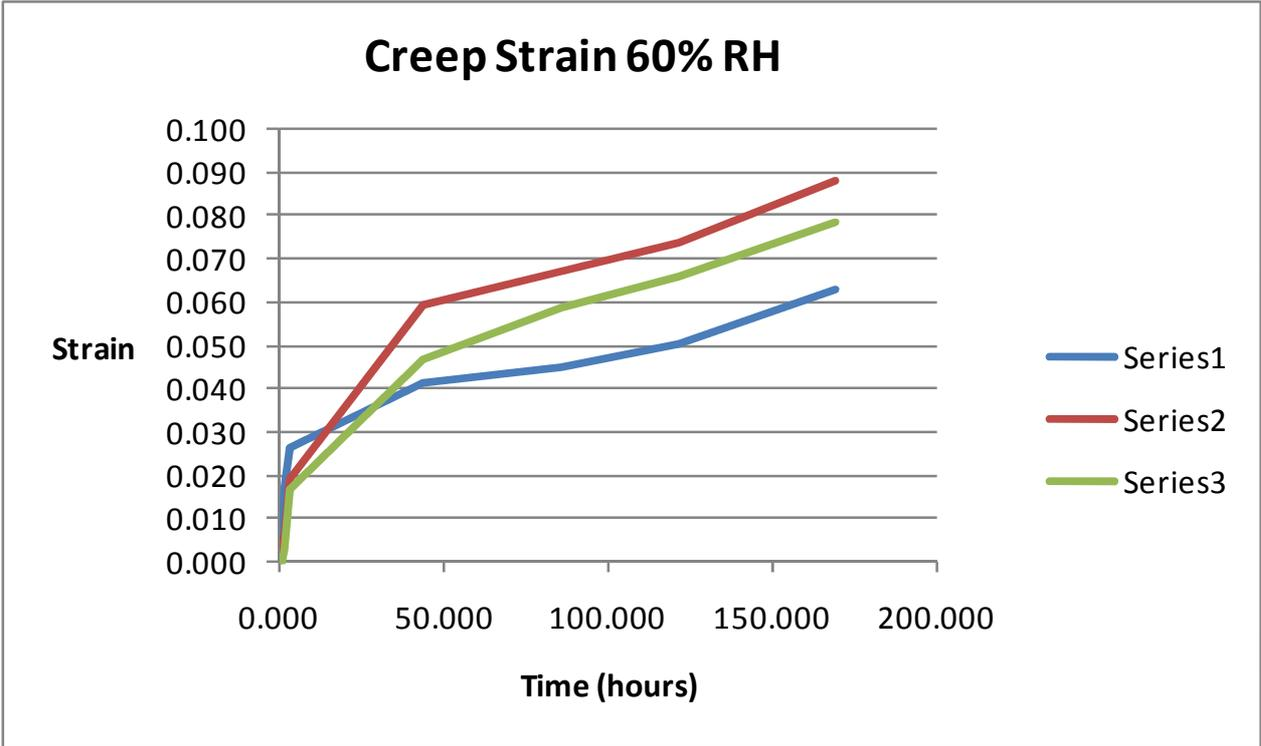
**Fig 3.7**Plot of Creep Strain Data at 60% RH
