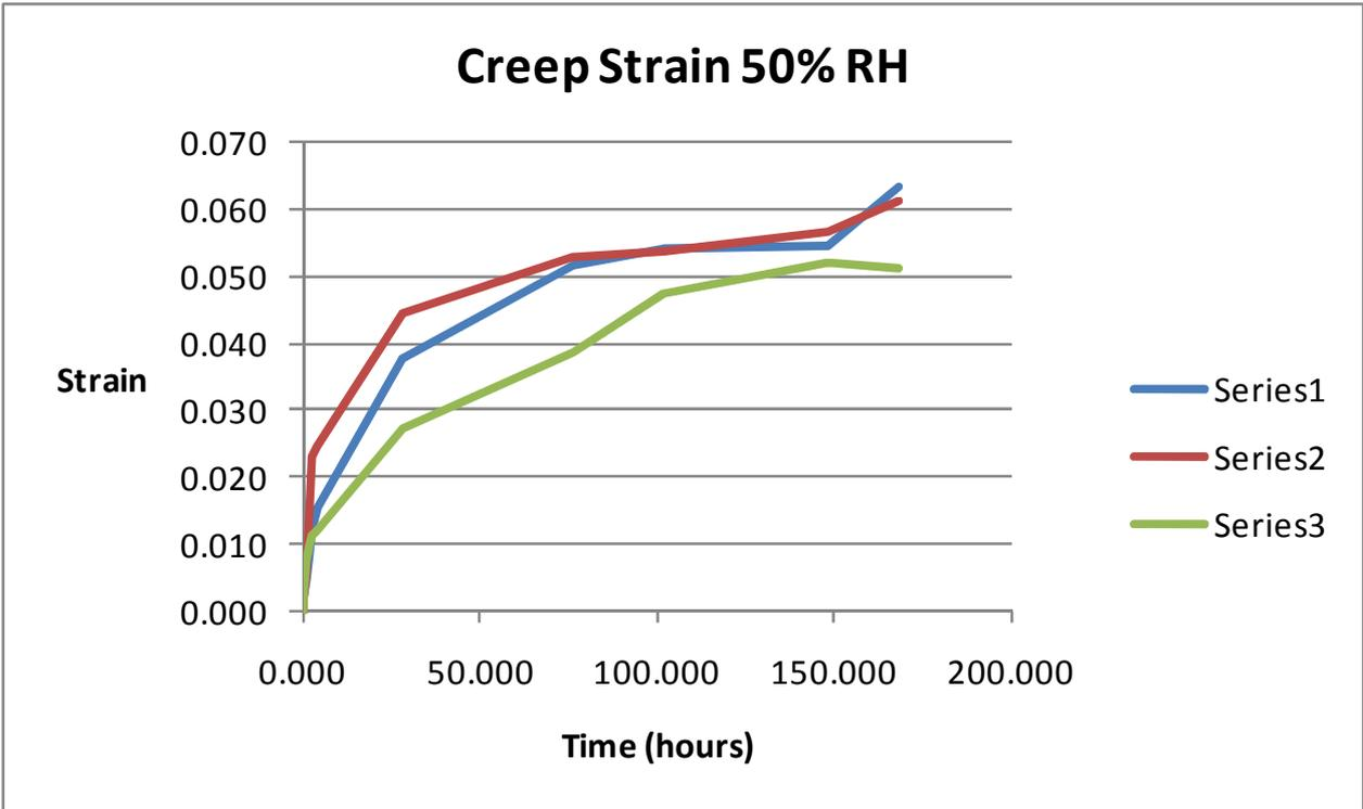
Figure 3.6 Plot of Creep Strain Data at 50% RH
