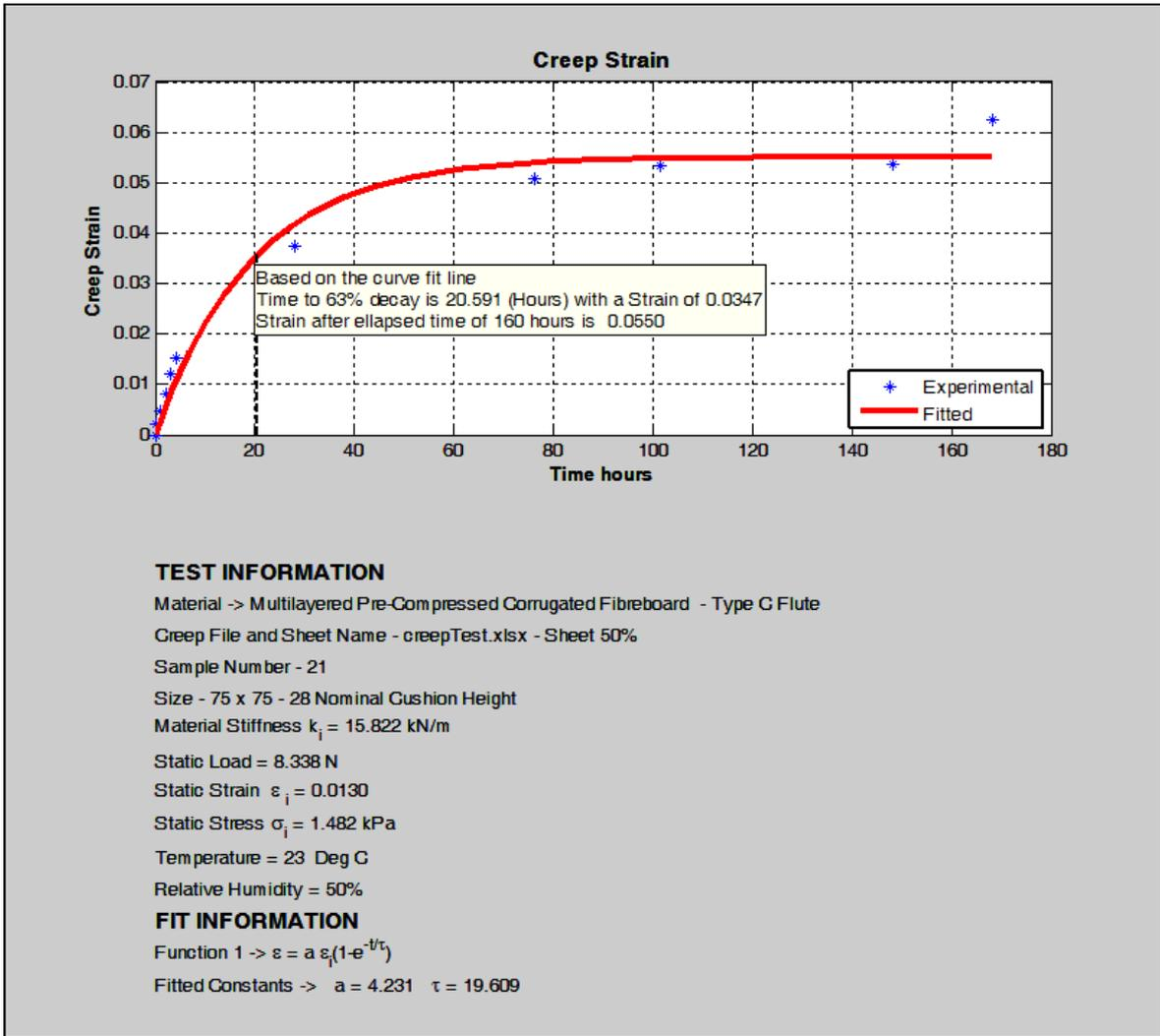
Figure 4.10 Creep Experimental and Simulation sample 21 at 50% RH using Equation 4.5
