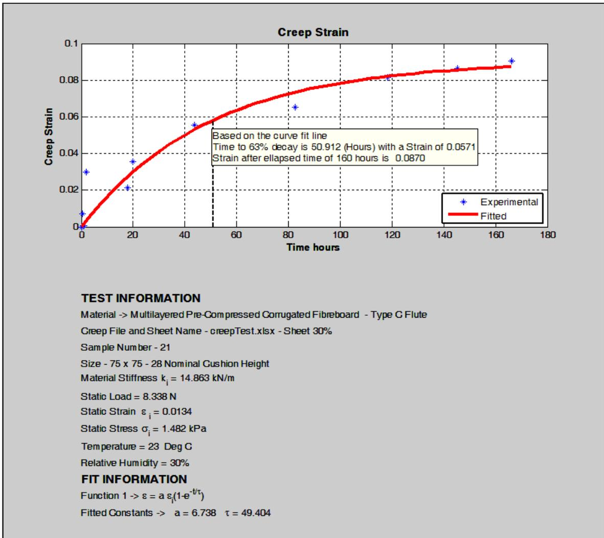
Figure 4.9 Creep Experimental and Simulation sample 21 at 30% RH using Equation 4.5
