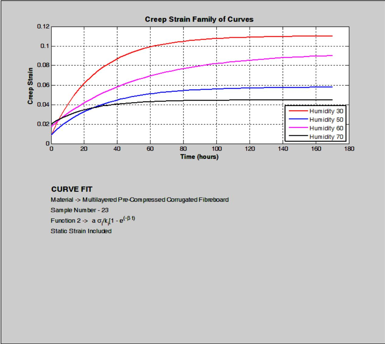
Figure 4.22 Simulated Curve Family for Sample 23 over the experimental Humidity Range, Static Strain
