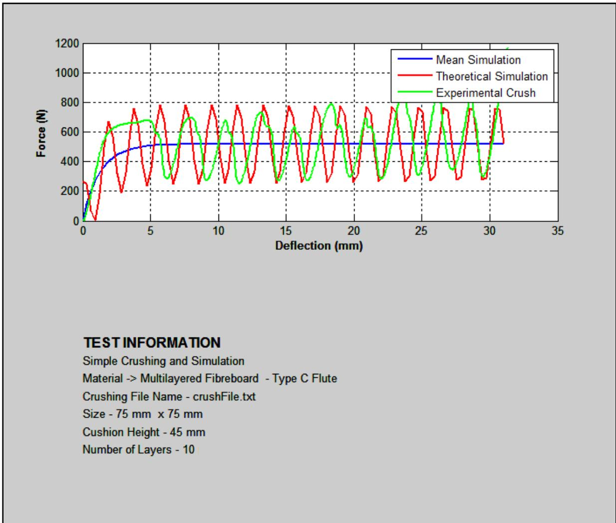
Figure 4.2 Pre-Compressing Mechanisms – Experimental and by Modeling
