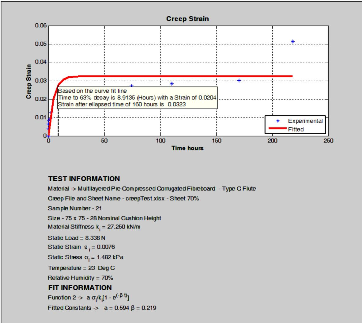
Figure 4.16 Creep Experimental and Simulation sample 21 at 70% RH using Equation 4.6
