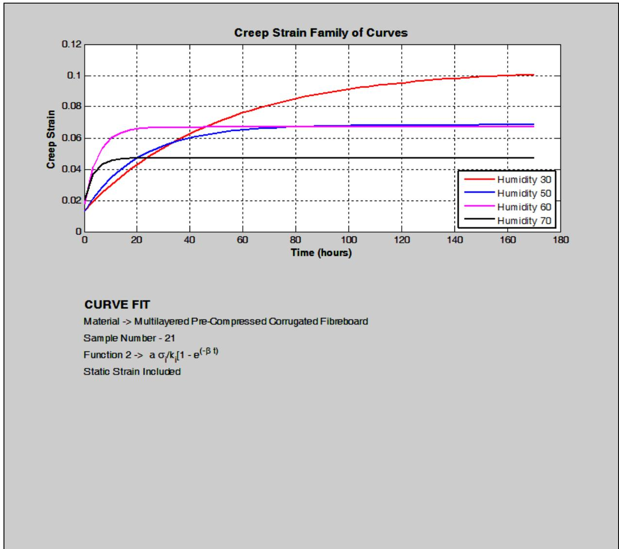
Figure 4.18 Simulated Curve Family for Sample 21 over the experimental Humidity Range, Static Strain
