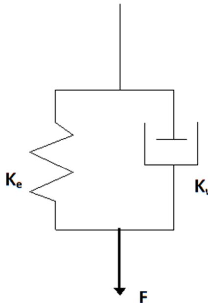
Figure 2.4 Voigt Model of Viscoelasticity
