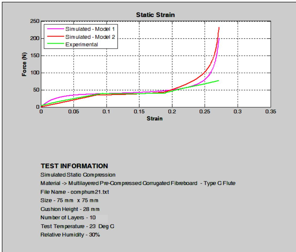
Figure 5.1 Cushion Compression and Simulation at 30% RH using Equation 5.1 and 5.2
