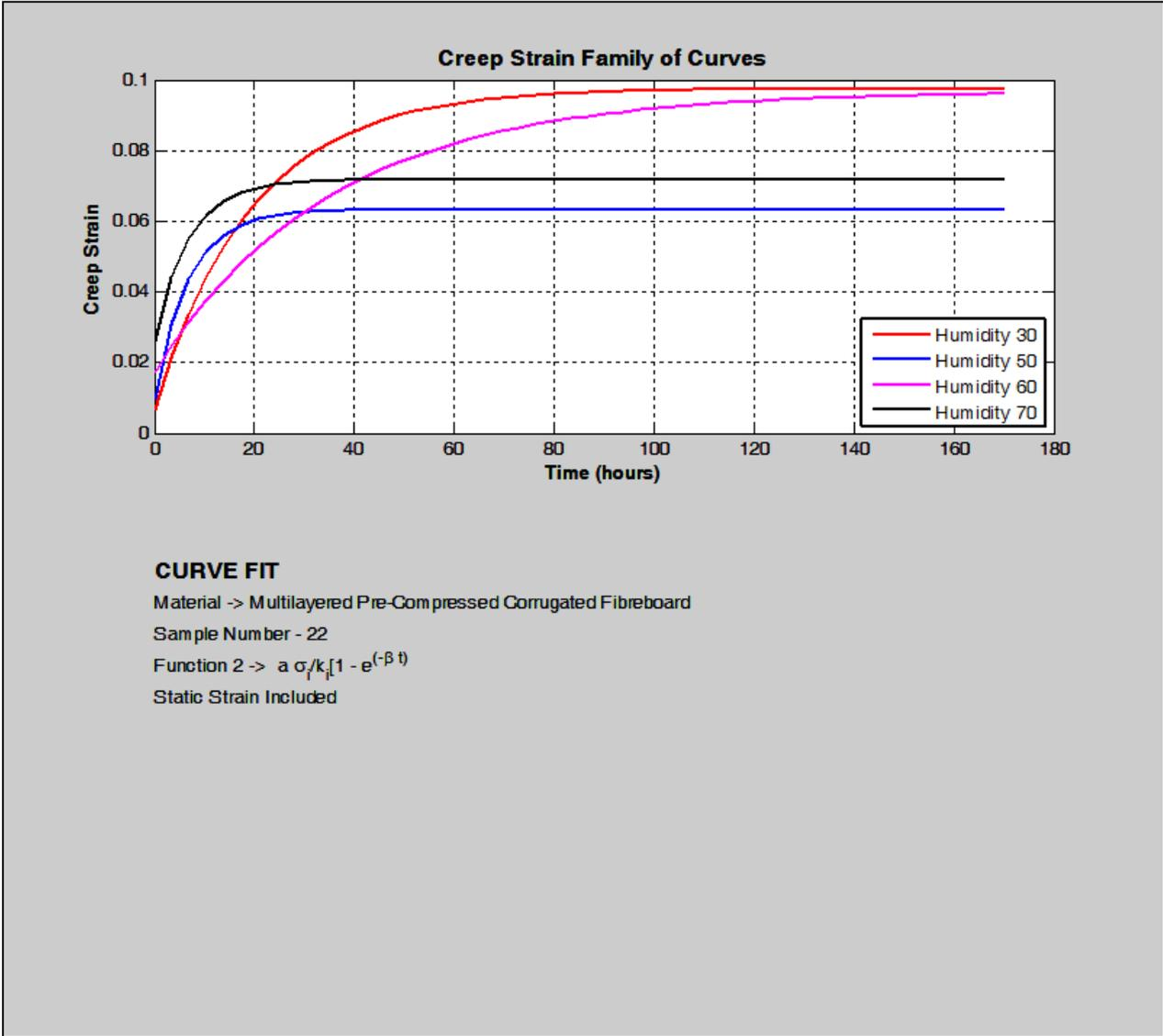
Figure 4.20 Simulated Curve Family for Sample 22 over the experimental Humidity Range, Static Strain
