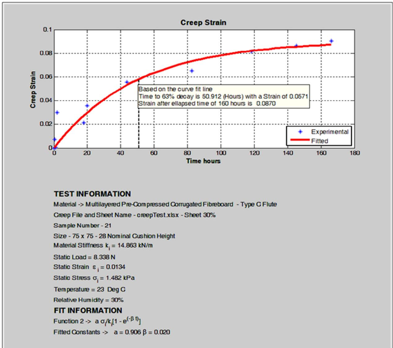
Figure 5.3 Typical Curve Fitting for sample 21 using equation 5.4
