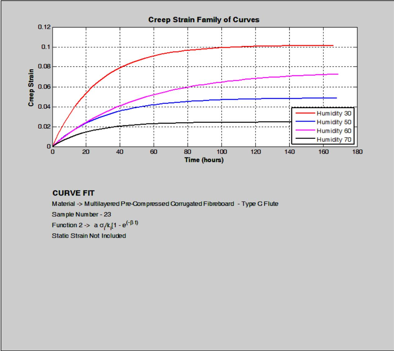
Figure 4.21 Simulated Curve Family for Sample 23 over the experimental Humidity Range, no Static Strain
