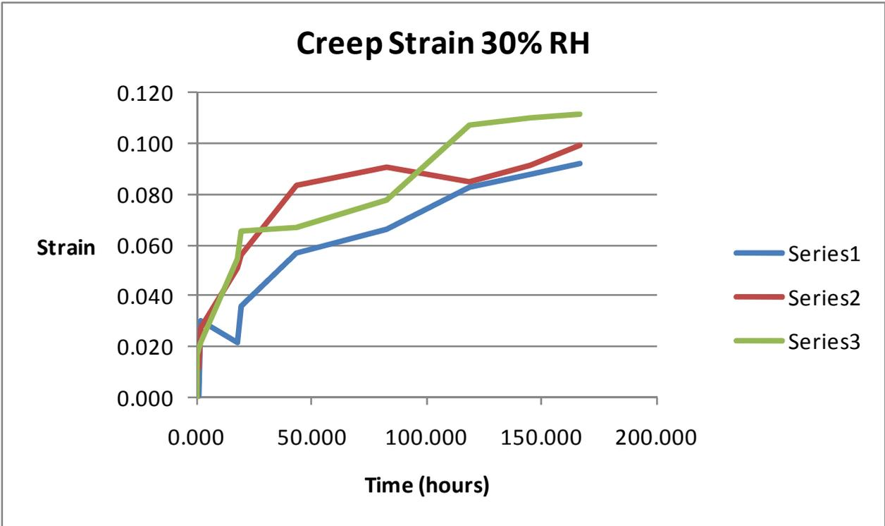
Figure 3.5 Plot of Creep Strain Data at 30% RH (Preliminary Test)
