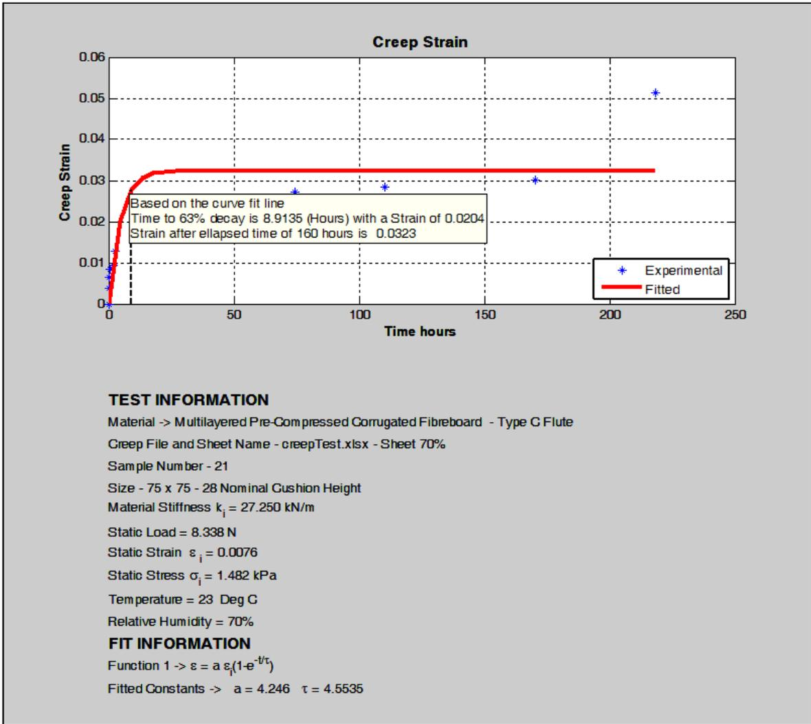
Figure 4.12 Creep Experimental and Simulation sample 21 at 70% RH using Equation 4.5
