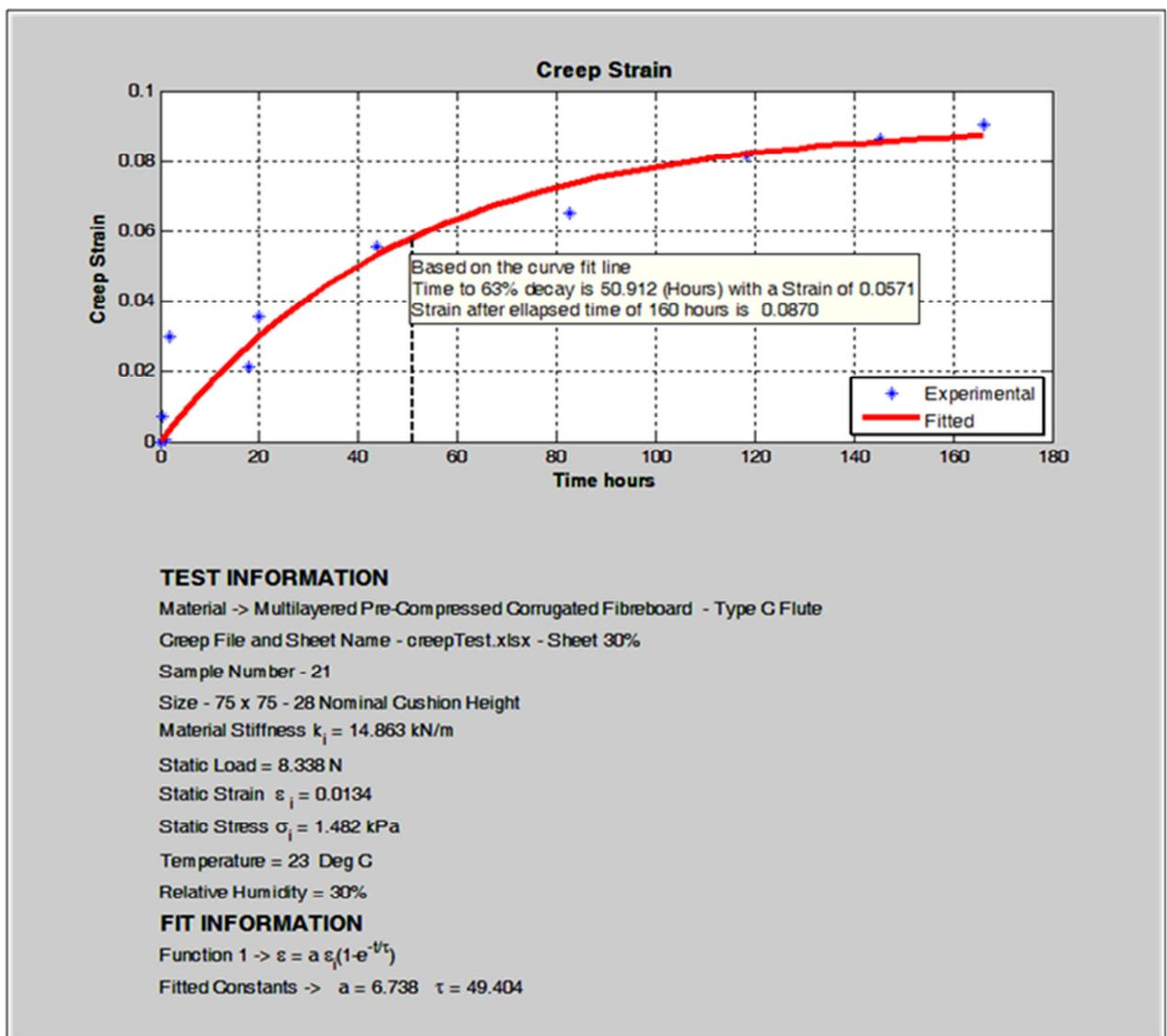
Figure 5.2 Typical Curve Fitting for sample 21 using equation 5.3
