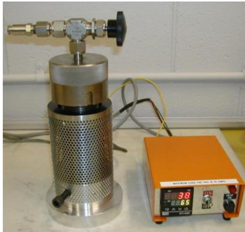
**Figure 3-3** Hydrogenation chamber located at VU
