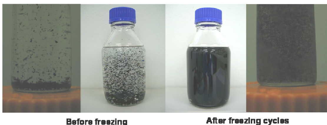
Figure 3-22 Improvement of the CNT dispersion after 3 freezing cycles
