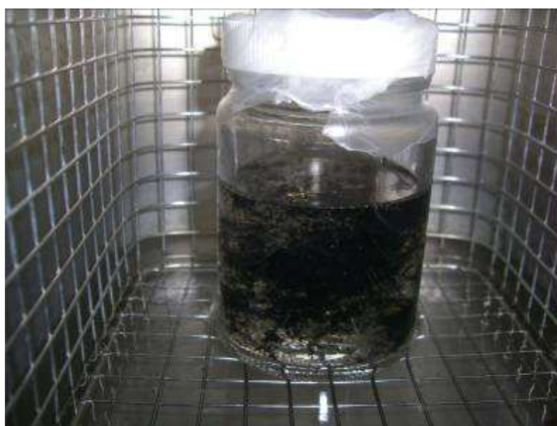
Figure 3-9 Example of solution sonicated in the bath sonicator. The bath is composed of deionised water
