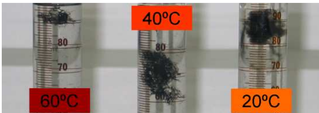
Figure 3-19 Dispersion state after sonication at 20, 40 or 60 °C for 30 min; this picture was taken after 180 min of rest and the CNTs were fully settled into bundle structures
