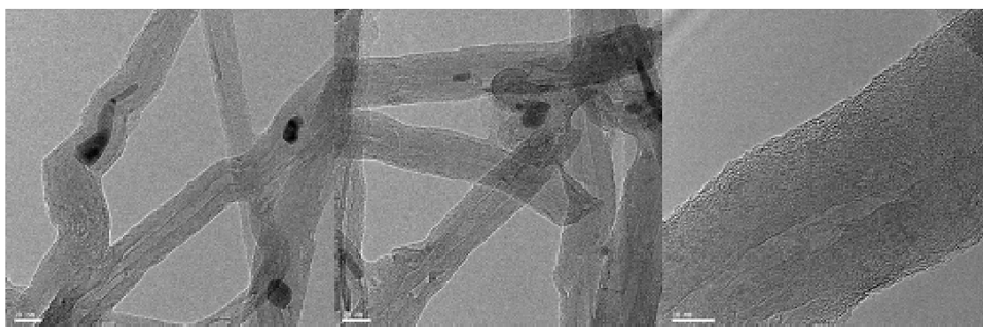
Figure 3-5 TEM of CCI CNTs after high shearing dispersion
