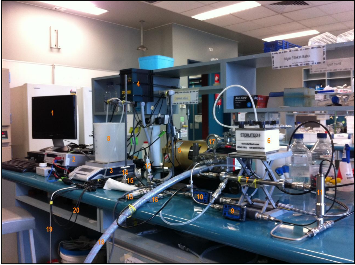
Figure 3.1: Experimental test rig used during membrane experiments. 1 – desktop computer for data logging, 2 – power meter, 3 – balance, 4 – variable speed drive, 5 – positive displacement pump, 6 – flat sheet test cell, 7 – ceramic membrane module, 8 – plastic container, 9 – feedwater flowmeter, 10 – reject water flowmeter, 11 – feedwater pressure recorder, 12 – reject water pressure recorder, 13 – product water pressure recorder, 14 – product water valve, 15 – reject water valve, 16 – recirculation valve, 17 – discharge pressure gauge, 18 – inlet line, 19 – reject line, 20 – pH and conductivity probes.
