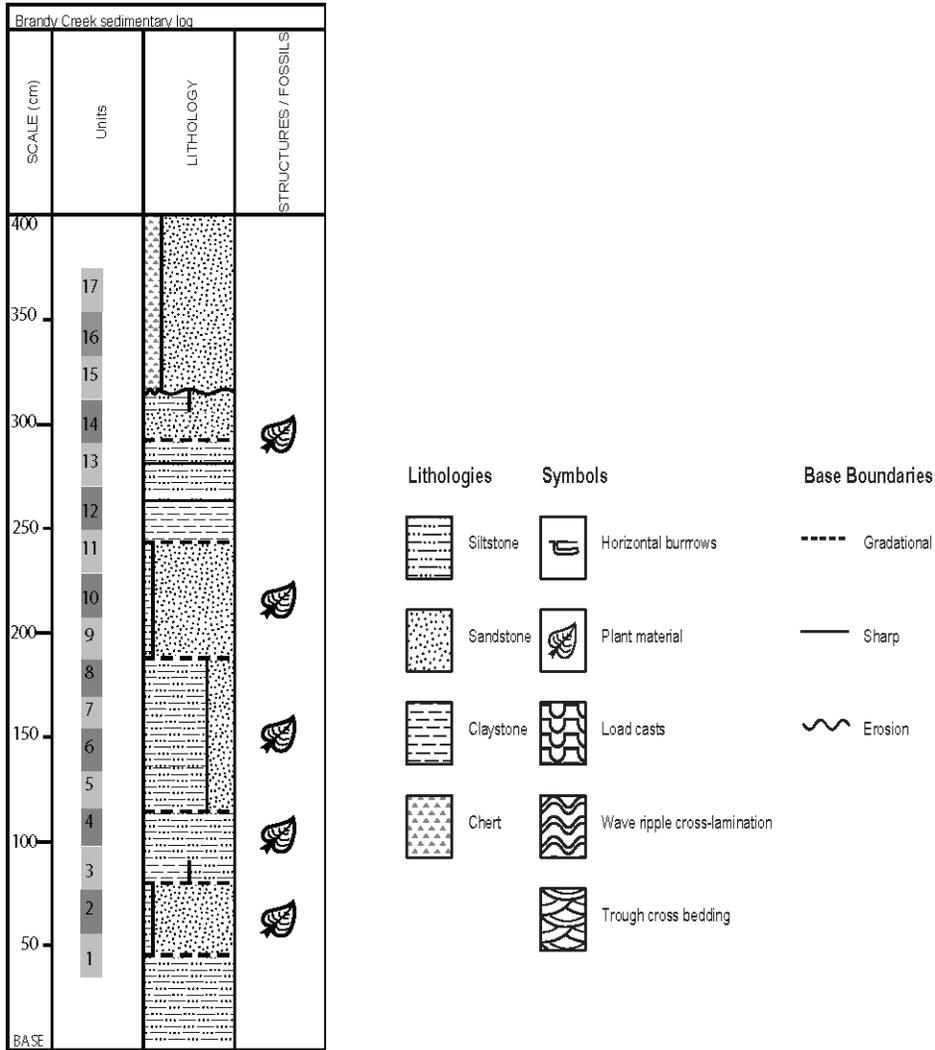
**Figure 2.2** Stratigraphic log of the Brandy Creek outcrop showing units, lithology and fossil structures present.
