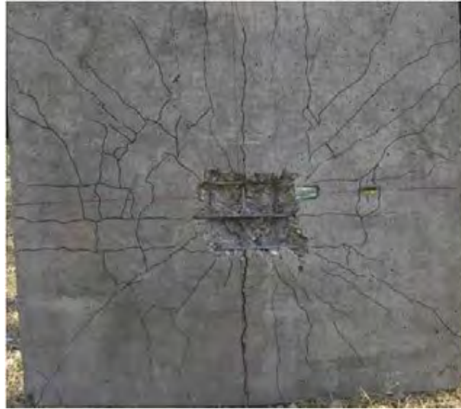
Figure 5.31: Spalling damage of Panel D – Experimental
