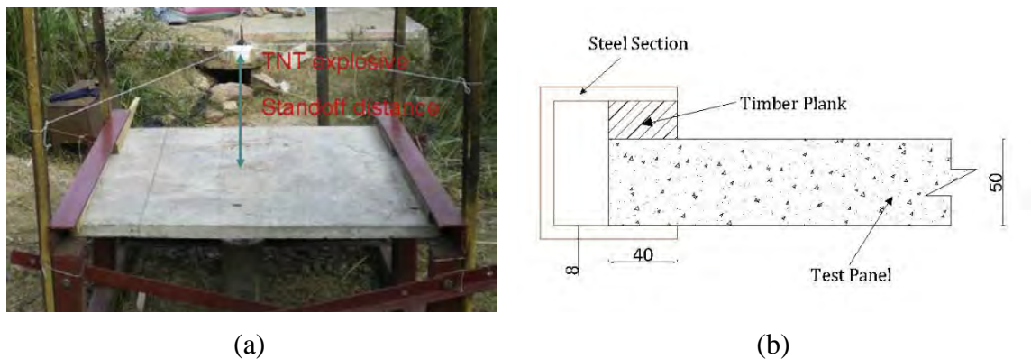
Figure 5.5: Fixing assembly detail for test panels (Source: Wang et al., 2012)
