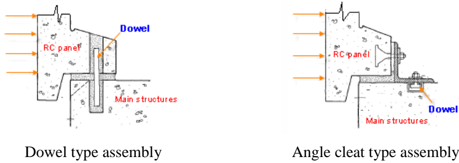
Figure 5.2: Typical fixing assemblies for concrete panels (Source: Brookes, 1998)
