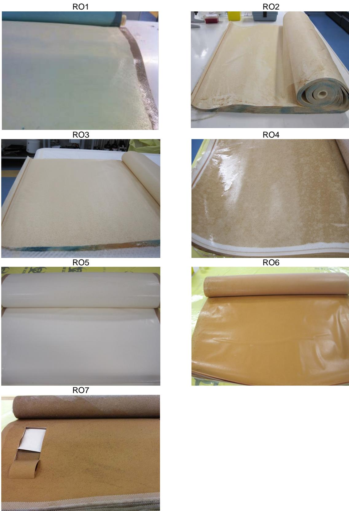
Figure SI 1. Photographs of the RO membranes from seven full-scale RO plants.
