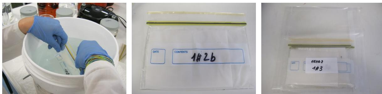
*Step 1. The coupons were enclosed in oxygen barrier plastic bags (resealable bags) with 20 mL*
