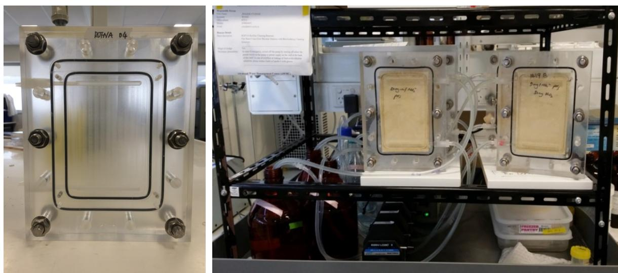
Figure 5. Photographs of the tailored cleaning cell (left); Cleaning system with five cleaning cells in parallel, cleaning solutions are recirculated by a peristaltic pump with five pump heads for 24 hours.
