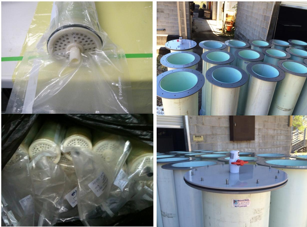
*Method 1. Module stored in vacuum sealed bags to simulate membrane preservation for storage out of the plant.*
