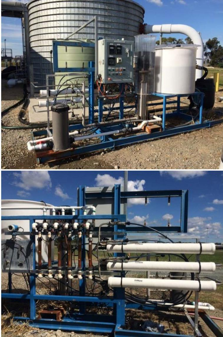
Figure 16. Photographs of the RO pilot-plant.
