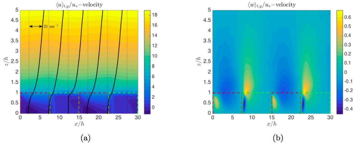
Figure 2 Contours of nondimensional average  $u$ -velocity with superimposed profiles of average  $u$ -velocity at a range of locations along the canopy. Note the contours (colours) are nondimensional but the profiles have an approximate dimensional scale as indicated. (b) Vertical velocity in the whole domain showing the strong up- (yellow) and down-drafts (blue) above and within the canopies. The canopy stripes are shown as dotted outlines.
