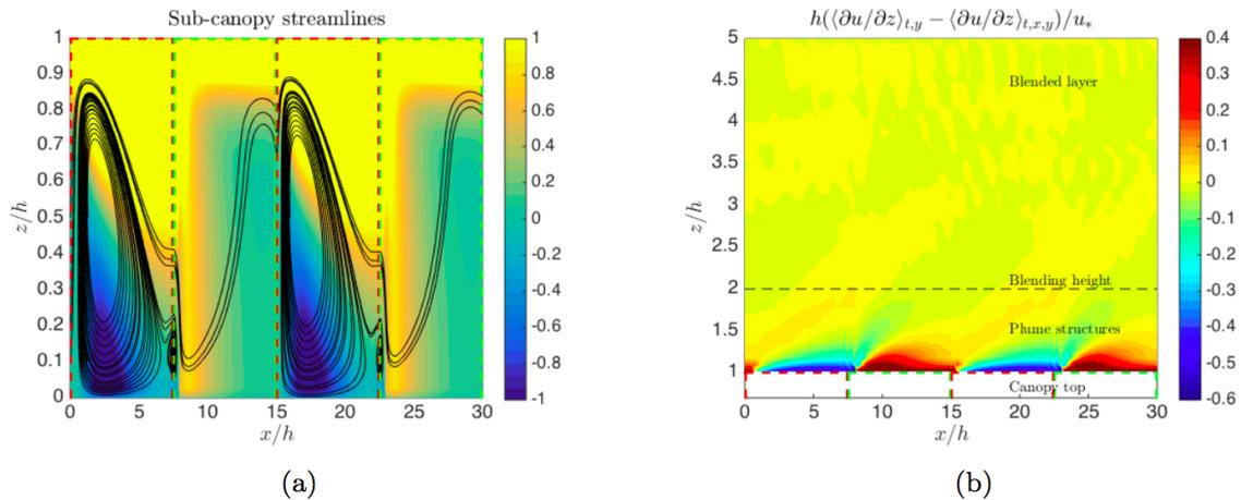
Figure 3 (a) Streamlines highlighting two recirculation vortices within the canopy. Superimposed on the nondimensional average  $u$ -velocity. (b) Contours of averaged velocity gradient difference above the canopy, clearly showing the plume structure immediately above the canopy. Above the blending height is a well-mixed boundary layer characterised by negligible fluctuations in the velocity gradients. Sub-canopy flow is omitted from this figure. The canopy stripes are shown as dotted outlines.
