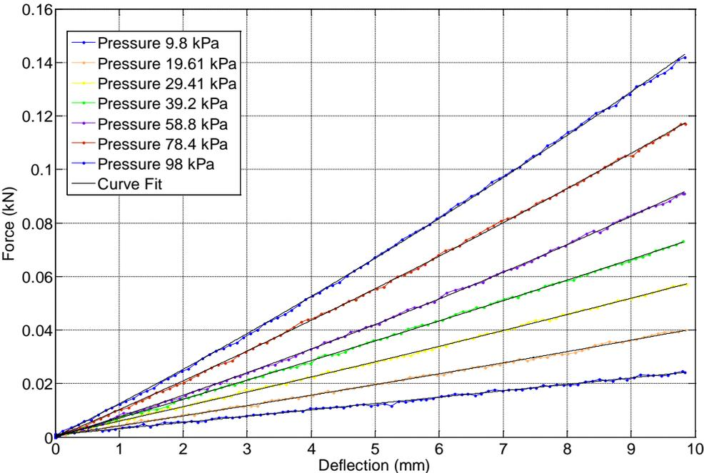
Figure 5. Inflated bladder / indenter compression characteristics
