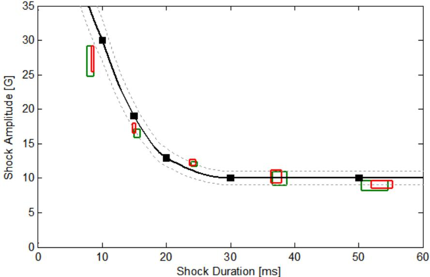
Figure 13: Trigger thresholds for magnet type indicator (10 g) along with published threshold values.
