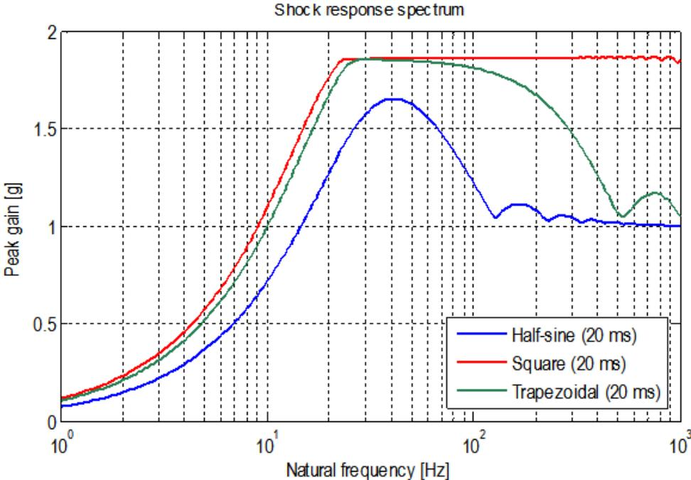
Figure 1. SRS for various shock pulse shapes.
