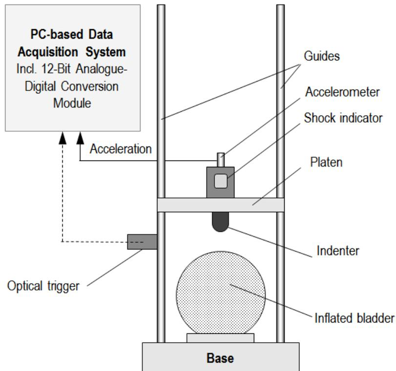
Figure 6. Free-fall shock generation apparatus.
