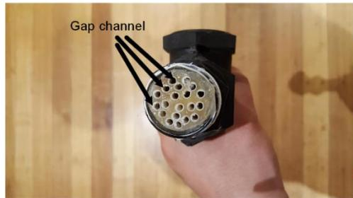
b) gap channel density (top view)
