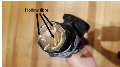
d) hollow fibre packing density (top view)
