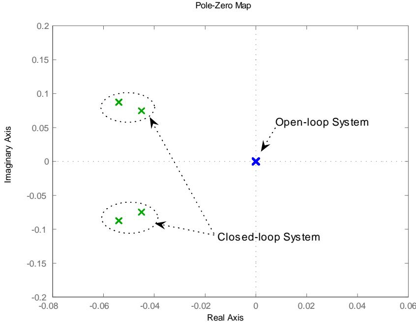
Fig. 2. Poles of open- and closed-loop systems.
