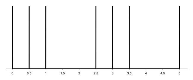
Figure 4.1: Flash pattern of the strobe lights as a function of time in seconds (cycle of three is repeatedly ongoing)
