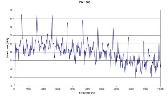
Figure F.2: Spectral analysis of the 85 dBA 520 Hz square wave in the testing bedroom. The fundamental frequency was found to be approximately 516 Hz.
