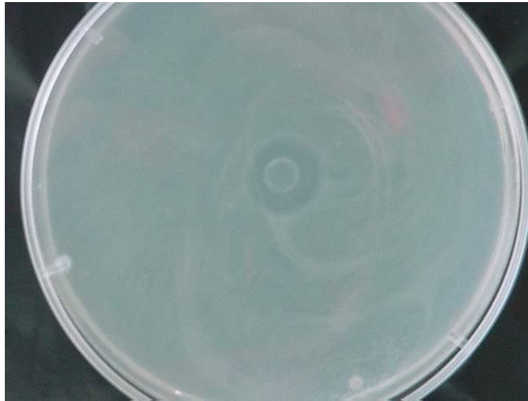
Fig. 1. Growth inhibition of E. coli by LLDPE film containing linalool or methylchavicol after 1 year of storage.
