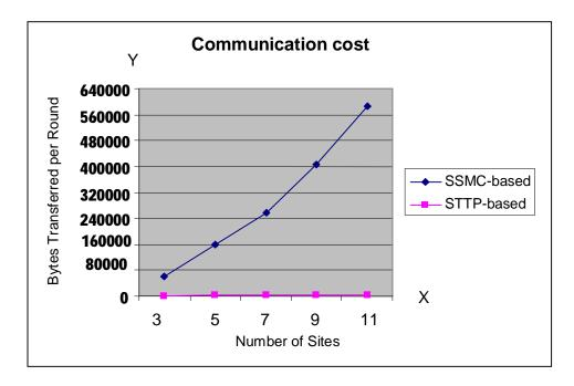
Figure 12: Communication cost comparison for association rules
