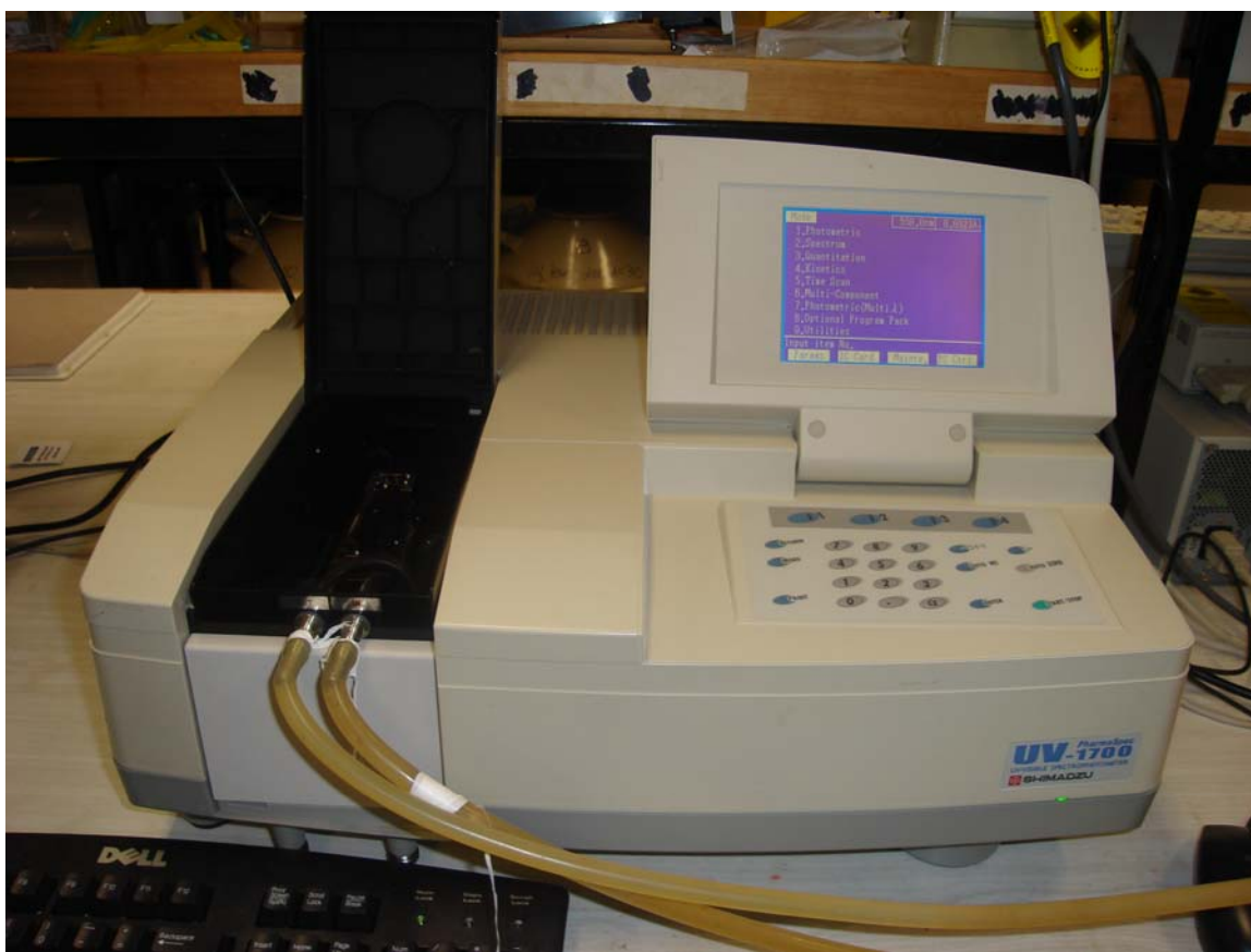
Figure 2.10. Temperature-controlled UV-1700 Pharma Spec UV-visible spectrophotometer used to quantitatively determine CS activity and protein concentration.
