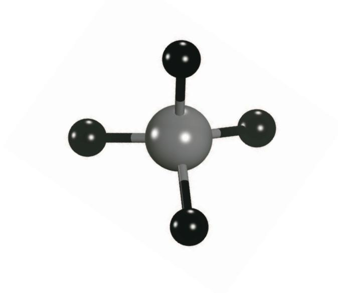
**Figure 4.1:** Tetrahedral structure of  $\text{SiO}_4^{2-}$ , showing 4 oxygen atoms surrounding the central silicon atom. [89].
