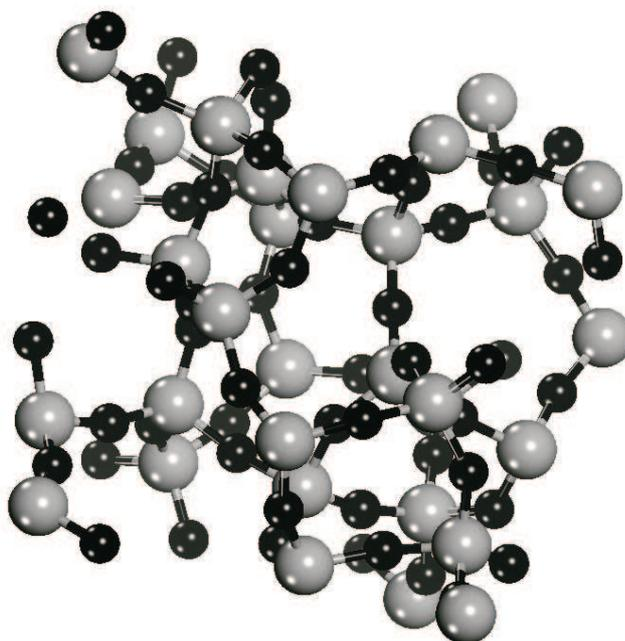
**Figure 4.2:** 3 - dimensional structure of SiO<sub>2</sub>, showing the interconnection of the tetrahedral units [89].
