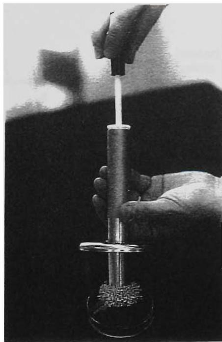
**Figure 2.1 :** Laboratory Magnetic Tester for harvesting oil-laden magnetic particles
