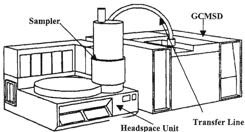
**Figure 7.2:** Example of a headspace (HS 40) coupled to a HP 5890 GC system (courtesy of Perkin-Elmer Australia and Hewlett-Packard Australia).
