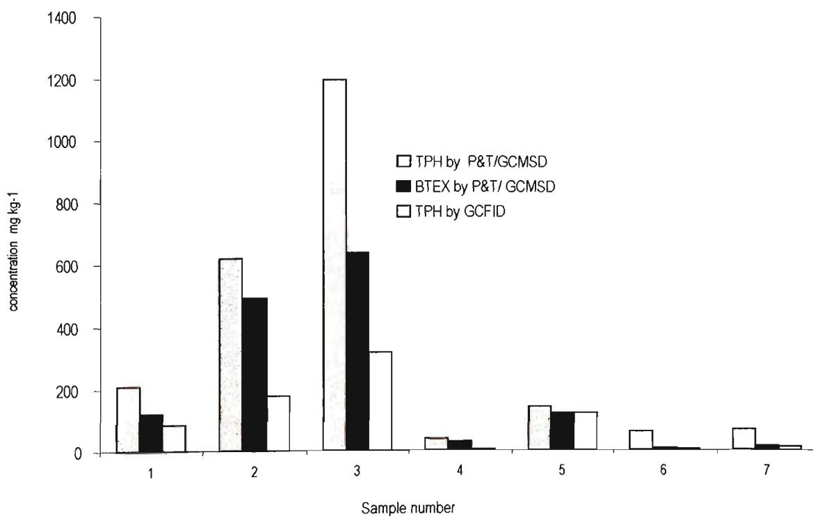
**Fig 8.5:** Comparison of BTEX and TPH(C<sub>6</sub>-C<sub>9</sub>) by P&T/GCMSD with TPH (C<sub>6</sub>-C<sub>9</sub>) by GCFID
