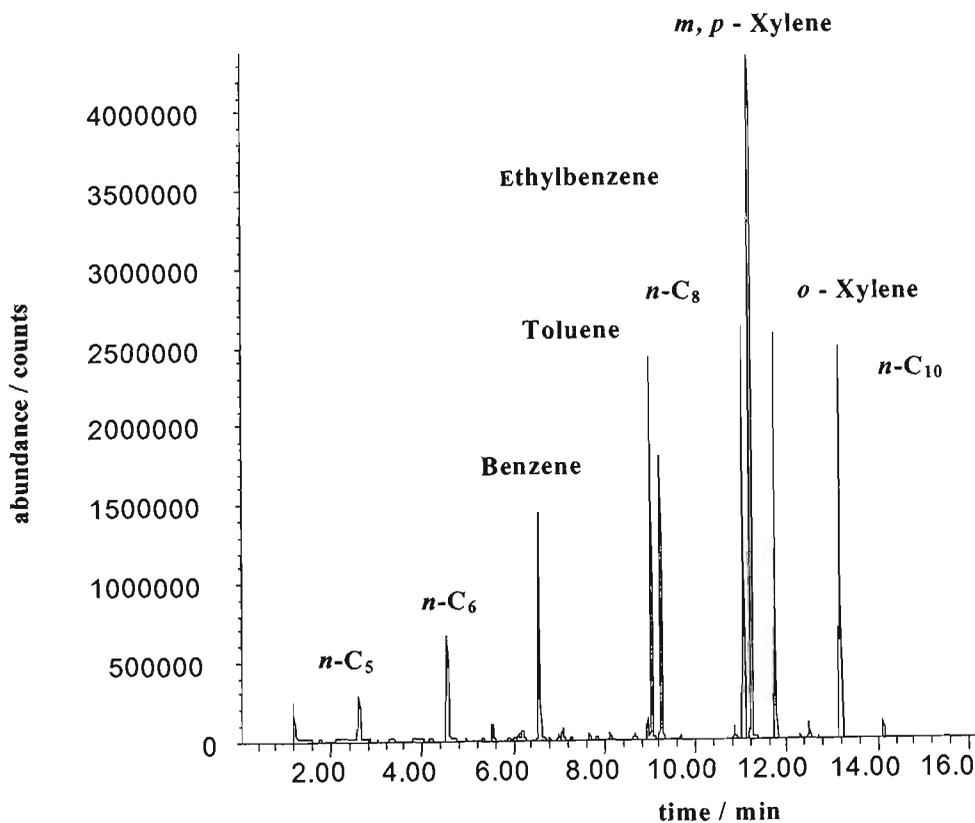
**Figure 8.2:** Profile of the TPH (C<sub>6</sub>-C<sub>9</sub>) standard containing aliphatic and aromatic hydrocarbons.
