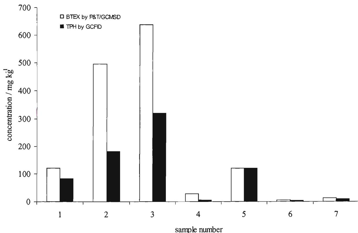
**Figure 8.1:** Comparison of BTEX and TPH (C<sub>6</sub>-C<sub>9</sub>) concentrations determined by P&T/GCMSD and GCFID.
