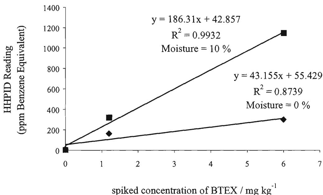
**Figure 2.5:** HHPID measurements of BTEX-spiked silt at different moisture contents.
