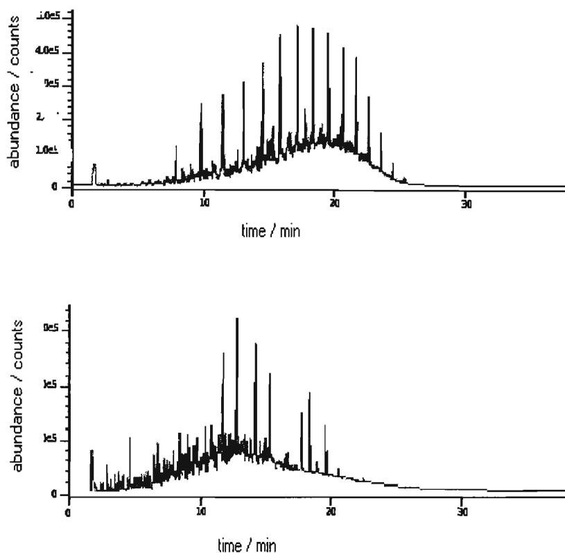
**Figure 1.4:** Un-weathered (top) and weathered (bottom) profiles of diesel (Weisman, 1998)<sup>1</sup>.
