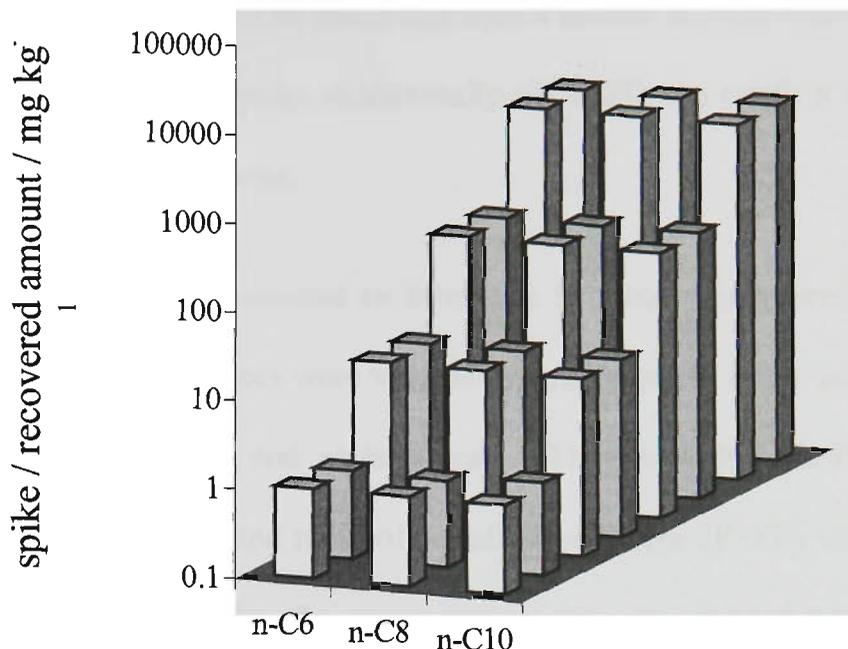
**Figure 8.4:** Comparison of Spiked *n*-Alkane concentrations at 10, 100, 1000 and 10000 mg/kg, with Recovered Levels. No Pairs of Values was Found to be Significantly Different at the 95% Confidence.
