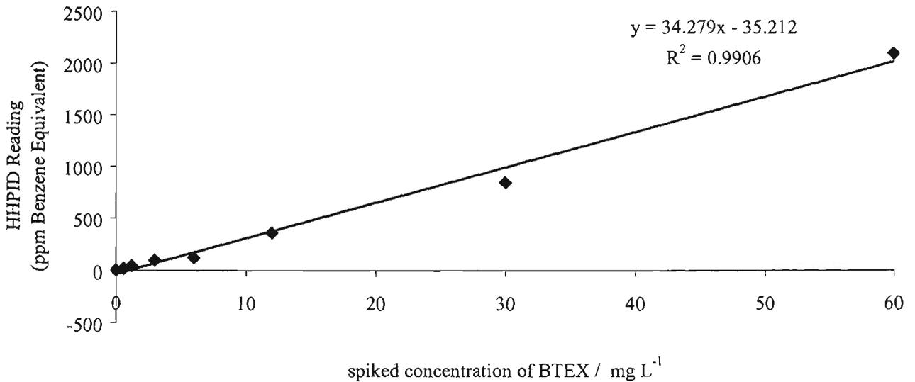
**Figure 2.2:** HHPID determination of BTEX-spiked water samples.
