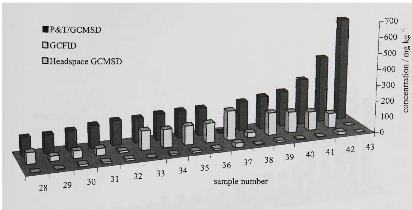
**Figure 7.6:** BTEX concentrations for clay soils (higher range).
