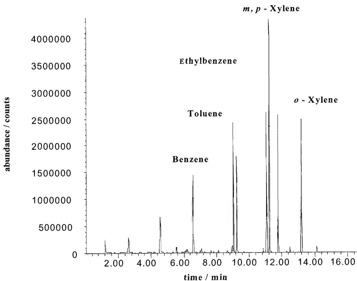
**Figure 7.3:** Total ion chromatogram of BTEX representing each component.
