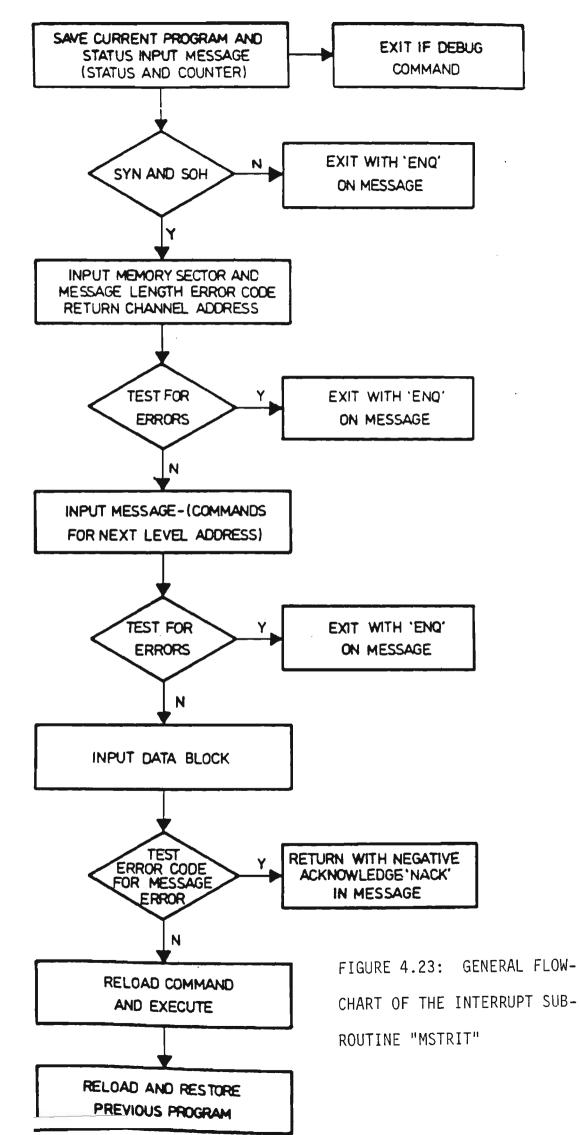
The detailed flowcharts in Appendix B represent the sequence of action carried out by the high speed data link sub-routines, ("MSTRIT", "SLV1IN" and "SLV2IN") of the model.
