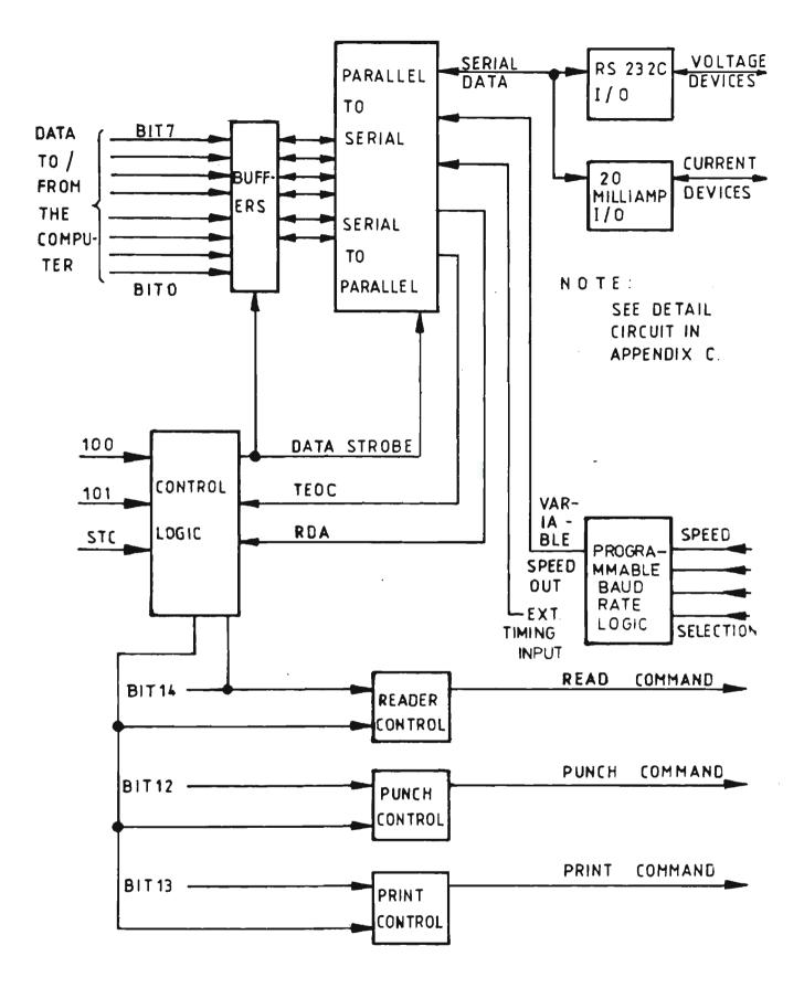
FIGURE 4.11 : SIMPLIFIED BLOCK DIAGRAM FOR THE SERIAL DATA INTERFACE CARD
