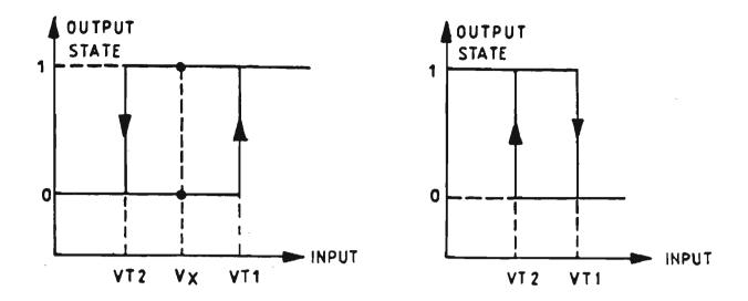
FIGURE 4.12B : THE INPUT/OUTPUT RELATIONSHIP OF THE SCHMITT TRIGGER
