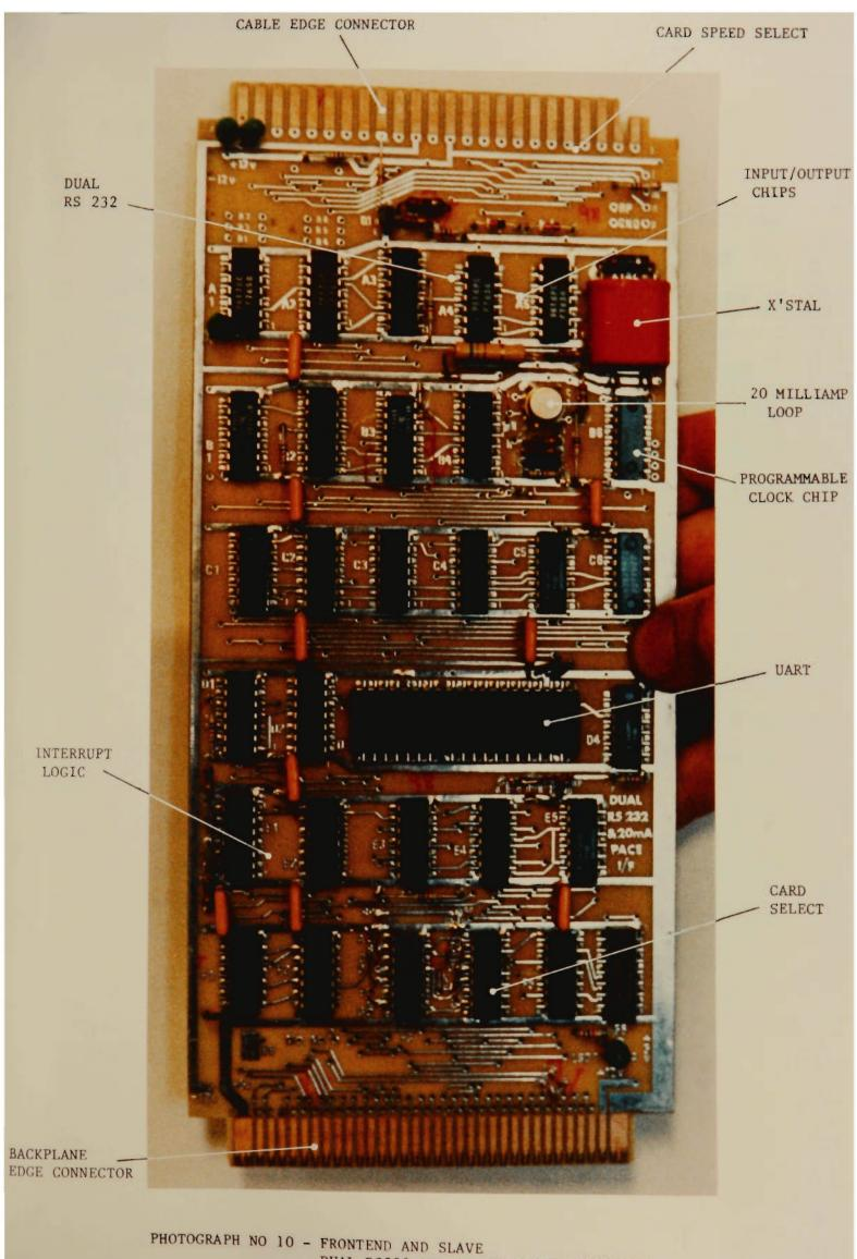
DUAL RS232 AND 20 MILLIAMP INTERFACE - HIGH SPEED SERIAL DATA LINK 4.2.4.2 The Basic Building Blocks of the High Speed Interfaces
