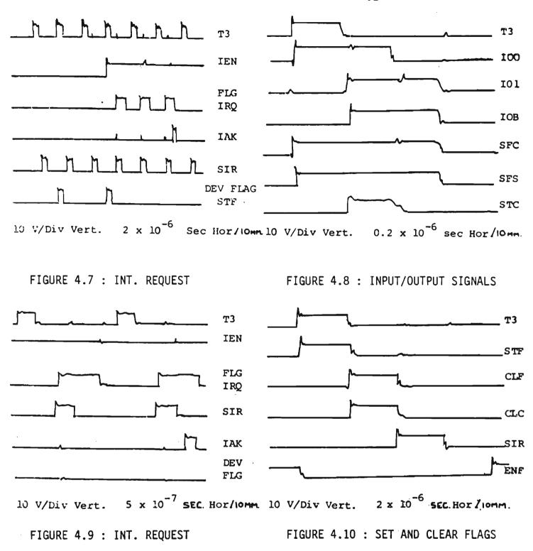
The following paragraphs show how the computer backplane signals were combined with the UART flags to implement the basic data transfer requirements for transmitting and receiving:
