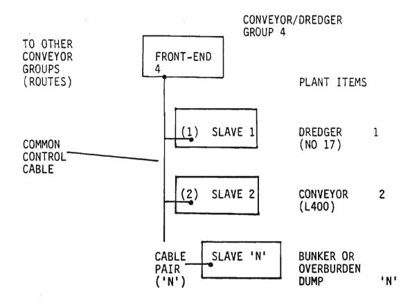
FIGURE 4.1 : COMMON CABLE FOR SUB-SYSTEMS OF THE SAME GROUP
