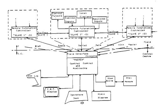
Figure 4 System Configuration - "DIRECT INTERFACING WITH SLA"
