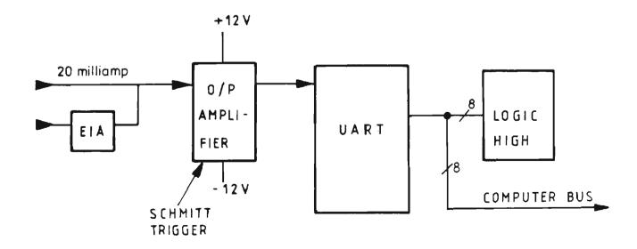
FIGURE 4.12A : BASIC INPUT BLOCK DIAGRAM
