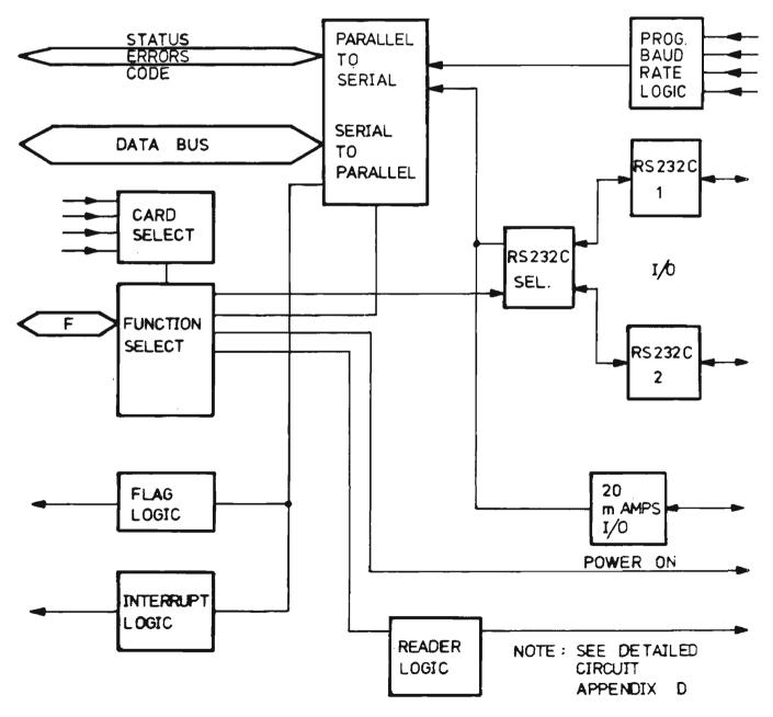
FIGURE 4.16 : A SIMPLIFIED BLOCK DIAGRAM FOR THE PACE
