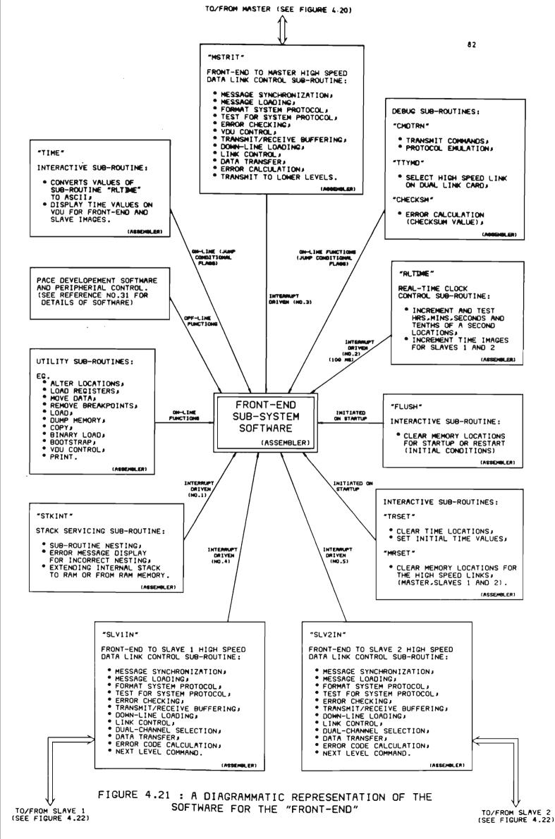
Sub-routine Priorities: The stack service sub-routine had the highest priority of all front-end sub-routines. As each sub-routine transferred the return address of the interrupted sub-routine and the contents of the registers to the internal stack, a check was made to determine if the number of words transferred to or from the internal stack had exceeded ten. This sub-routine could be initiated at any time but it did depend on the number of words on the stack during the transfer.
