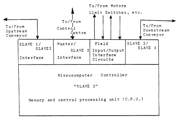
FIGURE 3.4 : INTERFACE REQUIREMENTS FOR A REMOTE SUB-SYSTEM
