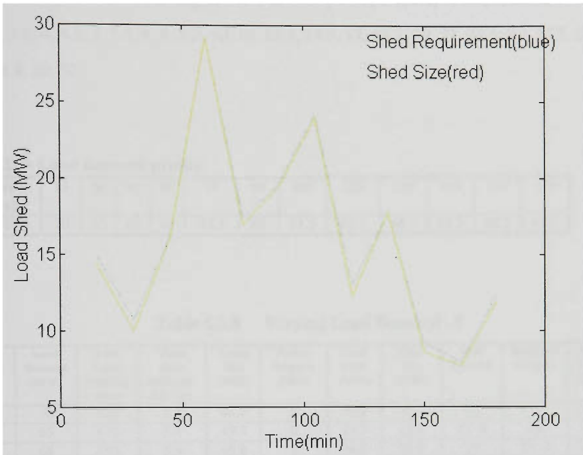
Figure 6.14 Comparison of Shed Requirement vs Shed Size in periods of variable Load Demand between 55.5 to 66.5 MW
