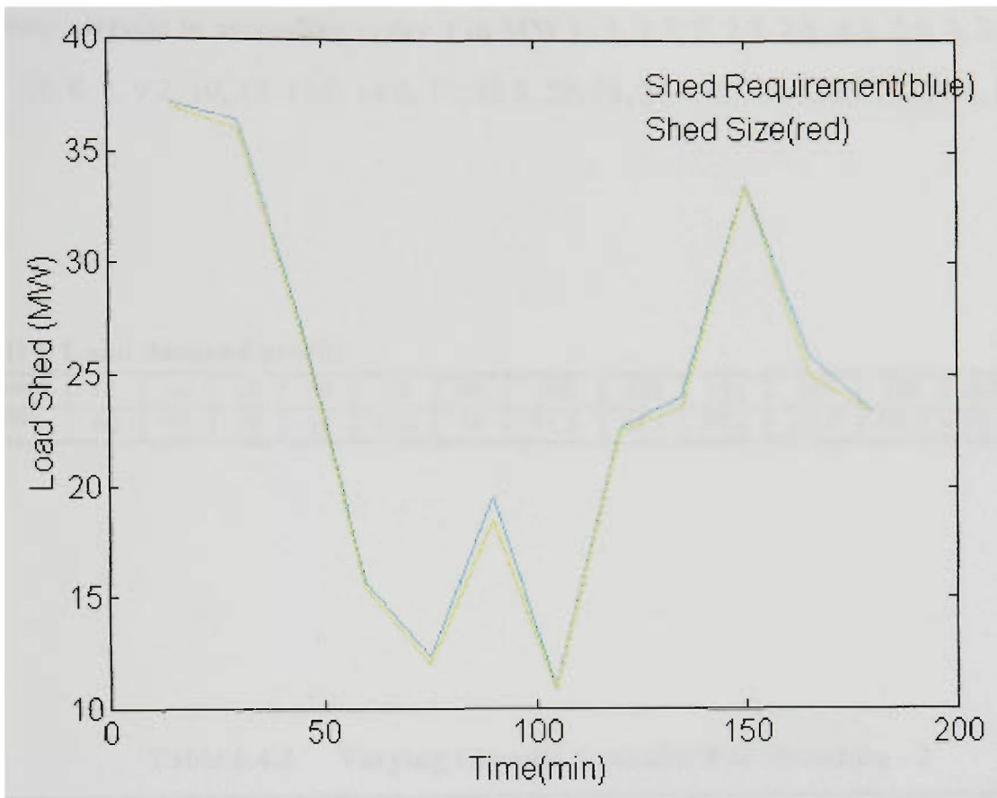
Figure 6.16 Comparison of Shed Requirement vs Shed Size with 36 circuits available for shedding.
