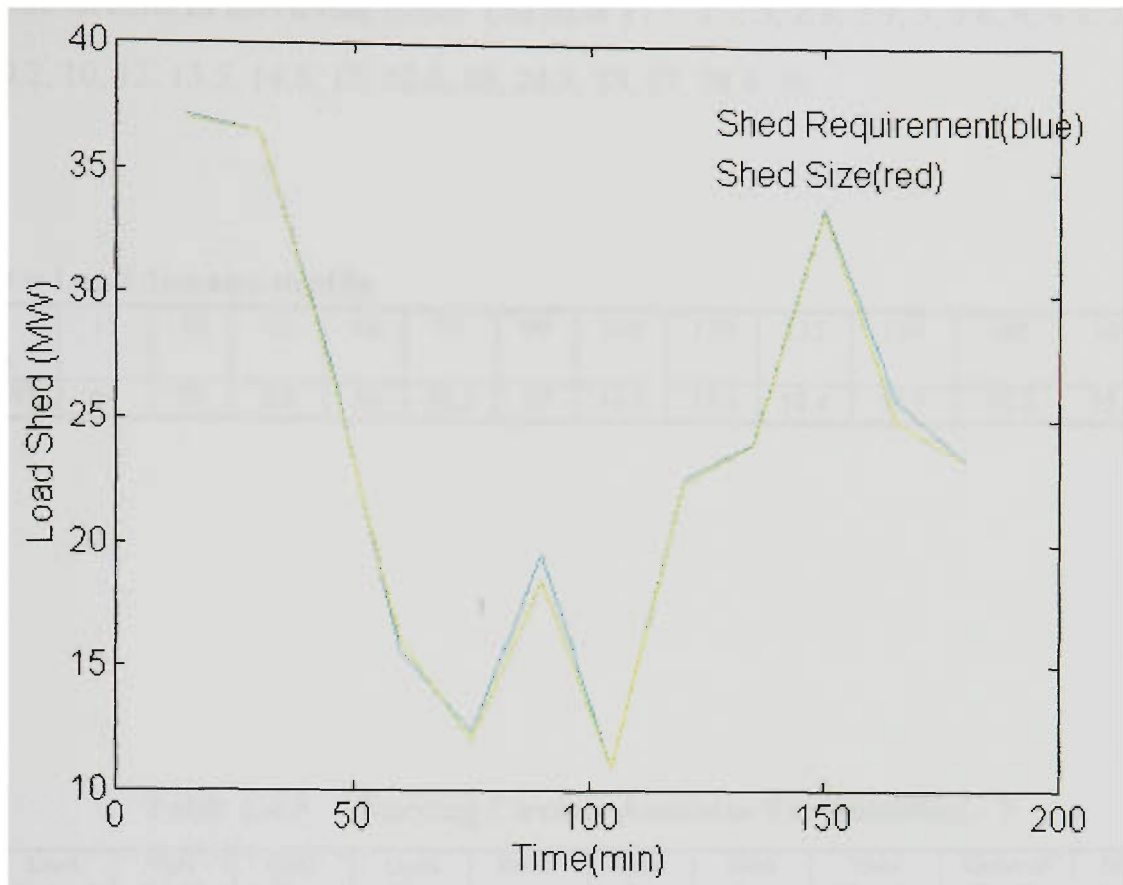
Figure 6.17 Comparison of Shed Requirement vs Shed Size with 32 circuits available for shedding
