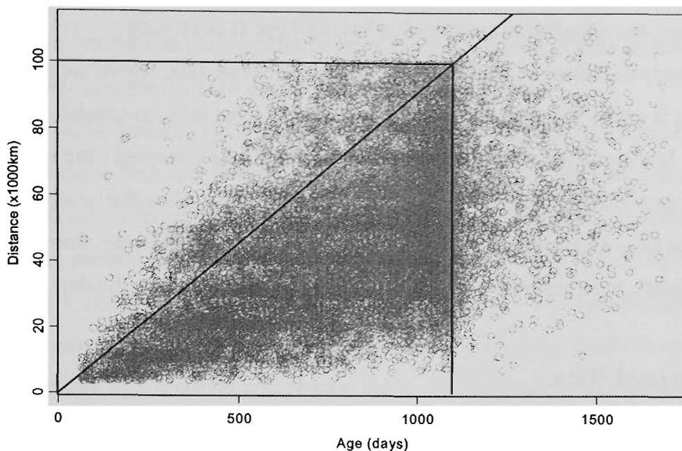
Fig. 5.1. *Vehicle usage rates, showing warranty limits and max usage rate for the full 3-year warranty (diagonal line).*
