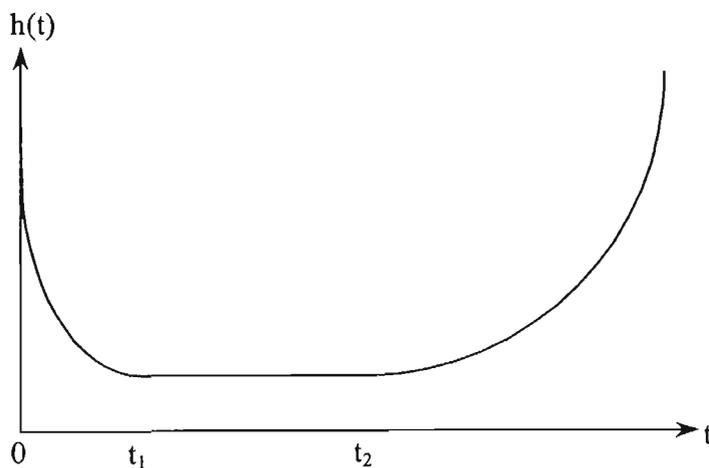
Fig. 5.2. Bath tub hazard rate. (Adapted from Fig. 1, Murthy and Blischke, 1992b.)
