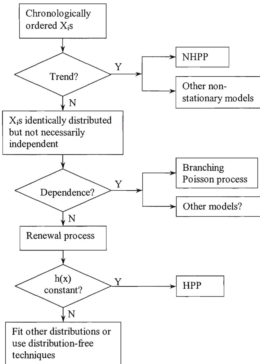
Fig. 3.1. *Statistical analysis of successive inter-arrival times of a repairable system.*
