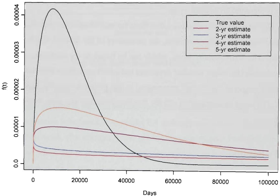
Fig. 7.11. Probability density function for the estimated  $\beta$  and  $\eta$  values.
