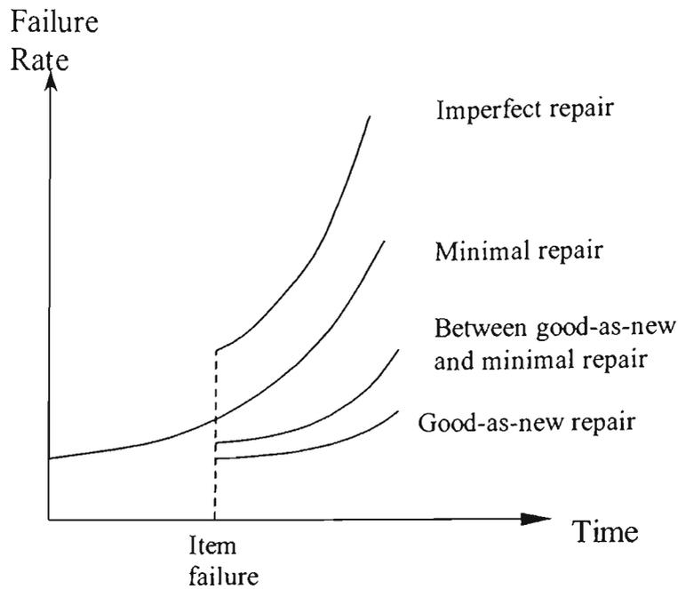
Fig. 3.3. Failure rates after various repairs.
