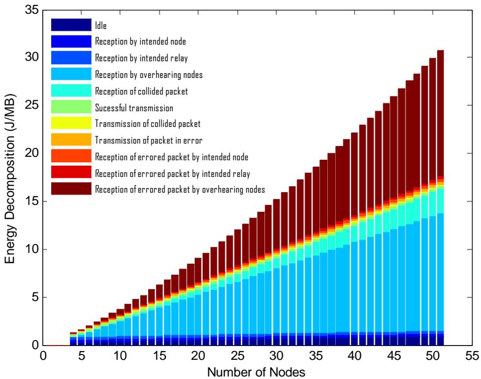
Figure 3.13: Decomposition of energy (J/MB) for rDCF(11, 5.5) in a channel with errors.
