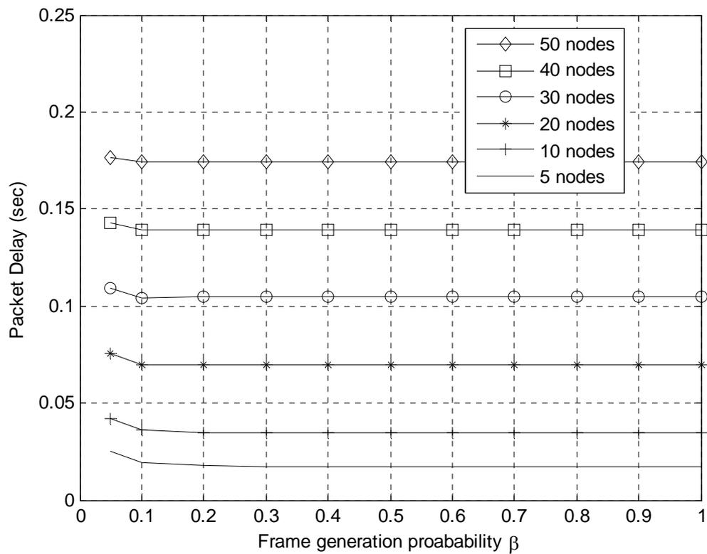
Figure 4.22: Non-saturated Packet Delay of ErDCF(11, 5.5) in an ideal channel.
