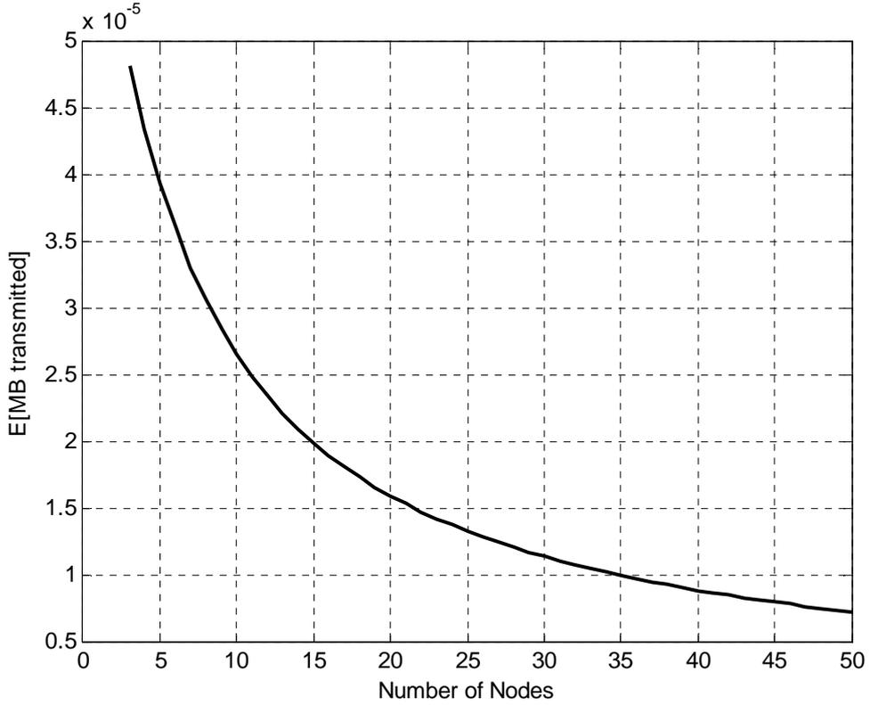
Figure 3.7: Average payload (MB) transmitted and received in one slot.
