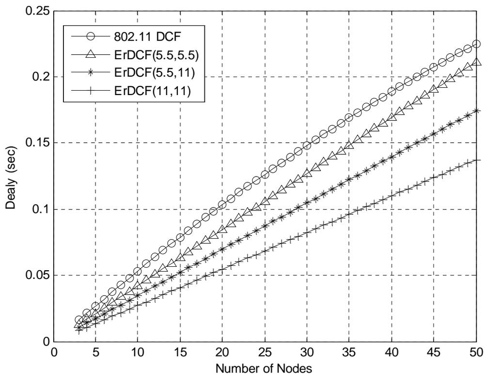
Figure 4.11: Delay of 802.11 DCF and ErDCF ( $R_1, R_2$ ) in an ideal channel.
