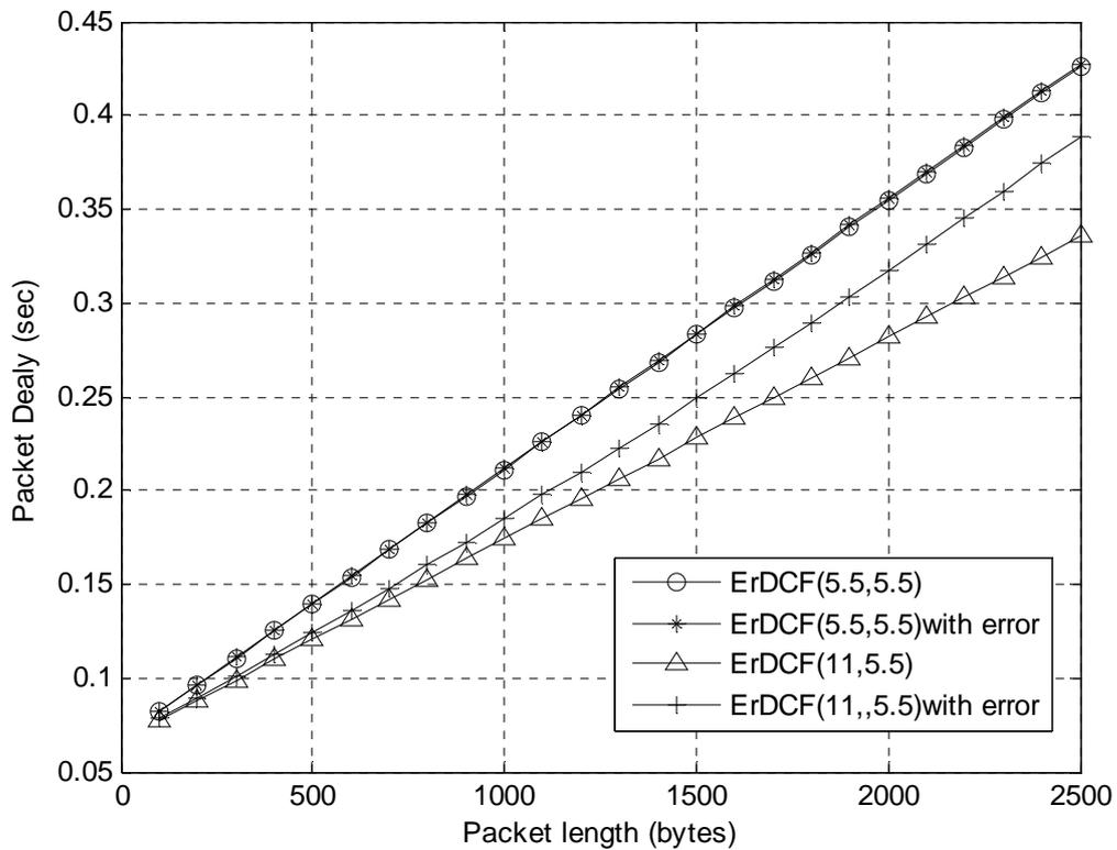
Figure 4.15: Impact of packet length on ErDCF ( $R_1, R_2$ ) in an ideal channel and with transmission errors.
