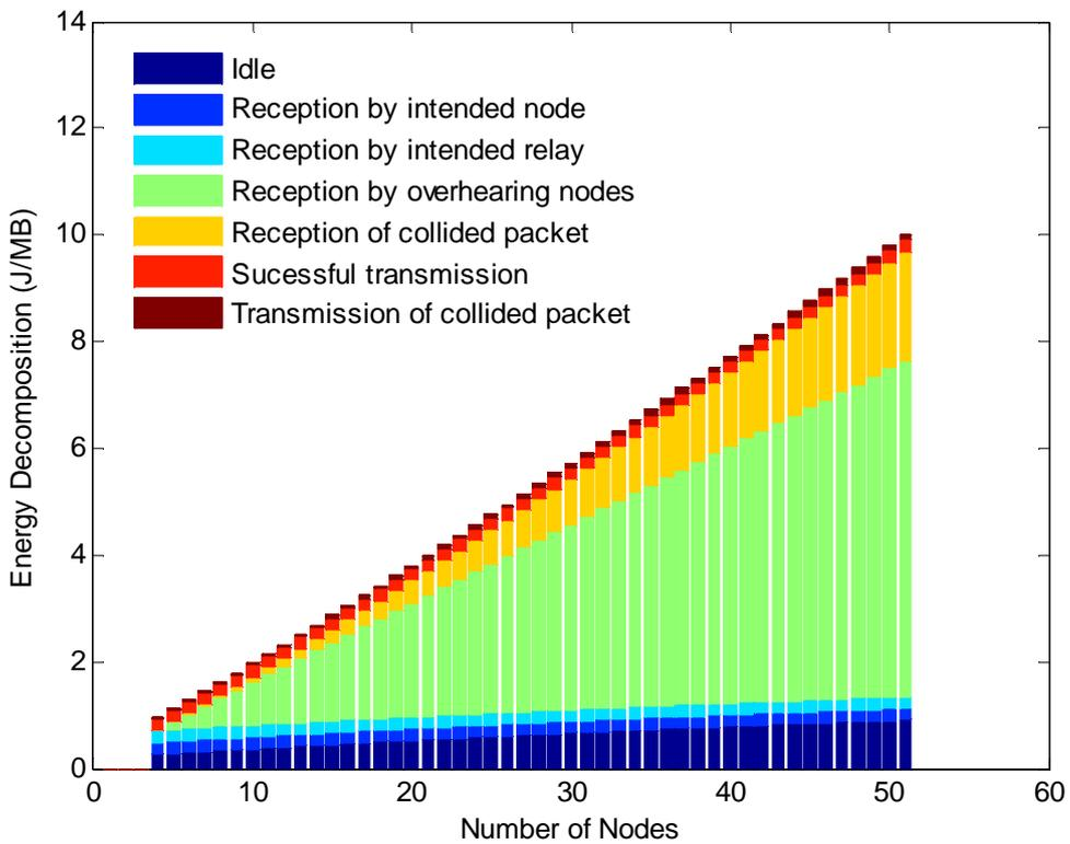
Figure 4.19: Decomposition of energy consumed (with energy savings).
