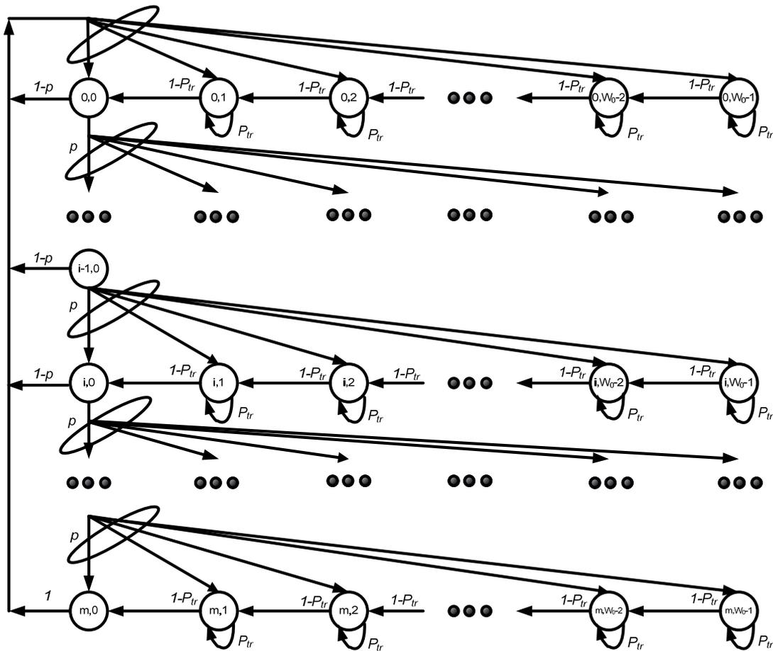
Figure 3.2: Discrete time Markov chain model.
