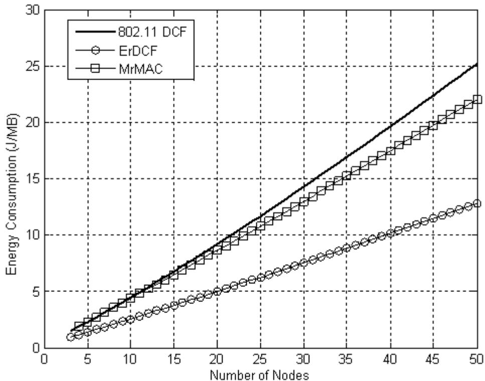
Figure 5.9: Energy consumption of MrMAC, ErDCF802.11 DCF and 802.11 DCF.
