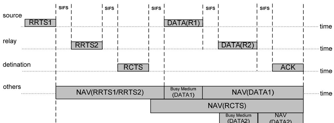
Figure 4.1: ErDCF Carrier Sensing Scheme.
