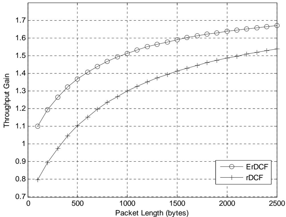
Figure 4.4: Throughput Gain over 802.11 DCF.
