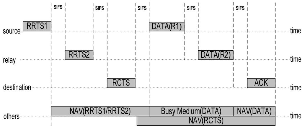
Figure 3.4: Carrier sensing scheme of rDCF.
