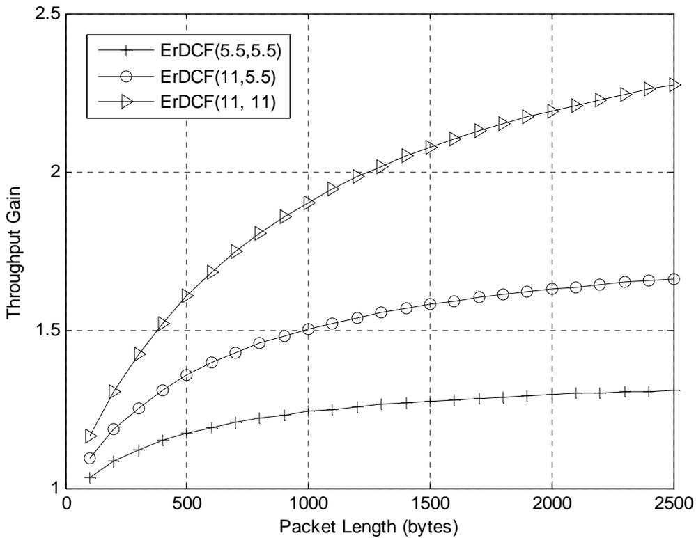
Figure 4.7: Throughput Gain over 802.11 DCF.
