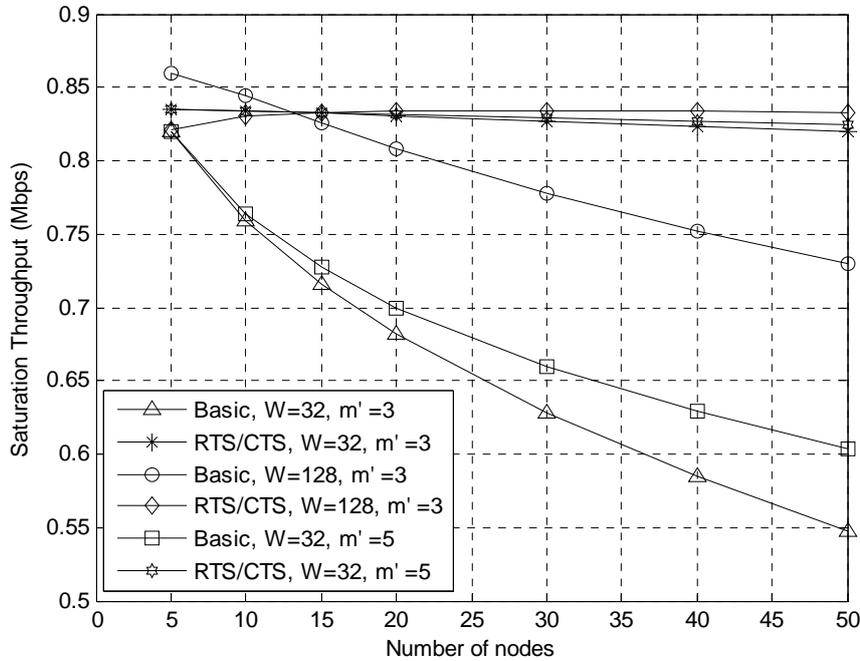
Figure 2.6: Saturation Throughput Analysis.
