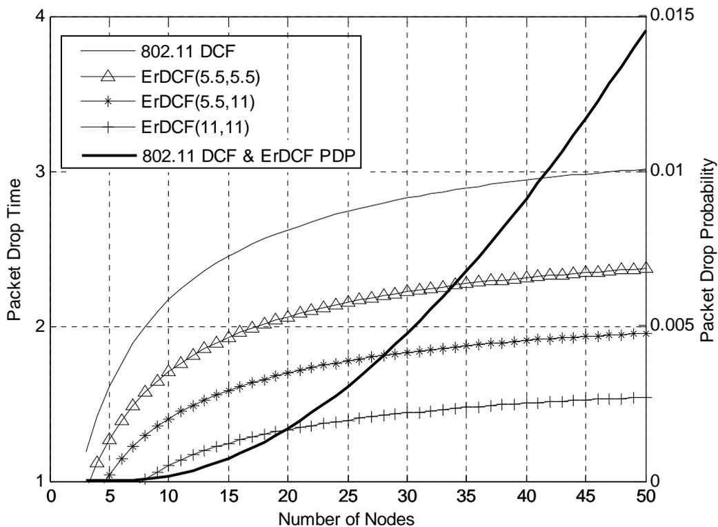
Figure 4.12: Packet Drop Time (PDT) and Packet Drop Probability (PDP) of 802.11 DCF and ErDCF ( $R_1, R_2$ ) in an ideal channel.
