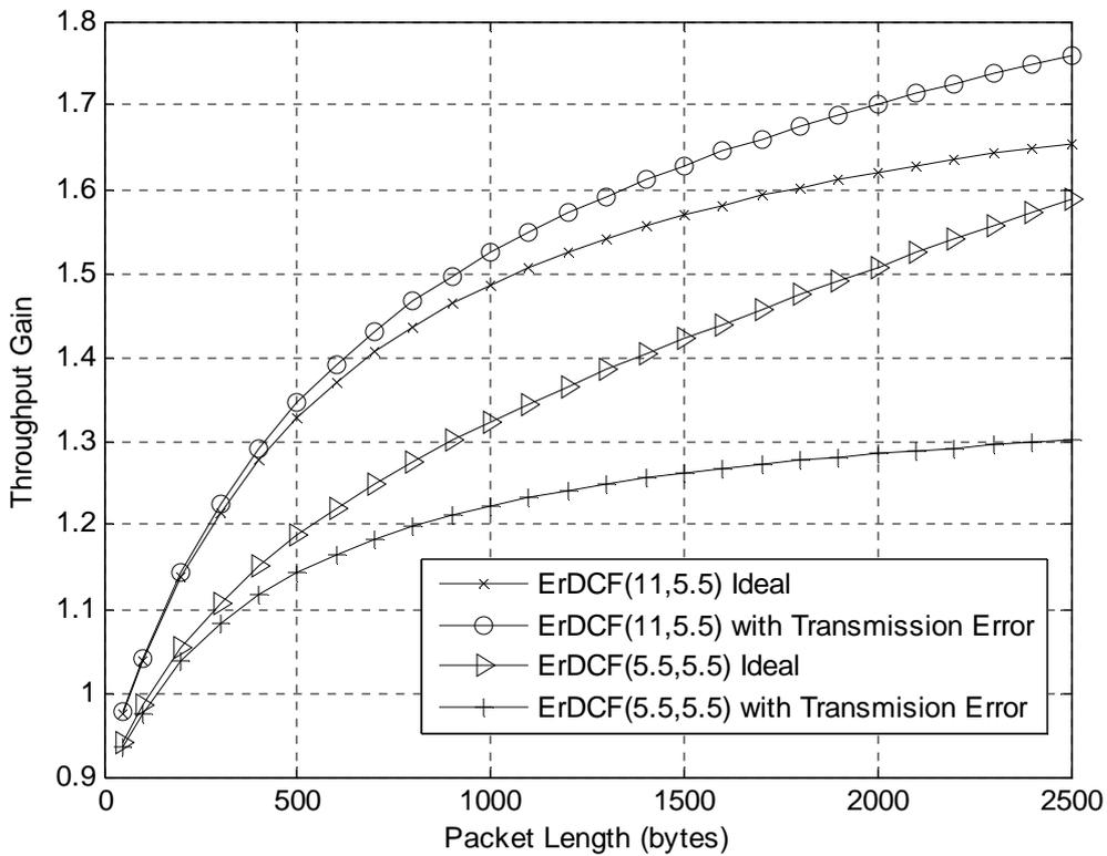
Figure 4.10: Throughput gain of ErDCF (11, 5.5) and (5.5, 5.5) in an ideal channel and with transmission errors.
