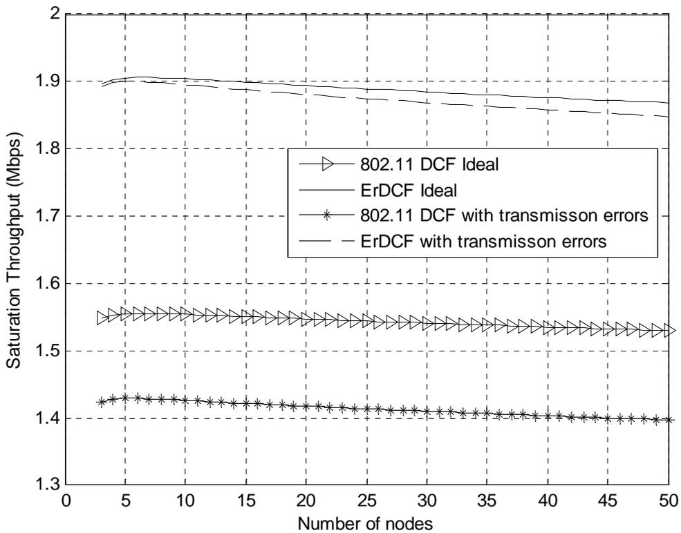
Figure 4.8: Performance of ErDCF (5.5, 5.5) and 802.11 DCF in ideal channel and with transmission errors.
