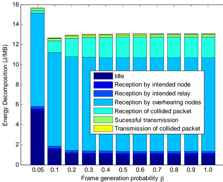
Figure 4.23: Non-saturated energy consumption of ErDCF(11, 5.5) in an ideal channel.
