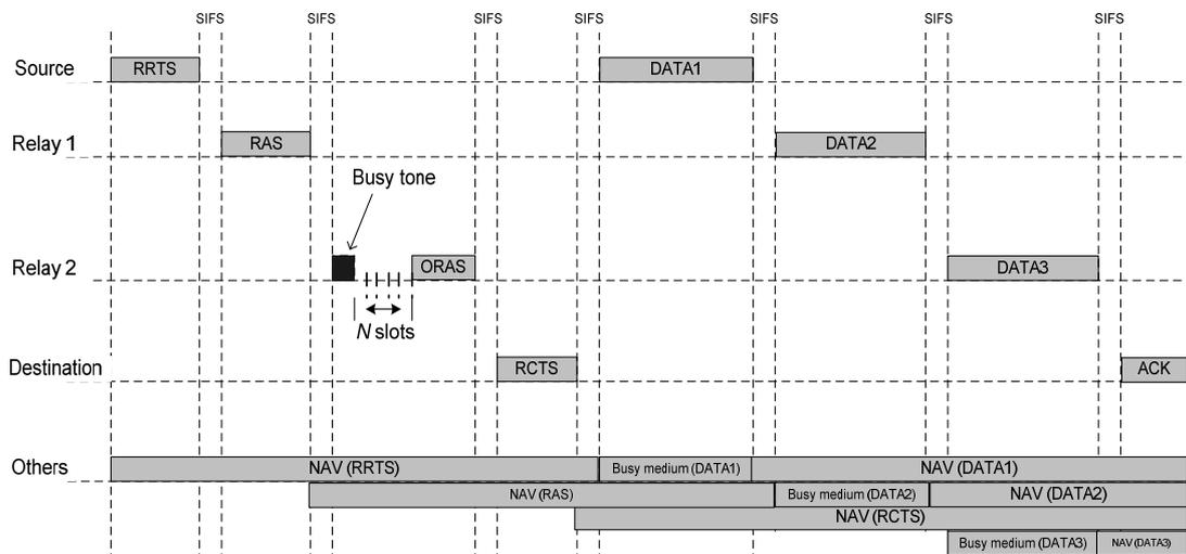
Figure 5.4: MrMAC carrier sensing scheme.
