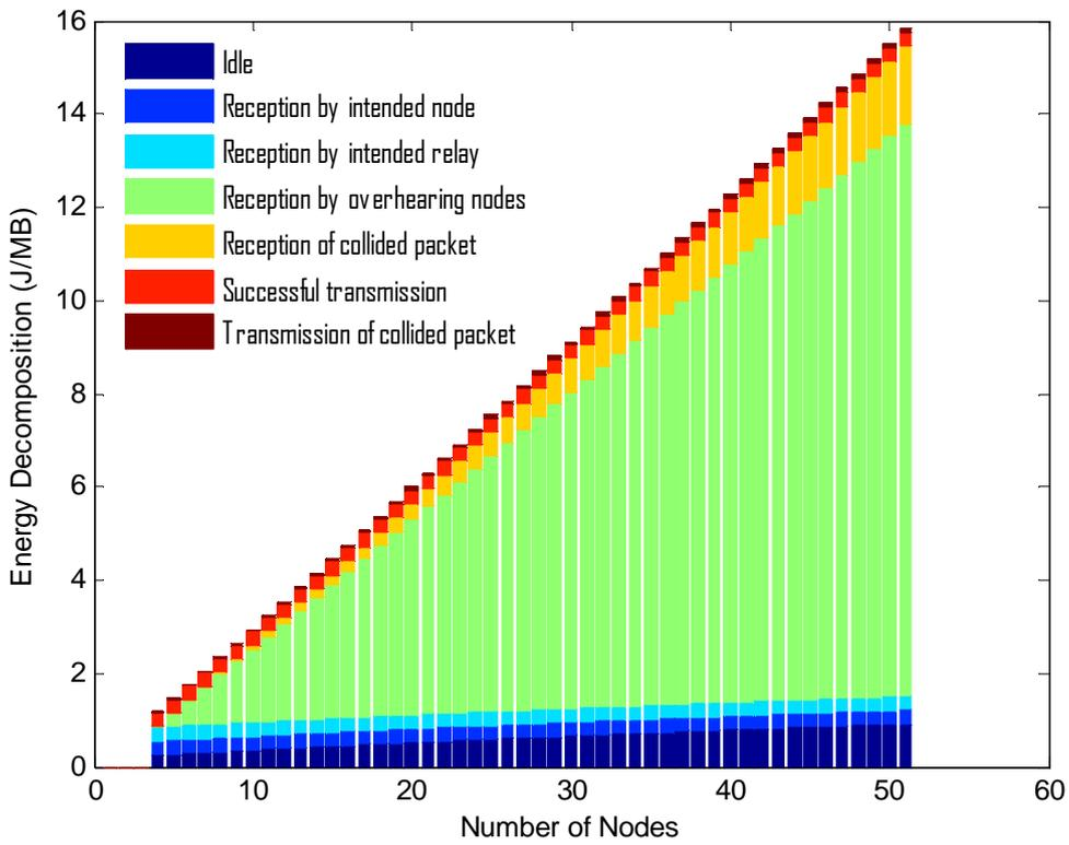
Figure 3.12: Decomposition of energy (J/MB) for rDCF(11, 11) in an ideal channel.
