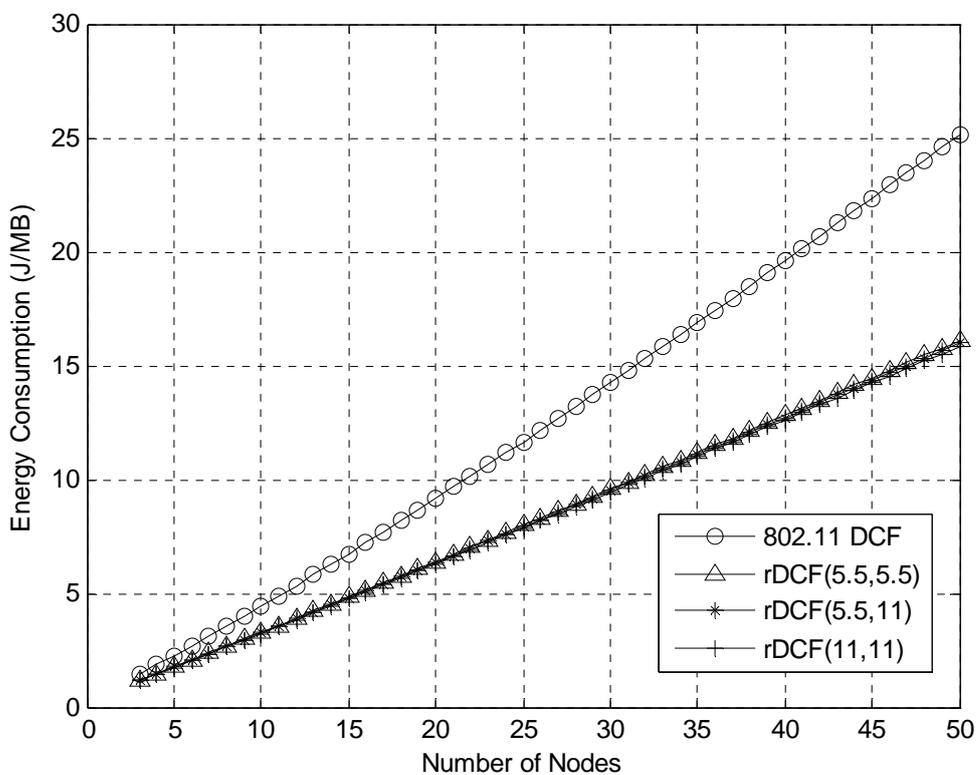
Figure 3.8: Energy consumed (J/MB) for 802.11DCF and rDCF in an ideal channel.
