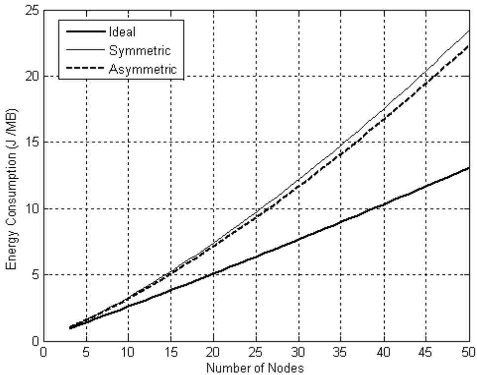
Figure 4.17: Energy consumed (J/MB) for ErDCF in channel errors.
