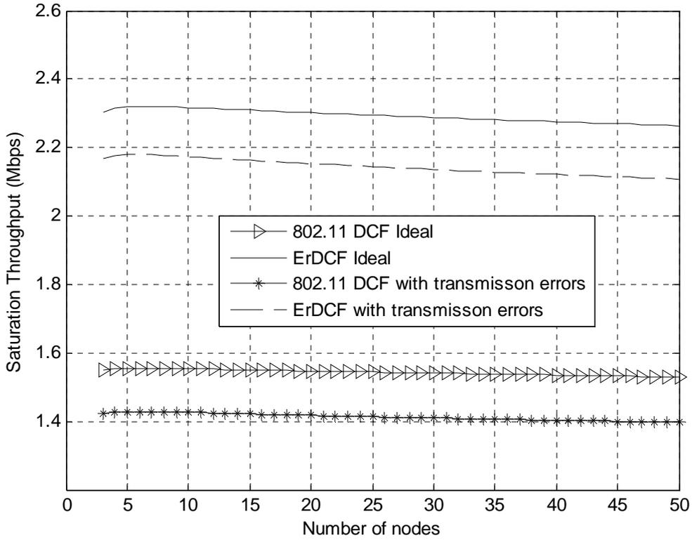
Figure 4.9: Performance of ErDCF (11, 5.5) and 802.11 DCF in ideal channel and with transmission errors.
