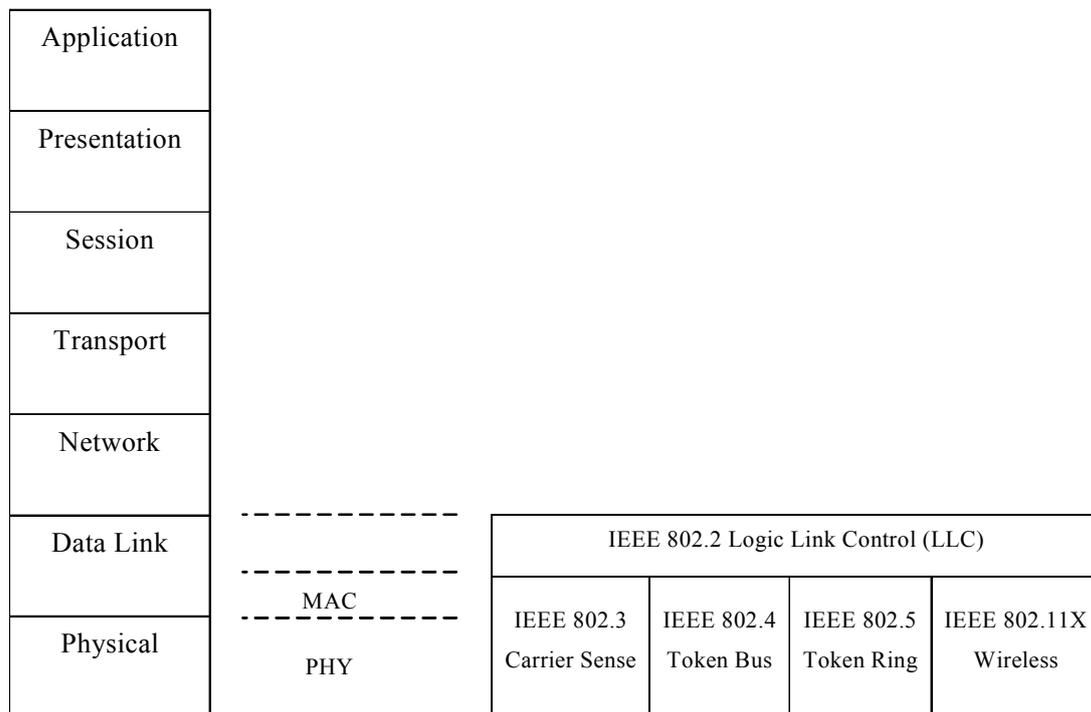
Figure 2.2: Relationship of IEEE 802.xx standards to OSI layers.
