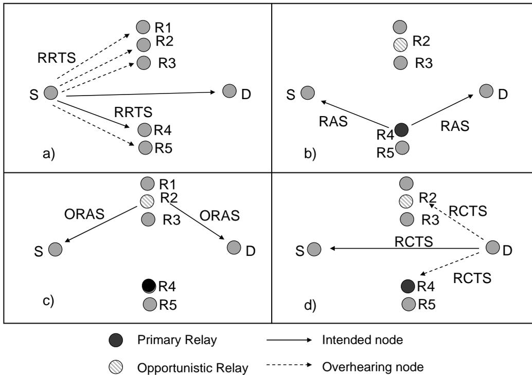
Figure 5.3: An illustration of the handshake in MRMAC.
