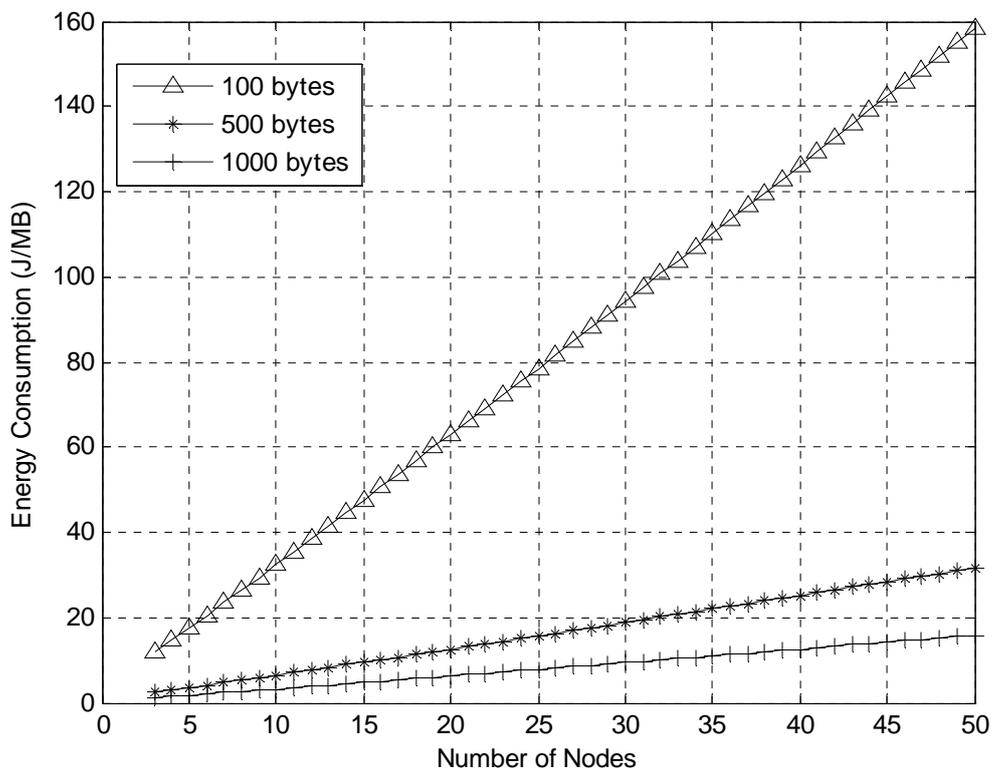
Figure 3.9: Energy consumed (J/MB) for rDCF (11, 11) in an ideal channel at different packet sizes.
