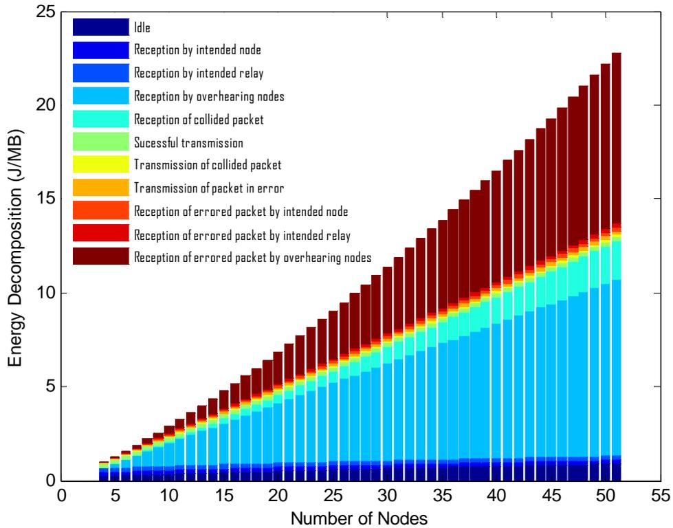
Figure 4.20: Decomposition of energy consumed with transmission errors.
