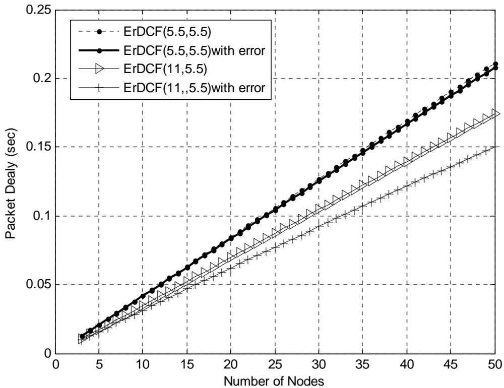
Figure 4.13: Comparing Delay of ErDCF ( $R_1, R_2$ ) in an ideal channel and with transmission errors.
