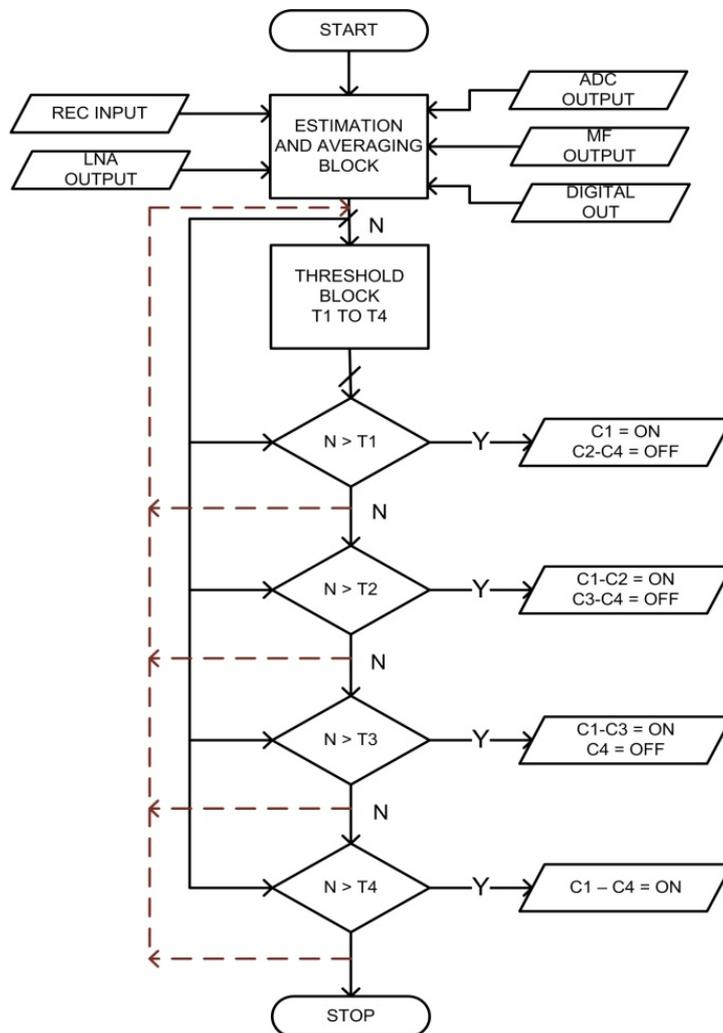
**Figure 6.18: Flow diagram of the different operating modes of the controller**
