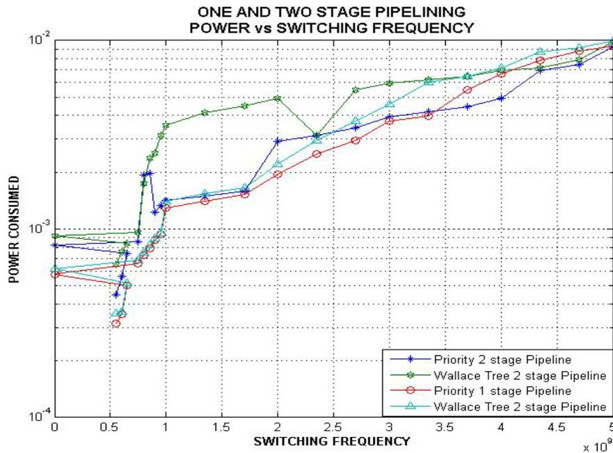
**Figure 5.20: Power performance versus switching speed for one and two stage pipelining**
