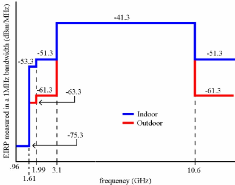
Figure 2.1: Spectral mask frequency occupancy of the UWB spectrum as defined by the FCC [4]
