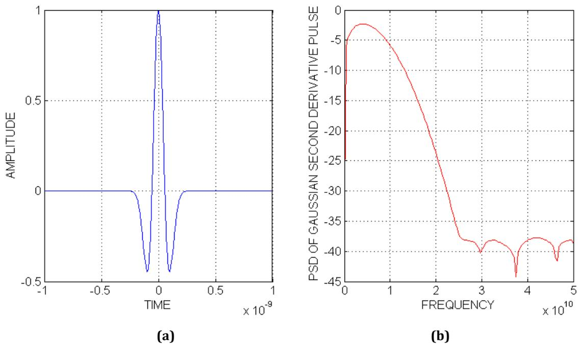
**Figure 2.8: Gaussian second derivative pulse and its corresponding frequency spectrum used for UWB communication**
