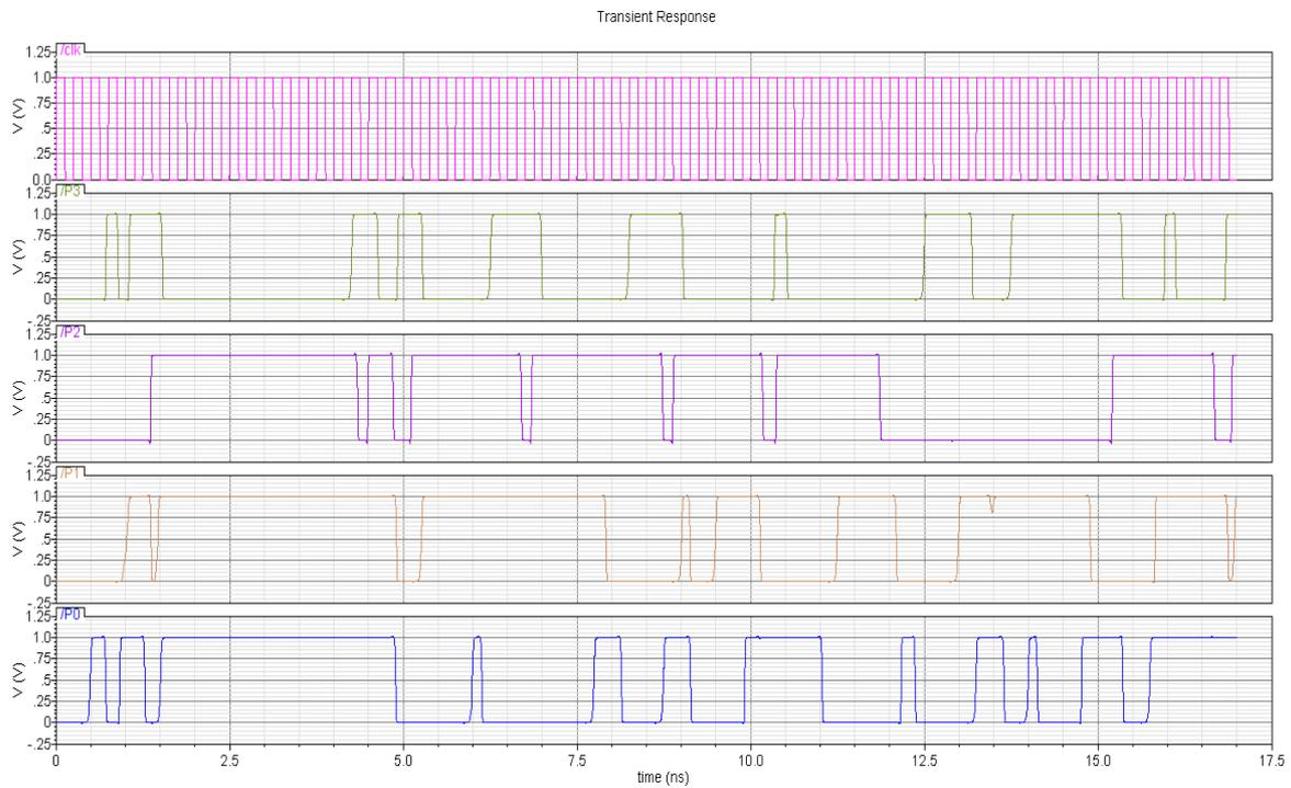
**Figure 7.7 (a): Positive node output of the 4 bit flash converter designed in this work**
