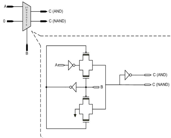
**Figure 5.15: Multiplexer based gate used in the encoder design**
