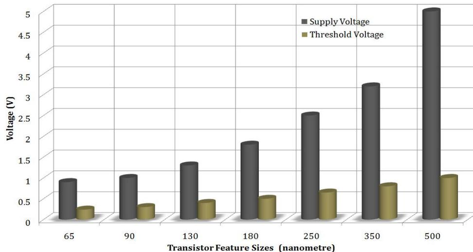
**Figure 4.4: Comparison of typical transistor supply and threshold voltages against the different technology nodes for features sizes ranging from 65nm to 500nm**
