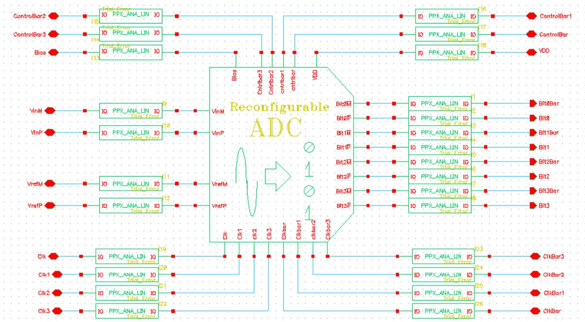
Figure 6.15: Pad level schematic of the fully differential novel reconfigurable ADC
