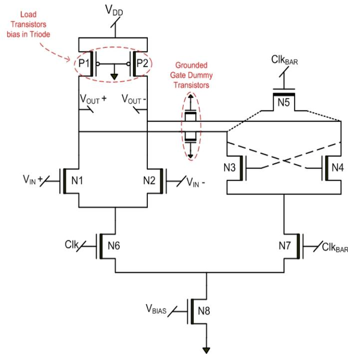
**Figure 4.11: Track and Latch circuit with the clock used as mode select and dummy transistors for glitch suppression**
