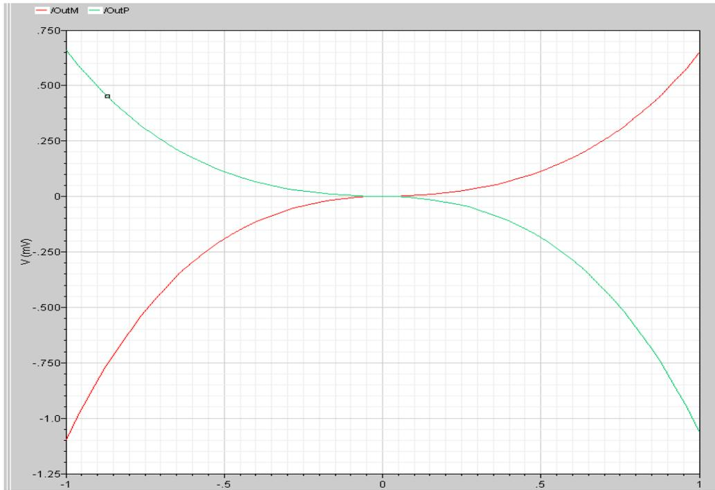
Figure 4.10: Pre-amplifier dc response of the preamplifier with minimal offset deviation from zero.
