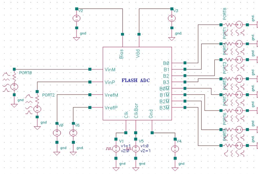
Figure 7.1: Testbench for the Flash ADC
