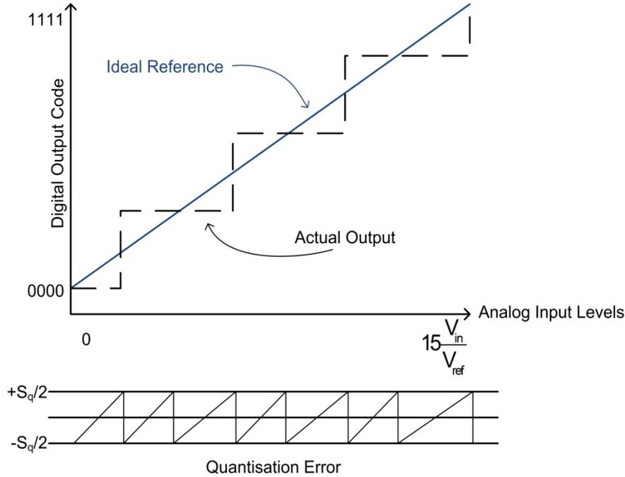
**Figure 5.1: Relation between the ADC input, output and the subsequent quantisation error for a ramp based analog input**
