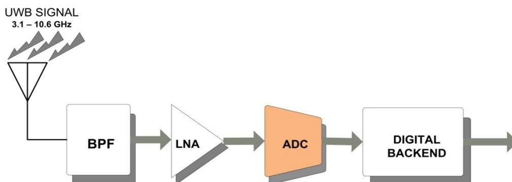
Figure 1.1: Block level diagram of UWB Receiver chain with ADC highlighted
