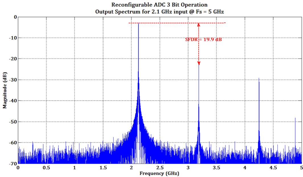
**Figure 7.10 (b): Output for the reconfigurable converter for 3 bit operation**
