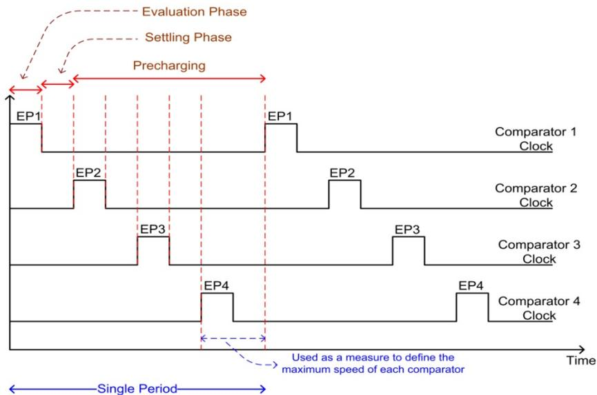
Figure 6.13: Clocking mechanism used in the reconfigurable design
