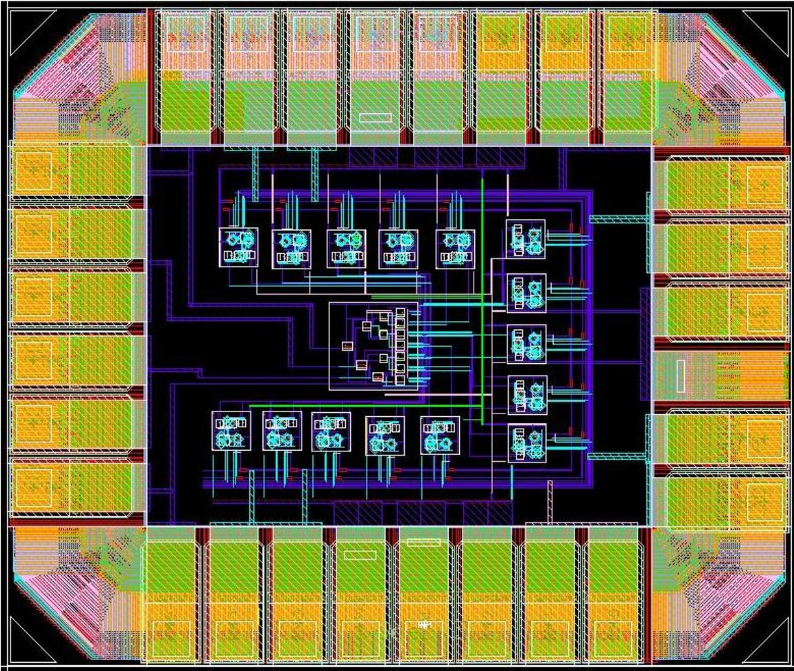
**Figure 5.25: Complete chip level layout implementation of the high speed Flash analog to digital converter**
