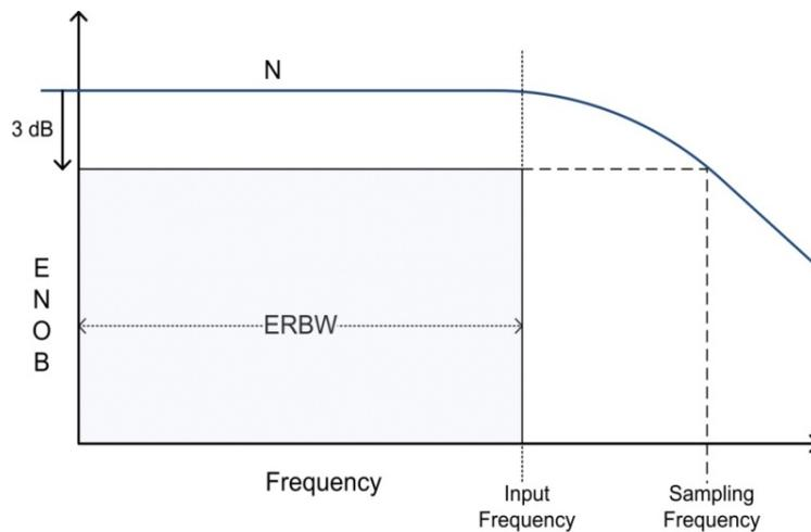
**Figure 5.5: Relation between the ENOB, ERBW and the sampling and input frequencies**
