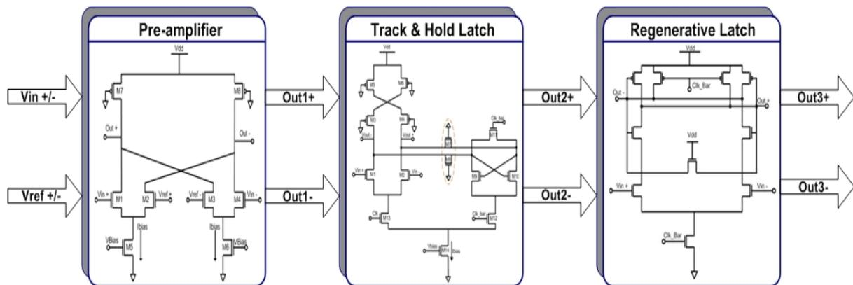
Figure 4.6: Block level schematic of the dynamic comparator implemented in this work
