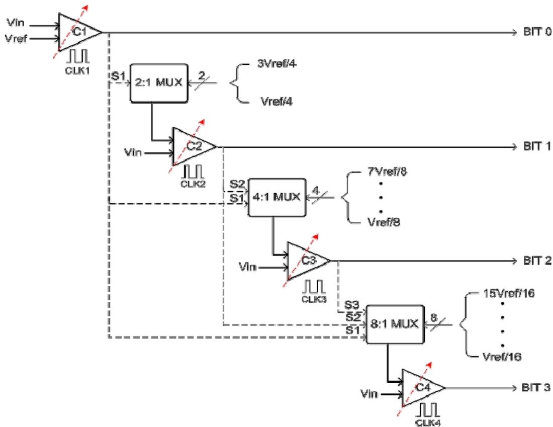
Figure 6.2: Basic representation of the reconfigurable architecture [100]
