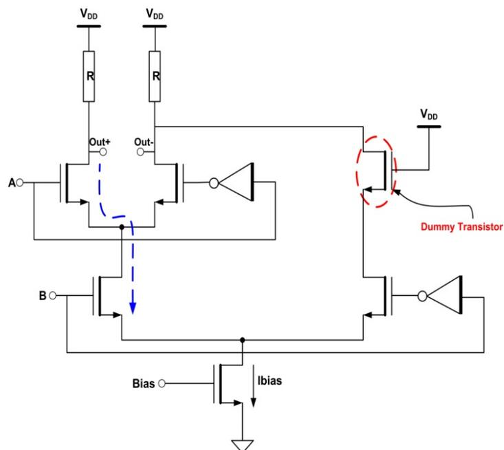
Figure 5.14: CML gate implementation for NAND/AND functionality
