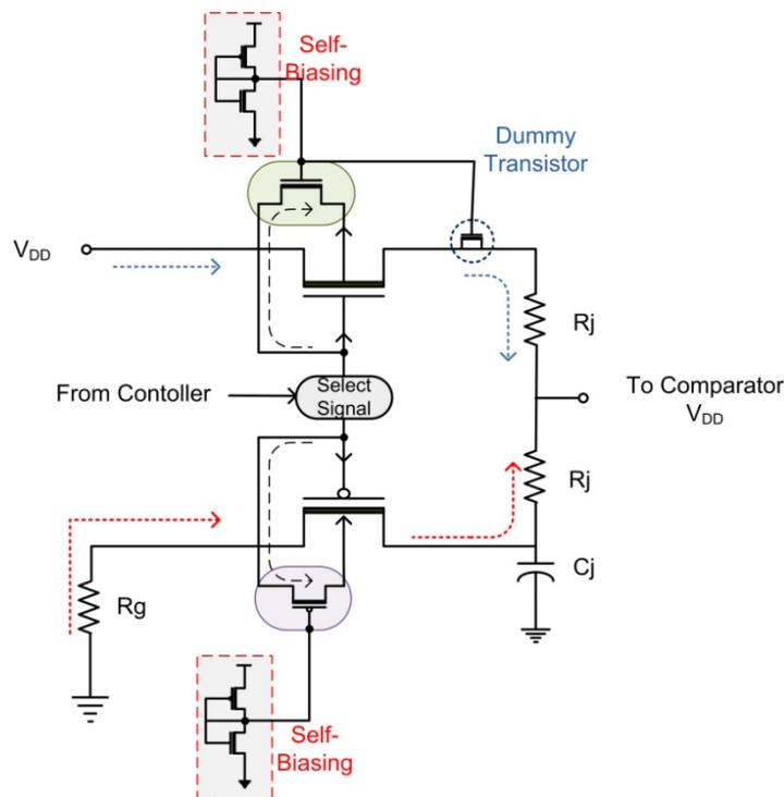
**Figure 6.11 (a): Enable circuit for reconfigurability**
