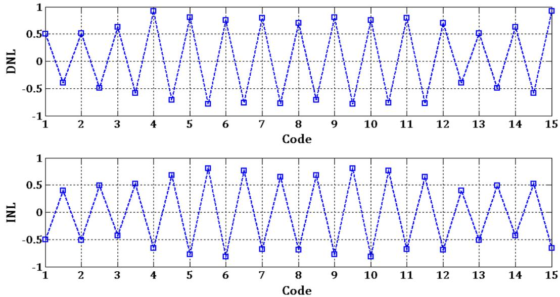
Figure 7.7 (b): Linearity Performance for Custom Flash Converter
