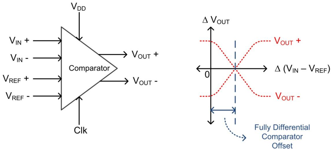
**Figure 4.2: Response of the fully differential comparator output with the deviation from origin corresponding to the offset**
