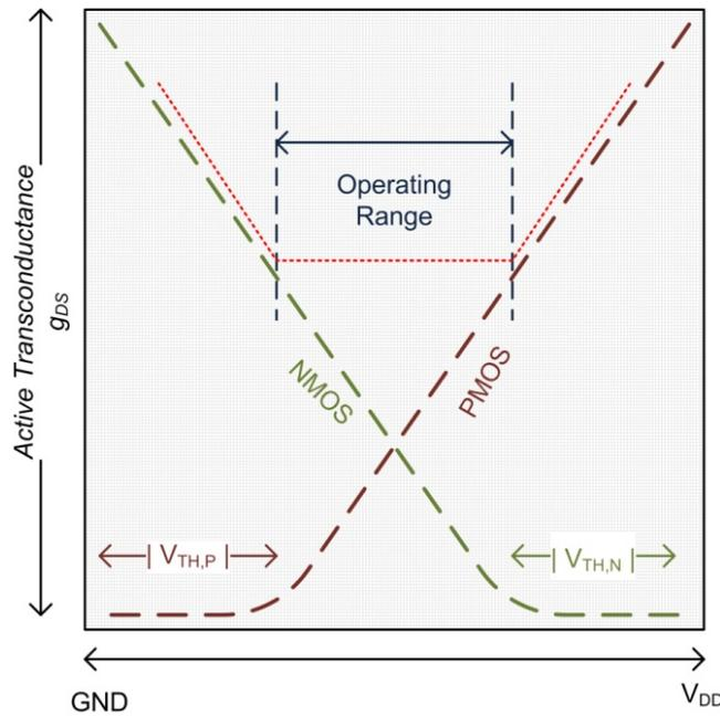
**Figure 6.5: Active operating range for the CMOS switch**
