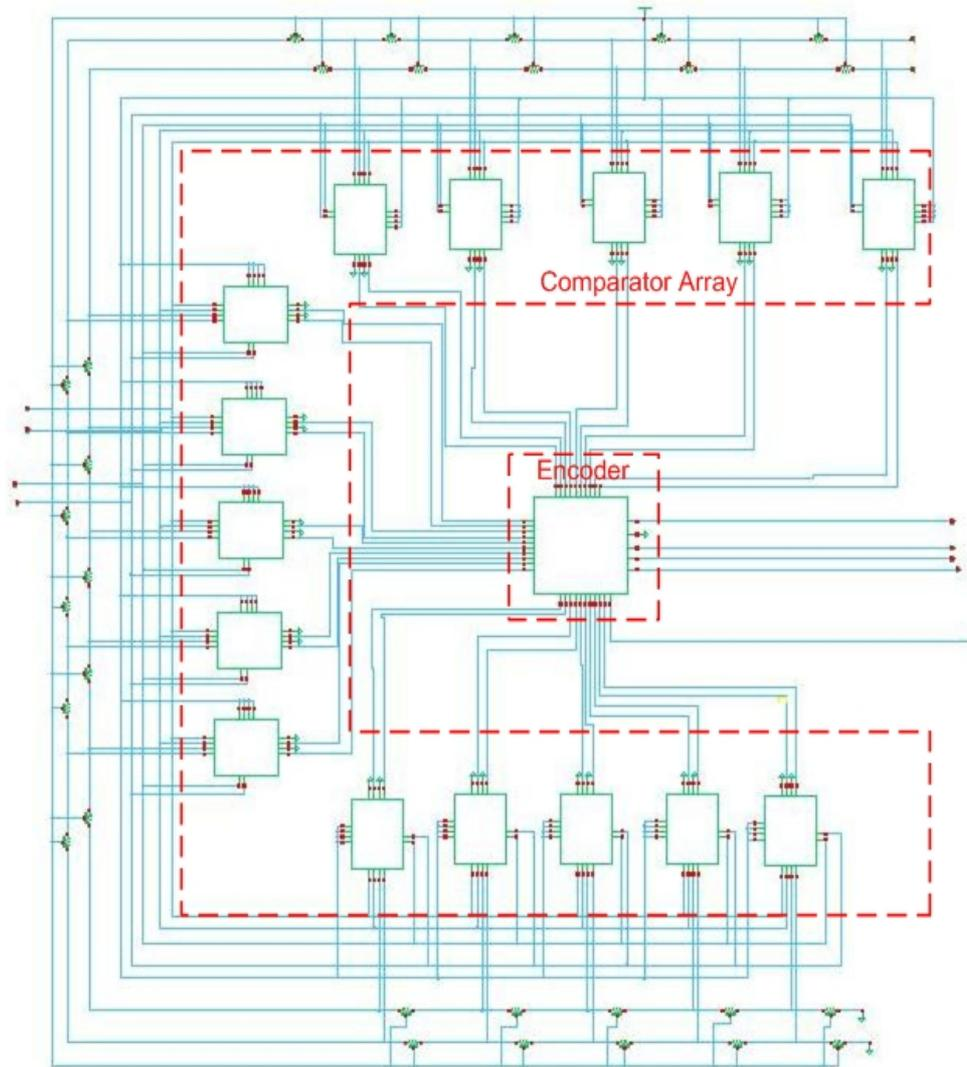
**Figure 5.23: Circuit schematic of the complete Flash Analog to Digital Converter**
