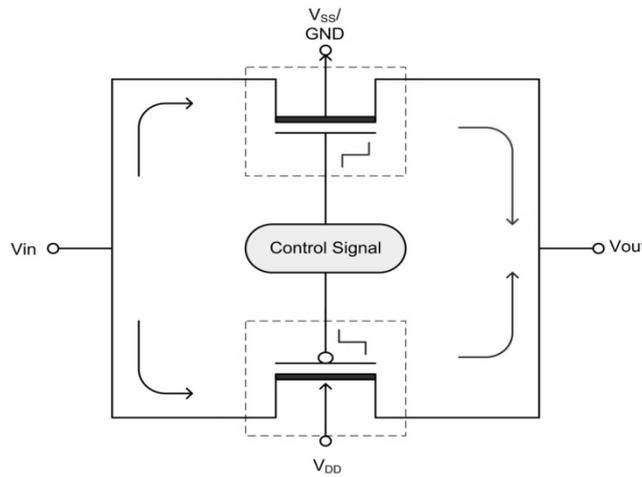
**Figure 6.4: Simple CMOS switch in PTC setting**
