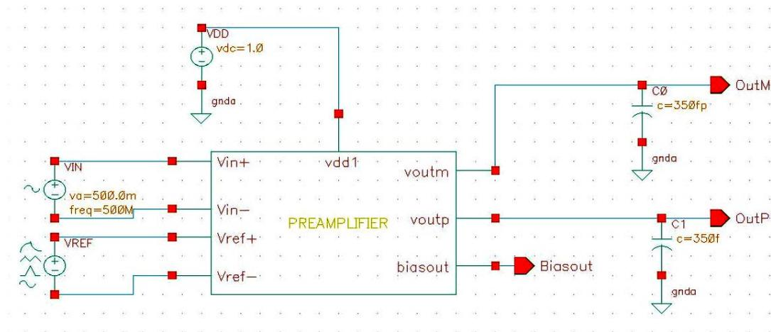
Figure 4.8: Test setup for the fully differential preamplifier with an input frequency of 500 MHz
