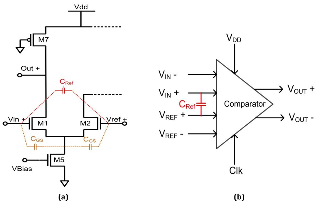
**Figure 5.7: Input feed through capacitances for the comparator (b) using Pre-amplifier half-circuit configuration (a)**
