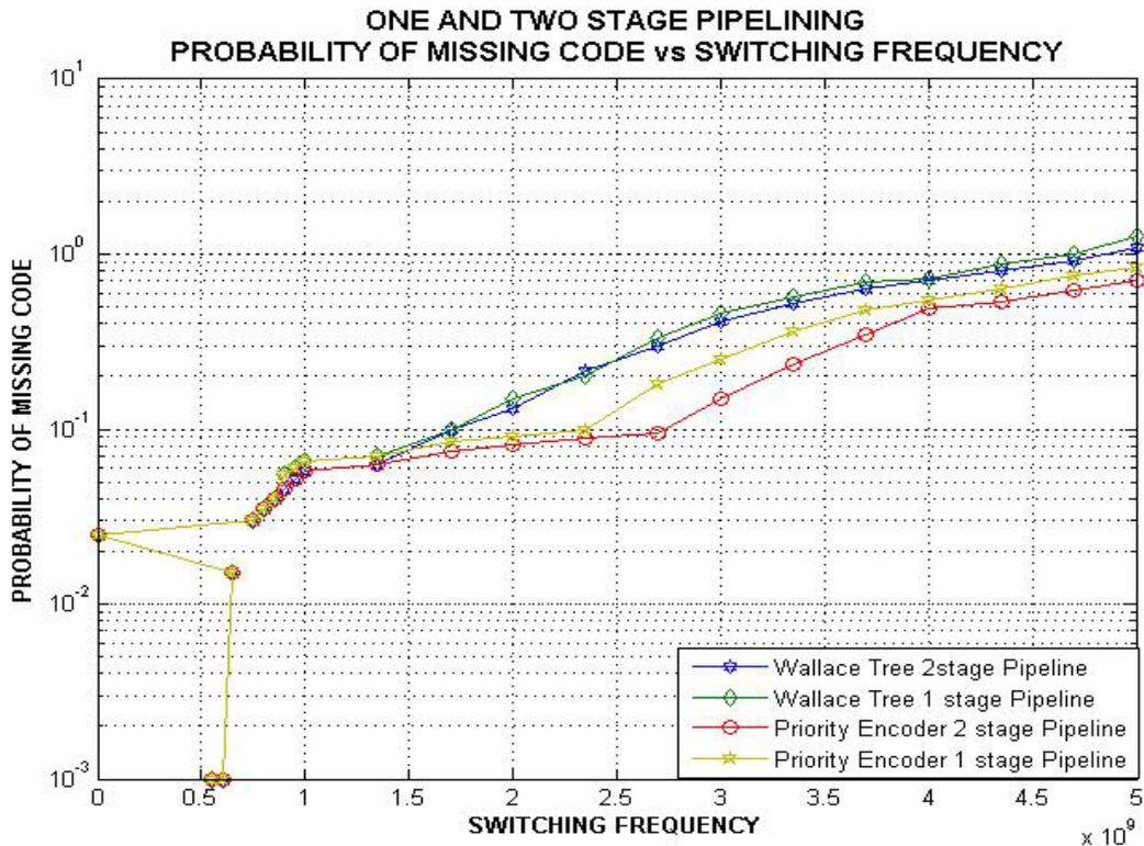
**Figure 5.21: Probability of Error versus the Switching frequency for one and two stage pipelining**
