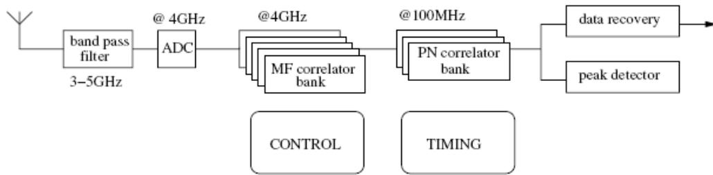
**Figure 2.13: Direct Sequence-Ultra Wideband receiver with a single high speed Analog to Digital Converter and a high speed digital backend [37]**
