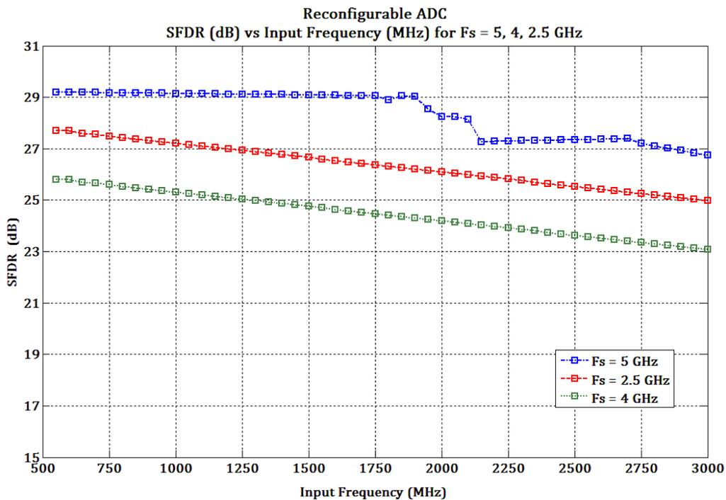
**Figure 7.11: SFDR variation versus input frequency sampled at 5, 4 and 2.5 GHz**
