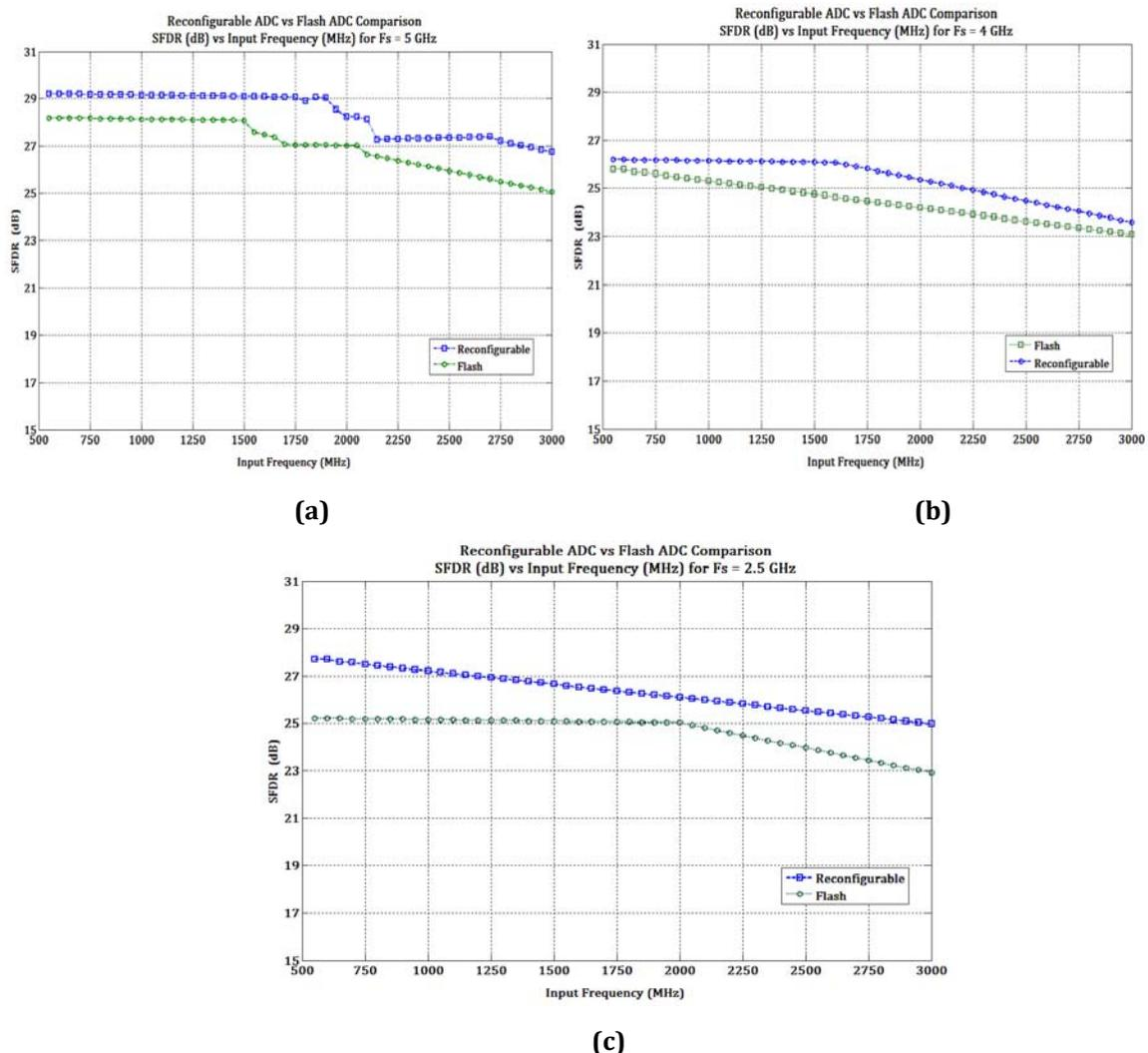
Figure 7.15 (a) to (c): Comparison of SFDR versus input frequency for Flash and Reconfigurable Converters at 2.5, 4 and 5 GHz sampling frequencies
