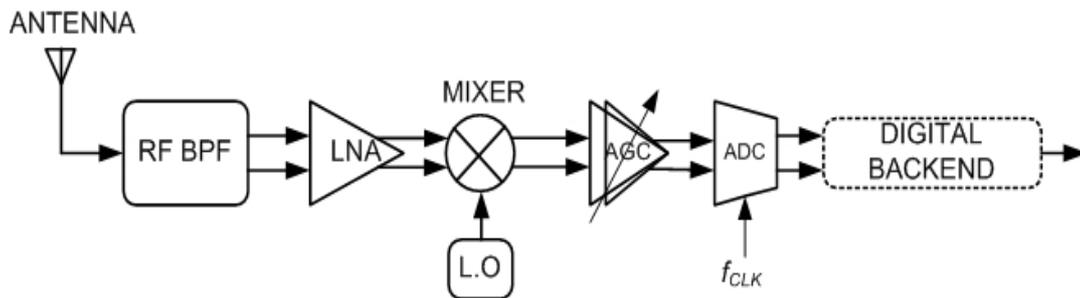
Figure 3.7: Typical Ultra Wideband receiver architecture used for high speed communications
