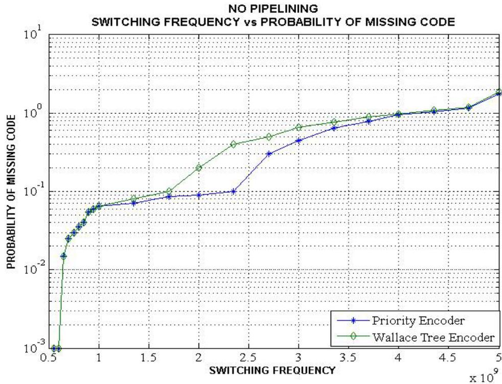
**Figure 5.19: Probability of Error versus Switching Frequency without pipelining**
