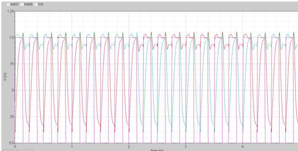
**Figure 4.14: Output of the regenerative latch offering a higher swing almost from rail to rail with a 3.5 GHz clock**
