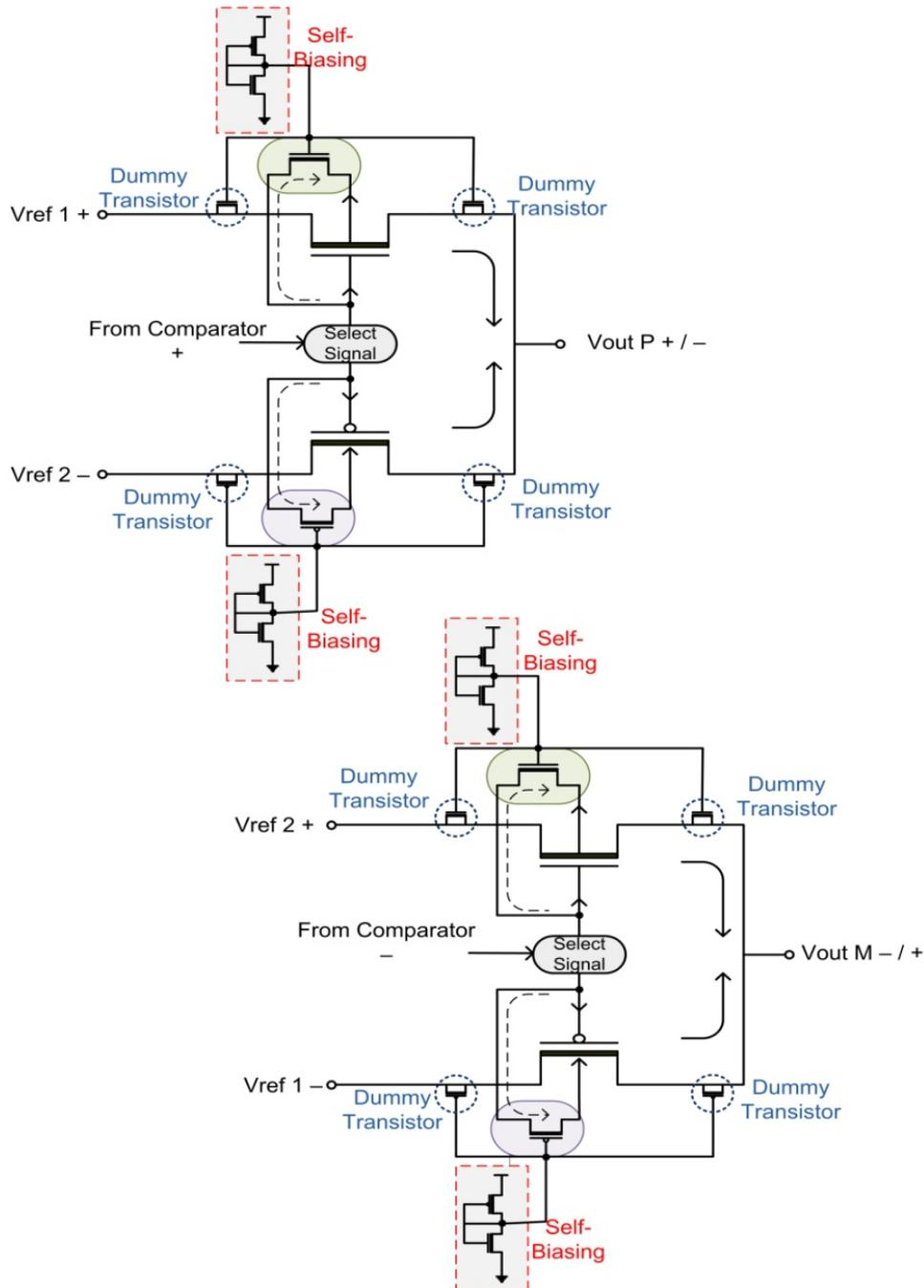
**Figure 6.10: Fully differential dynamic self-biased 2:1 analog multiplexer implemented for the reconfigurable converter**
