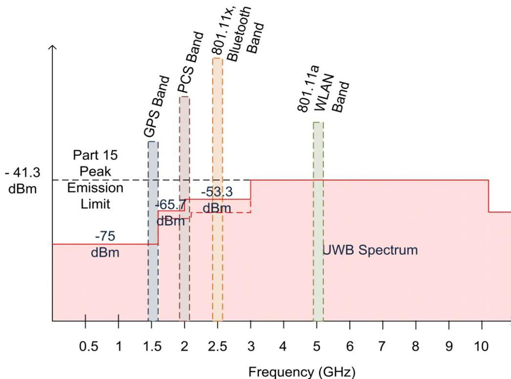
**Figure 2.9: Co-existence of Ultra Wideband with other narrowband communication schemes such as GPS, Bluetooth and WLAN**
