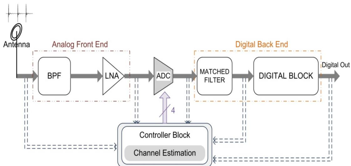
**Figure 6.17: Representation of the controller concept within the receiver chain for reconfigurability**
