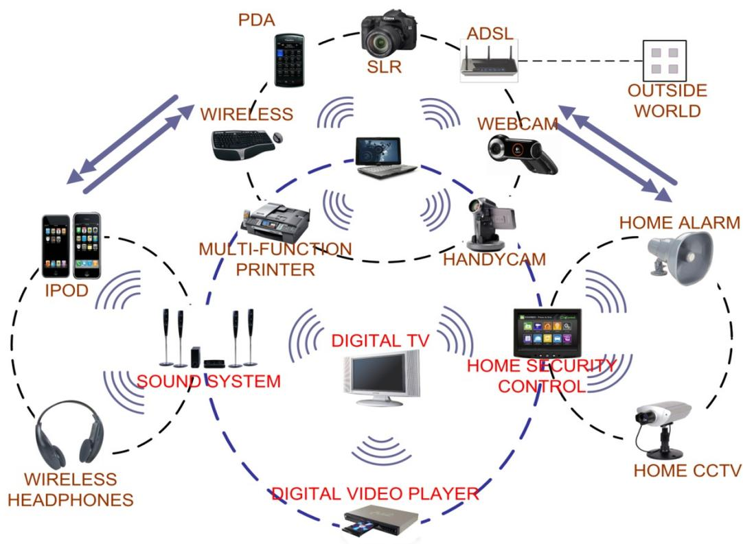
**Figure 2.2: Seamless connectivity offered by UWB medium for HOSO environment**
