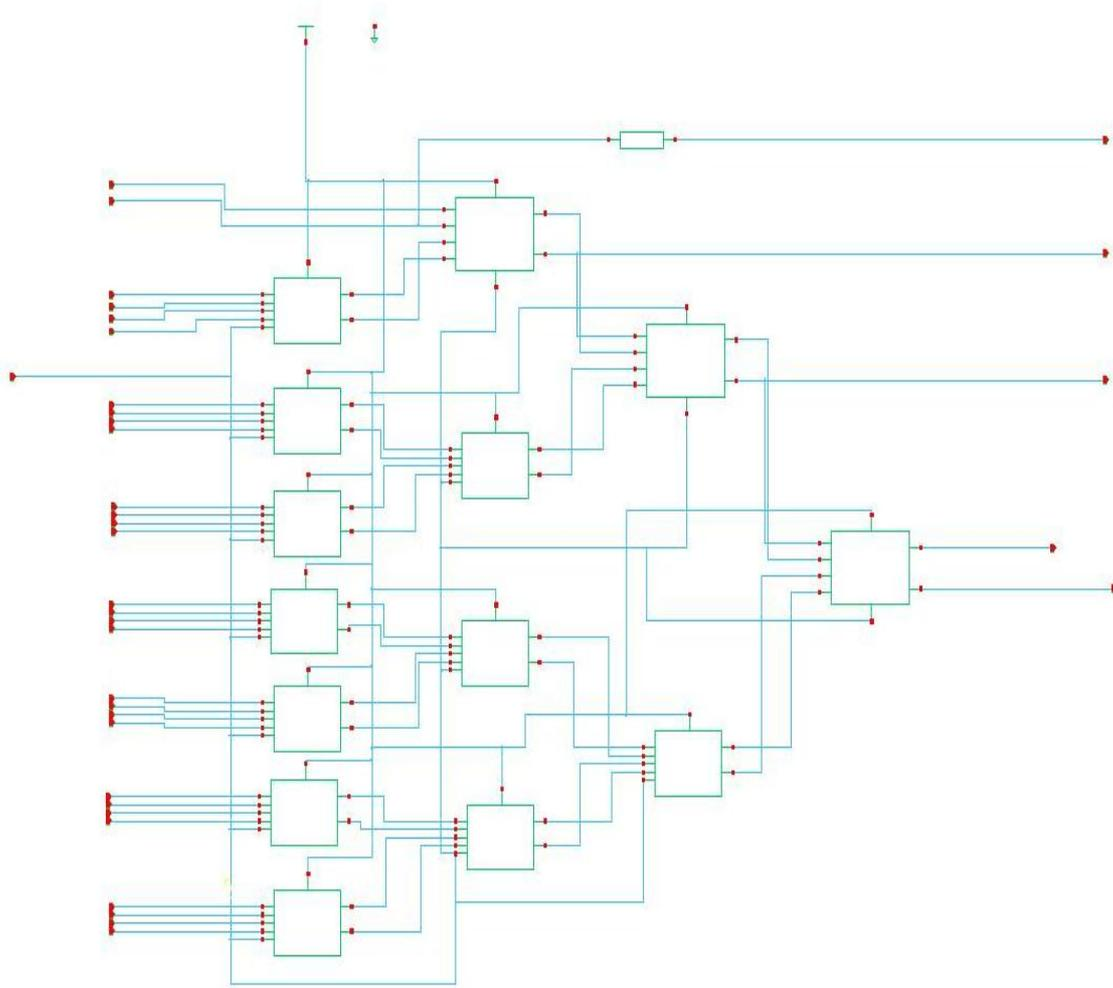
**Figure 5.22: Gate level circuit of the implemented encoder for the high speed FLASH ADC**
