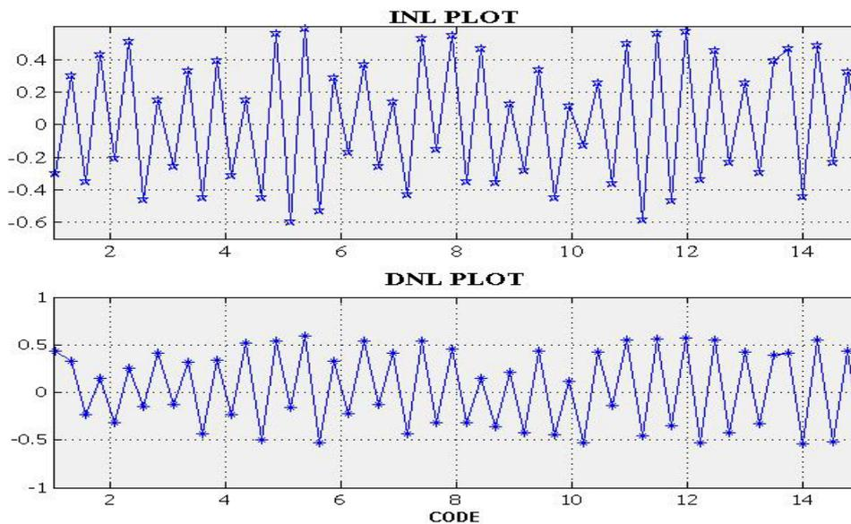
**Figure 7.14: Maximum INL and DNL for the reconfigurable converter during 4 bit operation**
