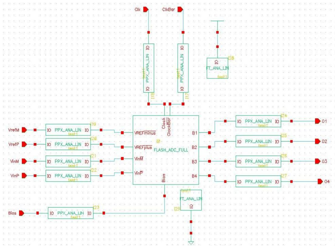
**Figure 5.24: Schematic of the Flash ADC with pad configuration at the various I/O's**
