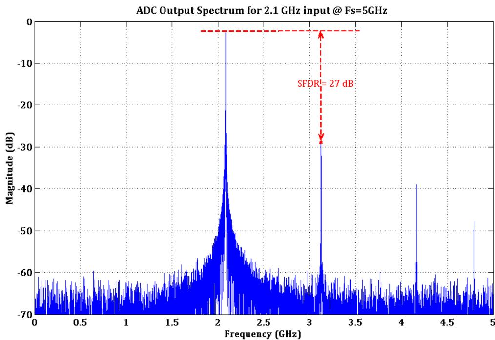
**Figure 7.3: Flash ADC Output FFT Spectrum for 2.1 GHz input sampled at 5 GHz**
