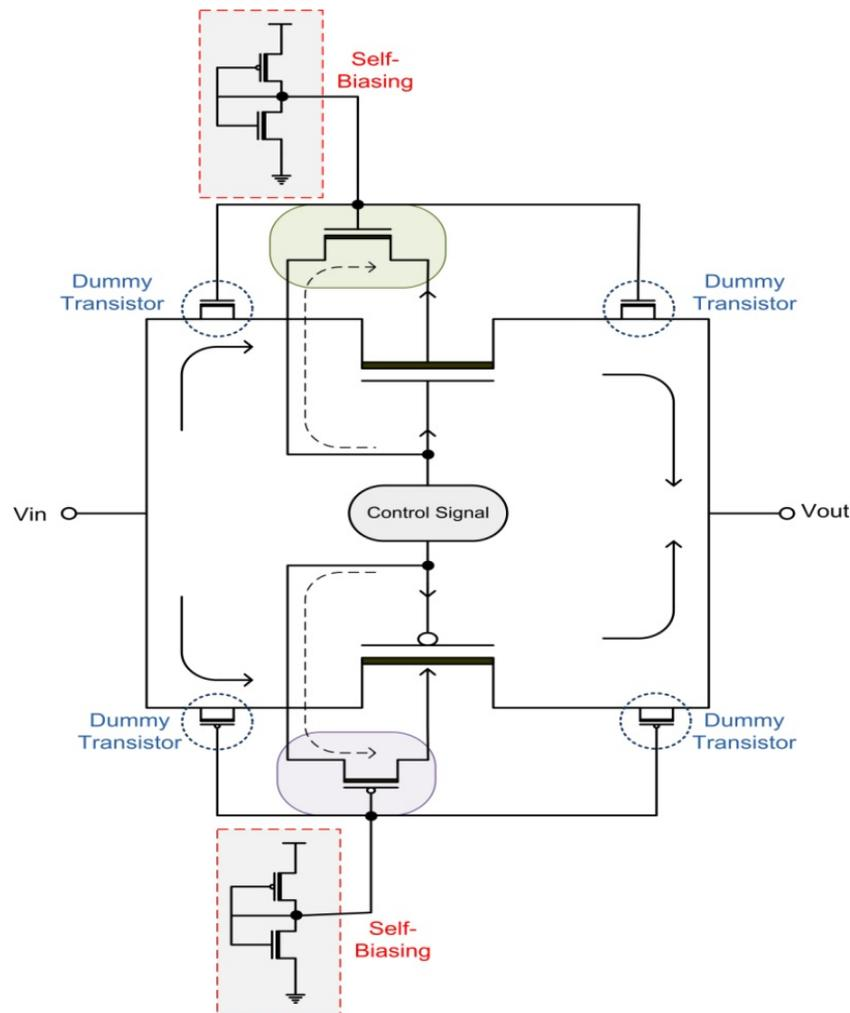
**Figure 6.8: Modified dynamic self-biased switch design used to implement 2:1 multiplexer**
