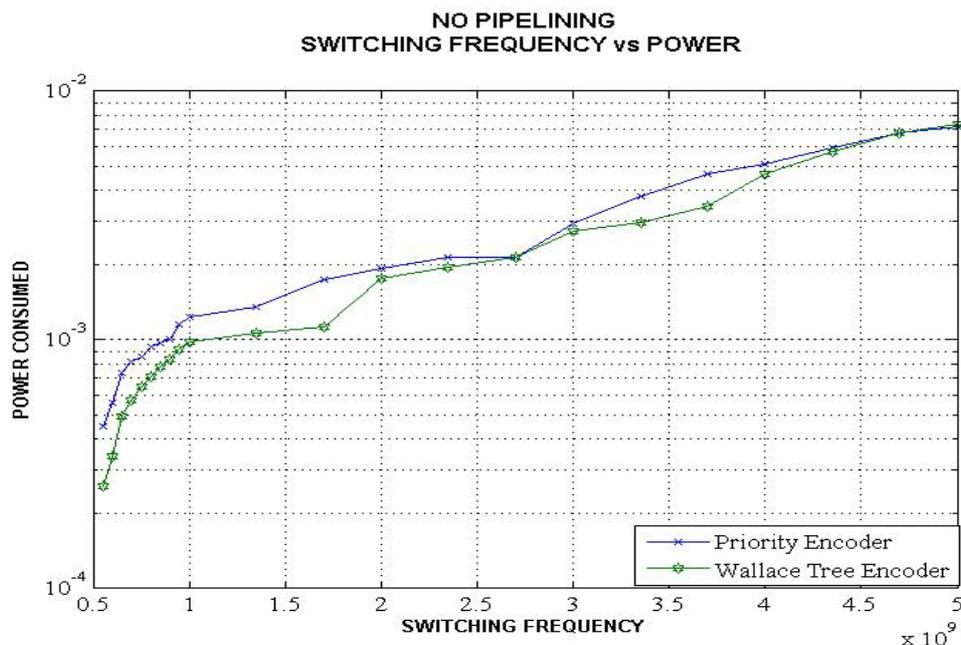
Figure 5.18: Power performance versus switching frequency without pipelining
