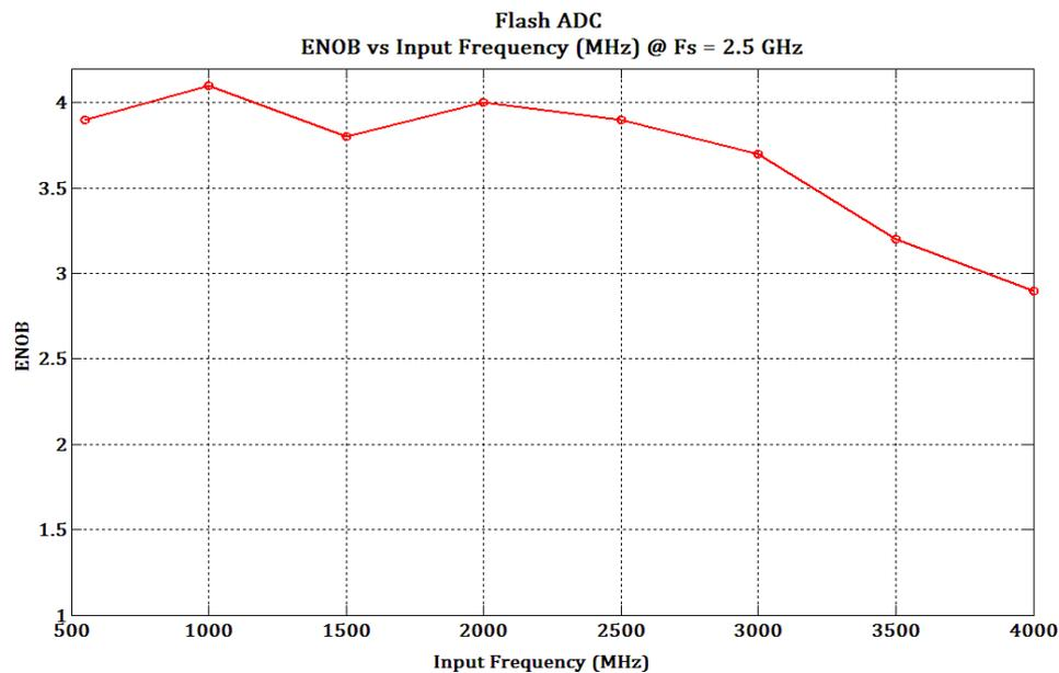
Figure 7.5: Change in the output ENOB for different input frequencies sampled at 2.5 GHz
