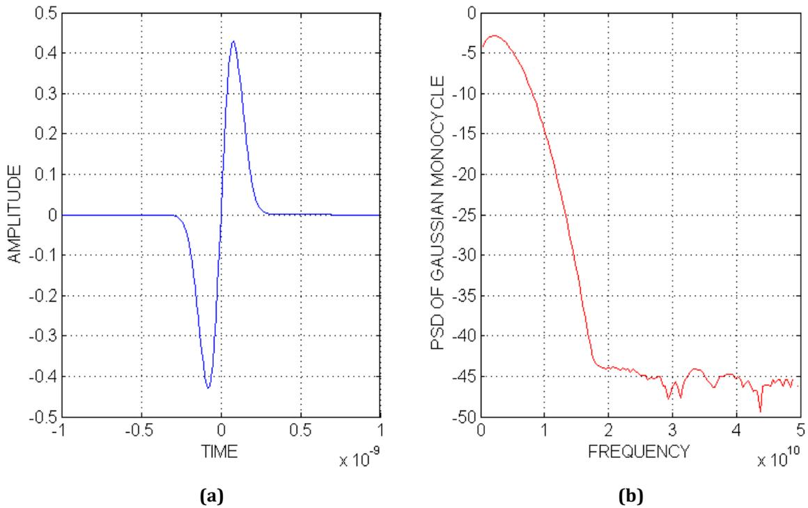
**Figure 2.7: Gaussian first derivative frequency pulse and its corresponding frequency spectrum used for UWB communication**
