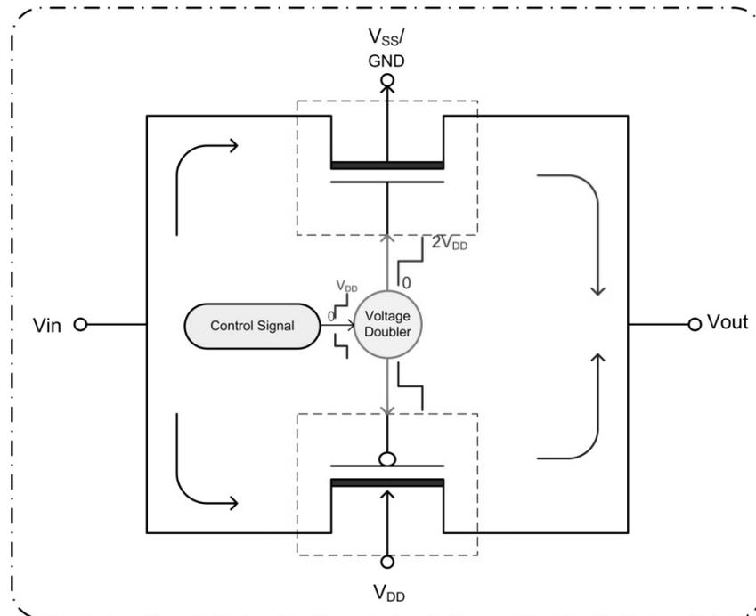
**Figure 6.6: Implementation of bootstrap process using a voltage doubler**
