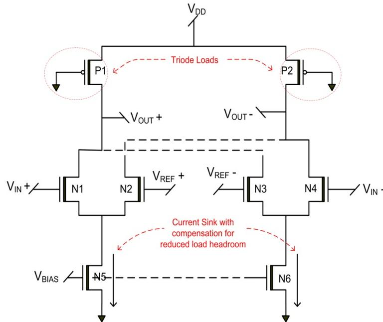
**Figure 4.7: Architecture of the high speed fully differential preamplifier consisting of NMOS differential pairs at the input and PMOS loads biased in triode**
