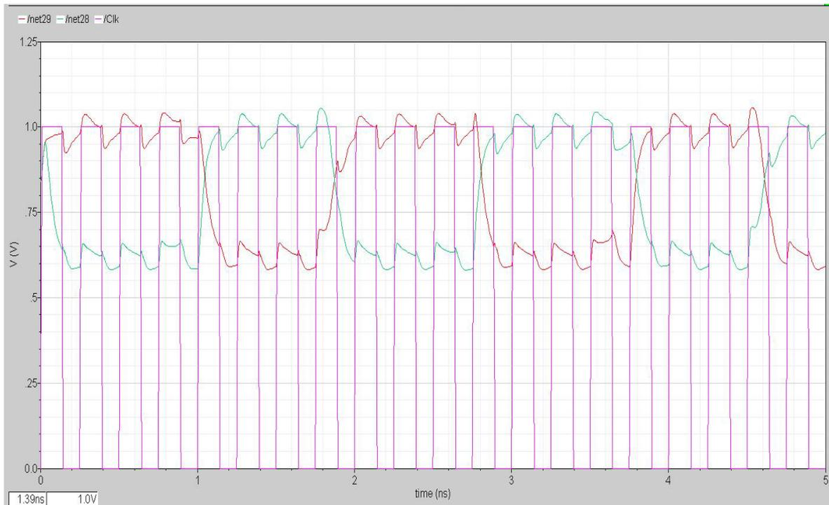
**Figure 4.12: Differential output response of the intermediate track and latch stage. The outputs have been interlaced over the clocking signal to provide an idea of the gain and the low swing operation of the latch**
