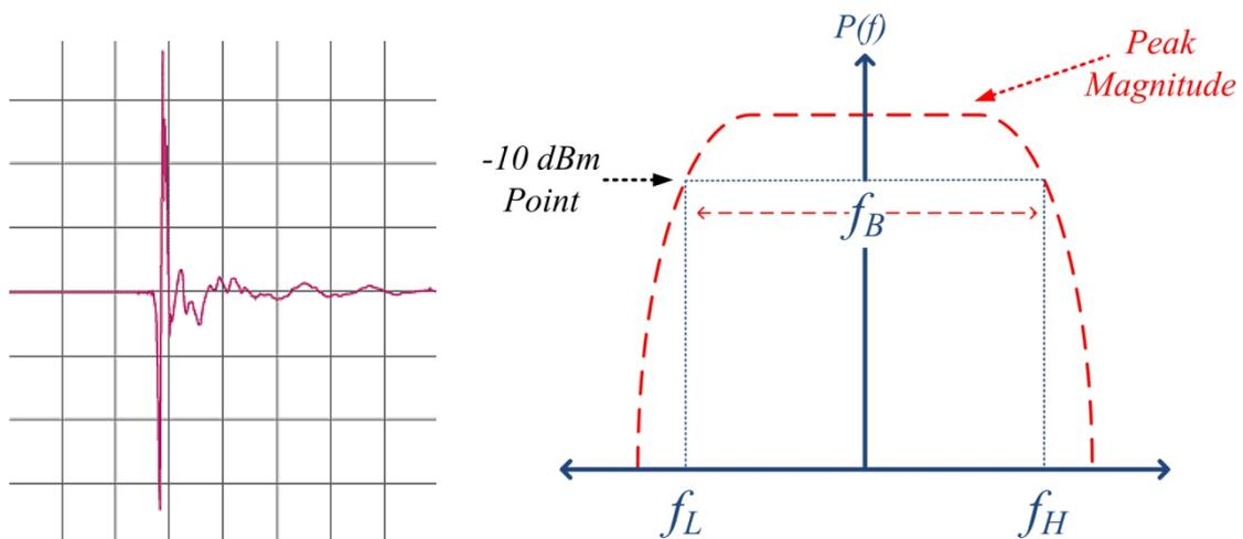
Figure 2.5: Illustration of a UWB pulse and frequency bandwidth for UWB signals with the fractional bandwidth, the upper and lower frequency limits and the -10dBm emission level [12]
