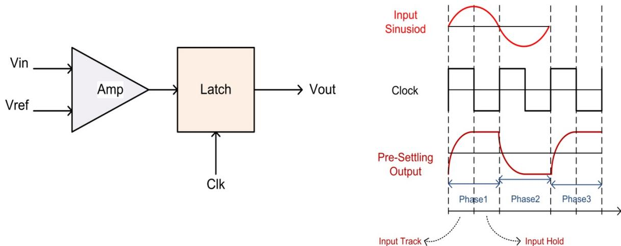
**Figure 4.1: Typical representation of a clock Track and Hold Comparator and its corresponding signalling scheme with pre-settling output**
