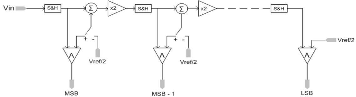
**Figure 6.1: Typical architecture of a pipeline ADC**
