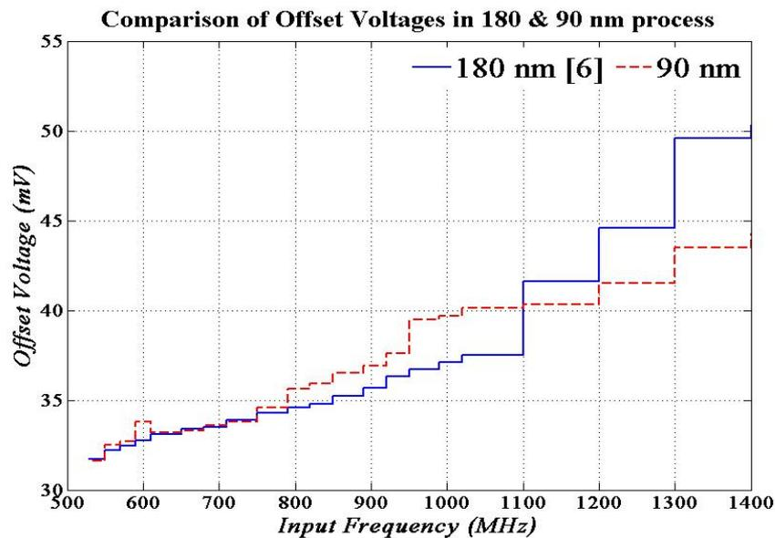
**Figure 4.18: Offset performance of the comparator against the input frequency for both 90nm and 180nm nodes**
