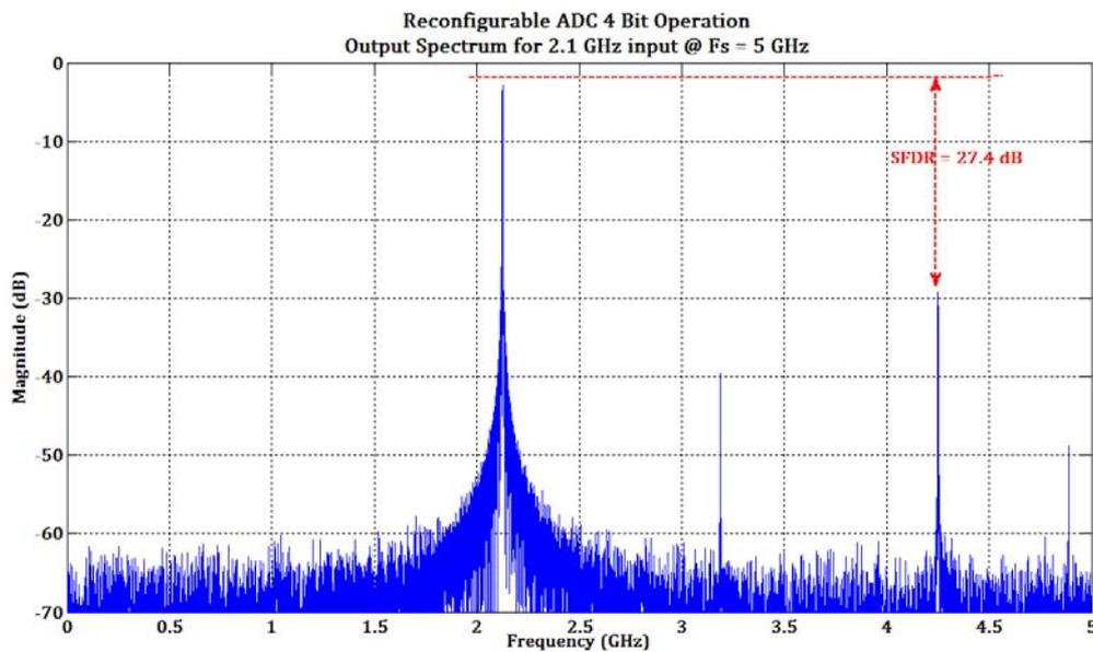
Figure 7.10 (a): FFT output for reconfigurable converter in 4 bit mode
