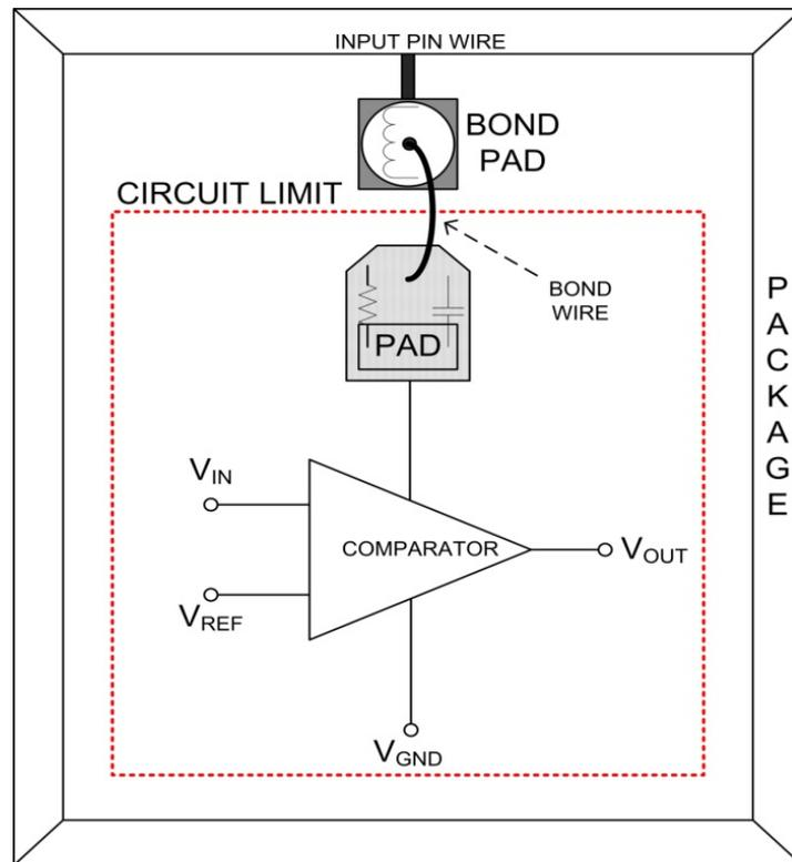
**Fig 4.3: Various components affecting the flow of supply voltage into the comparator circuit from package to circuit level**
