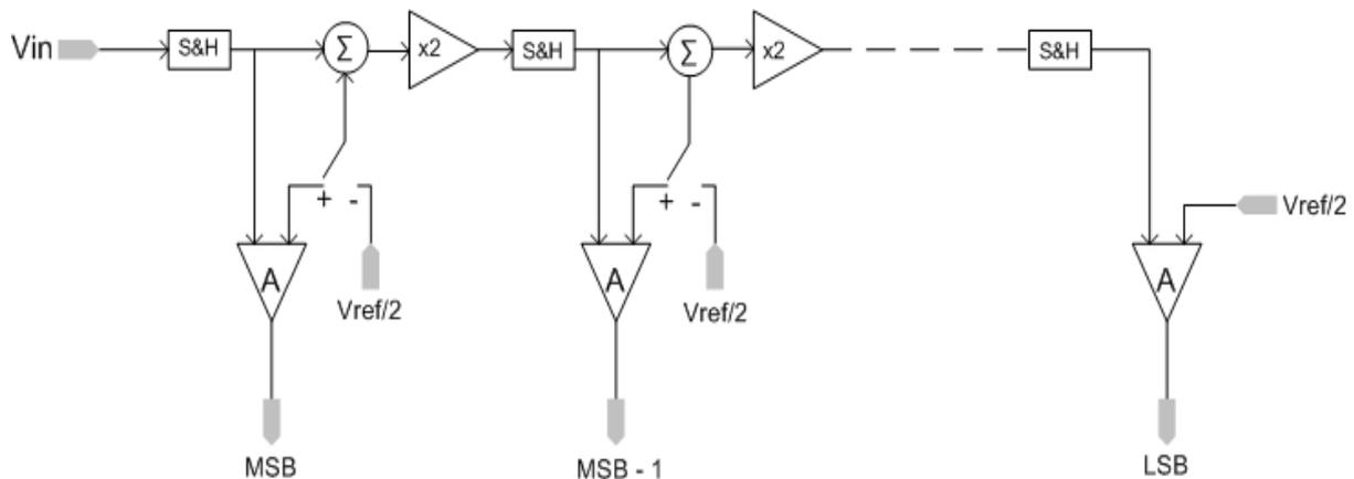
Figure 3.3: Structure of the pipeline analog to digital converter
