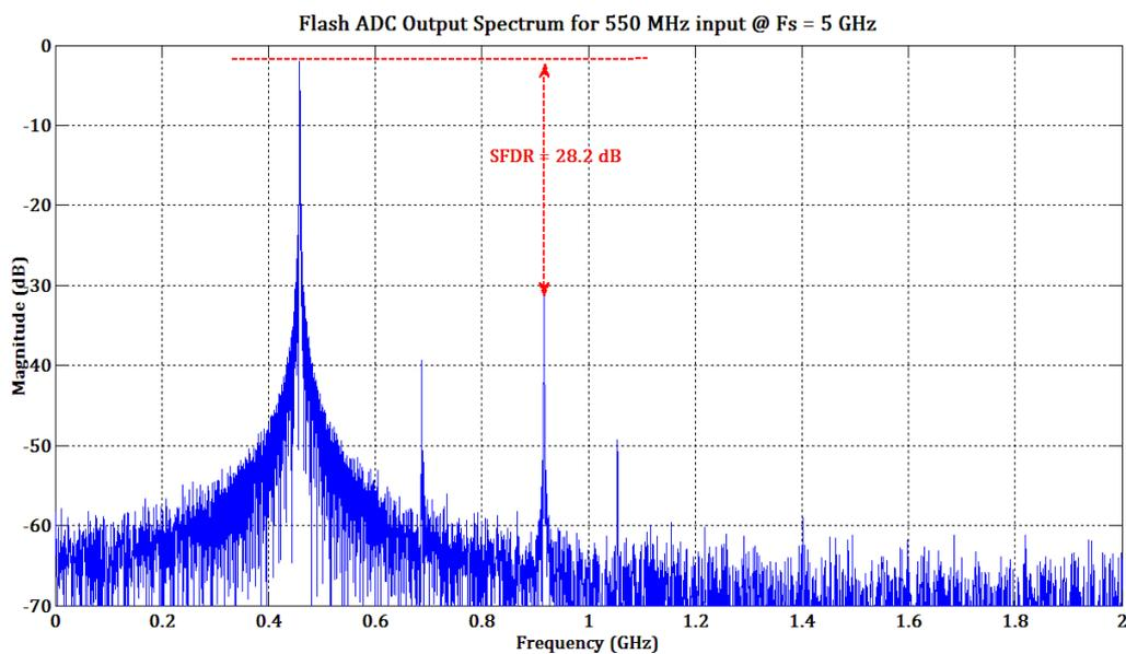
Figure 7.2: Flash ADC Output FFT Spectrum for 550 MHz input sampled at 5 GHz
