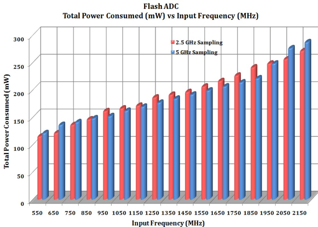
Figure 7.8: Power consumption of the Flash converter
