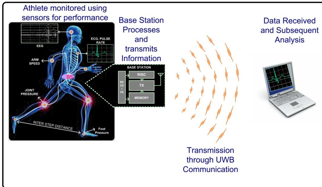
**Figure 2.3: Application of Ultra Wideband transmission scheme put to use in the continuous monitoring of an athlete's training session**
