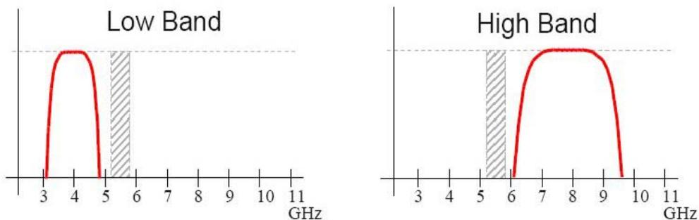
**Figure 2.12: Two main Direct Sequence-Ultra Wideband spectrum bands**
