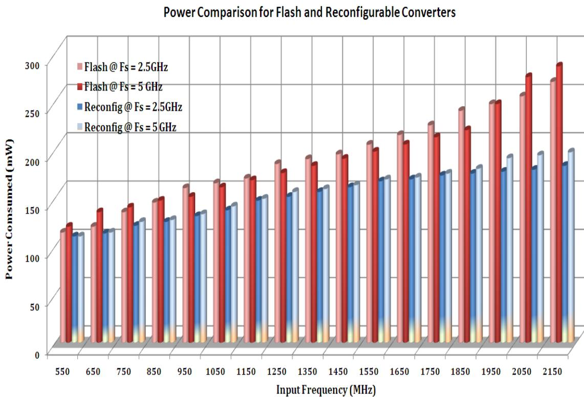
**Figure 7.16: Comparison of the power consumed by the flash and reconfigurable converters**
