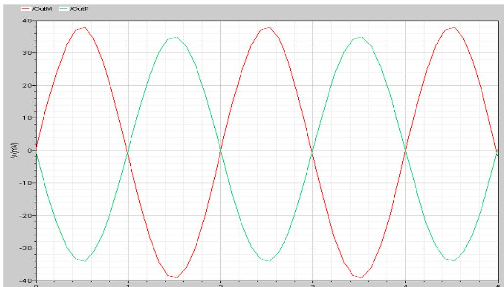
Figure 4.9: Transient output response of the preamplifier for a 30 mV input
