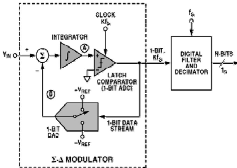
**Figure 3.5: Architecture of a Sigma-Delta Analog to Digital converter consisting of an integrator, comparator, switch DAC and decimation filter [45]**
