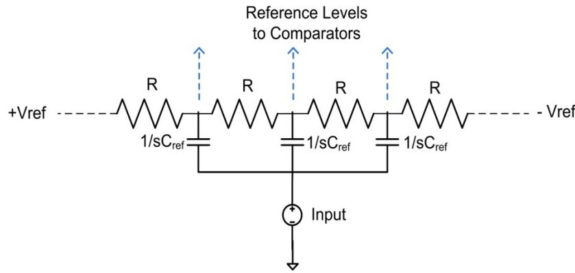
**Figure 5.8: Small signal circuit for input feed through analysis of the reference ladder used in Flash ADC**
