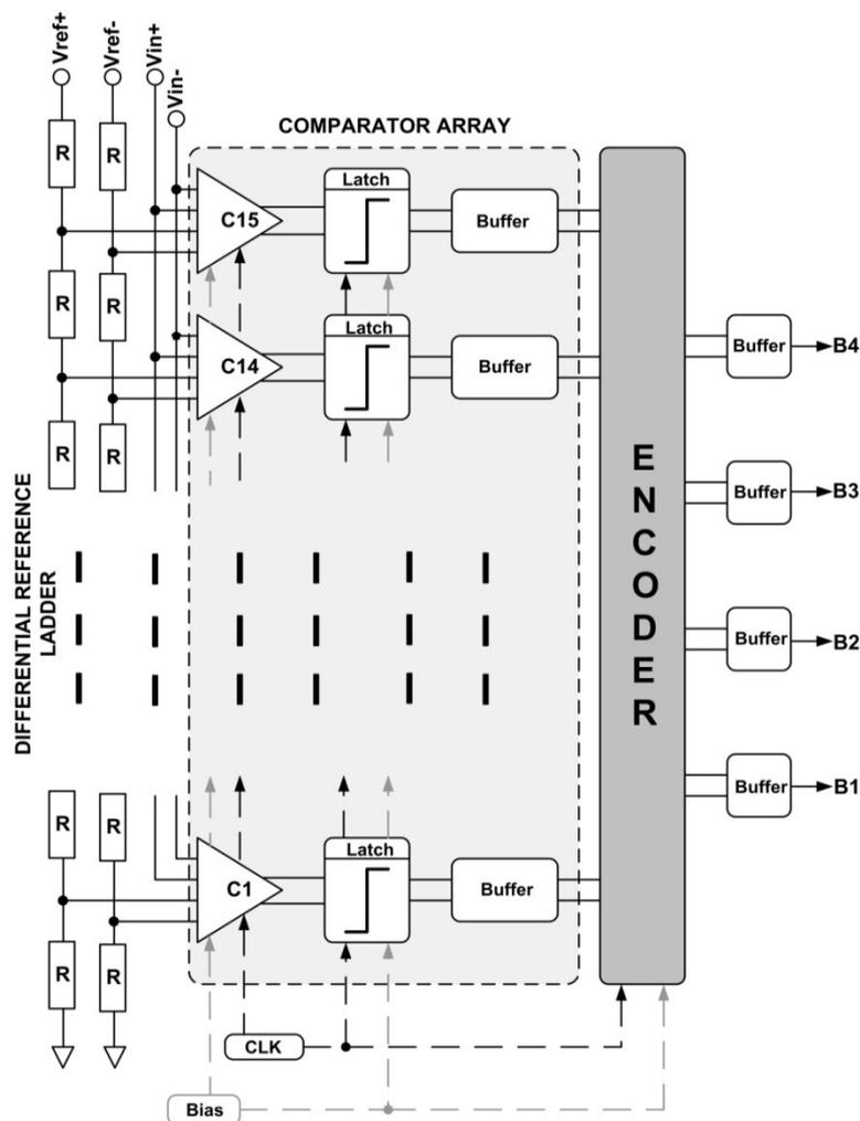
Figure 5.6: Illustrates a complete 4-bit Flash ADC system including differential reference ladder, comparator array and encoder
