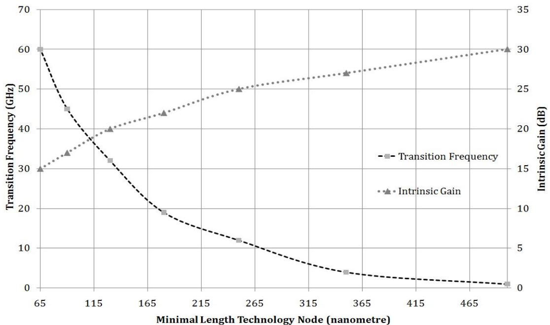
**Figure 4.5: Variation in the Transition Frequency and Intrinsic Gain for a single transistor with overdrive of 0.4 V for different technology nodes at minimal length [66-68]**
