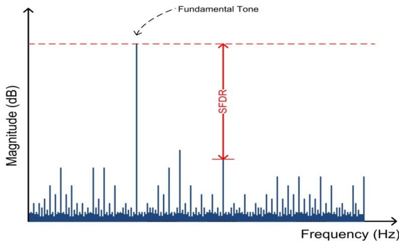
Figure 5.4: SFDR measurement range for an analog to digital converter
