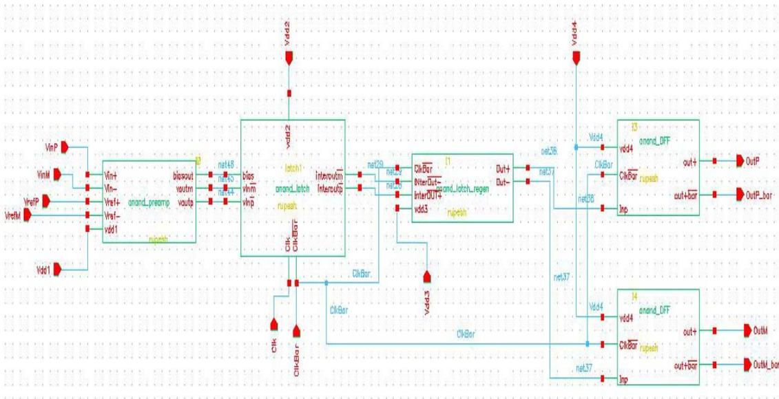
**Figure 4.15: Final implementation of the 4 stage comparator consisting of an open loop preamplifier, two latching stages with positive feedback and a output buffer**
