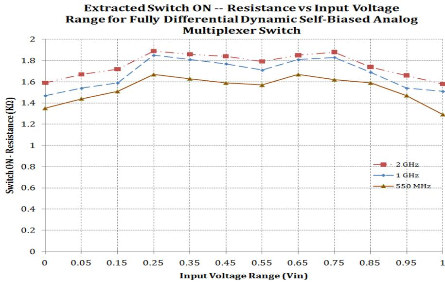
**Figure 6.9: Extracted ON resistance for different input frequencies of the novel modified fully differential dynamic self-biased switch**
