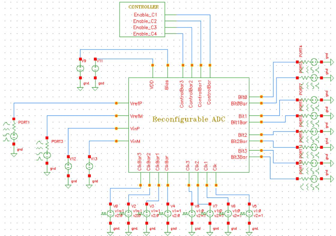
Figure 7.9: Test bench of the implemented differential reconfigurable converter
