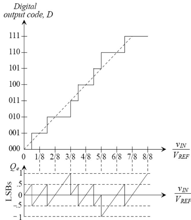
**Figure 5.2: Differential non linearity of the analog to digital converter along with the deviation in quantisation levels [76]**
