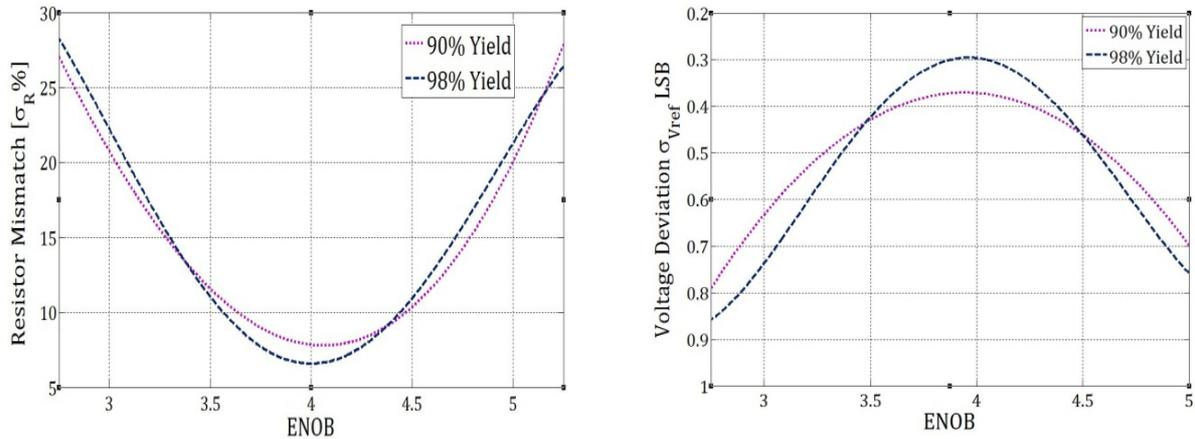
**Figure 5.10: Mismatch and voltage deviation for the resistor ladder**
