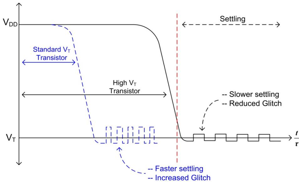
Figure 6.12: Settling time comparison between SVT and HVT transistors
