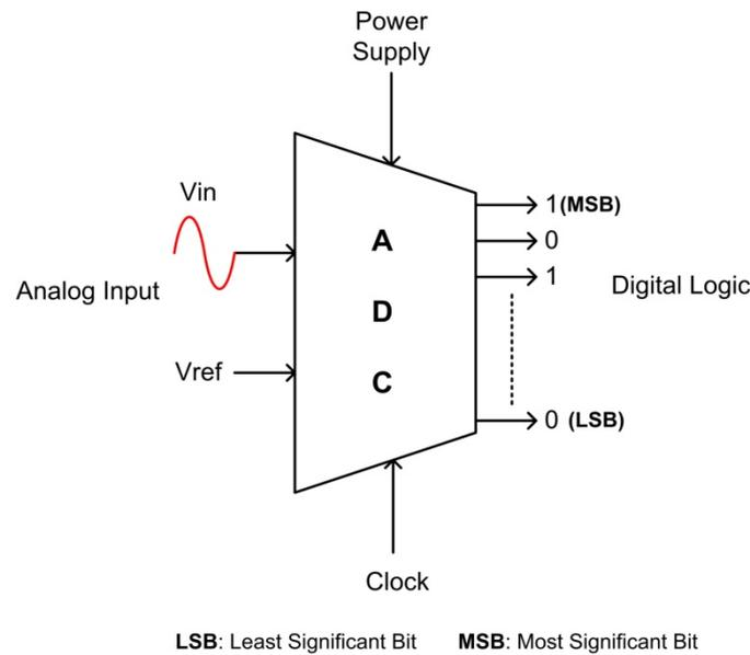
**Figure 3.1: Functional representation of the analog to digital conversion process**
