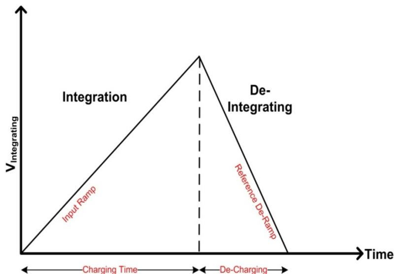
Figure 3.6: Timing diagram for a dual slope integrating analog-to-digital converter
