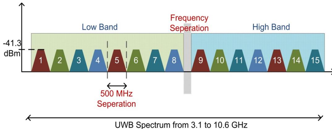
**Figure 2.10: MBOA proposal for 3.1 to 10.6 GHz Ultra Wideband frequency spectrum with each band having a minimum frequency of 500 MHz**
