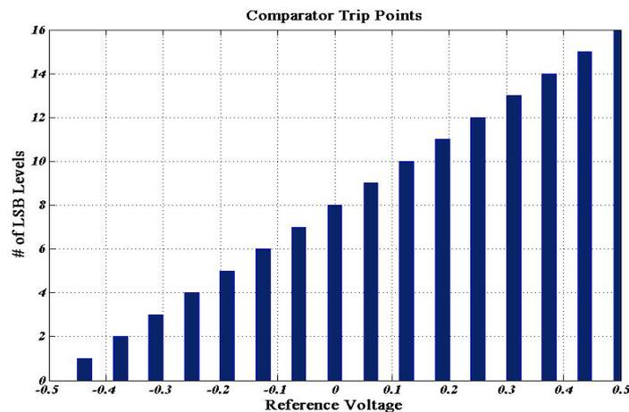
**Figure 4.16: Different comparator trip points used to test functionality for a 4 bit FLASH Analog to Digital Converter reference levels**
