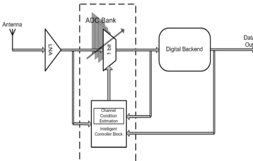
**Figure 1.2: Representation of the Novel Reconfigurable Architecture**
