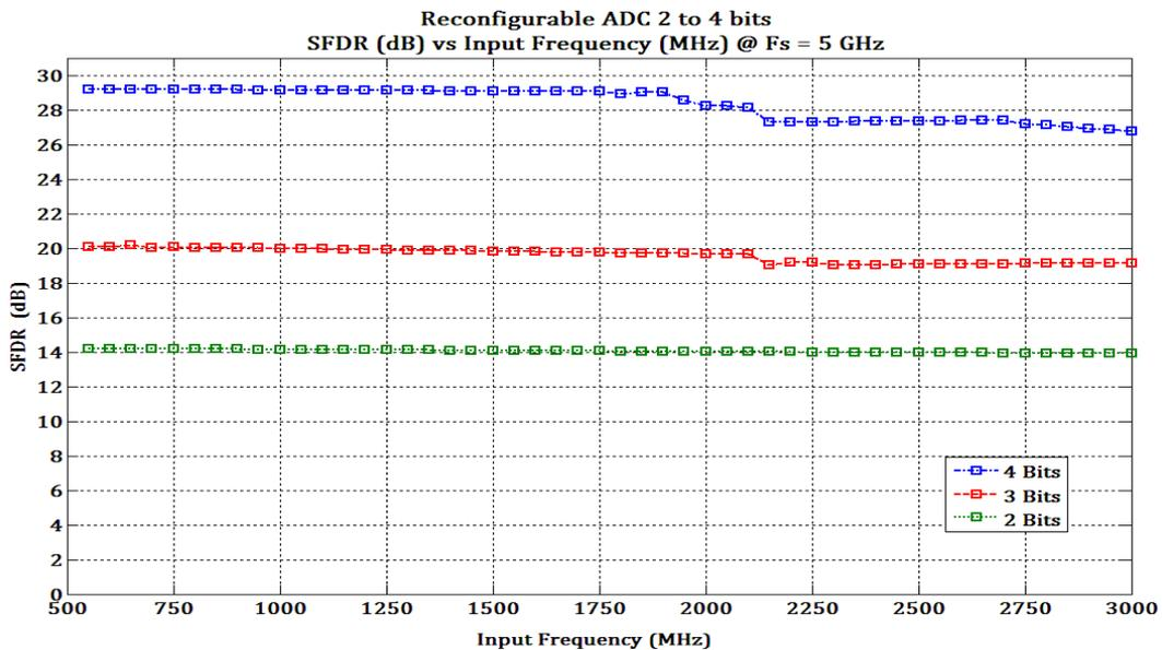
**Figures 7.12 (a) and (b): Variation in the SFDR for different input frequencies of the reconfigurable converter operating from 2 to 4 bits, sampled at 2.5 and 5 GHz respectively**
