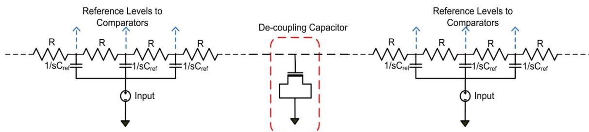
**Figure 5.9: Reference net de-coupled into sections using an active NMOS as the dynamic de-coupling capacitor**
