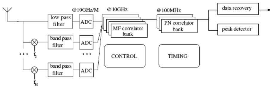
**Figure 2.11: Channelized MB-OFDM UWB receiver topology consisting of parallel ADC and high performance Matched Filters [32]**
