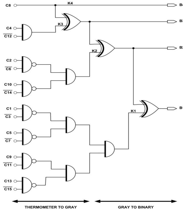
Figure 5.12: Gate level implementation of the thermometer to binary encoder
