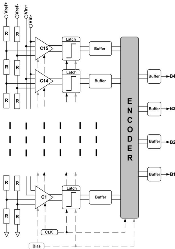
**Figure 3.2: Typical FLASH Analog to Digital Converter architecture with the reference ladder network, comparator bank and encoder**
