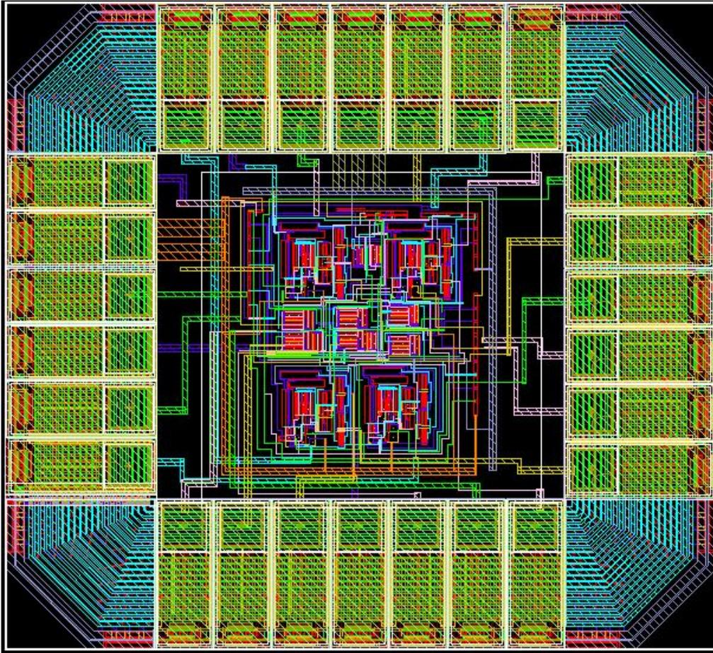
**Figure 6.16: Complete chip level layout implementation of the novel reconfigurable analog to digital converter**
