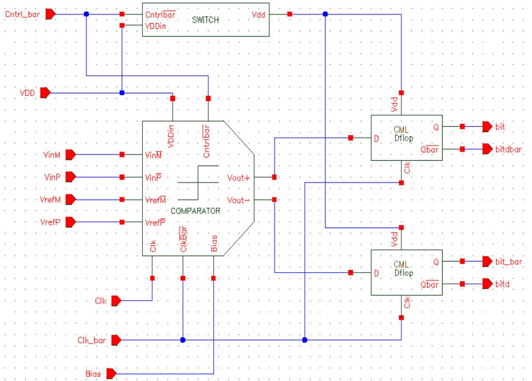
**Figure 6.11 (b): Comparator circuit with the enable circuit**
