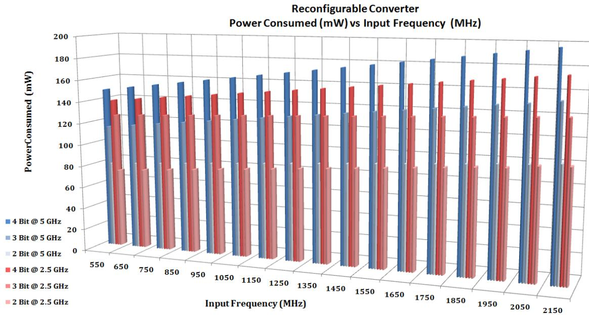
**Figure 7.15: Power consumption of the reconfigurable converter along with estimated impact of controller consumption**
