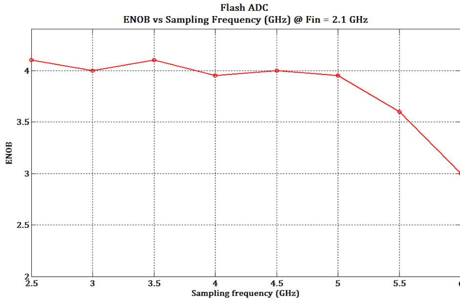
**Figure 7.6: Change in output ENOB for different sampling frequencies for a 2.1 GHz sinusoidal input signal**
