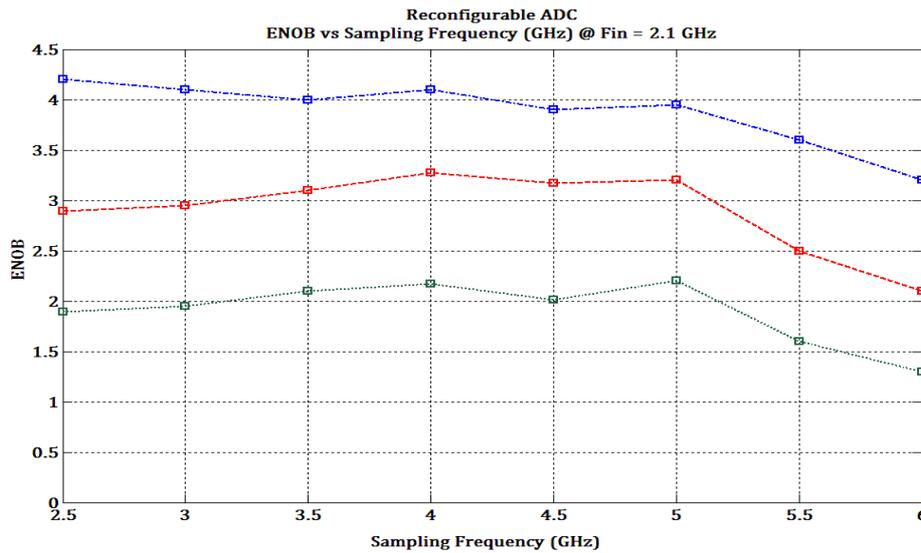
**Figure 7.13: Variation in ENOB versus the sampling frequency during 2 to 4 bit operation for 2.1 GHz input signal**
