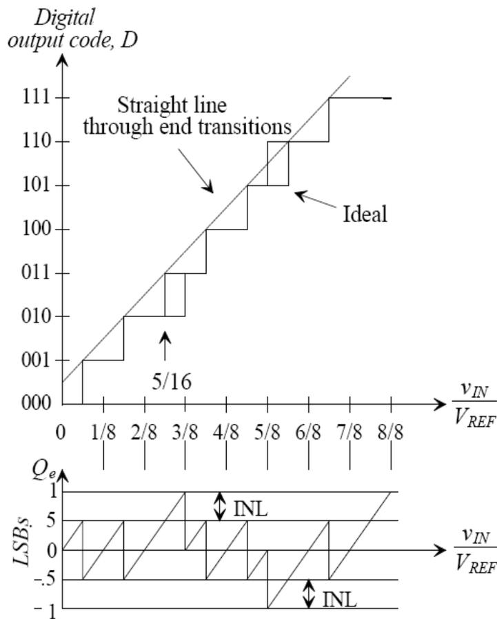
**Figure 5.3: Integral non linearity of the analog to digital converter along with the deviation in quantisation levels [76]**
