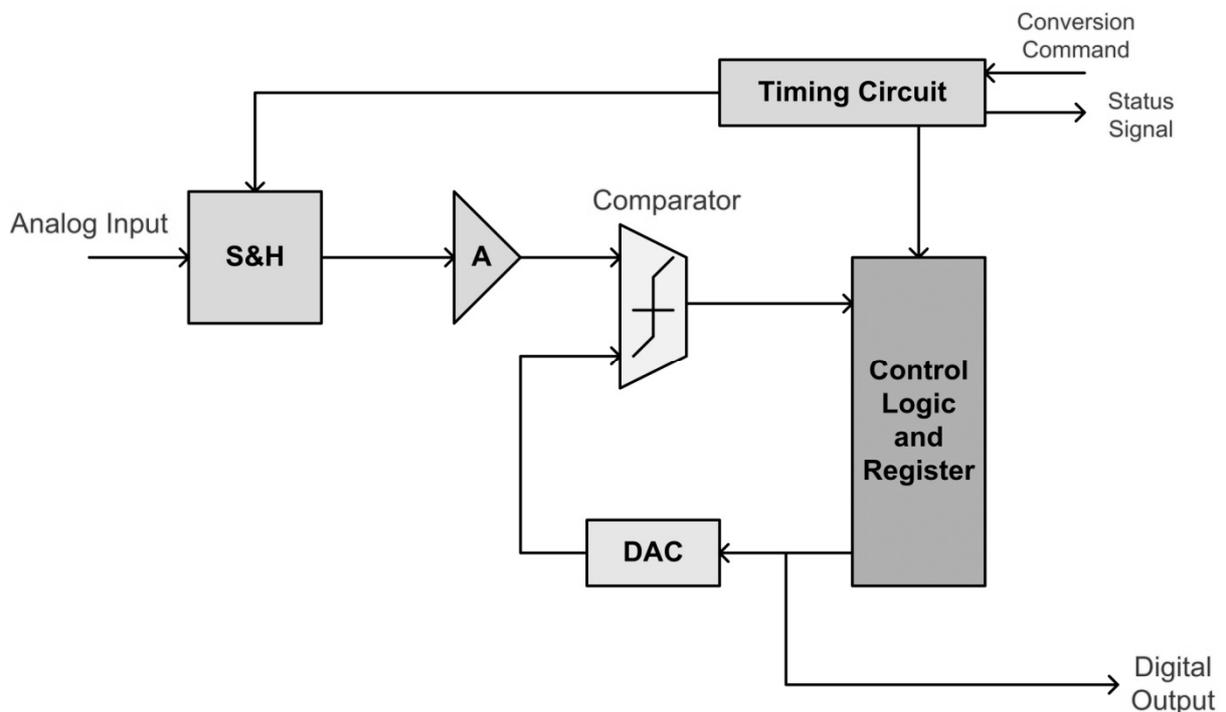
Figure 3.4: Successive Approximation Register (SAR) mixed signal device
