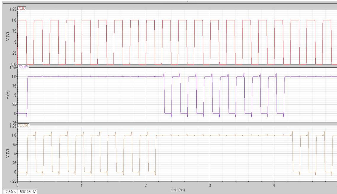
**Figure 4.17: Final comparator output at the end of the buffer stage which was used to settle the output slewing that was prevalent in the previous stage**
