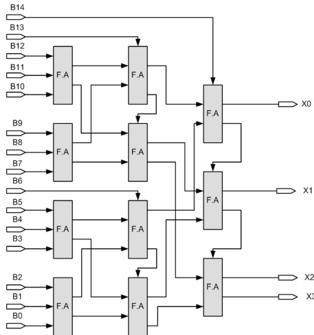
**Figure 5.13: Thermometer to binary encoder using the Wallace Tree methodology**
