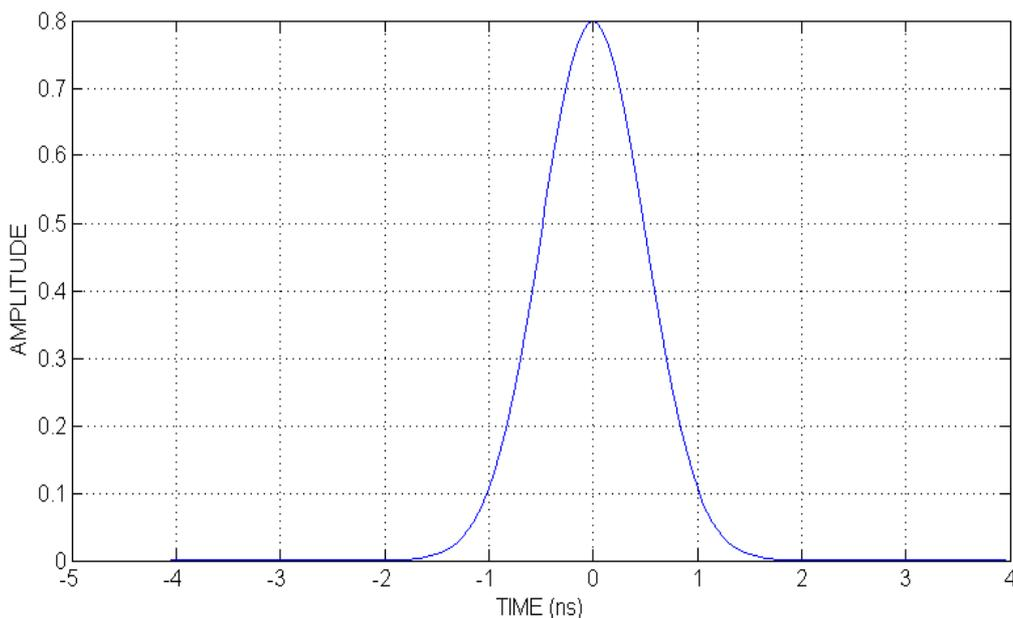
**Figure 2.6: Pulse shape of a typical Gaussian signal used for UWB communication**
