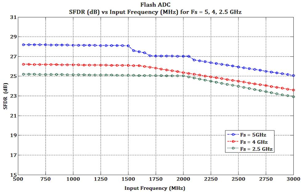
Figure 7.4: Comparison of the SFDR vs the Input Frequency range for 3 different sampling rates
