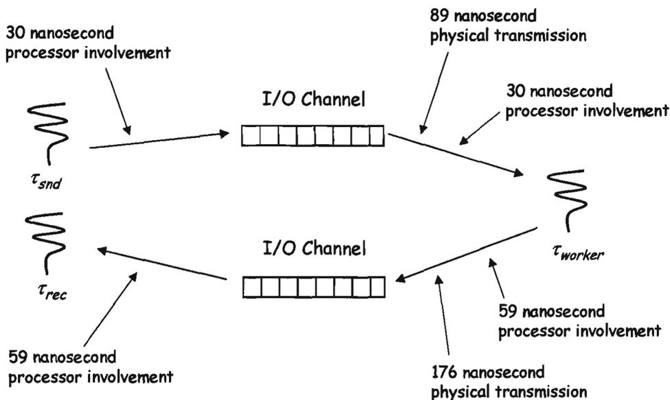
**Figure 5.11** Delay times to simulate network communication delays
