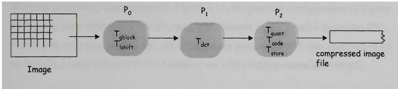
**Figure 4.10** Pipeline implementation of SV1 with 3 processors
