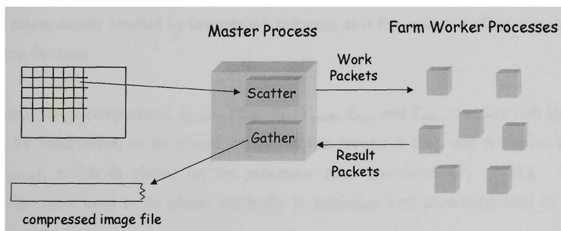
**Figure 4.12** Application of processor farm technique to image compression
