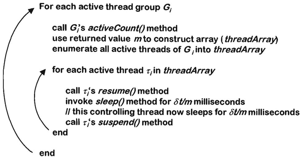
**Figure 5.9** Pseudocode for simulation algorithm SIM2
