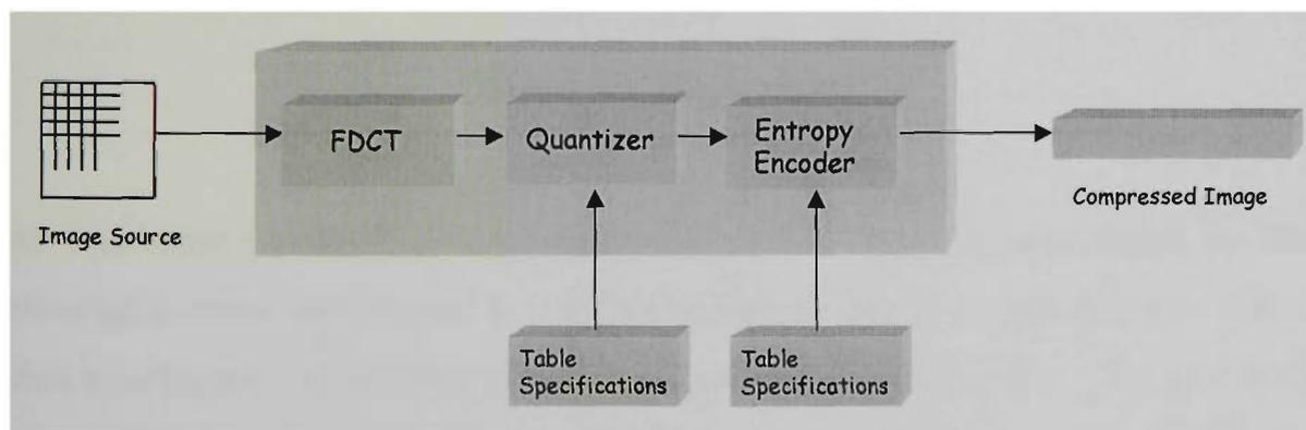
**Figure 3.3** General structure of DCT based encoder
