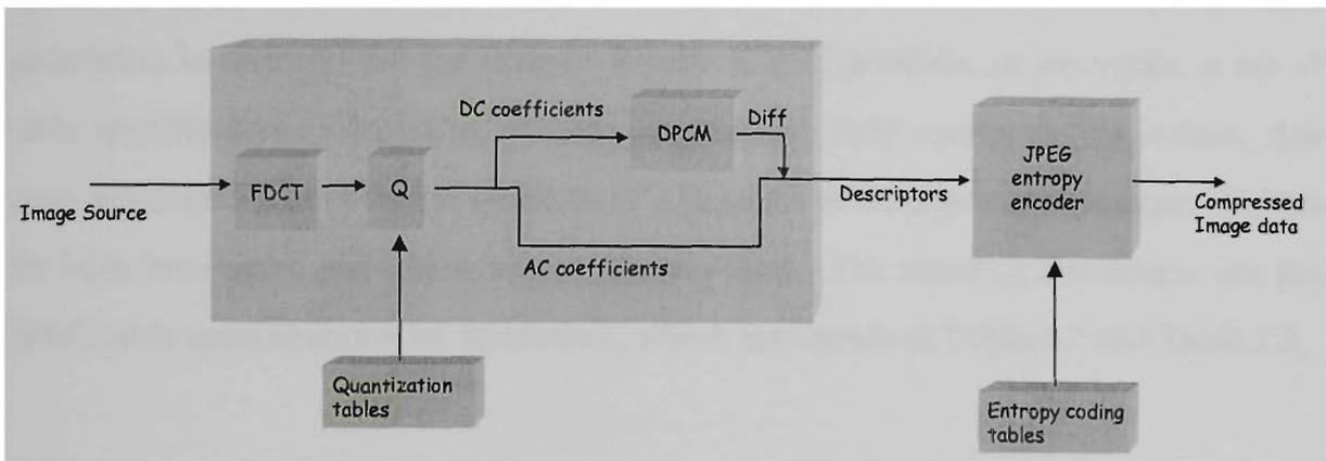
**Figure 3.12** Baseline sequential-DCT encoder model
