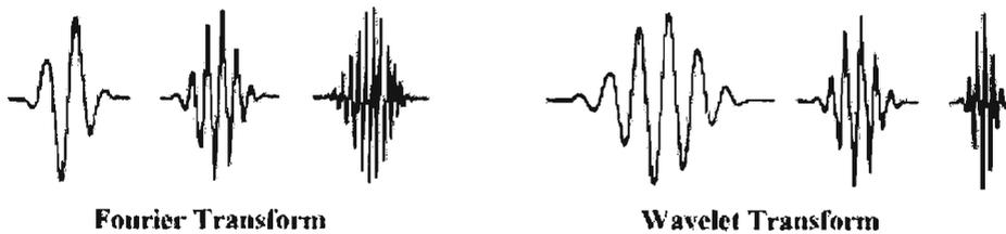
**Figure 2.17** Discrete fourier basis functions vs. scaled wavelet basis functions
