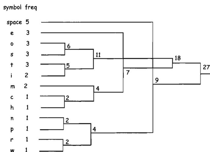
**Figure 2.3** Huffman tree built from frequencies in Table 2.2
