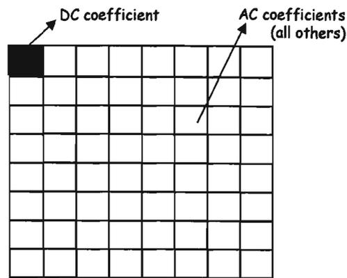
Figure 3.7 Transformed block coefficients
