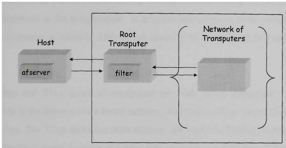
**Figure 3.18** General form of transputer system connected to PC host
