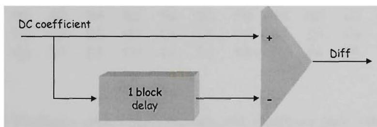
**Figure 3.13** DPCM model for DC coefficient encoding
