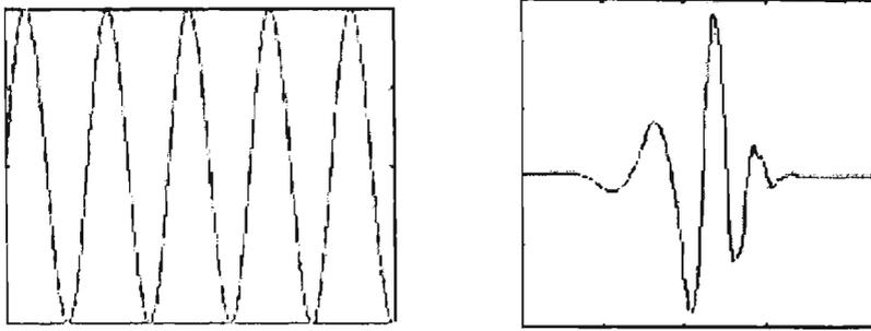
**Figure 2.15** Comparison of sine wave and Daubechies wavelet
