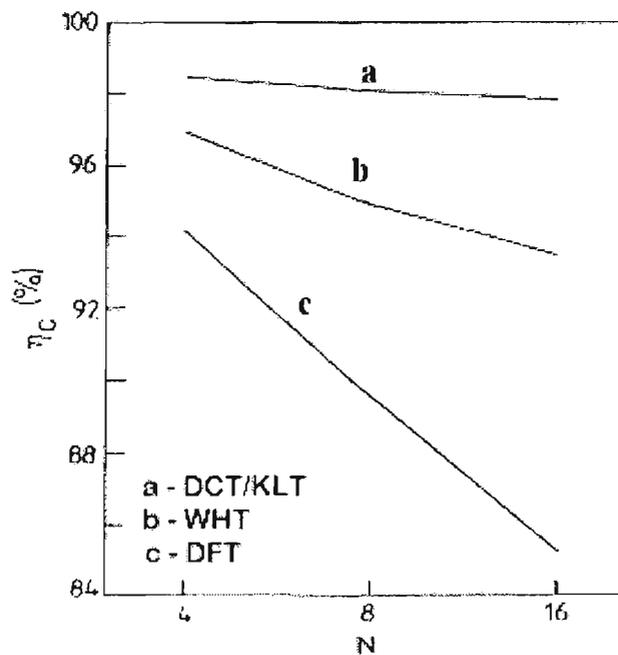
Figure 2.13 Decorrelation efficiency as a function of transform block size [15]
