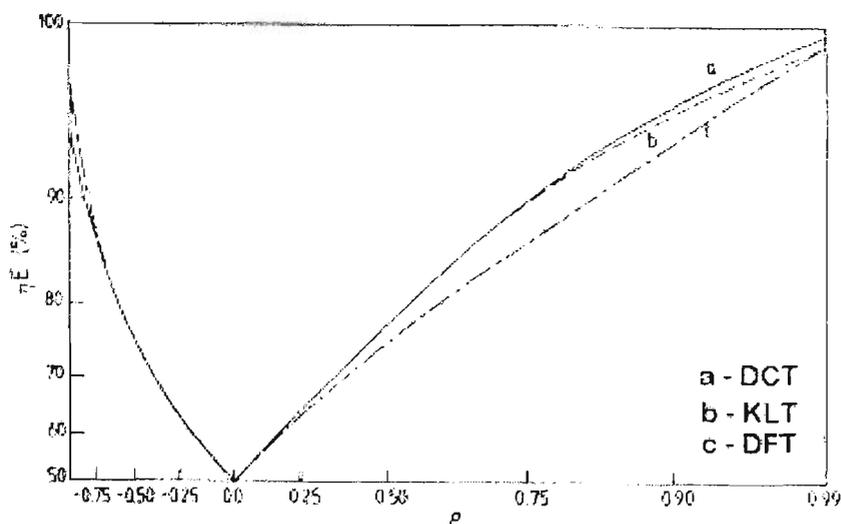
**Figure 2.10** Energy packing efficiency as a function of correlation coefficient [15]
