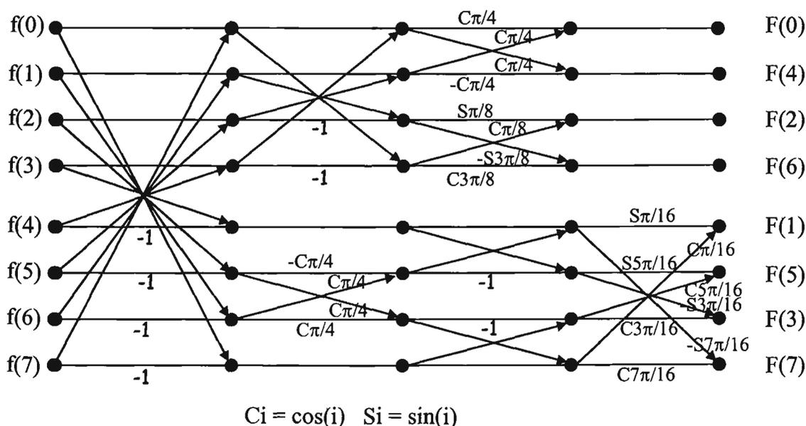
Figure 3.11 Signal flow graph for fast DCT [14], [70]
