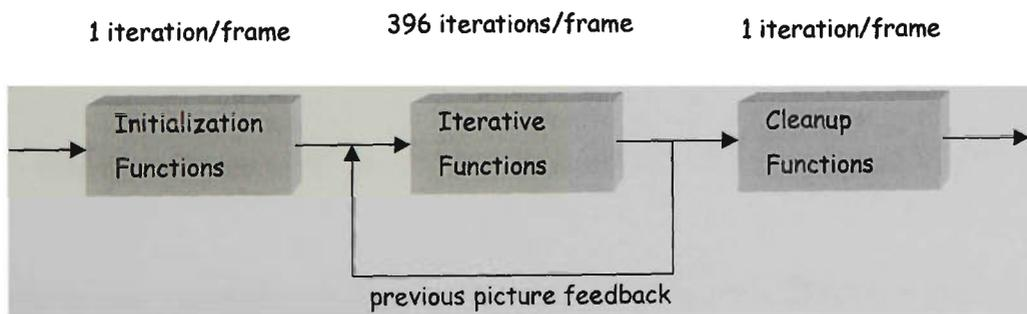
**Figure 3.25** Simplified representation of H.261 encoding execution
