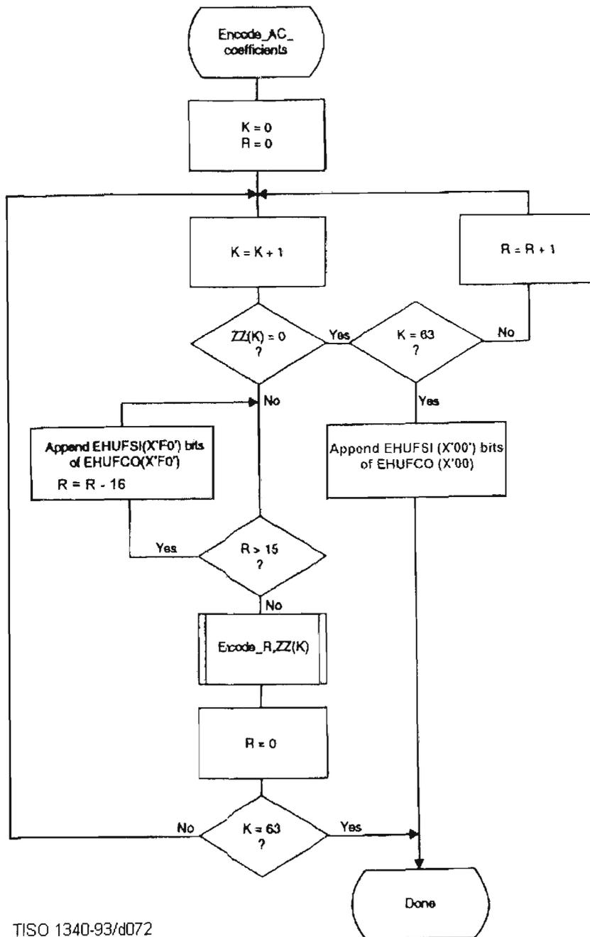
**Figure A.3** Sequential encoding of AC coefficients with Huffman coding
