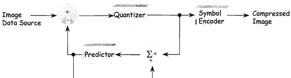
Figure 2.7 DPCM lossy encoder block diagram
