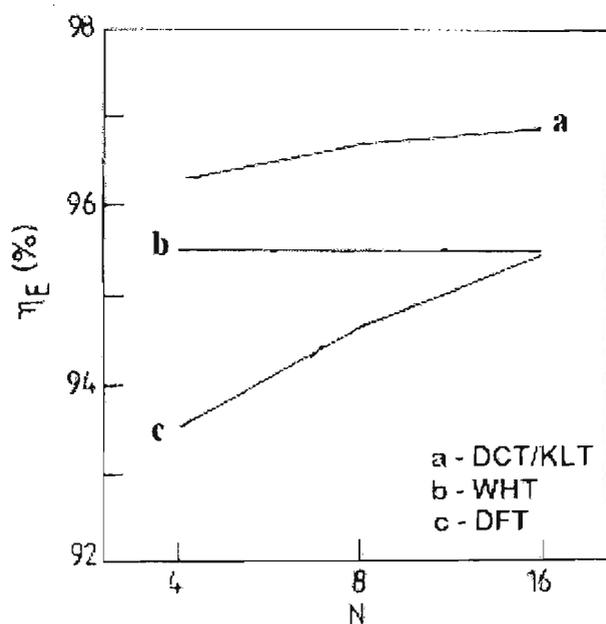
**Figure 2.11** Energy packing efficiency as a function of transform block size [15]
