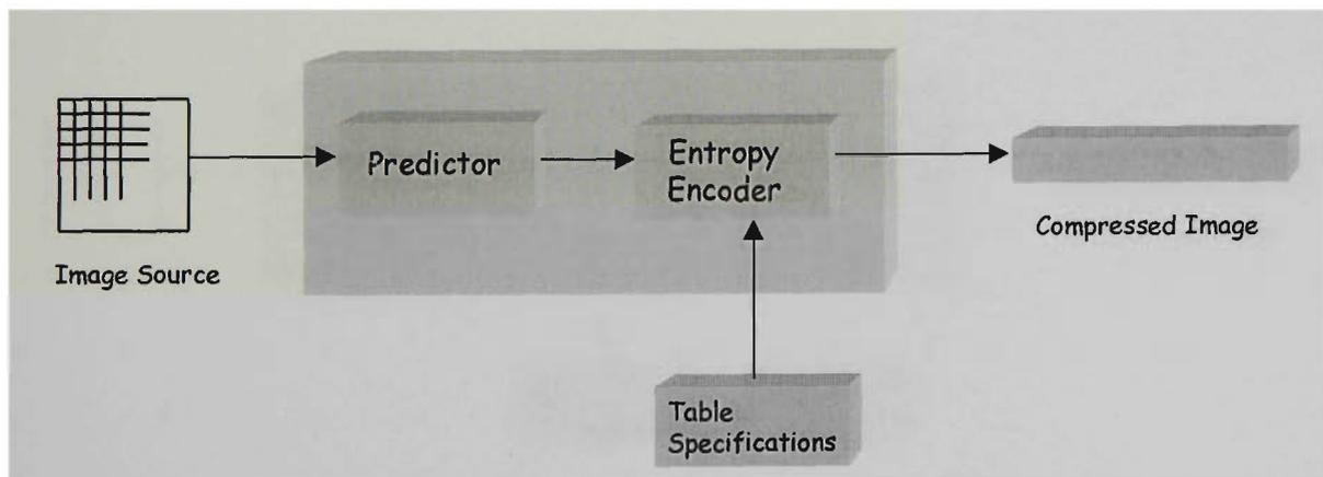
Figure 3.1 Structure of lossless encoder [52]
