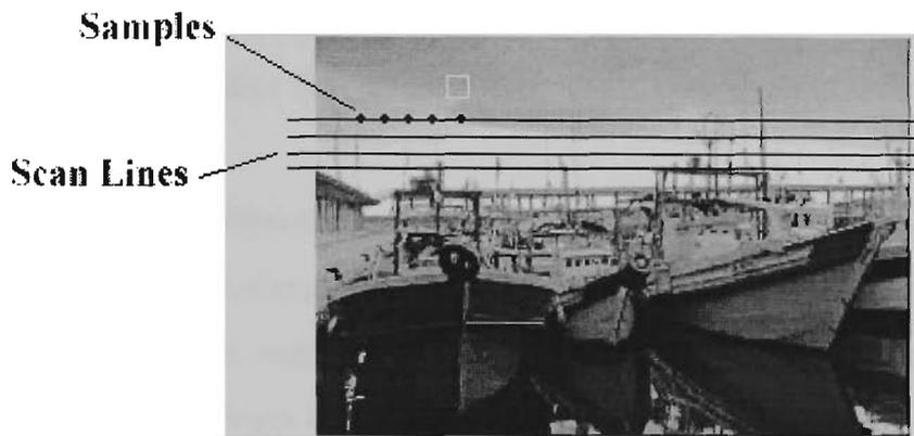
**Figure 2.1** Construction of digital image
