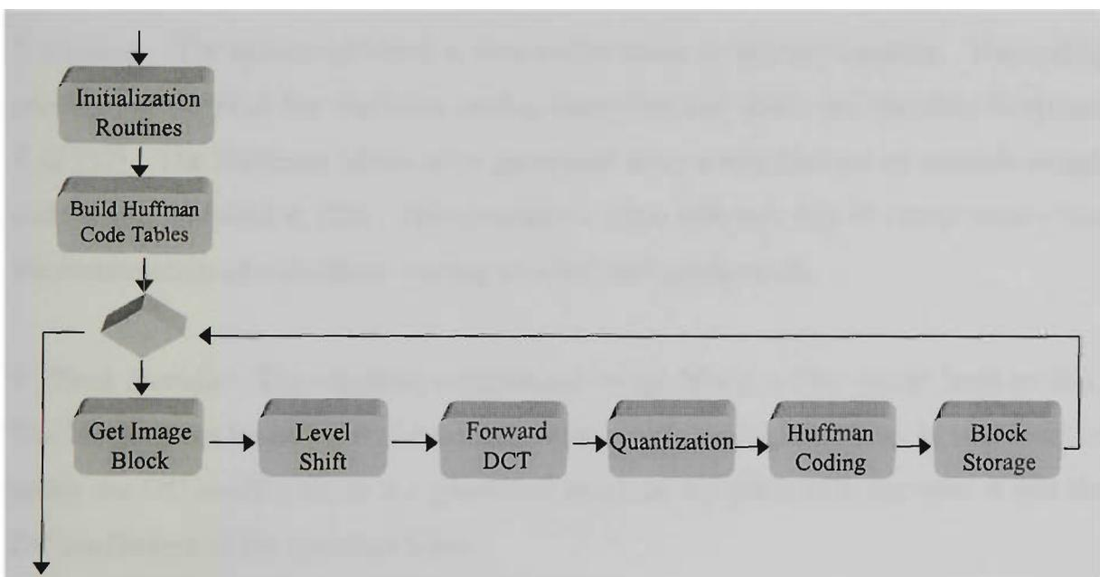
Figure 4.2 Sequential algorithm SV1 main components
