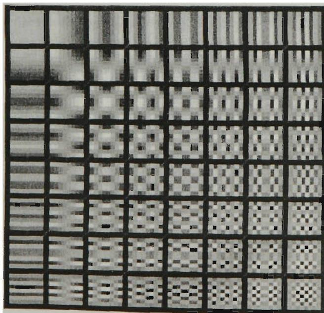
Figure 3.8 Two-dimensional  $8 \times 8$  DCT basis functions [70]
