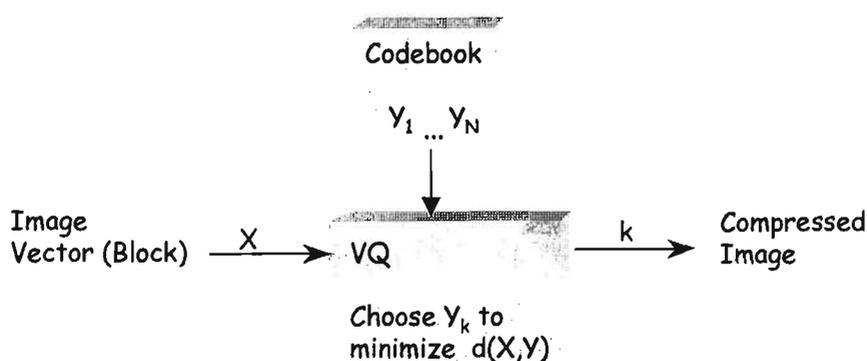
**Figure 2.14** Vector quantization block diagram
