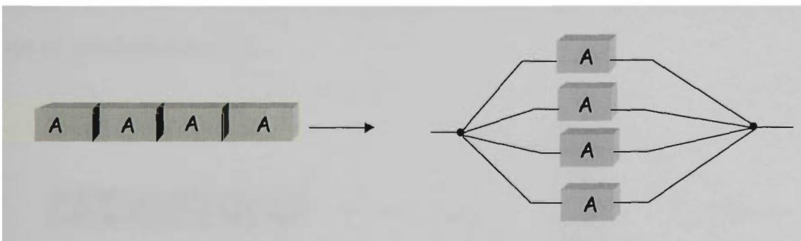
Figure 3.20 Homogeneous parallelization [10]
