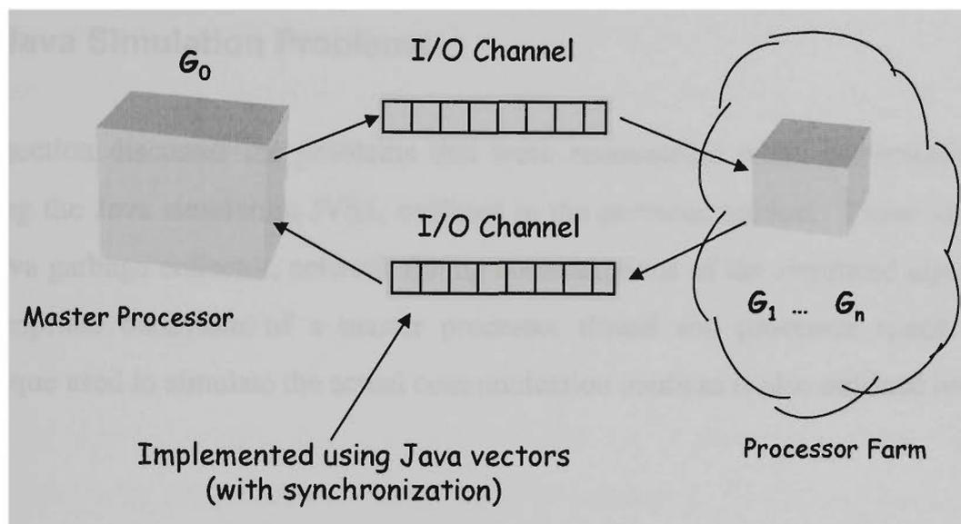
**Figure 5.10** Use of Java vectors to simulate message passing
