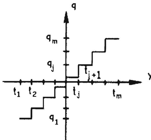
Figure 2.9 Typical I/O characteristics of a quantizer [48]
