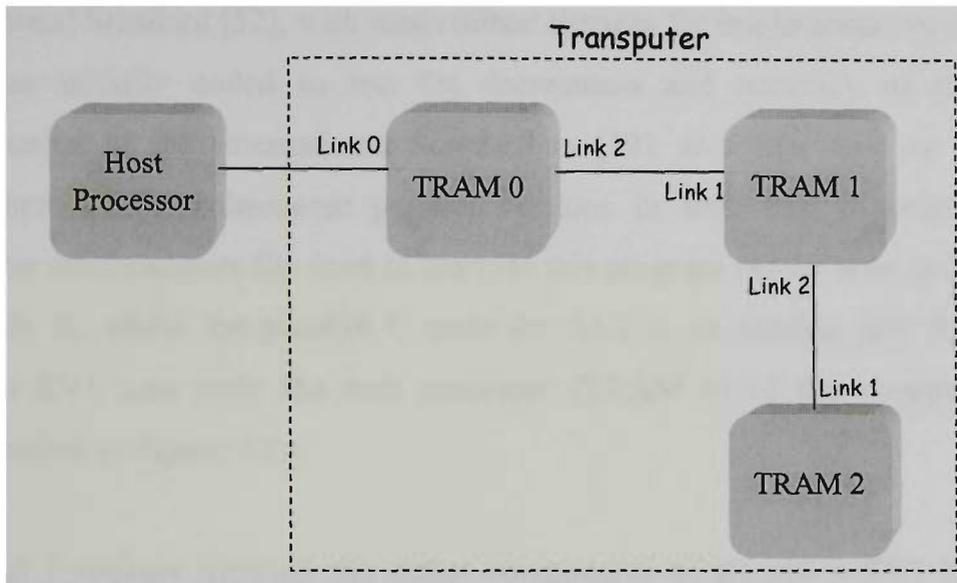
**Figure 4.1** Physical transputer configuration with three processors
