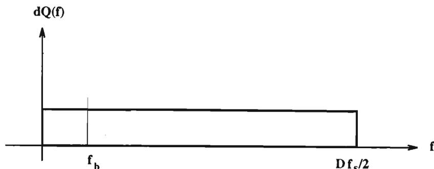
Figure 2.8: Oversampling for reducing the average level of quantization noise density, when  $Df_s \gg f_b$ , the baseband noise is much smaller than that of the conventional ADC converters.
