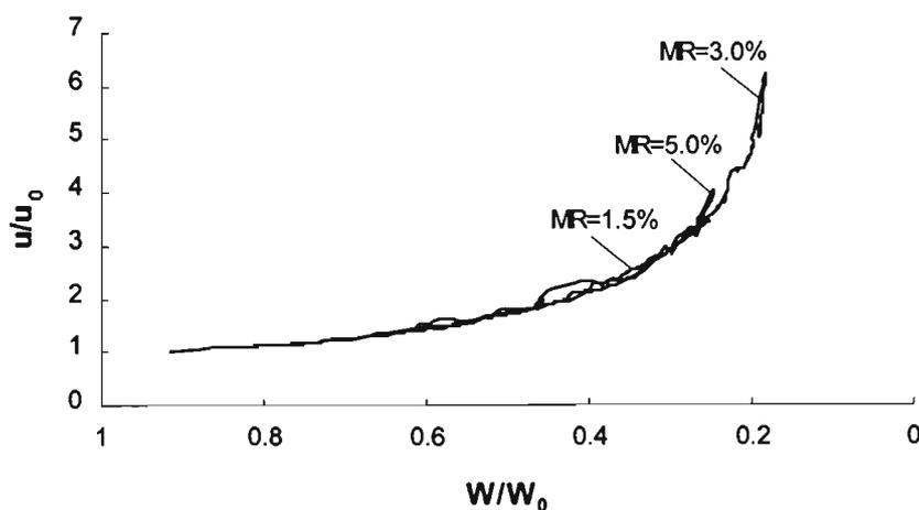
Fig. 6.8: Displacement change corresponding to different  $MR$  (cantilever beam).
