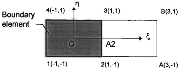
Fig. 4.3: A four-node isoparametric element.
