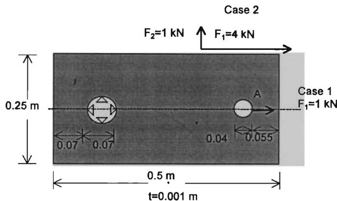
Fig. 5.9: Design domain of a lever arm.
