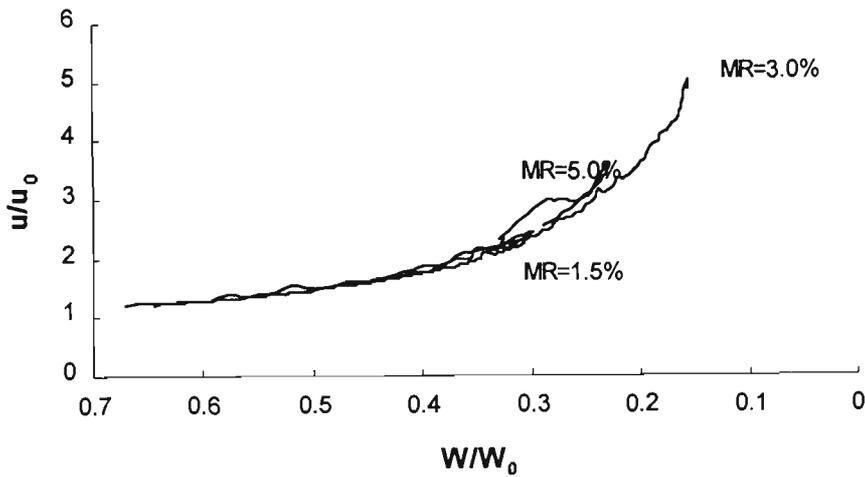
Fig. 6.14: Displacement change corresponding to different  $MR$  (three-point loaded beam).
