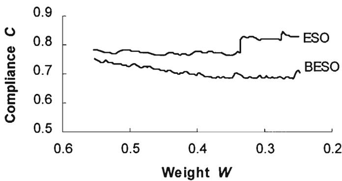
Fig. 5.14: Changes in mean compliance vs. structural weight (descending stage).
