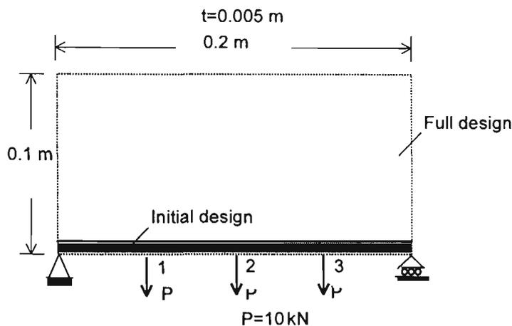
Fig. 5.1: Three-point loaded beam.
