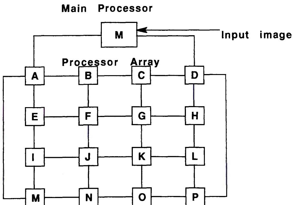
Figure 6: Mapping the source image onto a transputer network.
