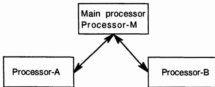
Figure 2: Tree topology for a network of three transputers
