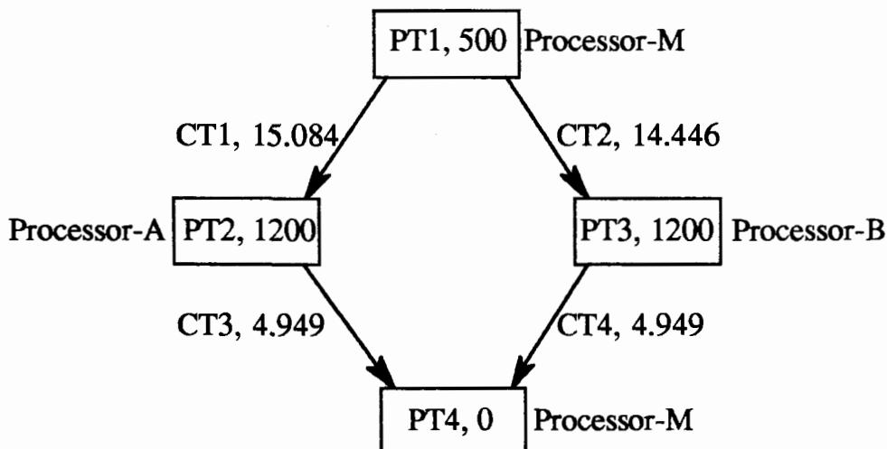
Figure 3: Task graph for three processors
