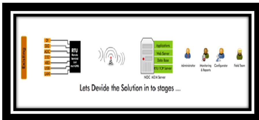
Figure 7.5: Existing M2M setup
