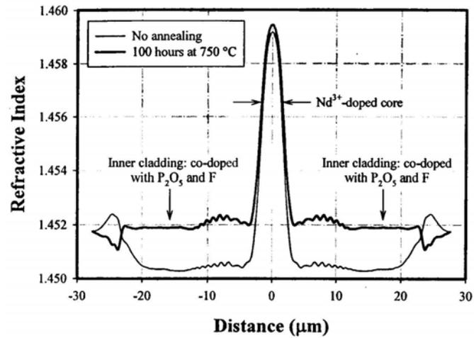
Figure 2.4.5 Refractive index profiles of the core of neodymium doped fibre, before and after annealing as detailed by Sidiroglou *et al* [2003].
