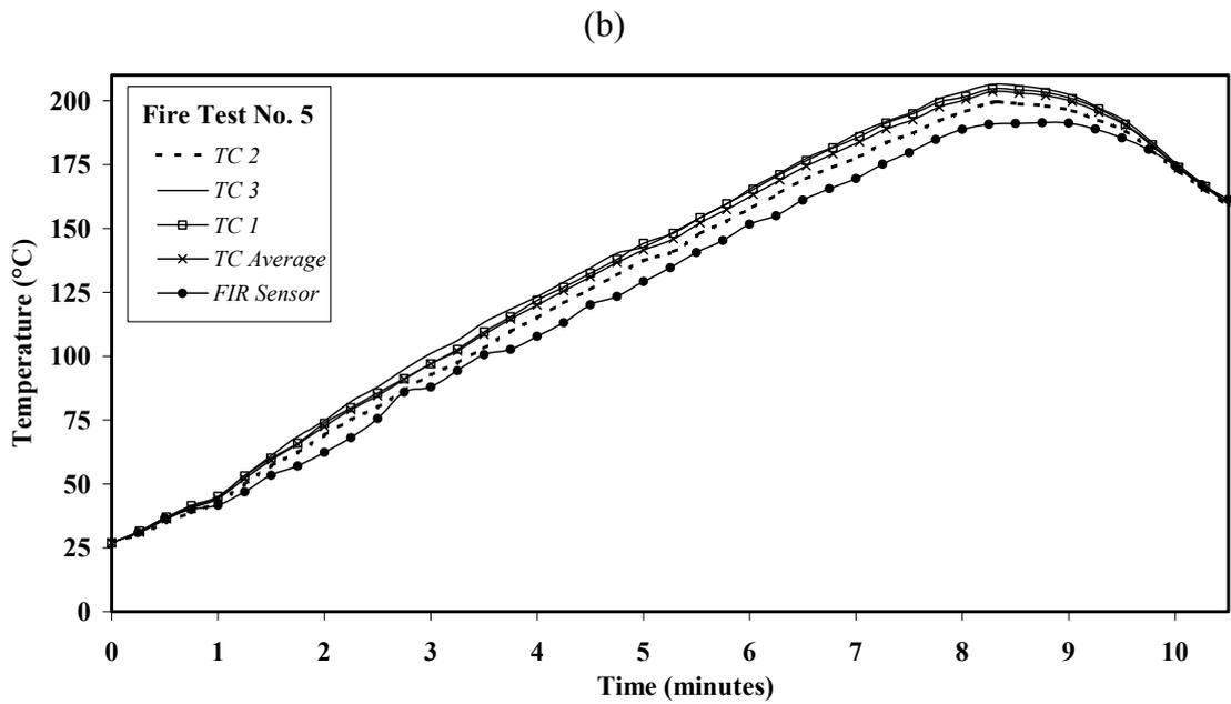
Figure 4.4.3 Measurement of large windowpanes (600 mm x 600 mm) with the FIR sensor and thermocouples during fire simulation tests 4 and 5, shown by (a) and (b) respectively. (TC = thermocouple.)
