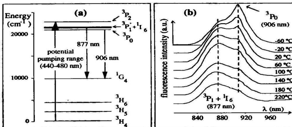
Figure 2.4.2 (a) Simplified energy scheme of  $Pr^{3+}$  in ZBLAN (b) Emission of the  $^3P_0$  and ( $^3P_1 + ^1I_6$ ) levels at the shown temperatures [Maurice *et al*, 1997a].
