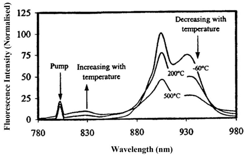
Figure 3.3.2 Fluorescence spectra at different temperatures measured by the temperature sensor used in the fire research. (The spectra were normalised to the peak fluorescence intensity at  $-60\text{ }^{\circ}\text{C}$ .) [Wade *et al*, 1999].
