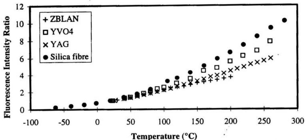
Figure 3.3.1 Normalised fluorescence intensity ratio values with respect to temperature for neodymium in various samples. (FIR values were normalised by taking the quotient of the FIR at each temperature and the FIR at room temperature.) [Wade *et al*, 1998].
