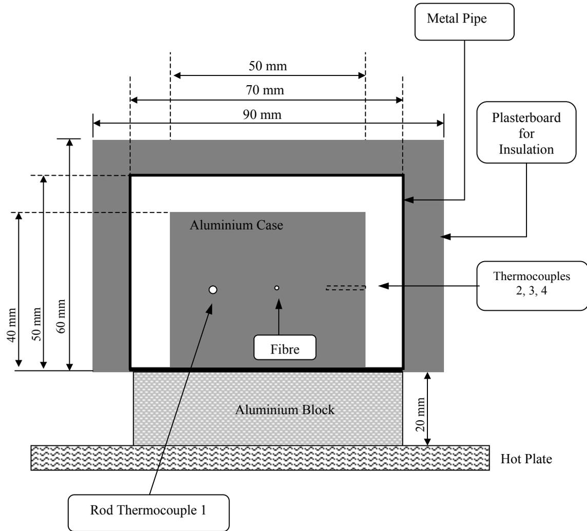
**Figure 4.2.4 Front cross-sectional view of the fibre housing on the hot plate for temperature calibration of the fluorescence intensity ratio sensor.**
