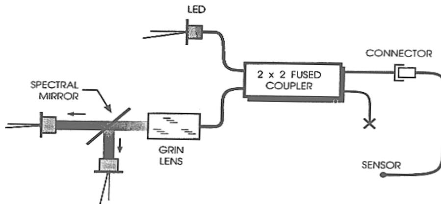
Figure 1.2.5 A Fabry-Perot interferometric sensor [Saaski and Hartl, 1992].
