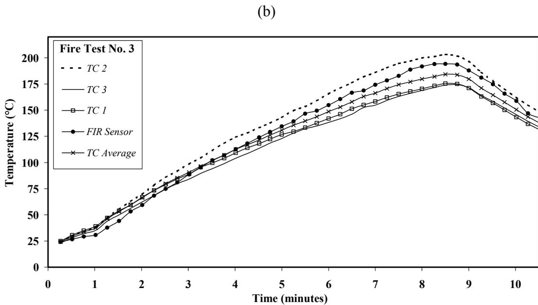
Figure 4.4.2 Measurement of small window glass (300 mm x 300 mm) temperature using the FIR sensor and thermocouples during fire simulation tests 2 and 3, shown by (a) and (b) respectively. (TC = thermocouple.)
