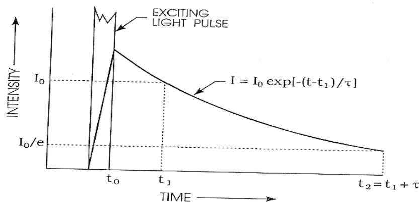
Figure 1.2.3 The two-point constant measurement is one technique used to measure fluorescence decay [Wickersheim and Sun, 1987].
