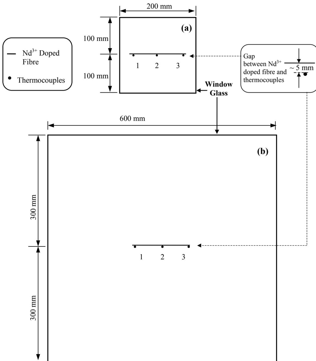
Figure 4.4.1 The placement of thermocouples (denoted by 1, 2 and 3) and neodymium doped fibre of length 150 mm attached to the centre of (a) the small windows (used in the fire simulation tests 2 and 3) and (b) the larger window as used in tests 4 and 6. Similar configurations were used for different lengths of doped fibre used in other fire simulations (see Table 4.4.1).
