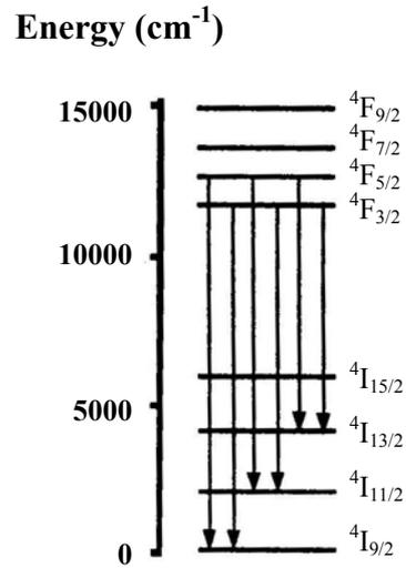
**Figure 3.2.1** Energy level diagram of neodymium ions showing the energy levels and pairs of fluorescence transitions from excited state levels as reported by Wade *et al* [2003].
