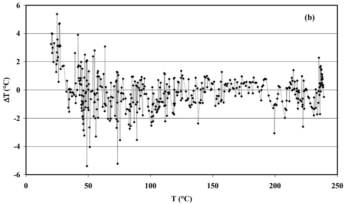
Figure 4.2.6 (a) a typical calibration result of the neodymium doped temperature sensor. (Doped-fibre length is 150 mm). The circles represent the variation of the FIR at the indicated temperatures. This data was fitted with a fourth order polynomial (solid line) and (b) the temperature differences between the experimental data and fourth order polynomial fit. (The lines joining the points are for an aesthetic purpose only.)
