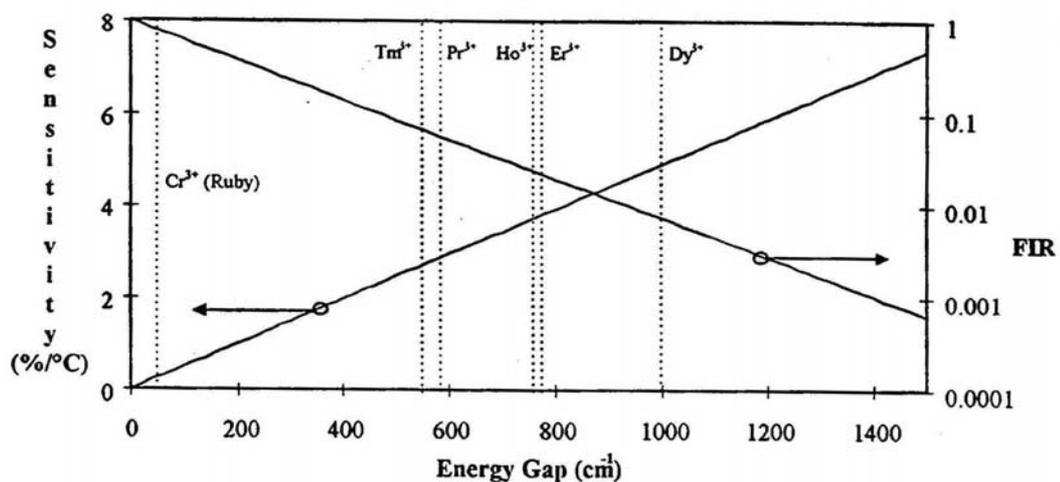
Figure 2.2.2 The change in FIR and sensitivity with respect to the energy gap between the two thermalising levels at room temperature for several rare earth ions [Baxter *et al*, 1996].
