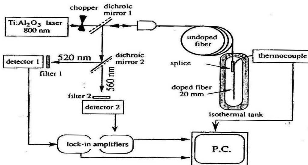
**Figure 2.4.1 Schematic of the FIR experimental sensor arrangement of Maurice *et al* [1995].**
