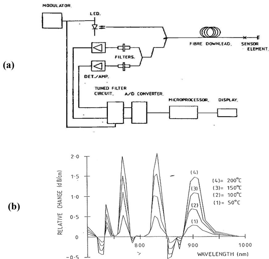
Figure 1.2.2 (a) Schematic diagram of the sensor system (b) The change in absorption with respect to temperature (relative to 20°C) by Appleyard *et al* [1990].
