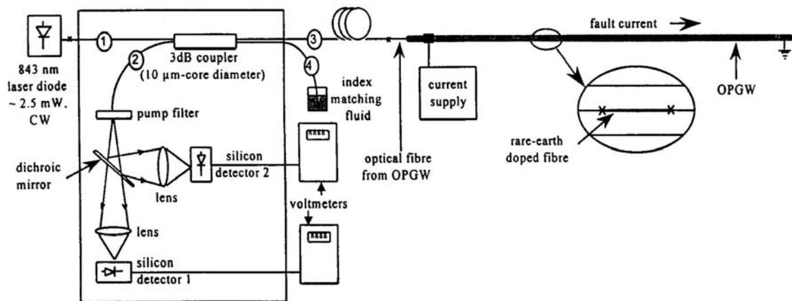
Figure 2.6.1 Experimental arrangement used to measure the thermal response of OPGW cables [Wade *et al*, 1996].
