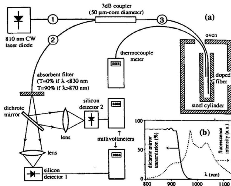
Figure 2.4.3 Ytterbium doped fibre temperature sensor reported by Maurice *et al* [1997].
