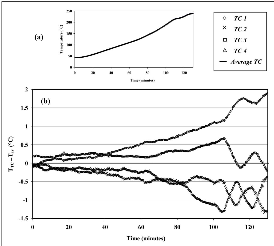
Figure 4.2.5 (a) Typical temperature measurements from the four thermocouples and their average temperature with respect to time and (b) for each thermocouple, the difference between the temperature and the average temperature of the thermocouples, as a function of time. These temperatures were recorded during a calibration of the sensor using the experimental arrangement shown in Figure 4.2.4. (TC = thermocouple.)
