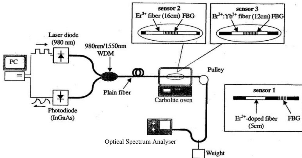
**Figure 1.3.1** Experimental arrangement used for the calibration of the dual temperature and strain sensors. The doped fibre and the fibre Bragg grating (FBG) configurations are shown. Sensor 1 is that used by Wade *et al* [2001a]. Sensors 2 and 3 are those used by Forsyth *et al* [2002].
