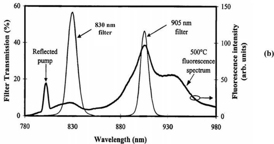
Figure 4.2.1 A variation of the prototype sensor used in the investigation of window glass breakage is shown by (a) the neodymium doped fibre sensor based on the fluorescence intensity ratio technique [Wade *et al*, 1999], and (b)  $\text{Nd}^{3+}$  fluorescence spectrum at 500 °C and the transmission spectra of the dichroic filters [Wade, 1999].
