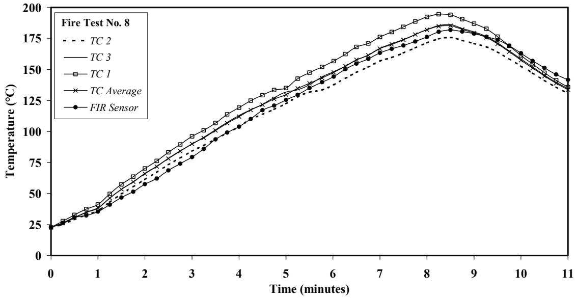
Figure 4.4.5 Measurement of large window glass (600 mm x 600 mm) temperature using the F/R sensor and thermocouples during fire simulation test 8. (TC = thermocouple.)
