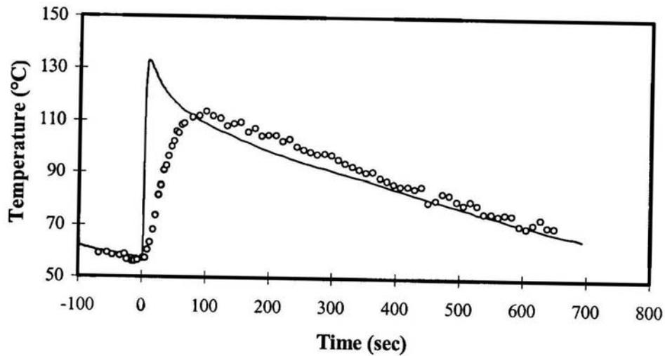
Figure 2.6.2 Optical fibre temperature (depicted by the circles) and OPGW cable temperature (solid line) during OPGW fault current test [Wade *et al*, 2003].
