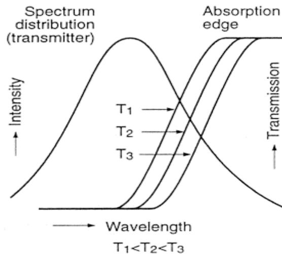
**Figure 1.2.1** Semiconductor transmission as a function of wavelength and temperature [Kyuma *et al*, 1982].
