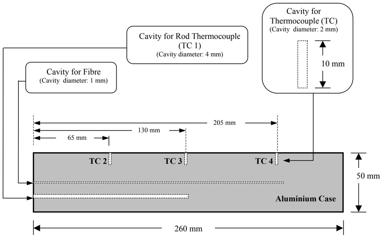
**Figure 4.2.3** Cross section of the aluminium case used to heat the neodymium sensor probe and thermocouples, as viewed from the top.
