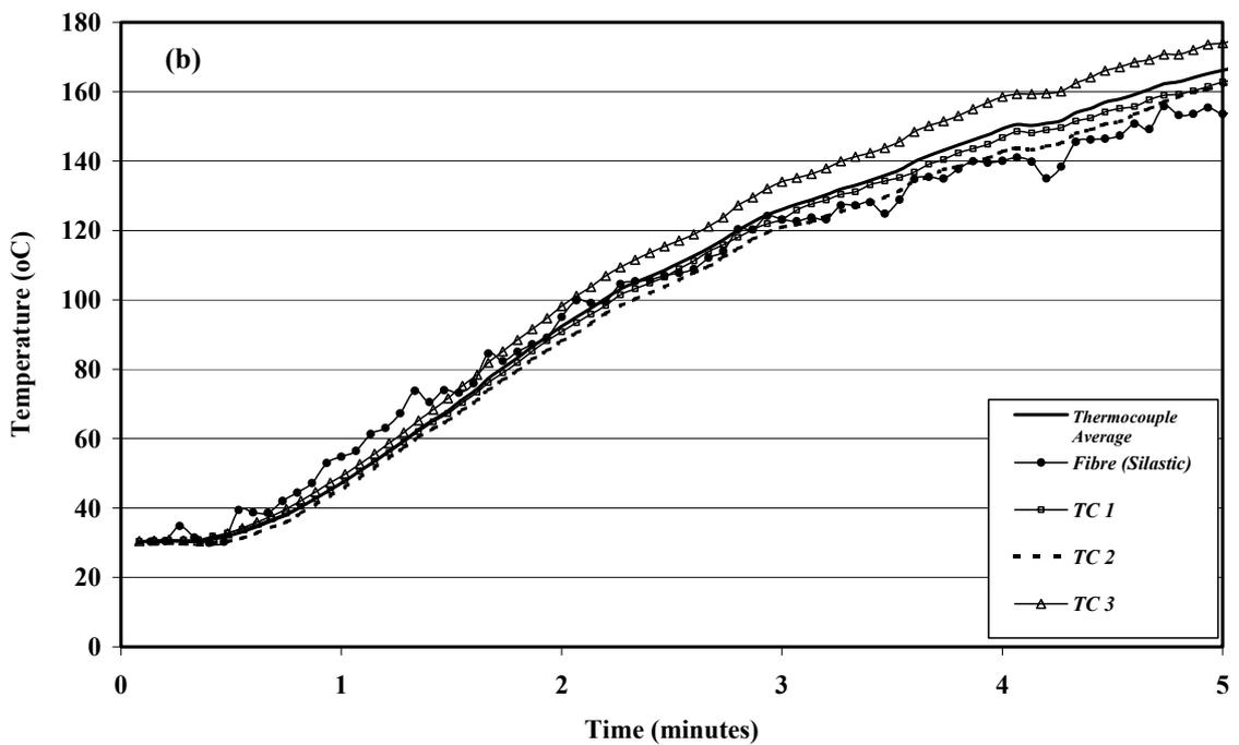
Figure 4.3.3 Performance of fluorescence intensity ratio sensor, with the probe coated in an adhesive. The results are for the fibre probe coated in *KS Bond* super glue shown in (a), and the fibre probe coated in *Silastic* silicon rubber shown in (b). (TC = thermocouple.)
