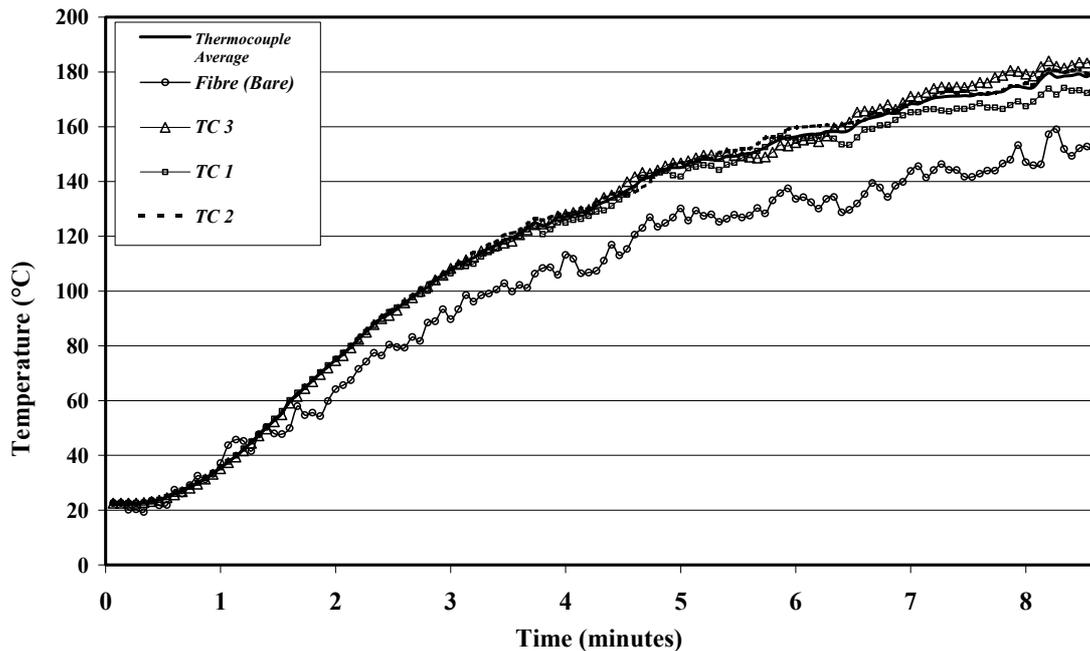
**Figure 4.3.2 Comparison of thermocouples and fluorescence intensity ratio sensor exposed to radiant heat in a bench scale test. The neodymium doped fibre probe was bare. (TC = thermocouple.)**
