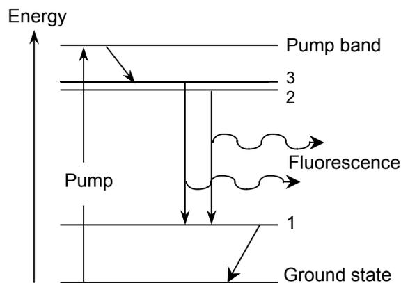
**Figure 2.2.1** Simplified energy level diagram for a generic rare earth ion showing fluorescence properties [Baxter *et al*, 1996].
