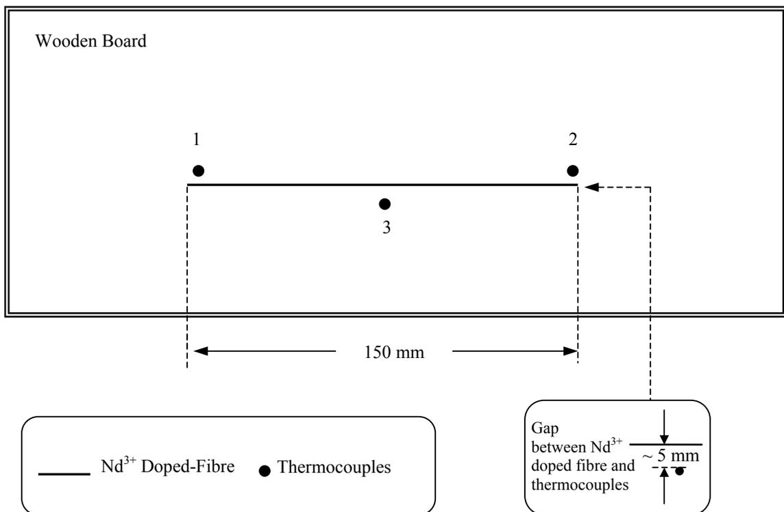
**Figure 4.3.1** Set-up of neodymium doped fibre and thermocouples for the small scale radiant heat tests. (Diagram is not to scale.)
