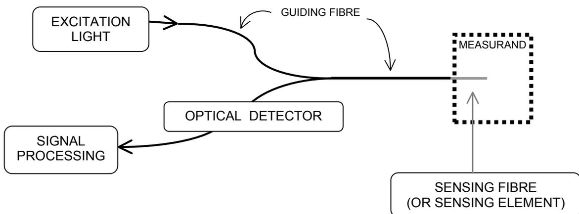
Figure 1.1.1 the basic operation of an optical fibre sensor system.
