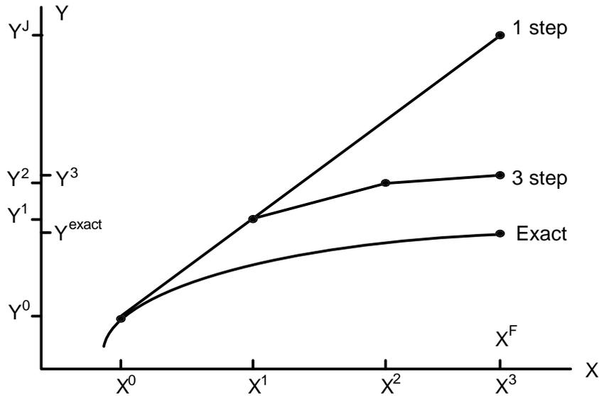
**Figure 3. Multistep process to reduce linearisation error**
