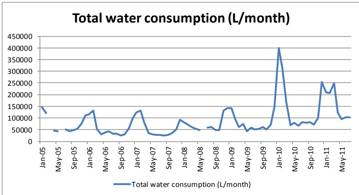
From this data it is possible to calculate the water consumption and therefore wastewater production per person per day. – see below.
