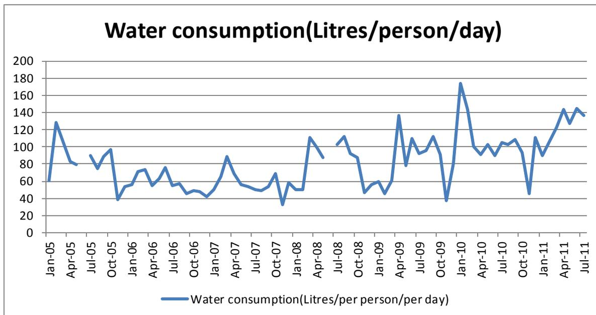
From this it is possible to see a steady increase in personal use over time. This is largely due to improved availability of potable water and relaxed restriction as a result. Based on this data, a design figure of 150 L/person/day should be used. It is expected that water use will be restricted at this level into the future.
