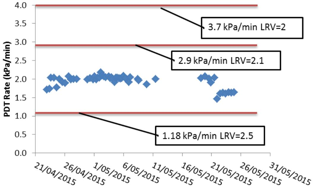
**Figure 18:** RO system PDT results.
