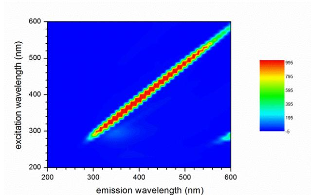
**Figure 23:** Fluorescence Excitation Emission Matrix for RO permeate (4/2/15).
