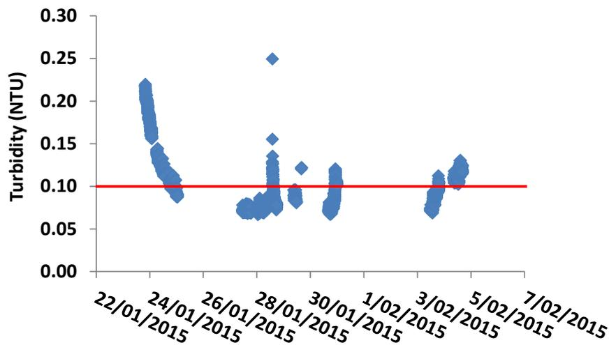
Figure 12: On-line turbidity values for the ceramic MF filtrate after the turbidity sampling point was moved to the BAC launder.
