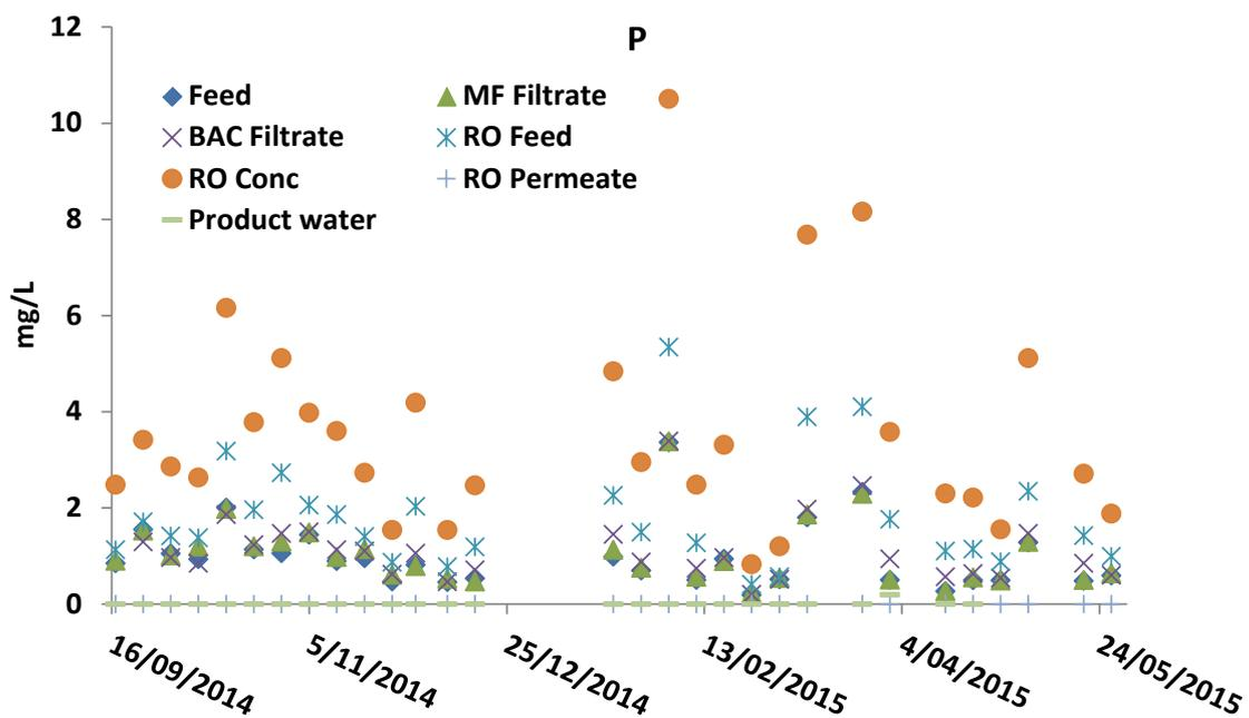
Figure B7 Phosphorus concentrations in the feed and following each treatment unit
