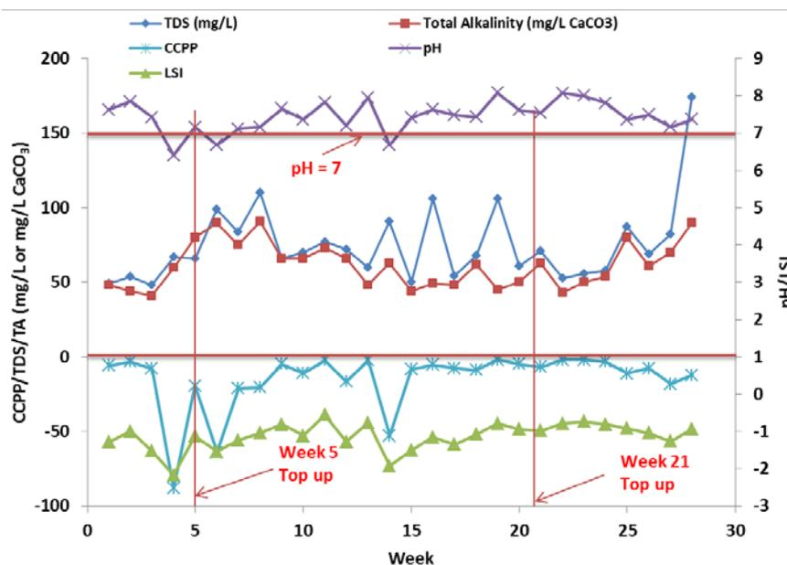
**Figure 25:** CCPP, LSI, pH, TDS and alkalinity of the product water.
