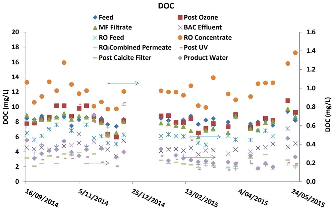
Figure B1b DOC concentrations in the feed and following each treatment unit (Linear scale)
