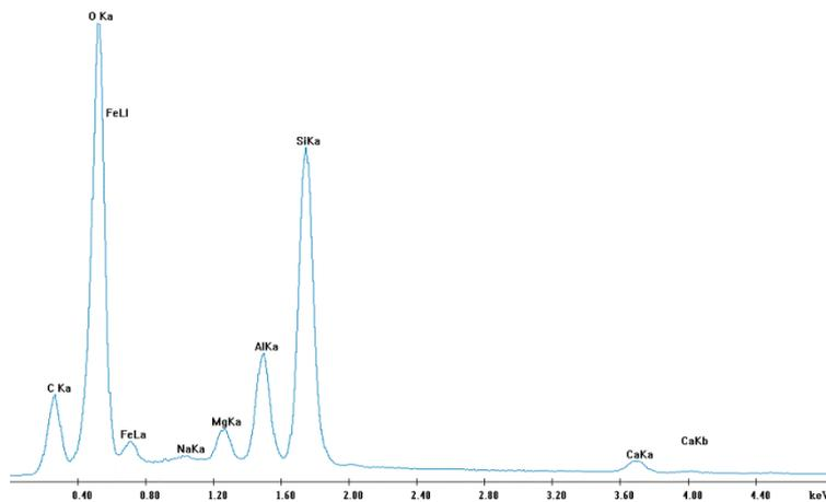
Figure D3. EDS for the non-dissolvable inorganic matter on the filter
