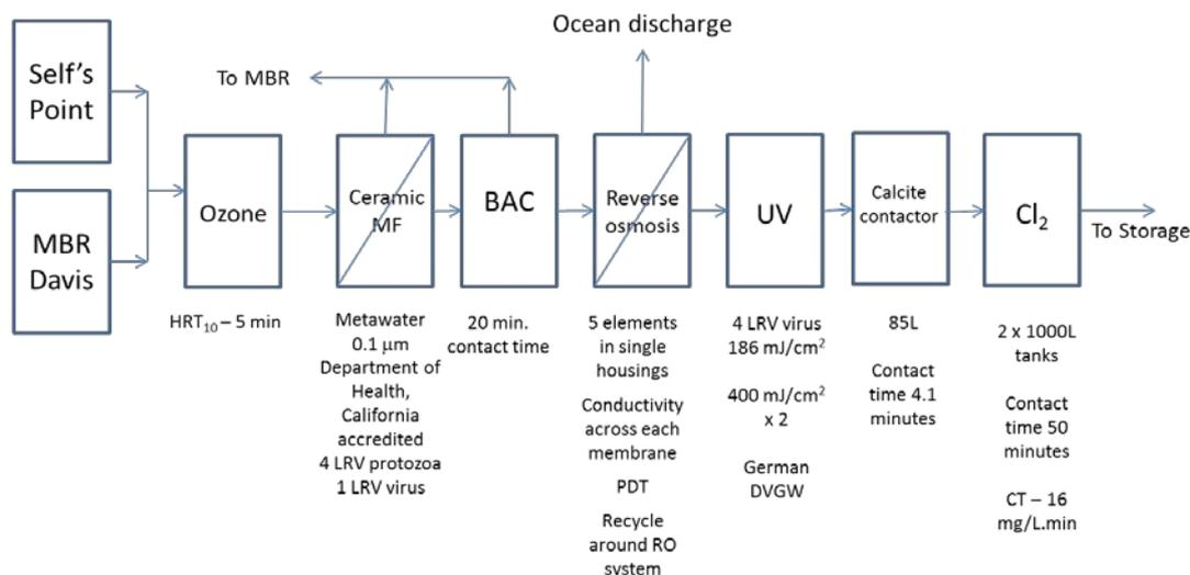
**Figure 2:** Schematic diagram of the AWTP Flowsheet.
