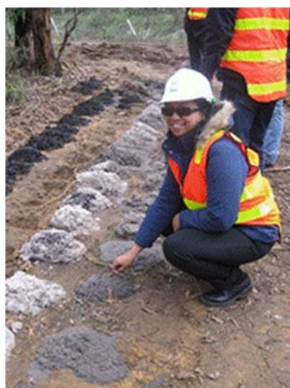
Figure 14 Dr Rinin Erinawati inspecting aquifer samples collecting during drilling (Photo: Gwynn Hatton, Barwon Water).
