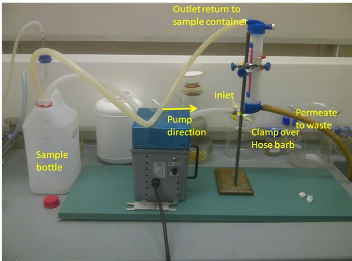
Figure C-10-2. Effluent sample concentration setup using Hemoflow FX80 dialysis filters.
