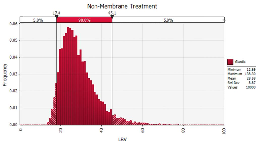
Figure 90 Combined multiple barrier Giardia LRV for a sand filtration-ozone-UV-chlorination treatment train.
