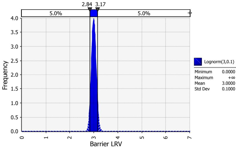
Figure 80. LRV for a single barrier with  $\mu=3$ ,  $s.d.=0.1$
