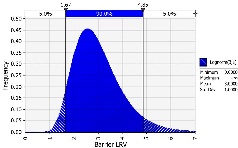
Figure 82. LRV for a single barrier with  $\mu=3$ , s.d=1
