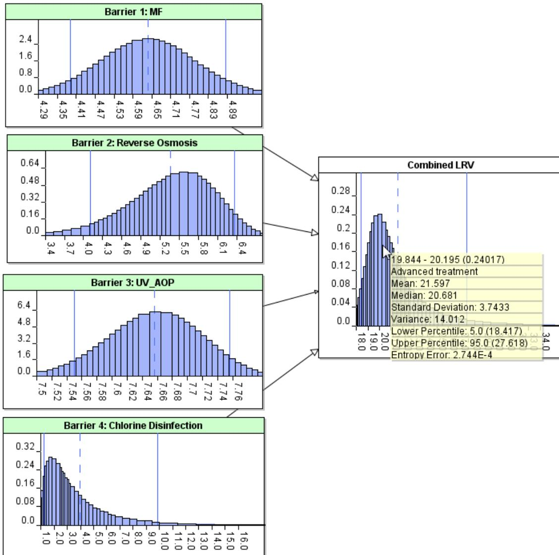
Figure 91 Combined multiple barrier Giardia LRV for a MF-RO-UV/AOP-CI treatment train modelled as a BN
