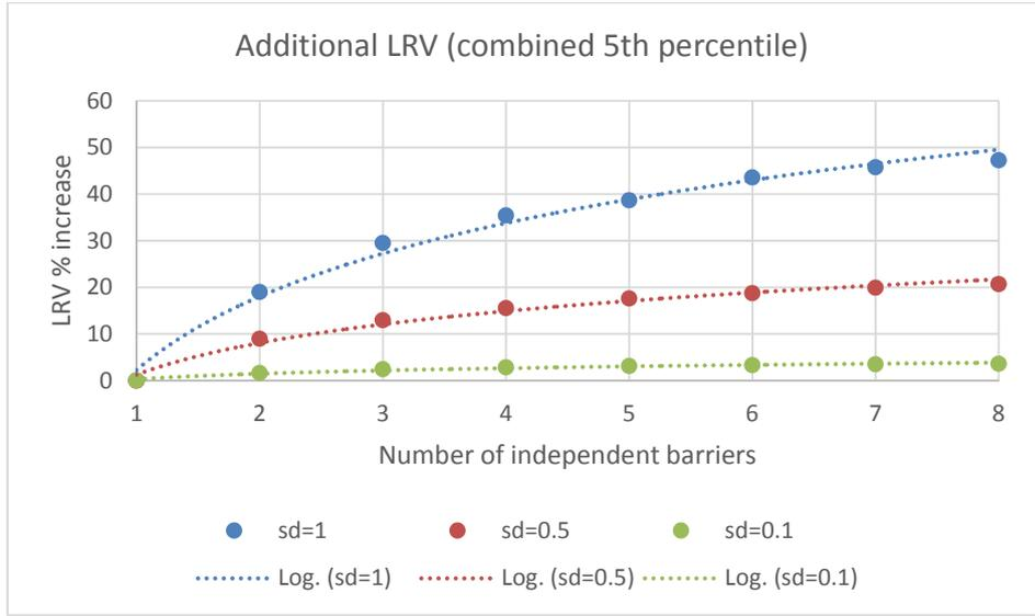
**Figure 88. Relative increase in attributable LRV for a combined multiple barrier 5<sup>th</sup> percentile, compared to summed individual barrier 5<sup>th</sup> percentiles.**
