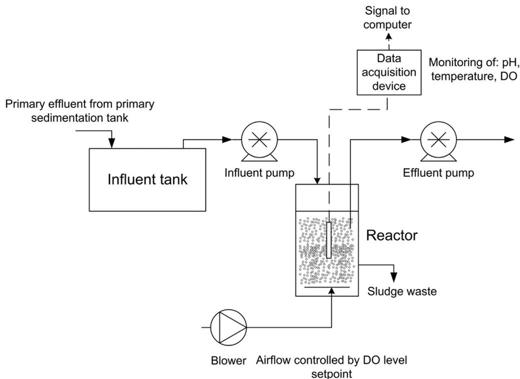
Fig. 2. Scheme of the activated sludge reactor.
