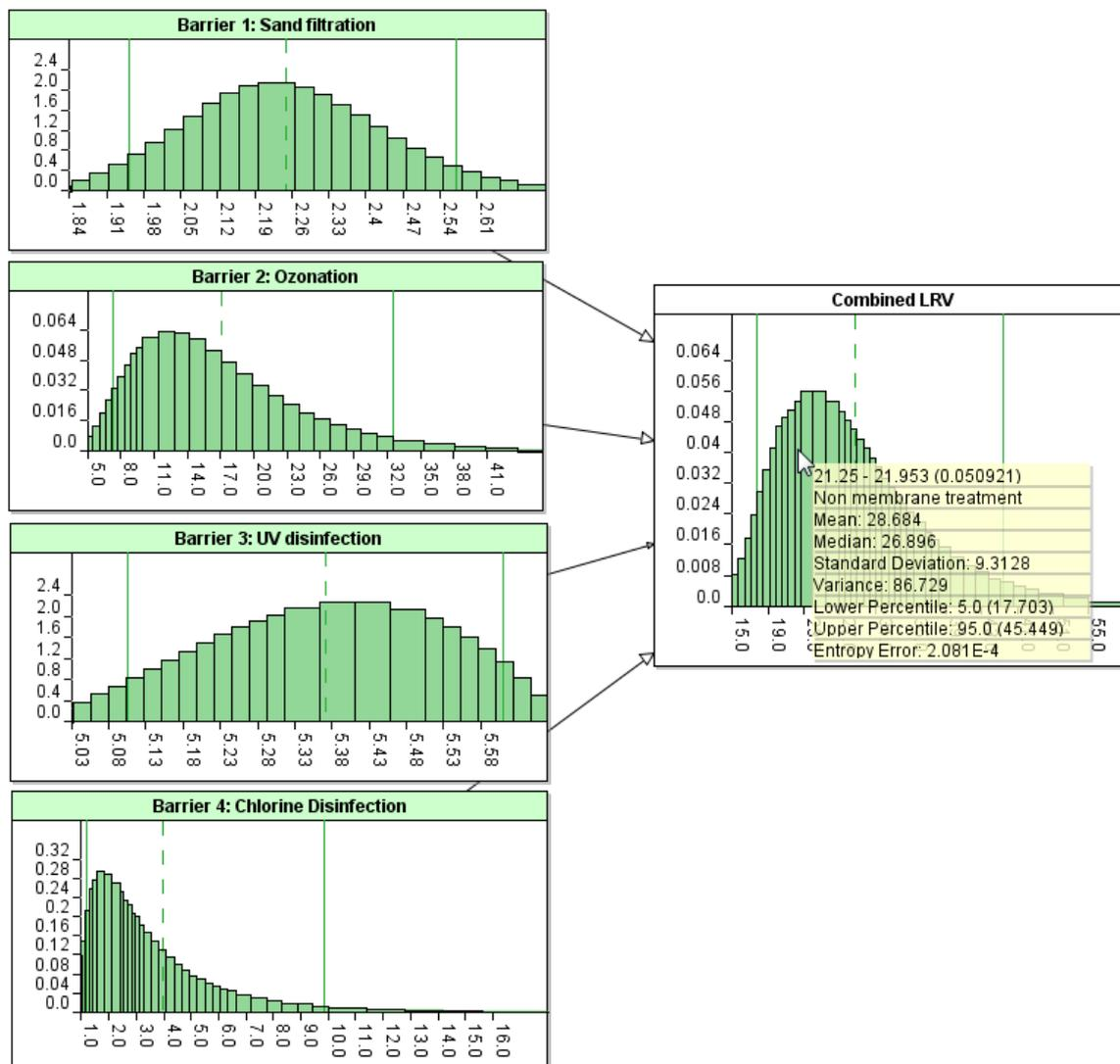
Figure 92 Combined multiple barrier Giardia LRV for a sand filtration-ozone-UV-chlorination treatment train modelled as a BN.
