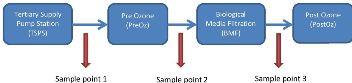
**Figure 31. Front end of Eastern Treatment Plant water recycling system showing the locations of sampling points SP1, SP2 and SP3**
