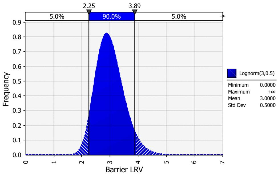
Figure 81. LRV for a single barrier with  $\mu=3$ ,  $s.d.=0.5$
