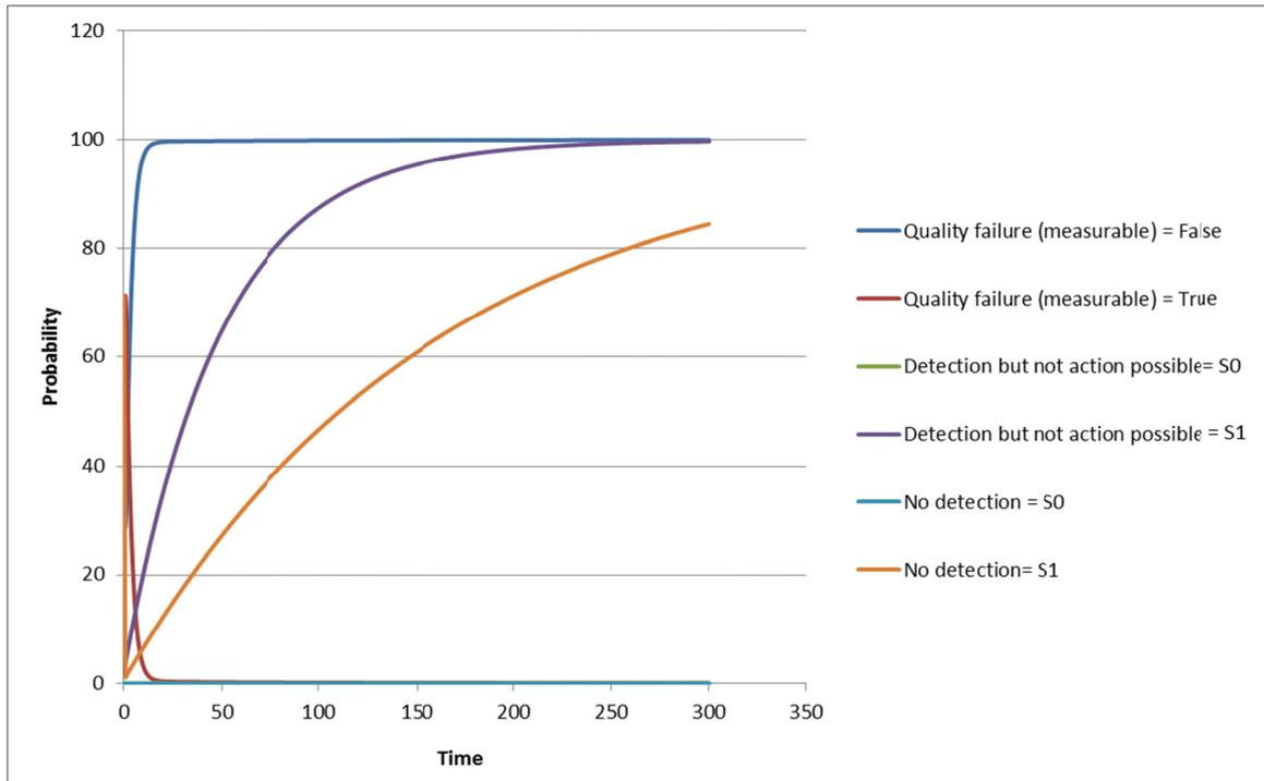
**Figure 76: temporal graph of quality failure event and sub events. S0 indicates the state in which the system is in failure mode and S1 in working condition without the use of back-up.**
