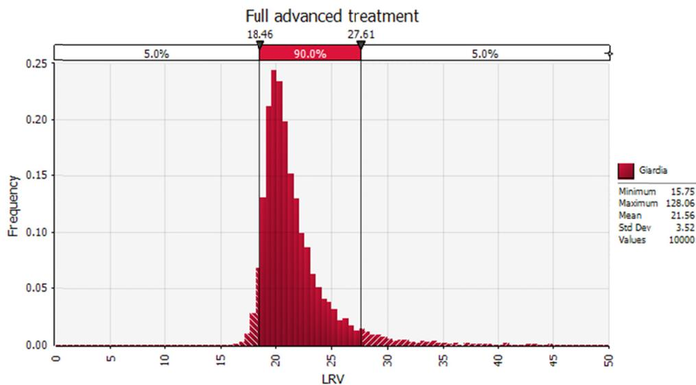
Figure 89 Combined multiple barrier Giardia LRV for a MF-RO-UV/AOP-CI treatment train.
