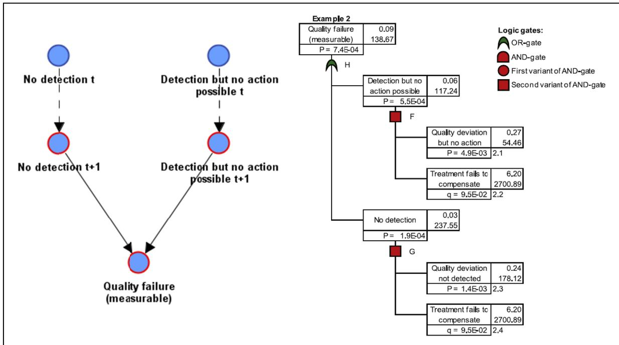
Figure 74: Dynamic Bayesian network model (left) and fault tree analysis (right) for example 1
