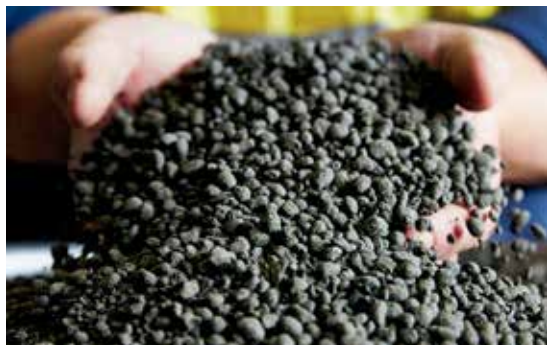
Figure 8 Bioprill® product from the Barwon Water plant.
