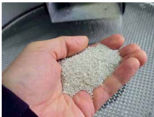
Figure 7 Struvite product from the Clean Water Services Plant in Oregon, USA.
