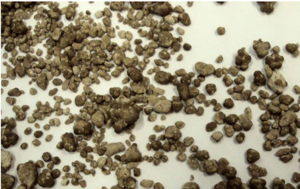
Figure 10. Photos of recovered solid (a) after drying to 45 wt% solids, (b) after granulation at 43 wt% solids.
