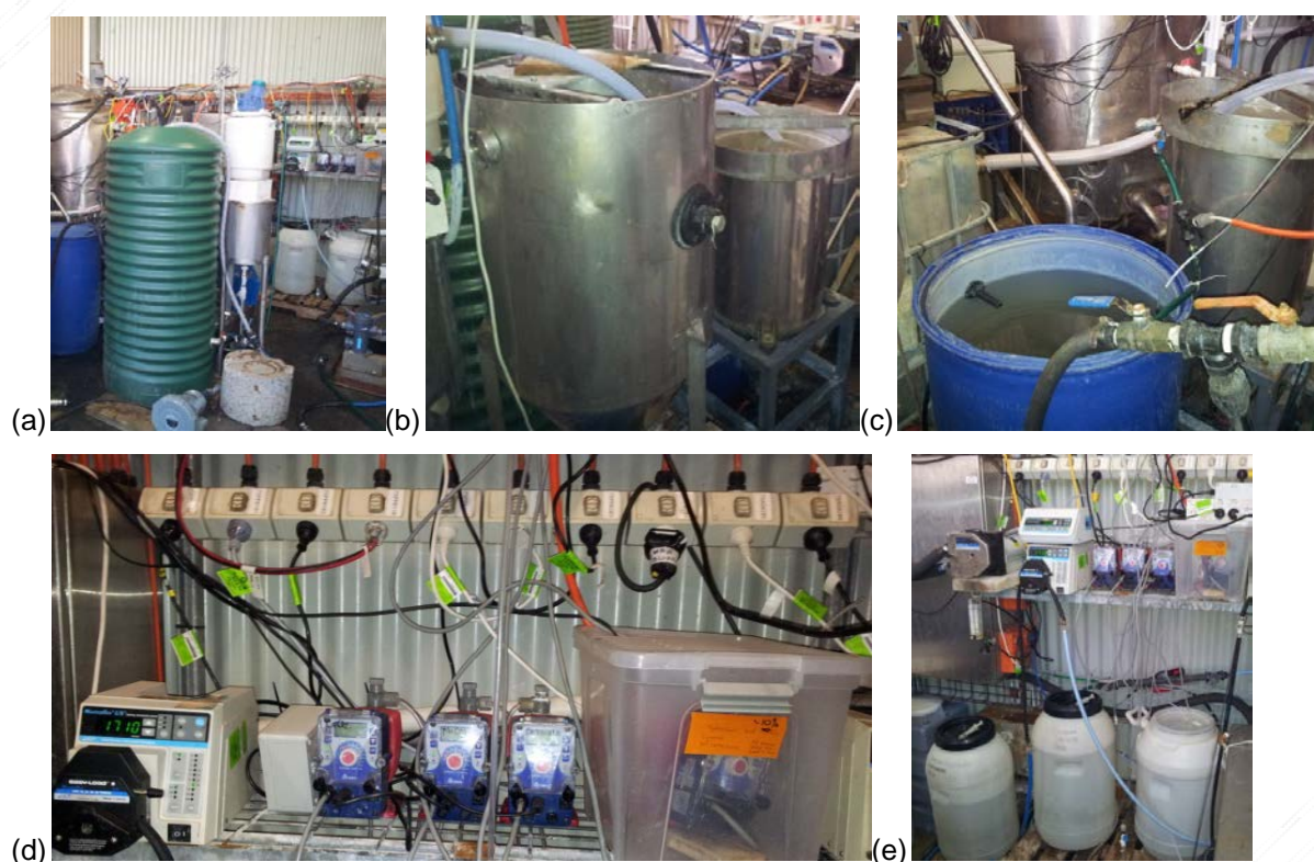
Figure 3. Photos of P and Ca removal pilot setup. (a) general setup showing green upright tank for CO 2 removal with blower at base, mixing tank centre-top, and chemical dosing on far right, (b) Clarifier 1 on left and Clarifier 2 on right, (c) product tank (blue) and clarifier 2 on right, (d) main flow pump on left with four chemical dosing pumps on right, (e) chemical dosing tanks at bottom and pumps above.
