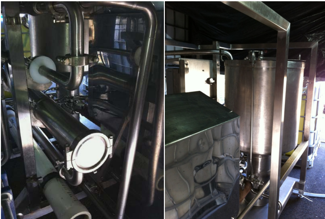
Figure 21. Reverse osmosis pilot plant.
