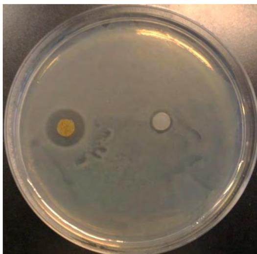
**Figure D-3.** Antimicrobial effect of films against *E. coli* after 24h of incubation at 37°C of (a) PLA film containing 20% w/w thymol and (d) PLA/kenaf film containing 20% w/w thymol and 20% w/w kenaf fibres.
