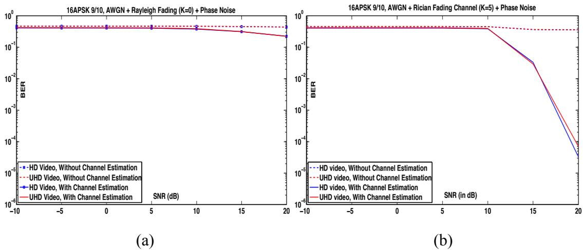
Figure 5.32: BER vs. SNR for 16APSK-9/10 (a) Rayleigh Fading (b) Rician Fading
