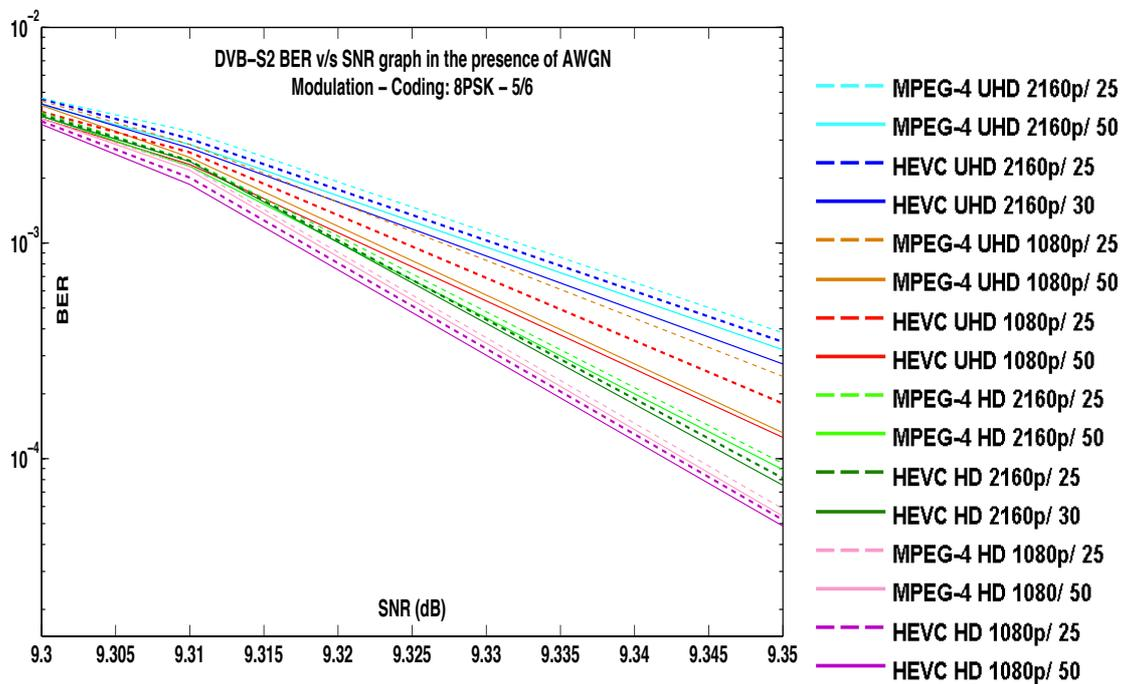
Figure 5.22: Signal performance of different video standards, when transmitted through 8PSK-5/6 in the presence of AWGN
