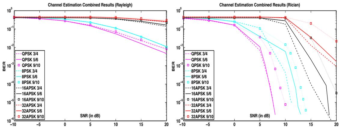
Figure 5.36: Combined results of channel estimation
