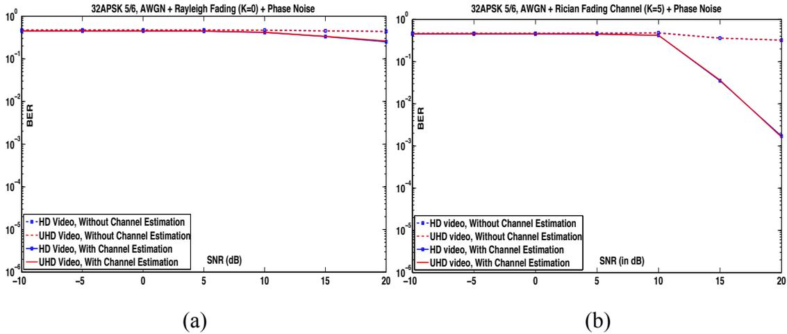
Figure 5.34: BER vs. SNR for 32APSK-5/6 (a) Rayleigh Fading (b) Rician Fading
