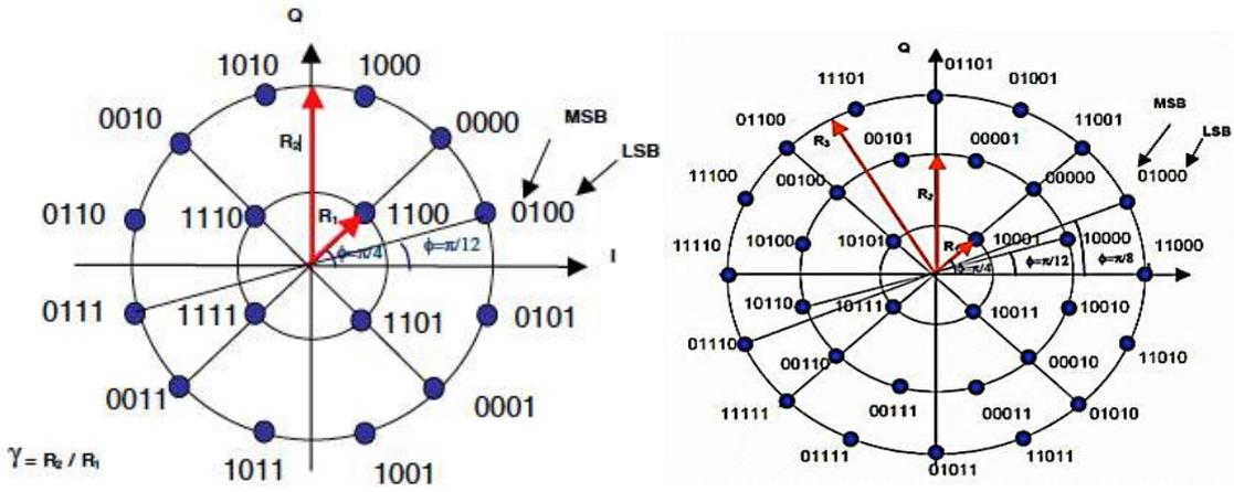
Figure 3.4: Constellation Diagram of 16APSK and 32APSK [25]
