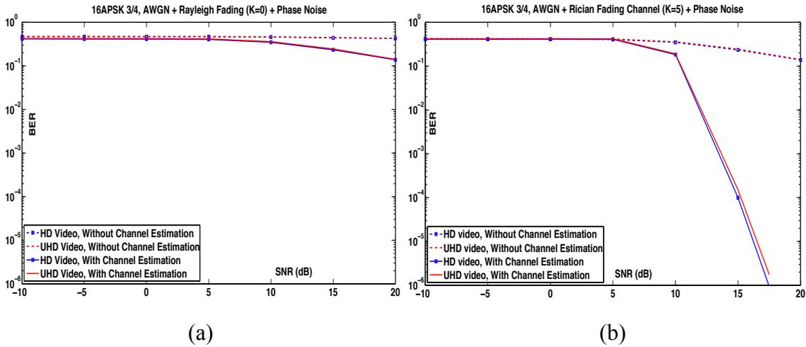
Figure 5.30: BER vs. SNR for 16APSK-3/4 (a) Rayleigh Fading (b) Rician Fading
