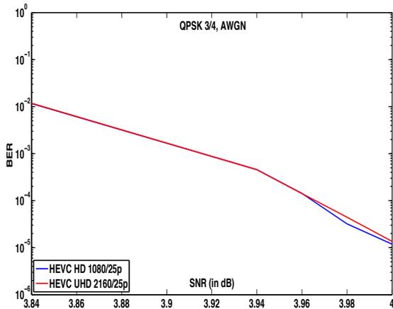
Figure 5.9: BER vs. SNR of UHD and HD for QPSK-3/4, with AWGN
