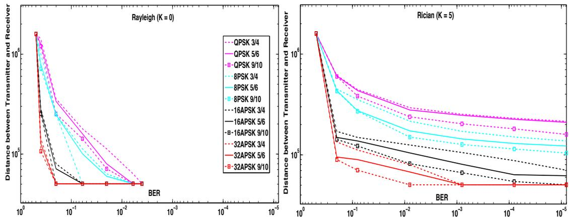
Figure 6.3: Distance between transmitter and receiver vs. BER for Rayleigh and Rician
