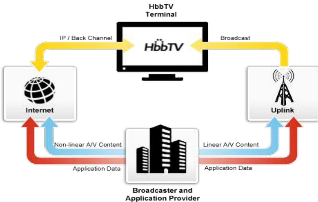
Figure 2.5: Hybrid television system architecture [55]
