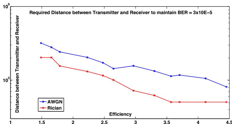
Figure 6.4: Distance between transmitter and receiver vs. Modulation Efficiency graph
