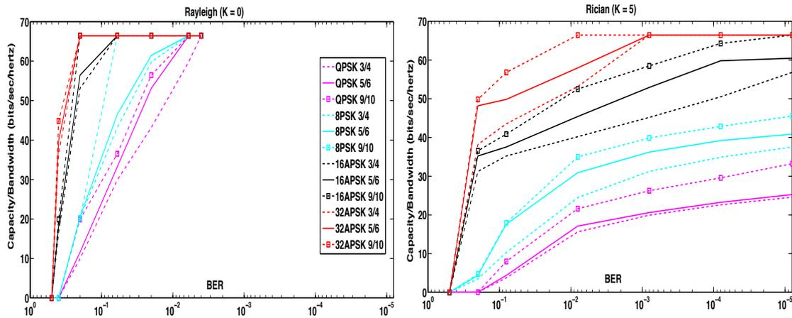
Figure 6.1: Capacity vs. BER graph for Rayleigh and Rician Fading Channel
