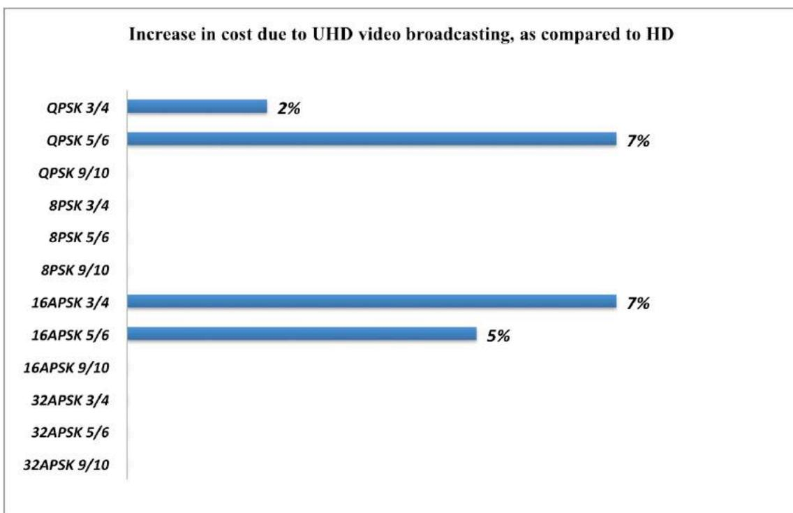
Figure 6.11: Increase in cost due to UHD video broadcasting as compared to HD
