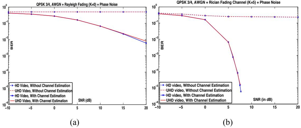
Figure 5.24: BER vs. SNR for QPSK-3/4 (a) Rayleigh Fading (b) Rician Fading
