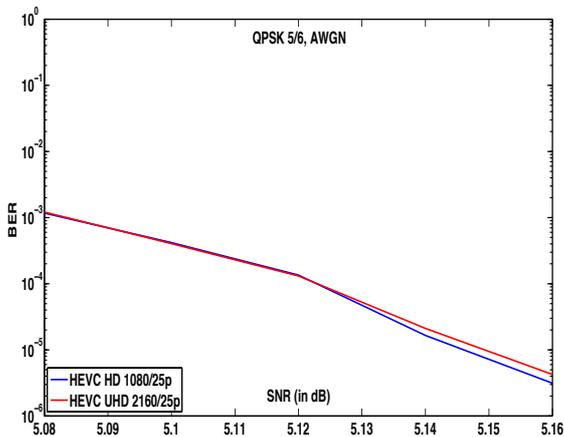
Figure 5.11: BER vs. SNR of UHD and HD for QPSK-5/6, with AWGN
