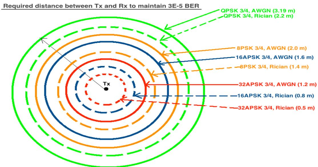
Figure 6.8: MODCOD scheme affecting the transmitter coverage area (apprx depiction)
