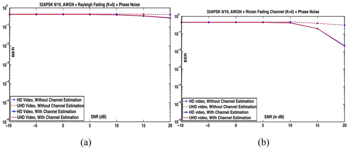
Figure 5.35: BER vs. SNR for 32APSK-9/10 (a) Rayleigh Fading (b) Rician Fading
