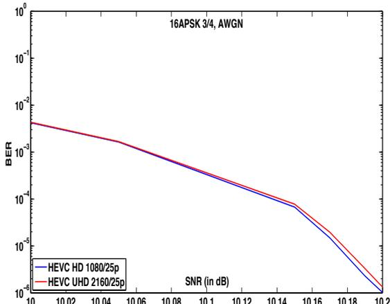
Figure 5.15: BER vs. SNR of UHD and HD for 16APSK-3/4, with AWGN
