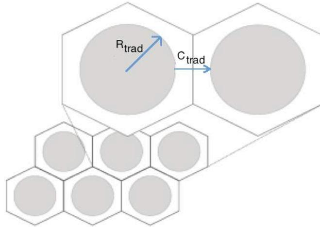
Figure 6.5: Hexagonal packing of co-channel traditional broadcasters [91]
