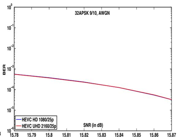
Figure 5.20: BER vs. SNR of UHD and HD for 32APSK-9/10, with of AWGN
