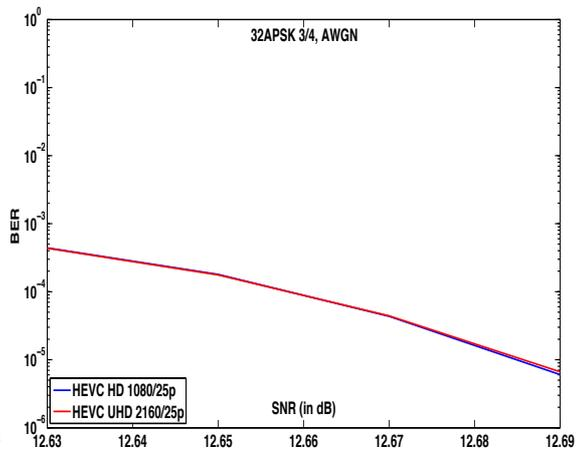
Figure 5.16: BER vs. SNR of UHD and HD for 32APSK-3/4, with AWGN
