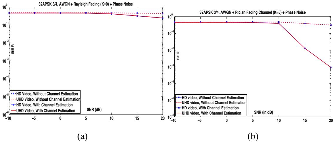
Figure 5.33: BER vs. SNR for 32APSK-3/4 (a) Rayleigh Fading (b) Rician Fading
