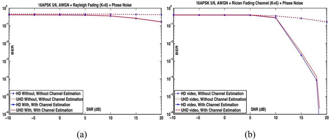
Figure 5.31: BER vs. SNR for 16APSK-5/6 (a) Rayleigh Fading (b) Rician Fading
