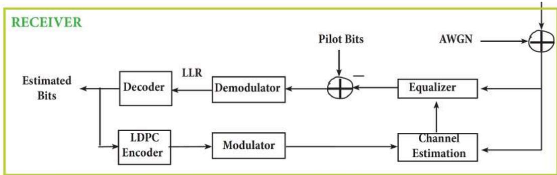
Figure 4.1 Channel Estimation Block Schematic
