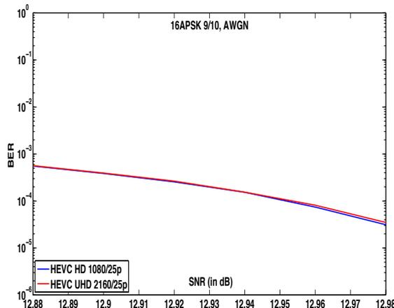
Figure 5.19: BER vs. SNR of UHD and HD for 16APSK-9/10, with of AWGN
