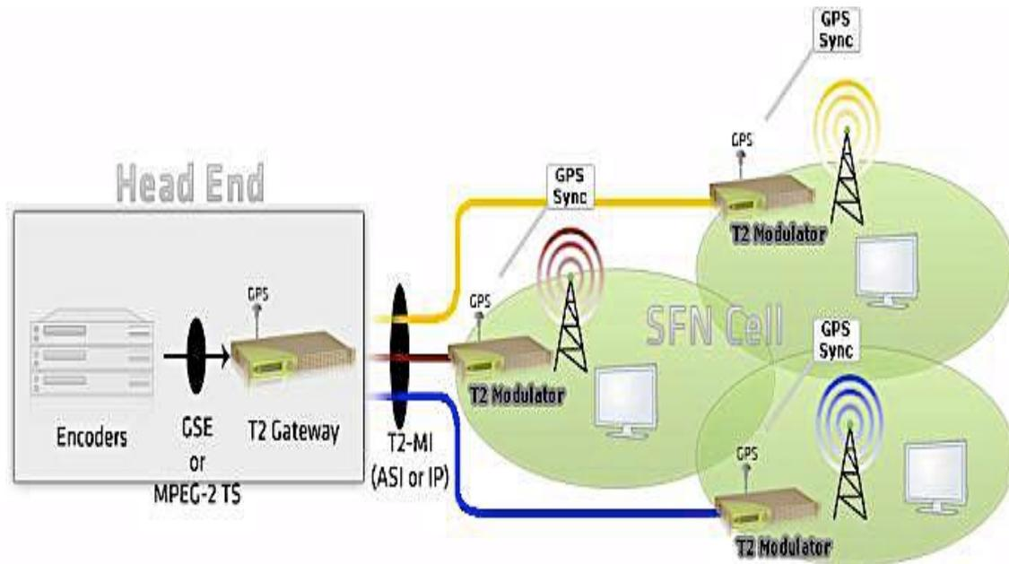
Figure 2.4: DVB-T2 System Architecture [49]
