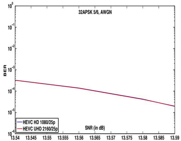
Figure 5.18: BER vs. SNR of UHD and HD for 32APSK-5/6, with AWGN
