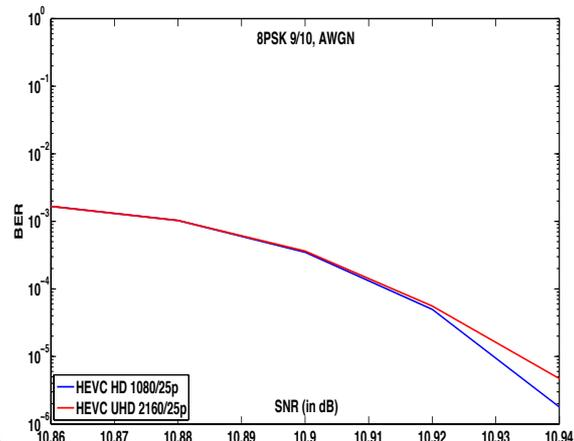
Figure 5.14: BER vs. SNR of UHD and HD for 8PSK-9/10, with AWGN
