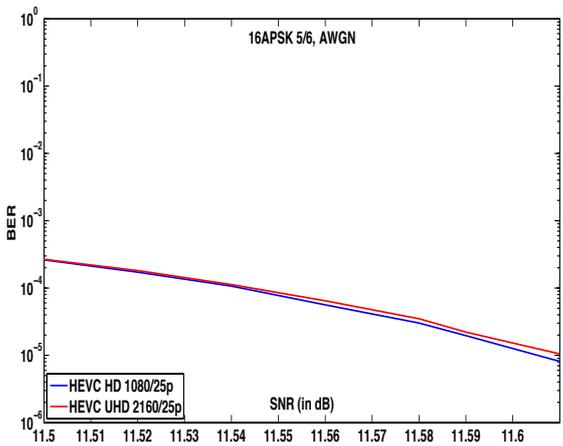
Figure 5.17: BER vs. SNR of UHD and HD for 16APSK-5/6, with AWGN
