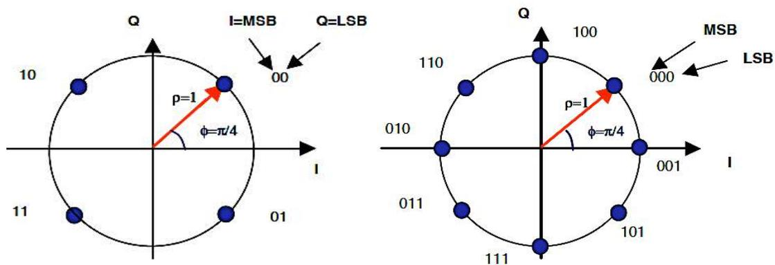
Figure 3.3: Constellation Diagram of QPSK (left) and 8PSK (right) [25]
