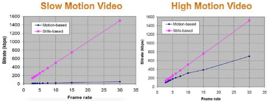
Figure 5.21: Understanding frame rate: For videos (motion based), as frame rate increases, bit rate decreases [85]
