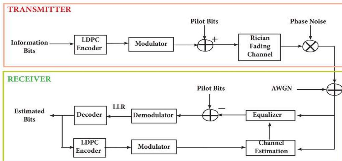
Figure 3.2: DVB-S2 block schematic [46]
