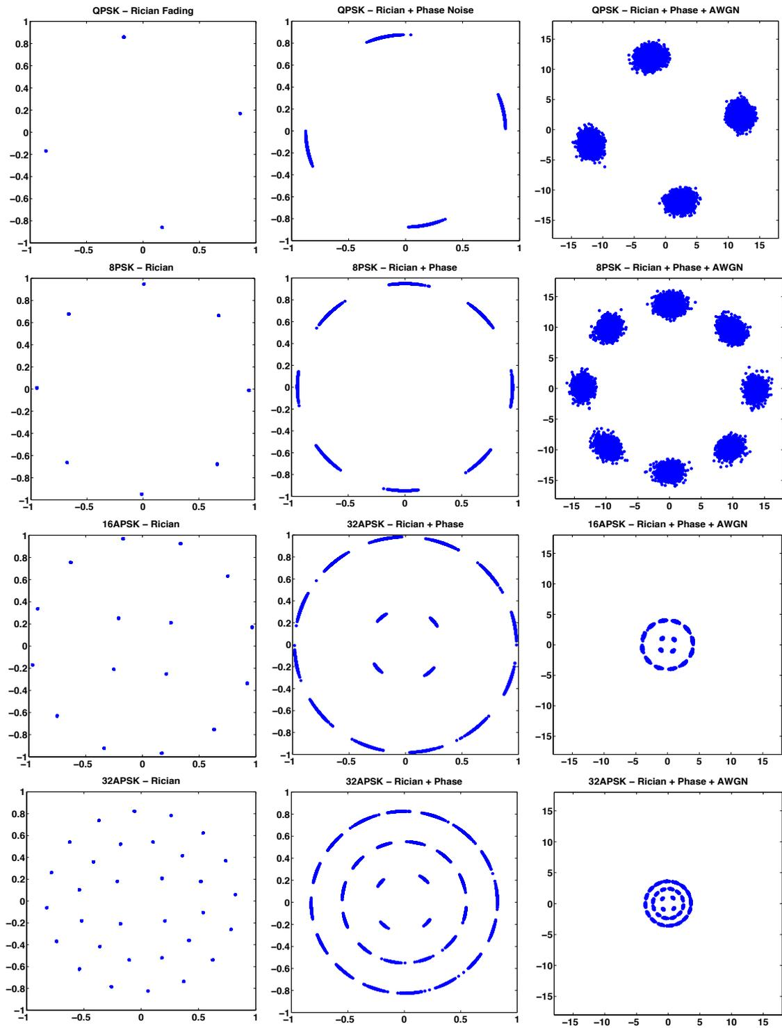
Figure 5.23: Constellation diagrams of different modulation schemes with noise, at SNR=20dB for Rician Fading Channel (K=5)
