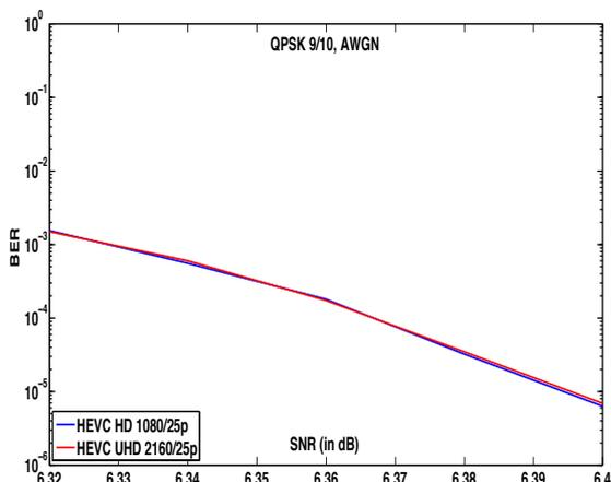
Figure 5.13: BER vs. SNR of UHD and HD for QPSK-9/10, with AWGN
