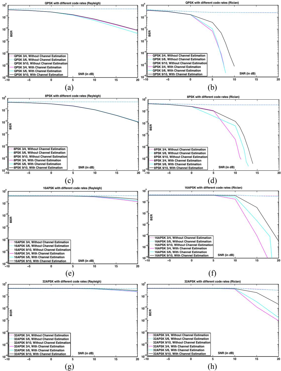
Figure 5.38: Comparison of modulation schemes for different code rates
