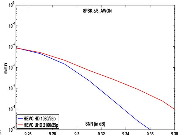
Figure 5.12: BER vs. SNR of UHD and HD for 8PSK-5/6, with AWGN
