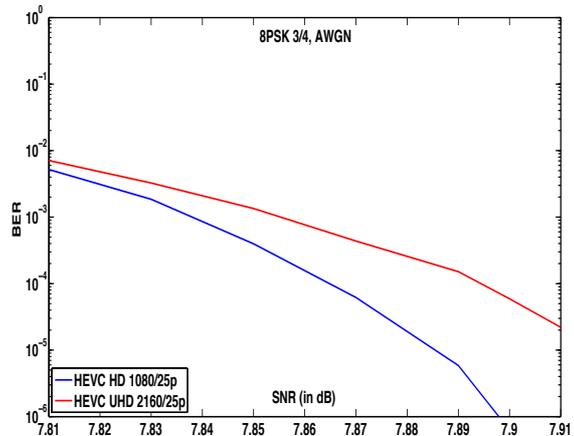
Figure 5.10: BER vs. SNR of UHD and HD for 8PSK-3/4, with AWGN
