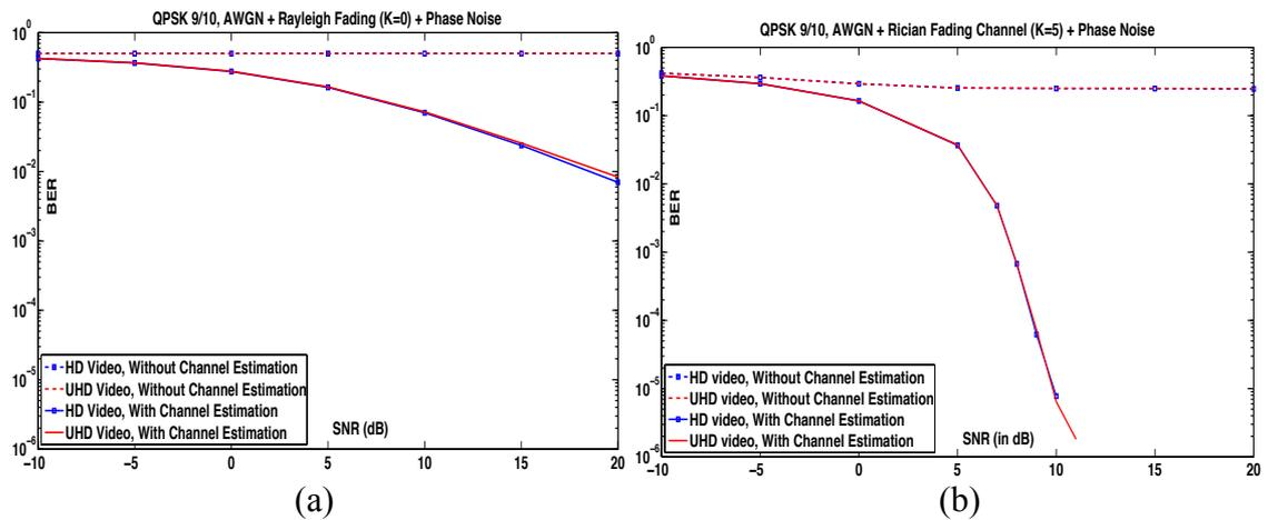
Figure 5.26: BER vs. SNR for QPSK-9/10 (a) Rayleigh Fading (b) Rician Fading
