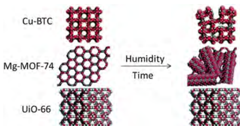
FIGURE 5.4: Cu-BTC, Mg-MOF-74 and UiO-66 structure change after water uptake [129]
