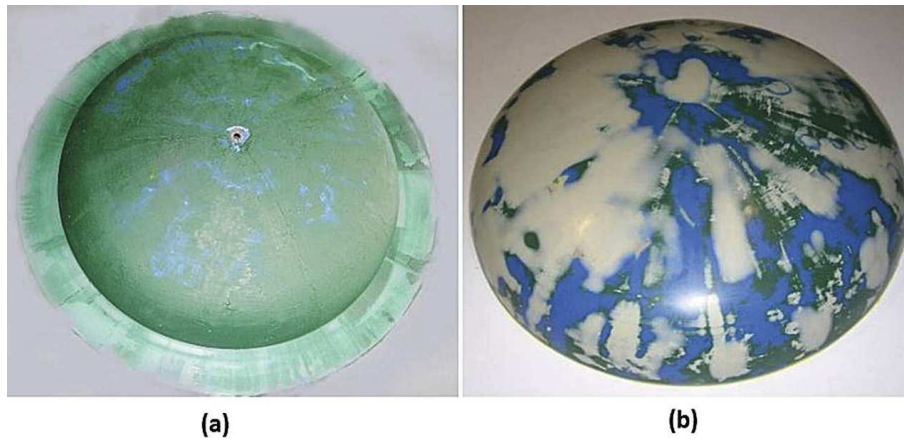
Fig. 7. Elliptical shell pattern made of polyurethane foam. (a) Covered by putty; (b) Polished.
