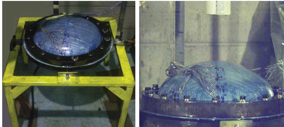
Fig. 12. Schematic of shell's boundary condition and gauge sensors instalment on the second sample.
