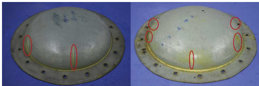
Fig. 14. Observation of failure in the shell's outermost ply ( k = 1 ) at pressure of P_f = 1.7 [MPa] at \varphi = [70-90] .
