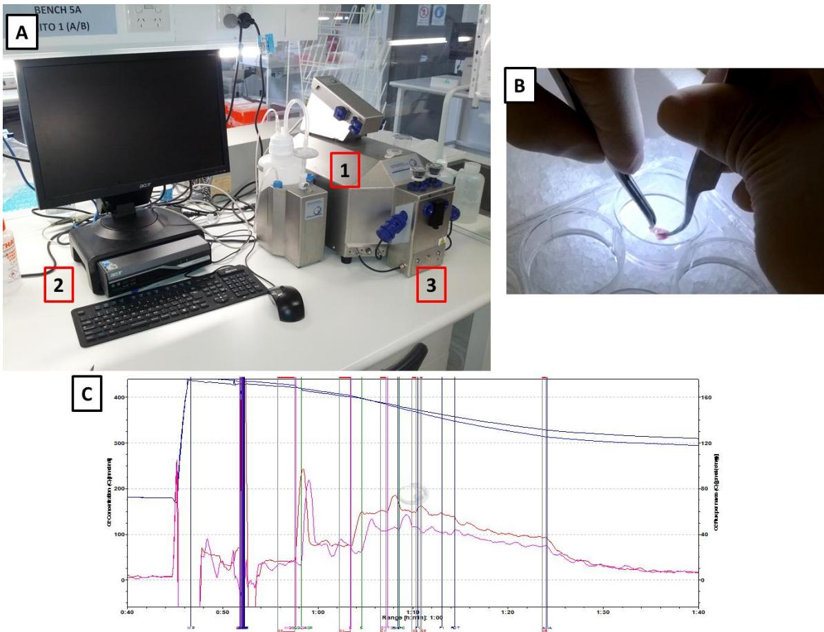
**Figure 2-3. Mitochondrial respiration apparatus, muscle fibre separation and respiration data.** A, Oxygraph-2k (1), computer system with DataLab software v5.1.0.2 (2), and O2k-Fluo LED2-Module (3). B, mechanical separation of muscle fibres, in preparation for permeabilisation procedure. C, Representative data obtained from DataLab software.
