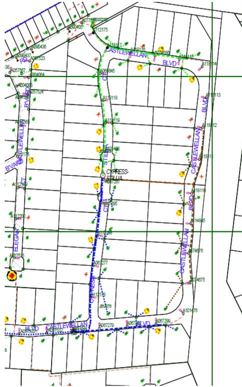
Fig. 5.1. LV Distribution Circuits from Cypress Stillia Distribution Substation
