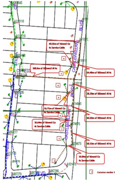
Fig. 5.2. Details of LV Distribution Circuit #4
