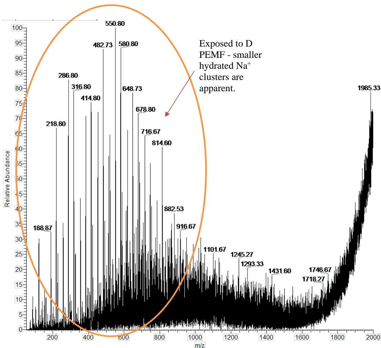
**Figure 5.5:** Electrospray spectrum of Na<sub>2</sub>CO<sub>3</sub> solution exposed to Device D for 10 minutes in positive ion mode. Larger clusters appear to have been broken up by the PEMF, with smaller clusters favoured.
