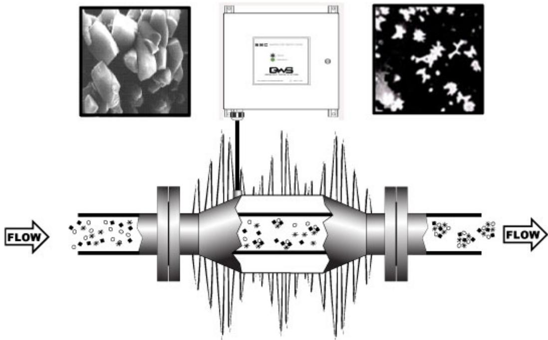
**Figure 3.3:** Schematic of the proposed mechanism of the WAVE™ PEMF device working in scale reduction - as indicated in manufacturer’s documents (Griswold Water Systems 2011).
