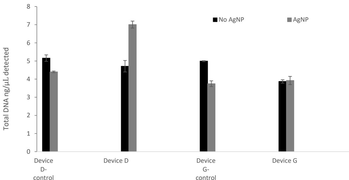
**Figure 4.1:** DNA leakage from *E. coli* cultured in the presence and absence of AgNPs for 1 hour and then exposed to (a) Device D PEMF unit and water bath for 7 hours (b) Device G PEMF unit and water bath for 7 hours; error bars are standard errors for three replicates readings.
