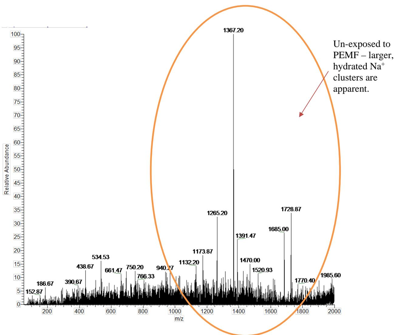
**Figure 5.4:** Electrospray spectrum of un-exposed Na<sub>2</sub>CO<sub>3</sub> solution in positive ion mode.
