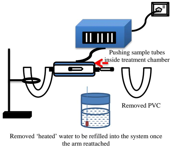
**Figure 3.7:** Placement of sample tubes inside the treatment chamber in static mode system.
