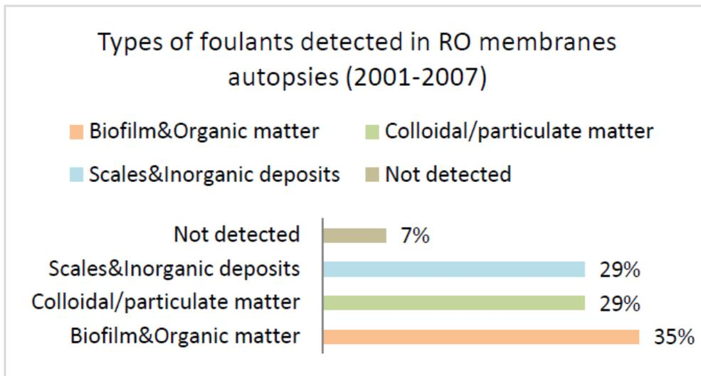
**Figure 1.1:** Types of foulants in RO membranes
