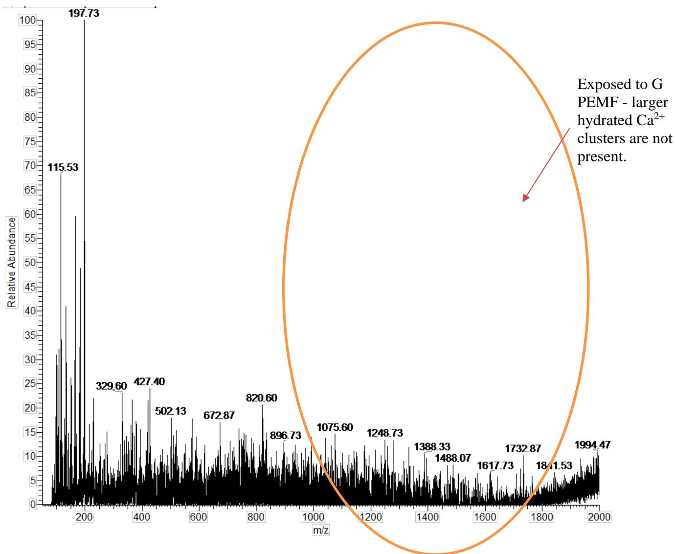
**Figure 5.8:** Electrospray spectrum of  $\text{Ca}(\text{NO}_3)_2$  solution exposed to Device G for 10 minutes in positive ion mode. Larger clusters appear to have been broken up by the PEMF.
