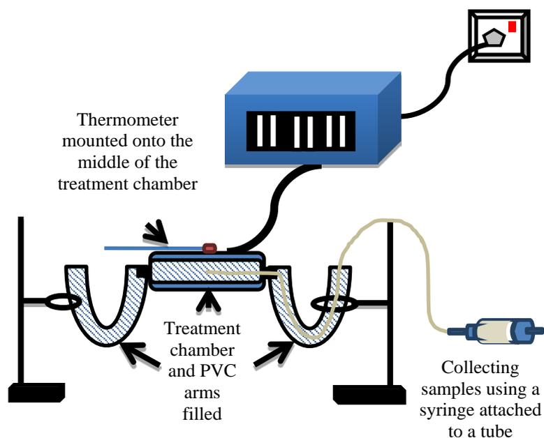
**Figure 3.6:** Schematic of sampling with the system flooded with test solution.
