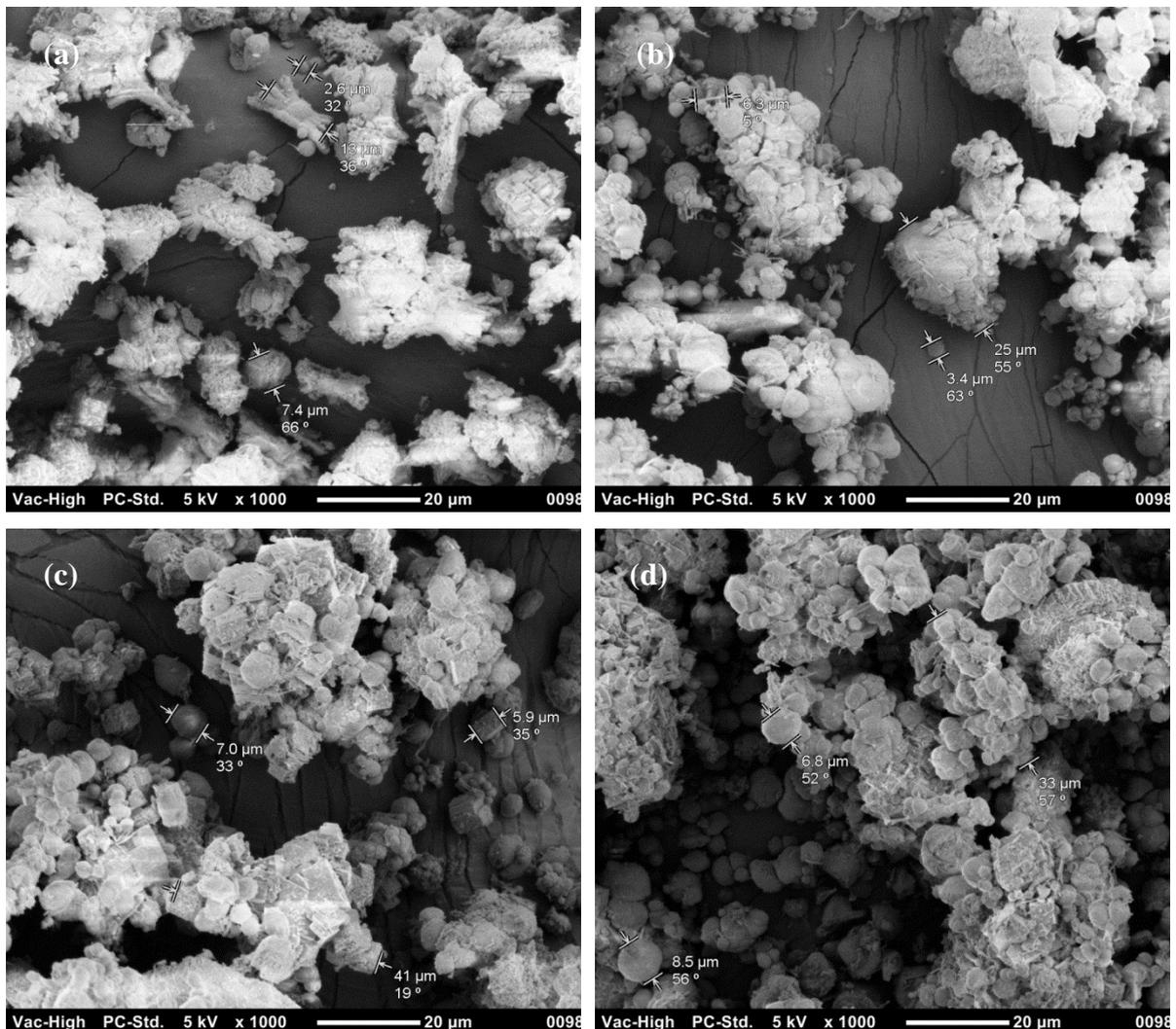
**Figure 5.1:** SEM images of dried precipitate mixtures of pre-exposed (30 min)  $\text{Na}_2\text{CO}_3$  mixed with un-exposed  $\text{Ca}(\text{NO}_3)_2 \cdot 4\text{H}_2\text{O}$  at room temperature, (a) Device D PEMF (b) Device D Control (c) Device G PEMF (d) Device G Control.
