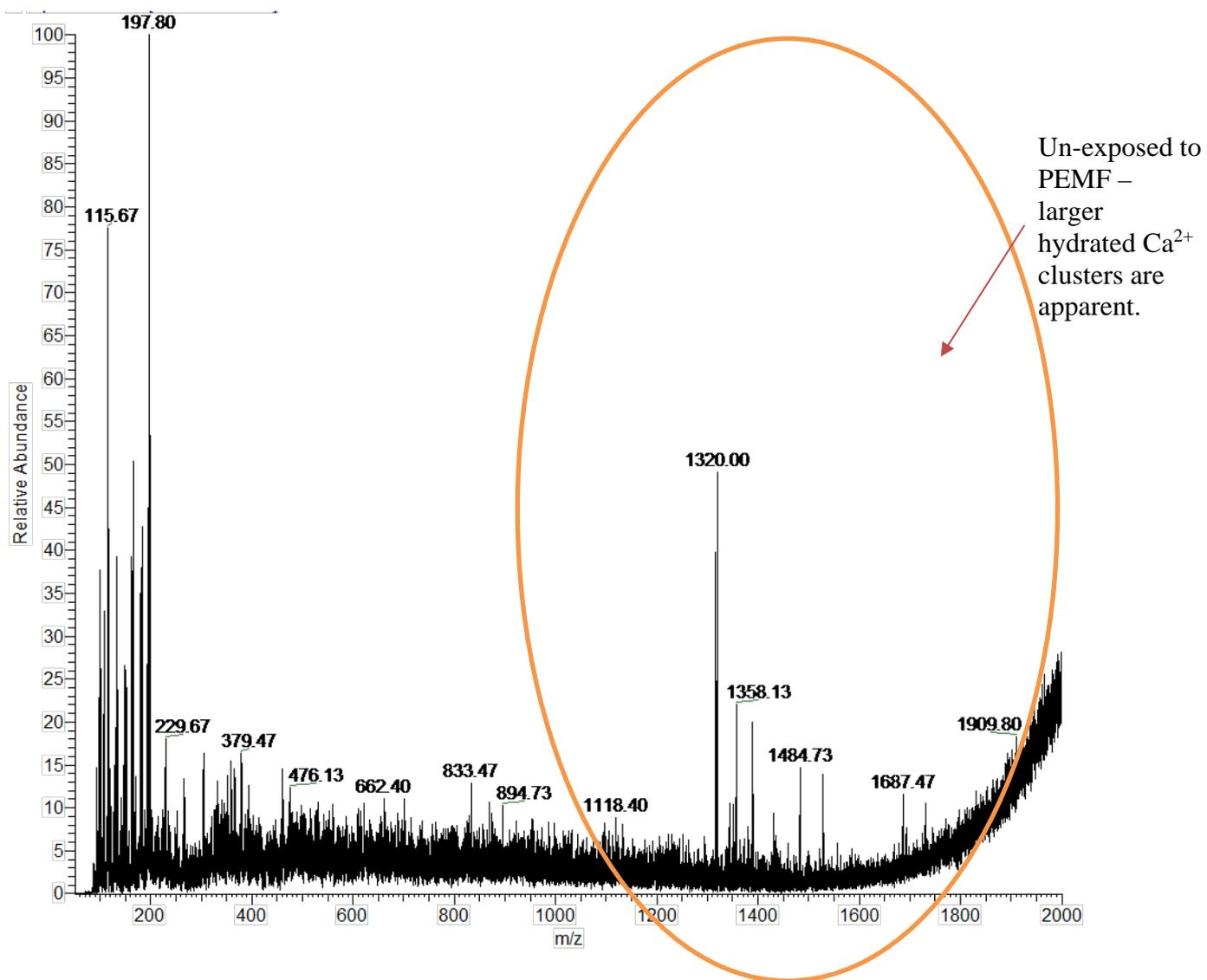
**Figure 5.6:** Electrospray spectrum of un-exposed  $\text{Ca}(\text{NO}_3)_2$  solution in positive ion mode.
