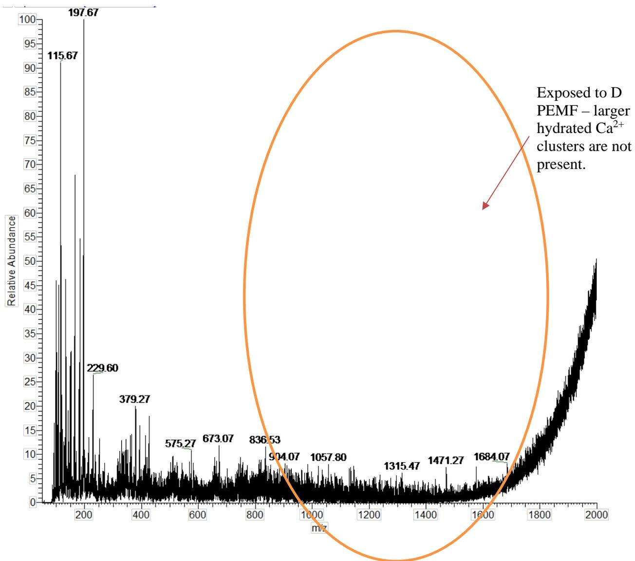
**Figure 5.7:** Electrospray spectrum of  $\text{Ca}(\text{NO}_3)_2$  solution exposed to Device D for 10 minutes in positive ion mode. Larger clusters appear to have been broken up by the PEMF.
