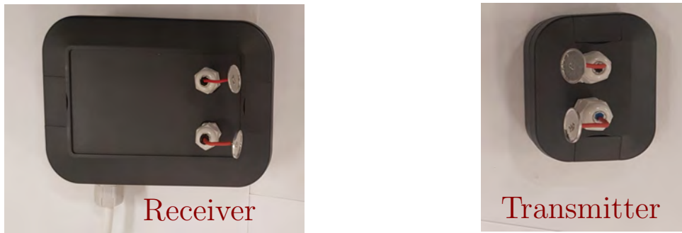
Fig. 6.2 Water proof IP67 encased receiver (left) and transmitter (right)
