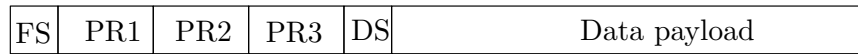
Fig. 5.2 transmitted packet structure. Here FS denotes the frame start followed by the consecutive preamble sequences denoted by PR1, PR2 and PR3. The data start sequence is denoted by DS followed by the transmitted payload.
