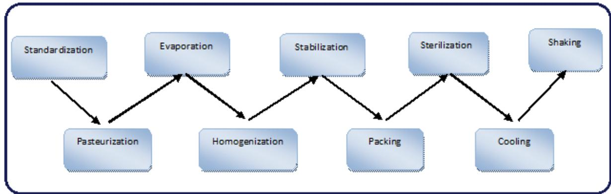
Figure 2.3: Manufacturing process of concentrated milk (based on Deeth and Lewis, 2016)
