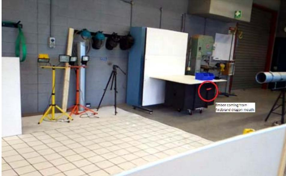
Figure 16: One of the firebrand coming from the firebrand dragon. Due to very fast movement of firebrand attempt to capture a still image was very hard
