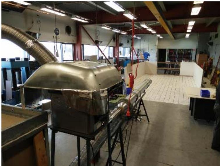
Figure 15: Firebrand dragon constructed at our facility to generate repeatable uniform firebrand shower.
